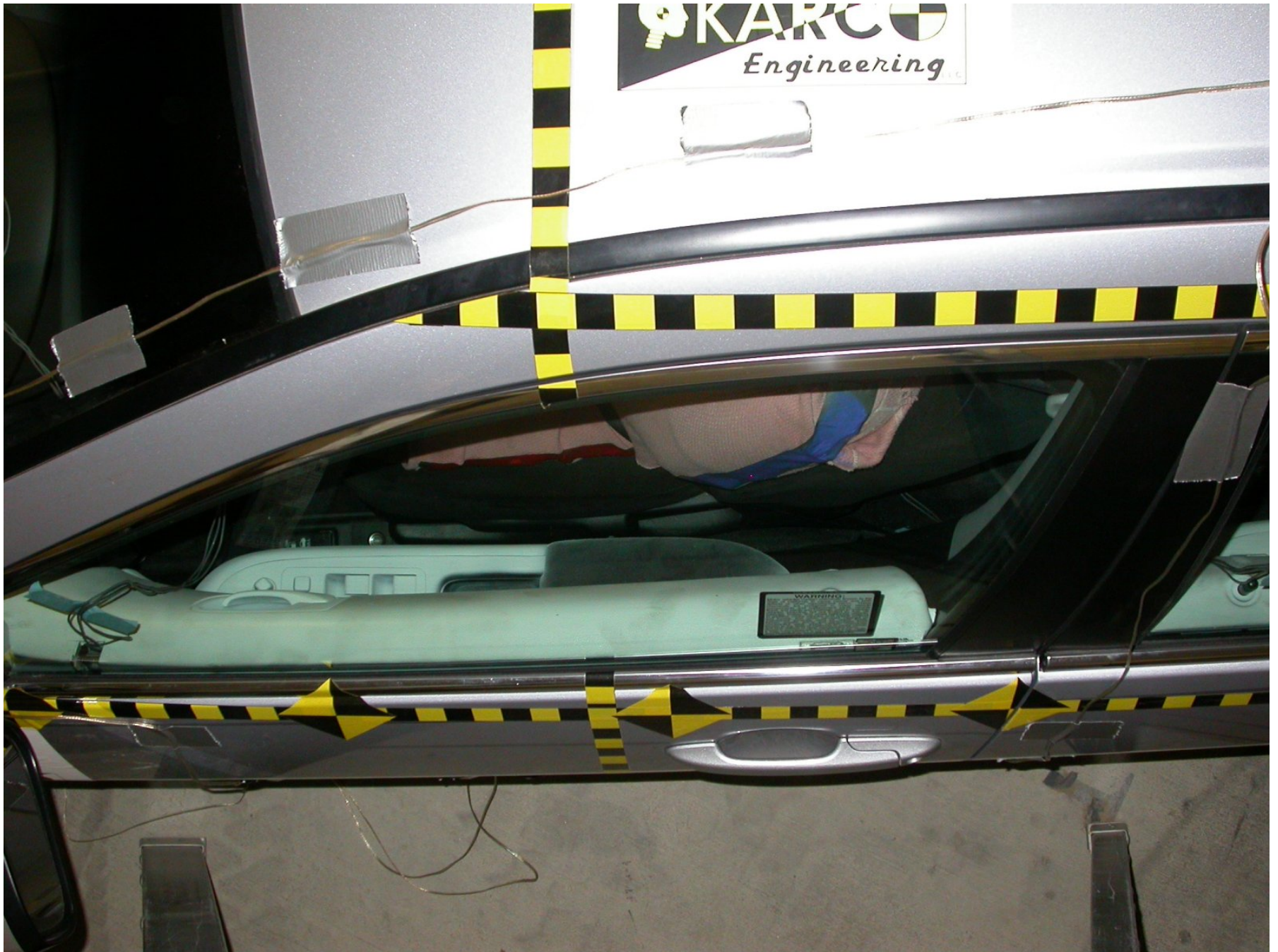
Figure A-32: Driver Dummy Clearance, Pre-Test
