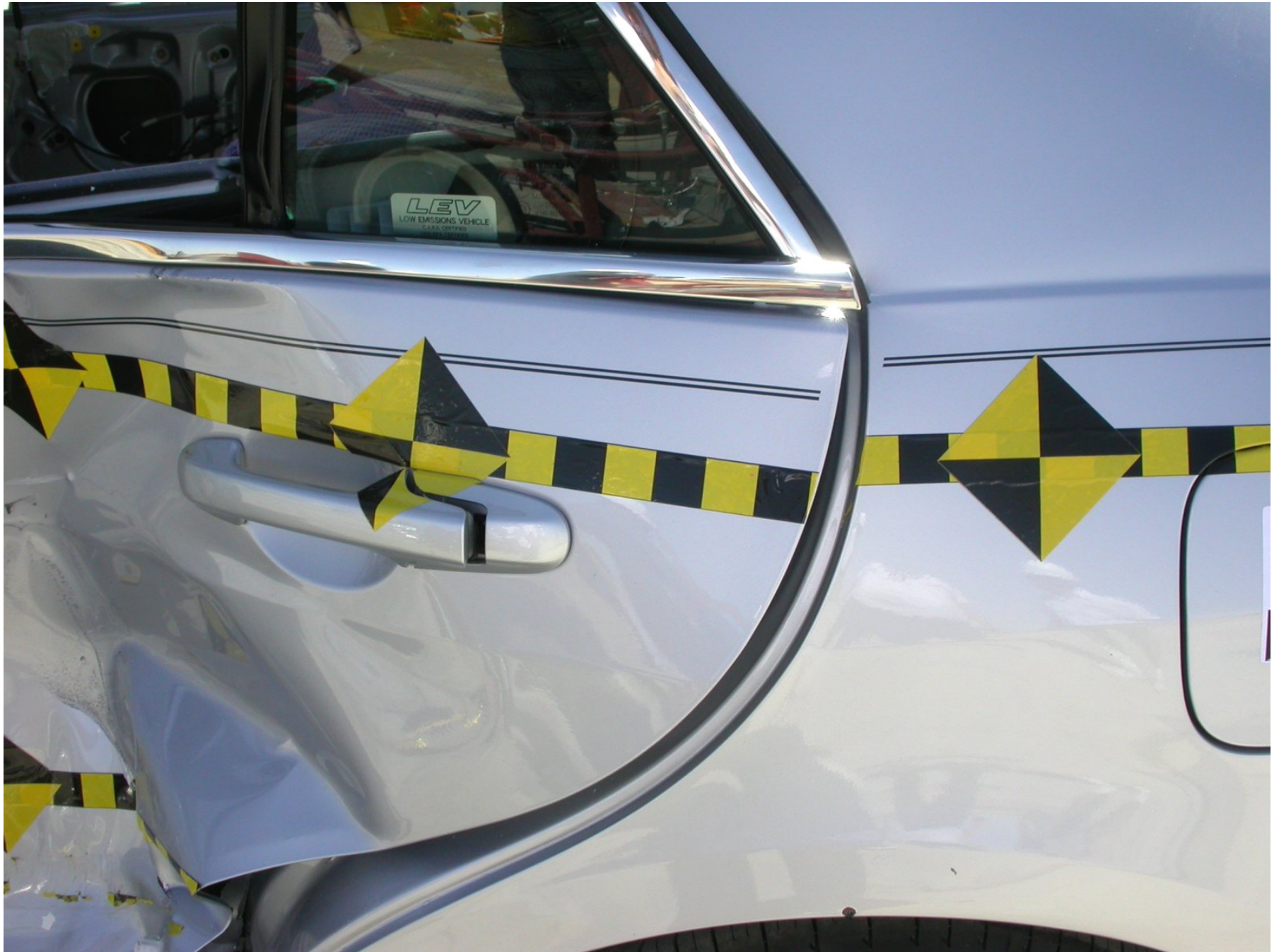
Figure A-28: Left Rear Door Closed, Post-Test
