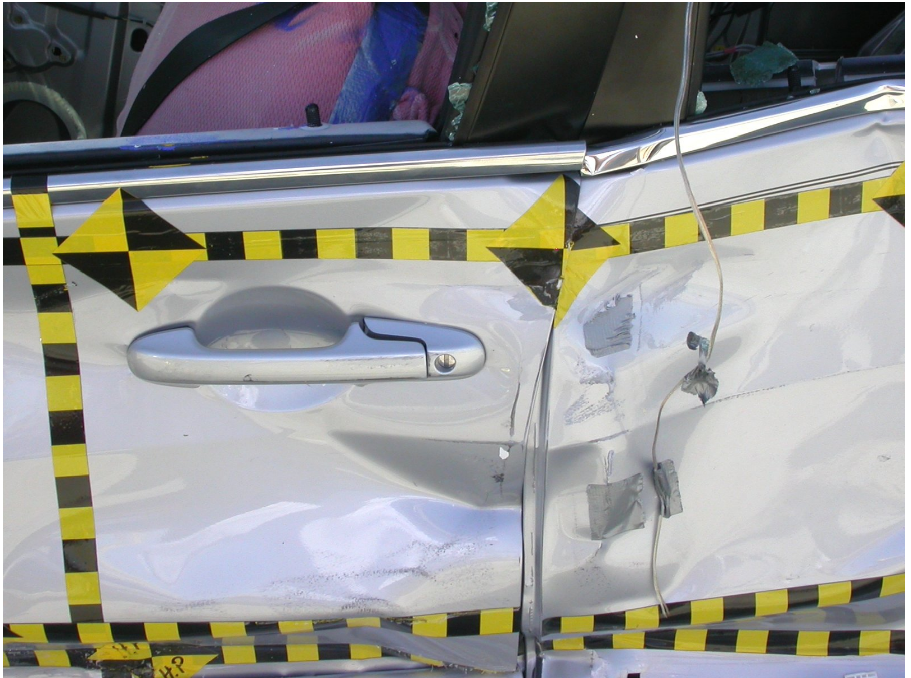
Figure A-26: Left Front Door Closed, Post-Test
