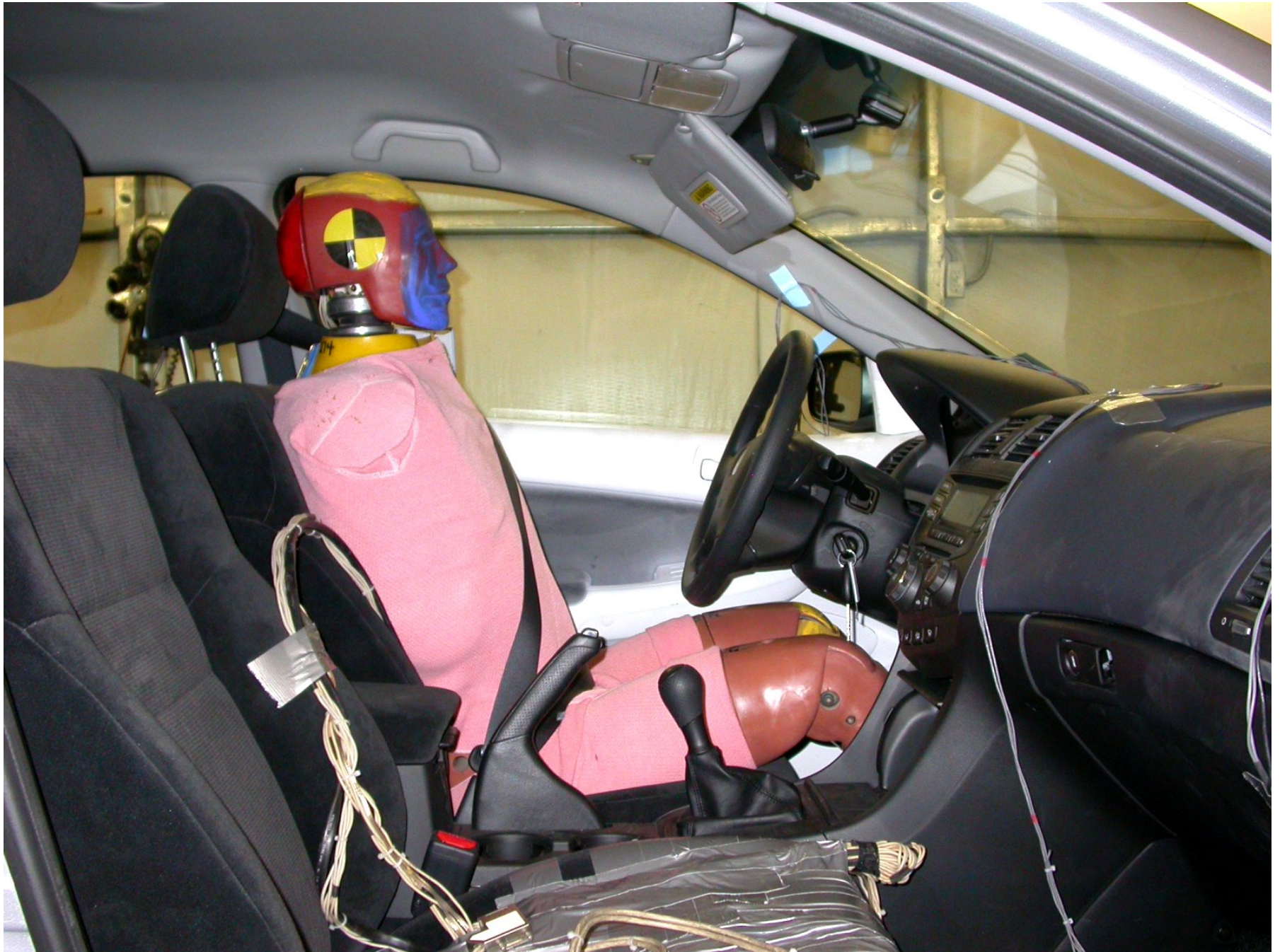
Figure A-34: Driver Dummy Inside View, Pre-Test
