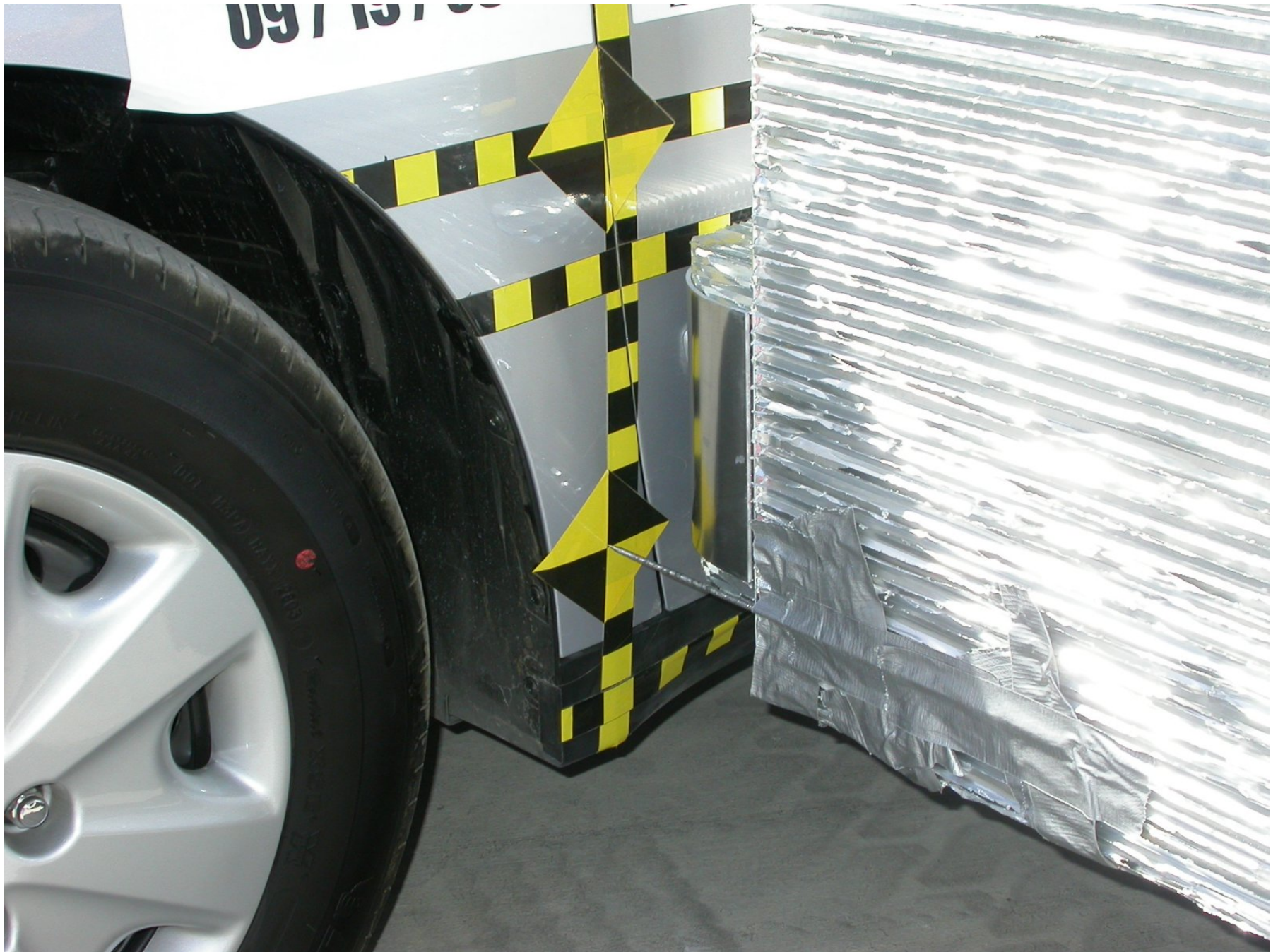
Figure A-19: Impact Point Target Set-up, Pre-Test
