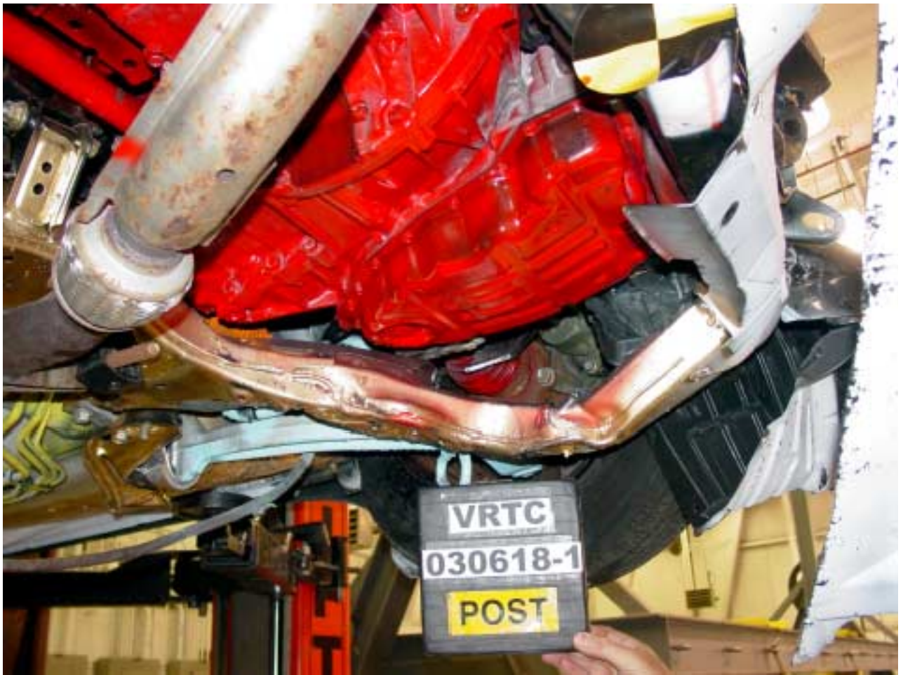
Figure A-82 Post-Test Vehicle Sub-Frame Damage - View 3
