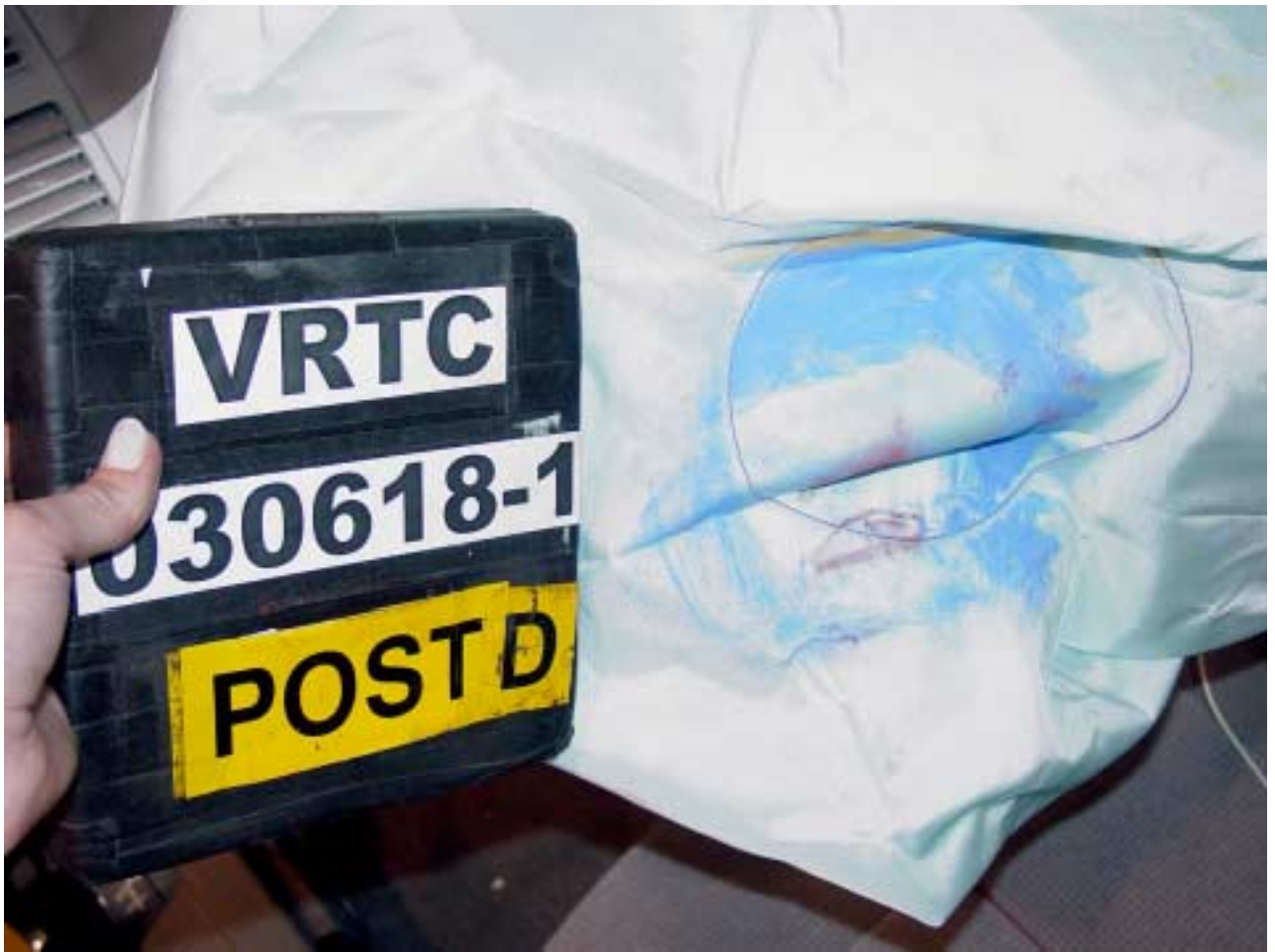
Figure A-66 Post-Test Driver Dummy Head Contact - View 2
