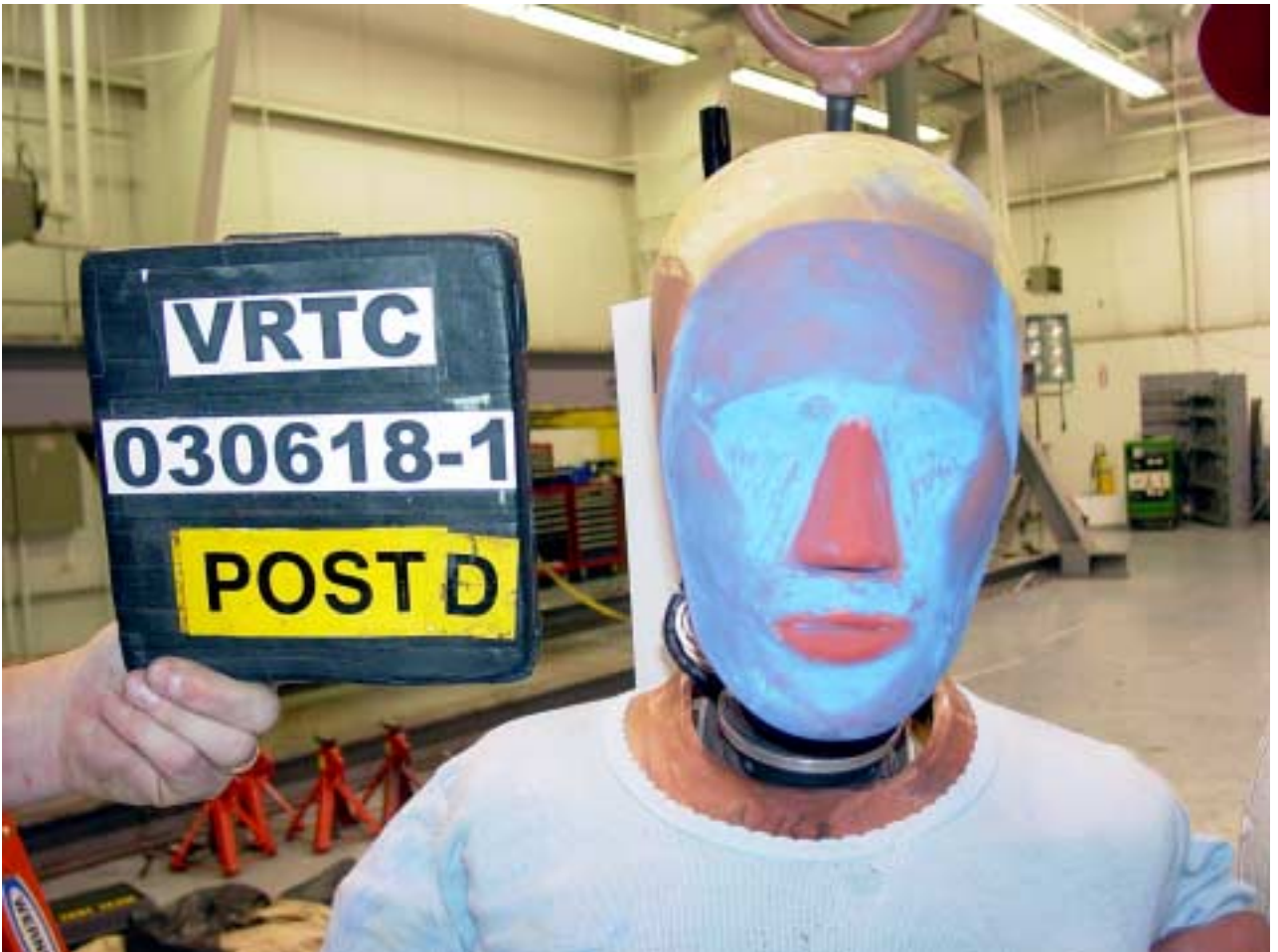
Figure A-65 Post-Test Driver Dummy Head Contact - View 1
