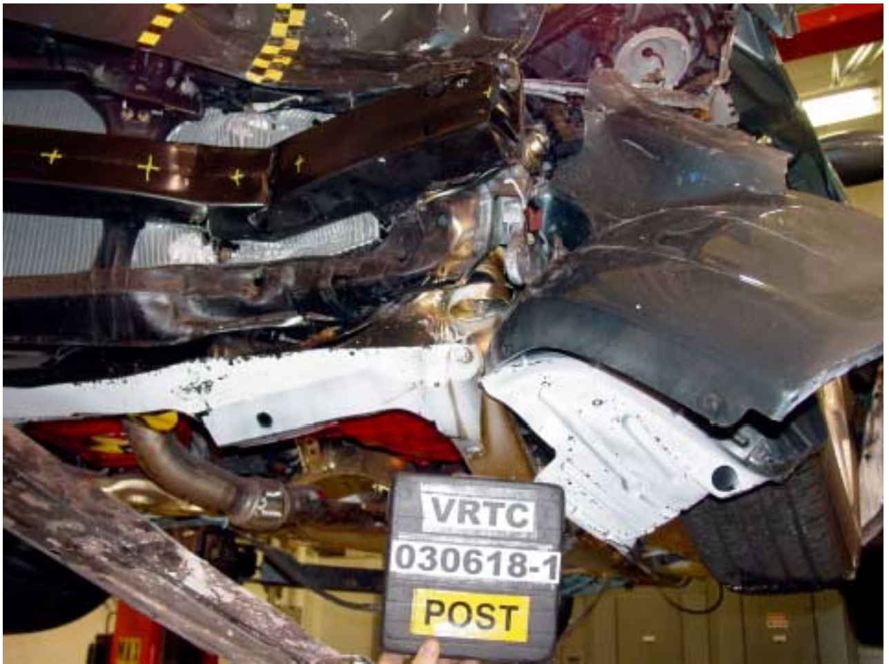
Figure A-76 Post-Test Bumper to Rail Attachment View
