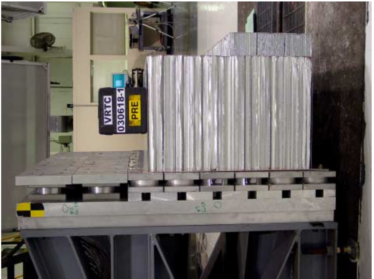
Figure A-42 Pre-Test Right Side Barrier Face View
