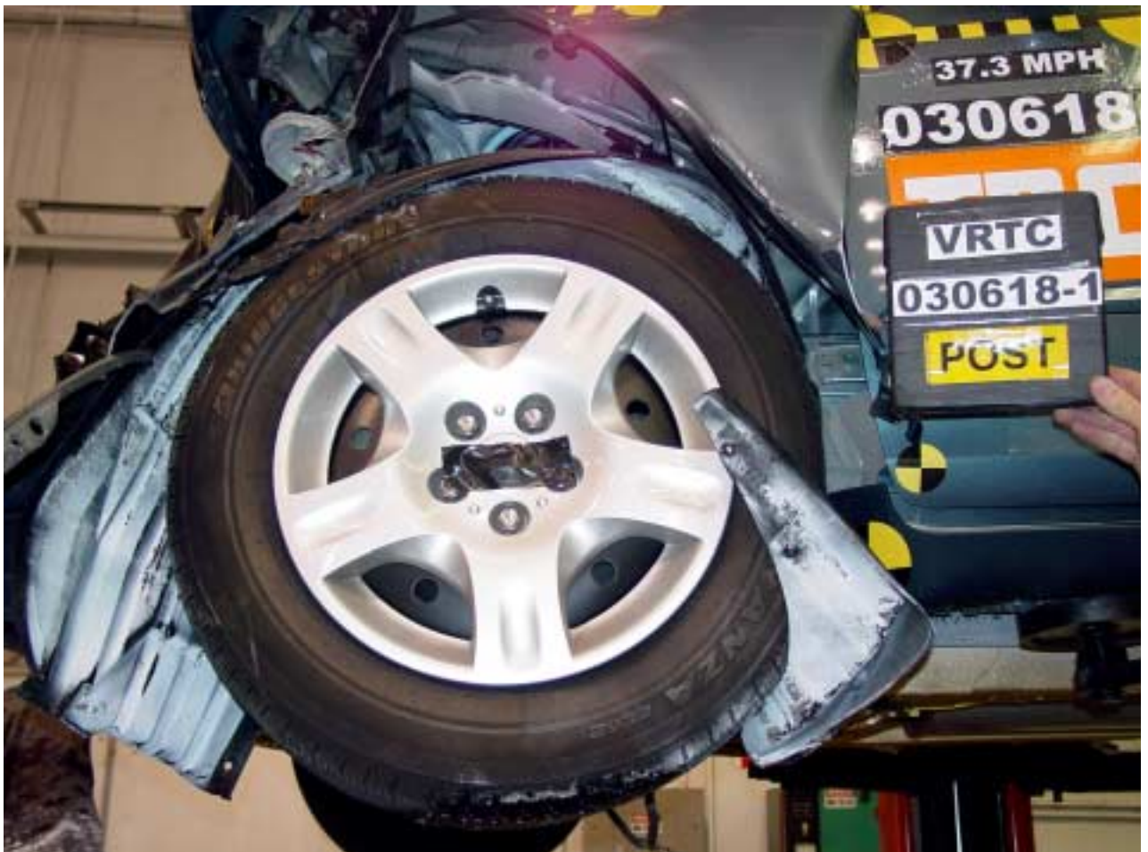
Figure A-77 Post-Test Wheel/Tire Deformation View
