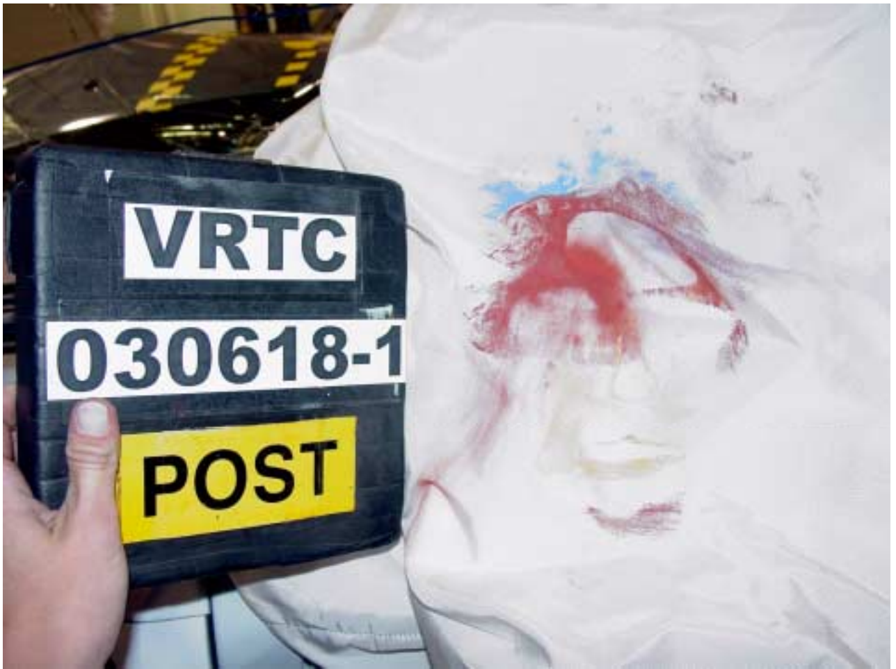
Figure A-72 Post-Test Passenger Dummy Head Contact - View 2
