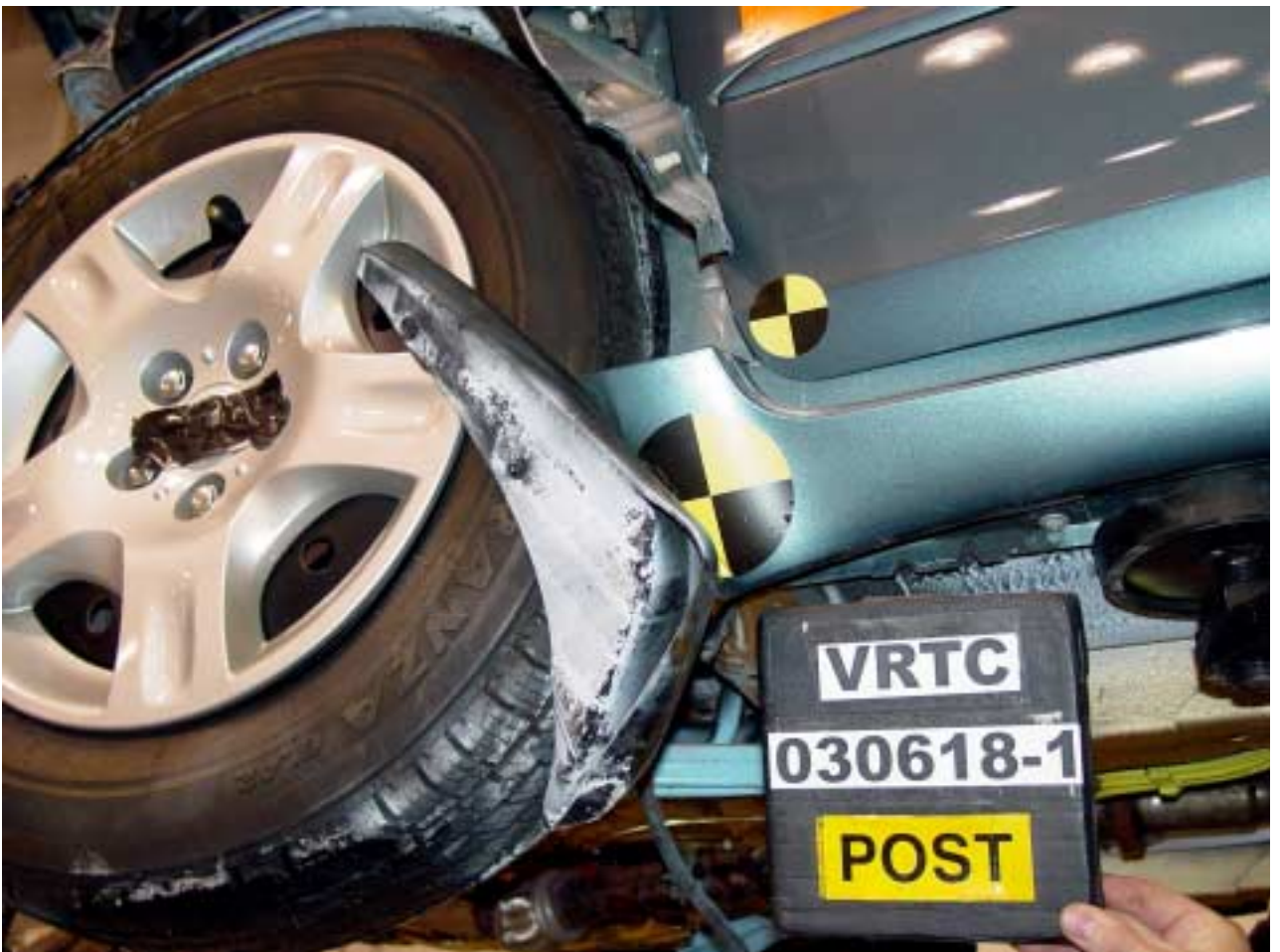
Figure A-79 Post-Test Wheel to Rocker Contact View
