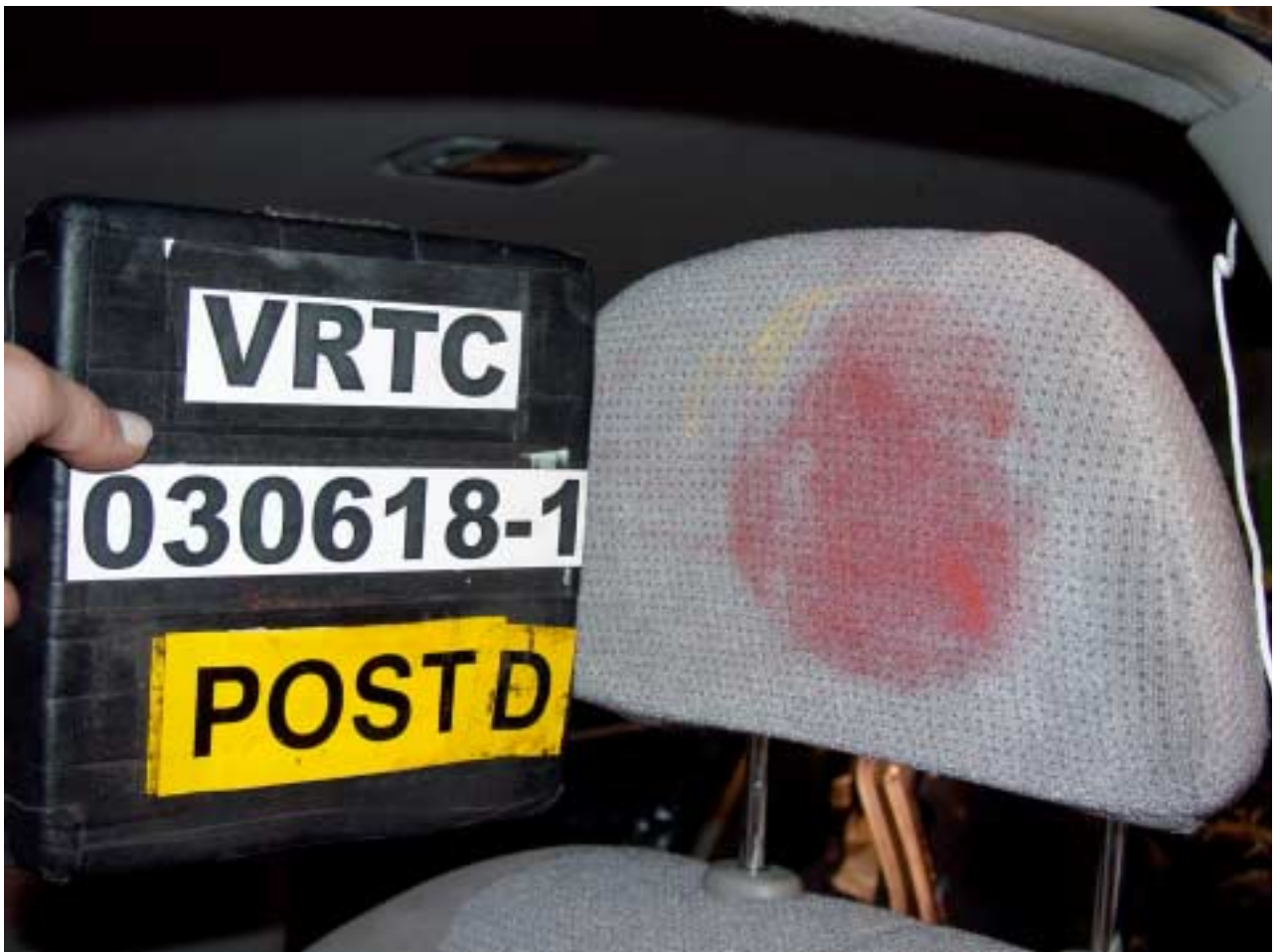
Figure A-67 Post-Test Driver Dummy Head Contact - View 3
