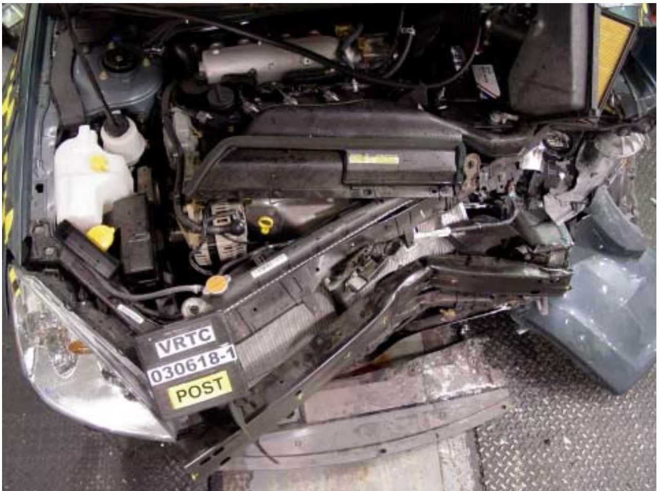
Figure A-85 Post-Test Bumper Damage View
