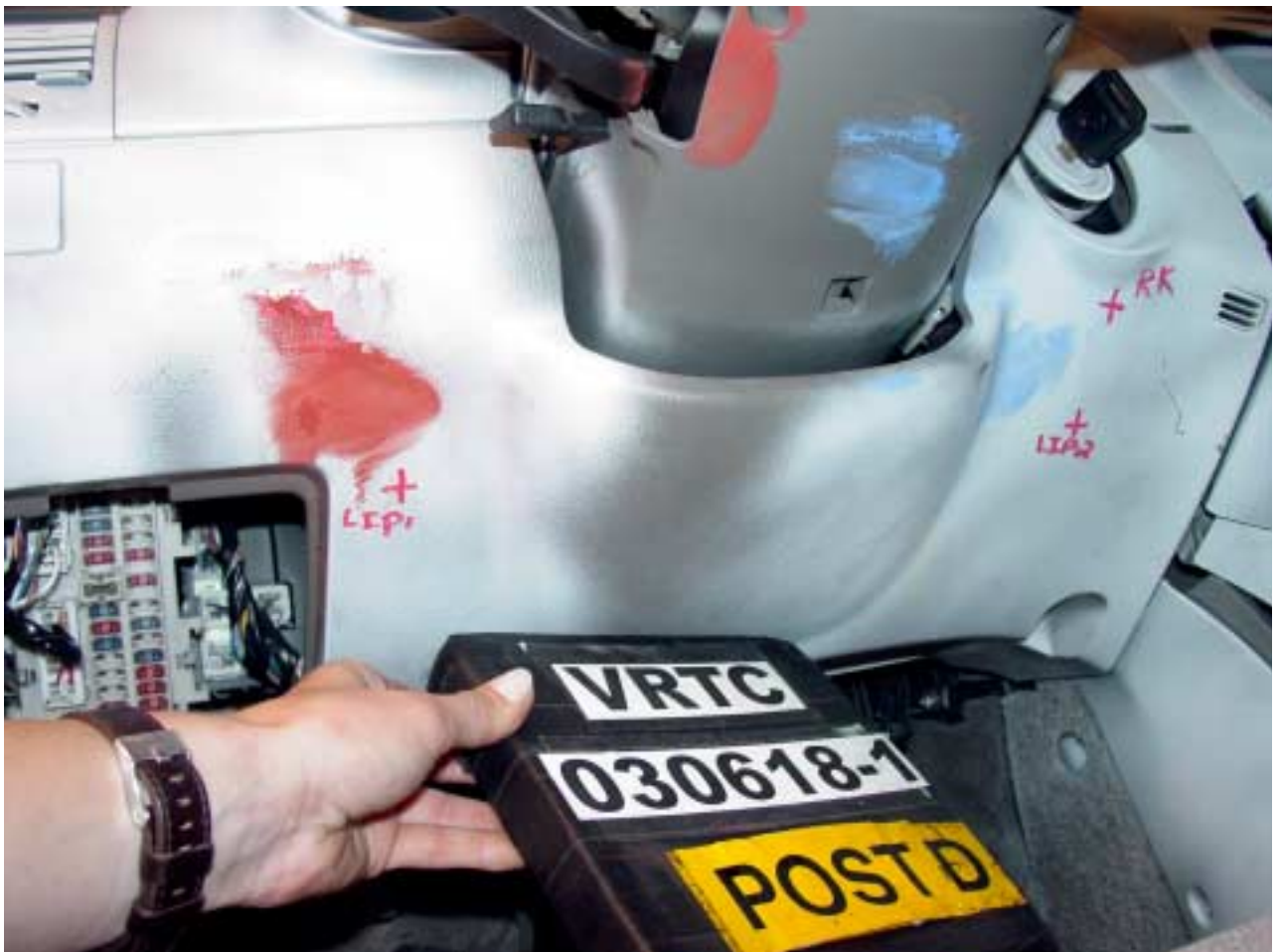
Figure A-69 Post-Test Driver Knee Contact - View 2
