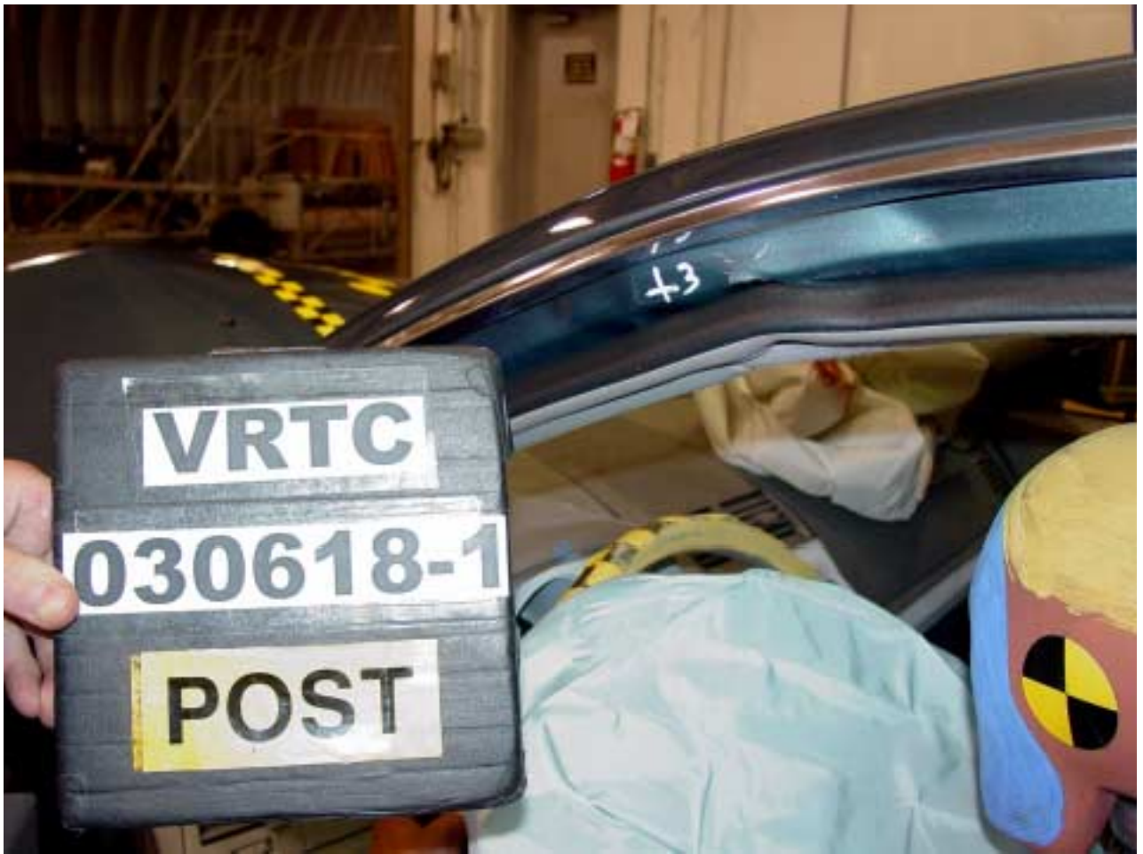
Figure A-84 Post-Test Vehicle Roof Deformation - View 2
