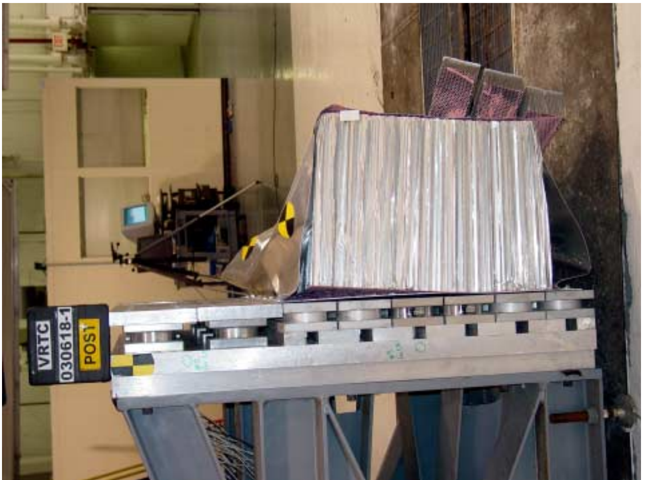
Figure A-43 Post-Test Right Side Barrier Face View
