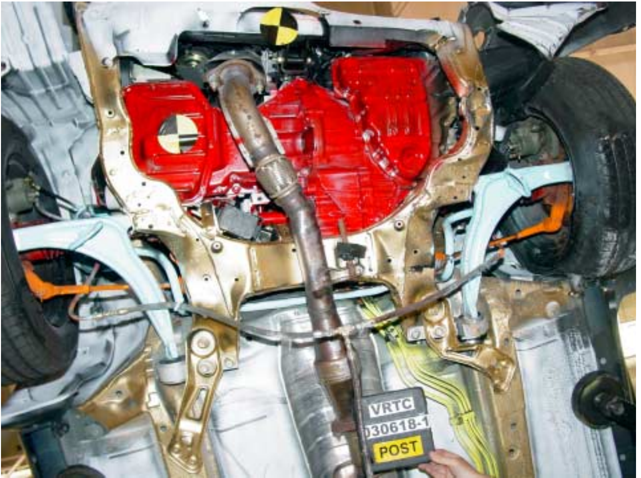
Figure A-80 Post-Test Vehicle Sub-Frame Damage - View 1
