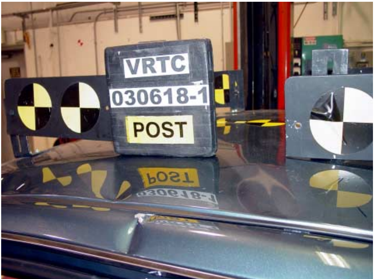
Figure A-83 Post-Test Vehicle Roof Deformation - View 1
