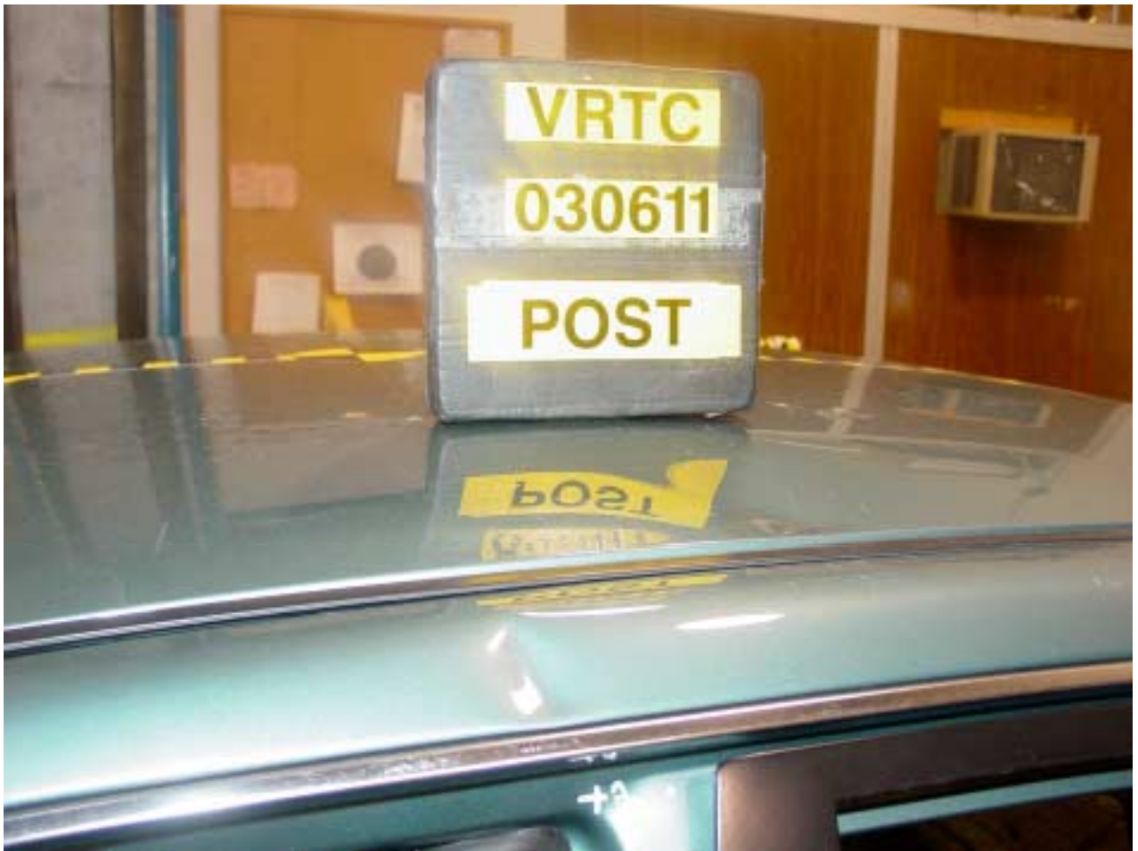
Figure A-81 Post-Test Vehicle Roof Deformation - View 2
