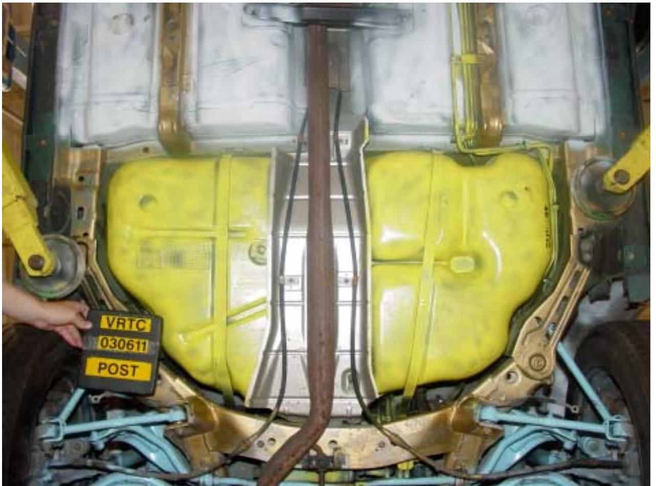
Figure A-24 Post-Test Rear Mid Underbody View
