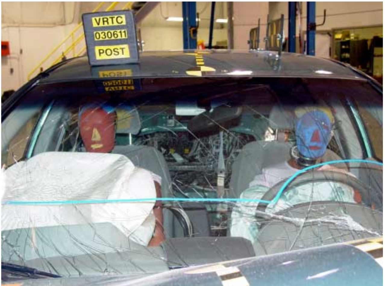
Figure A-44 Post-Test Driver and Passenger Dummies Front View
