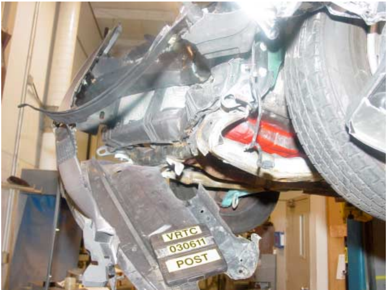
Figure A-75 Post-Test Bumper to Rail Attachment View
