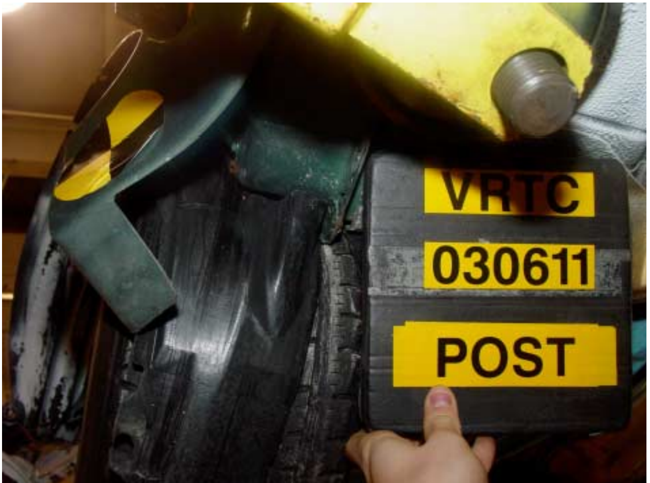
Figure A-76 Post-Test Wheel/Tire Deformation View
