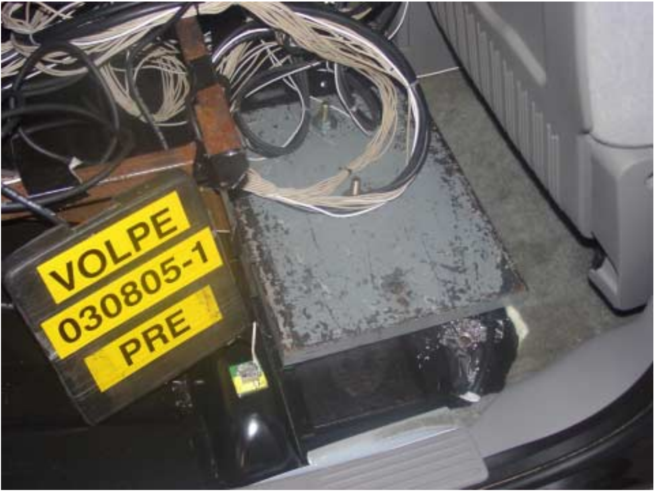
Figure A-65 Pre-Test Vehicle Ballast View
