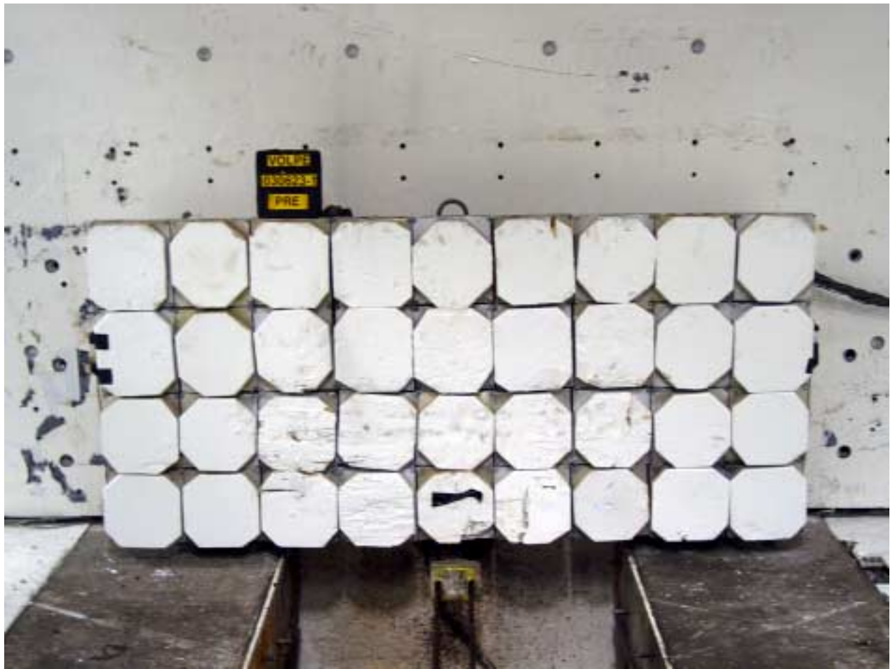
Figure A-77 Pre-Test Load Cell Barrier View
