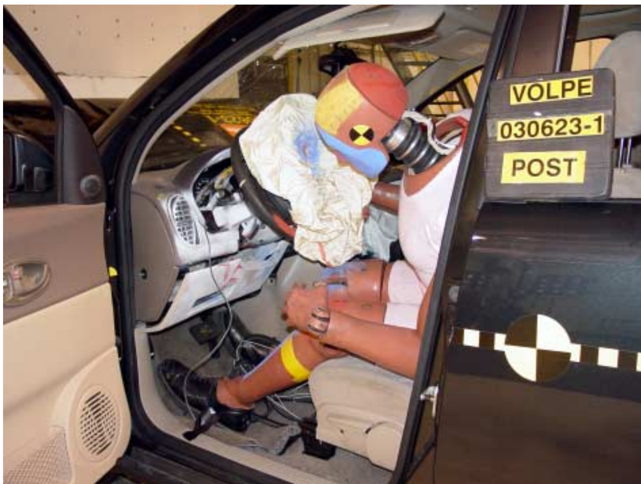
Figure A-44 Post-Test Driver Dummy & Vehicle Interior - View 2
