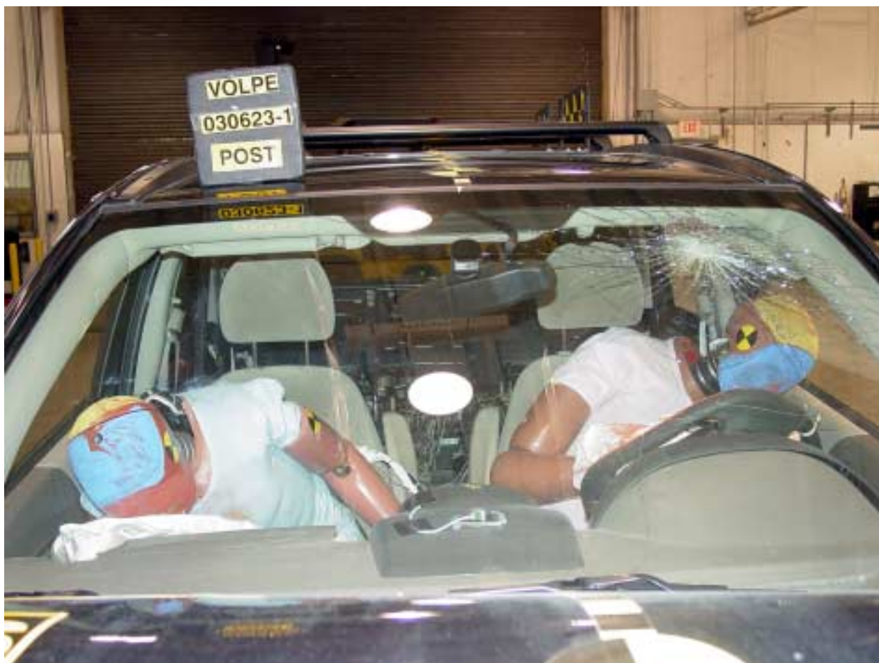
Figure A-36 Post-Test Driver and Passenger Dummies Front View
