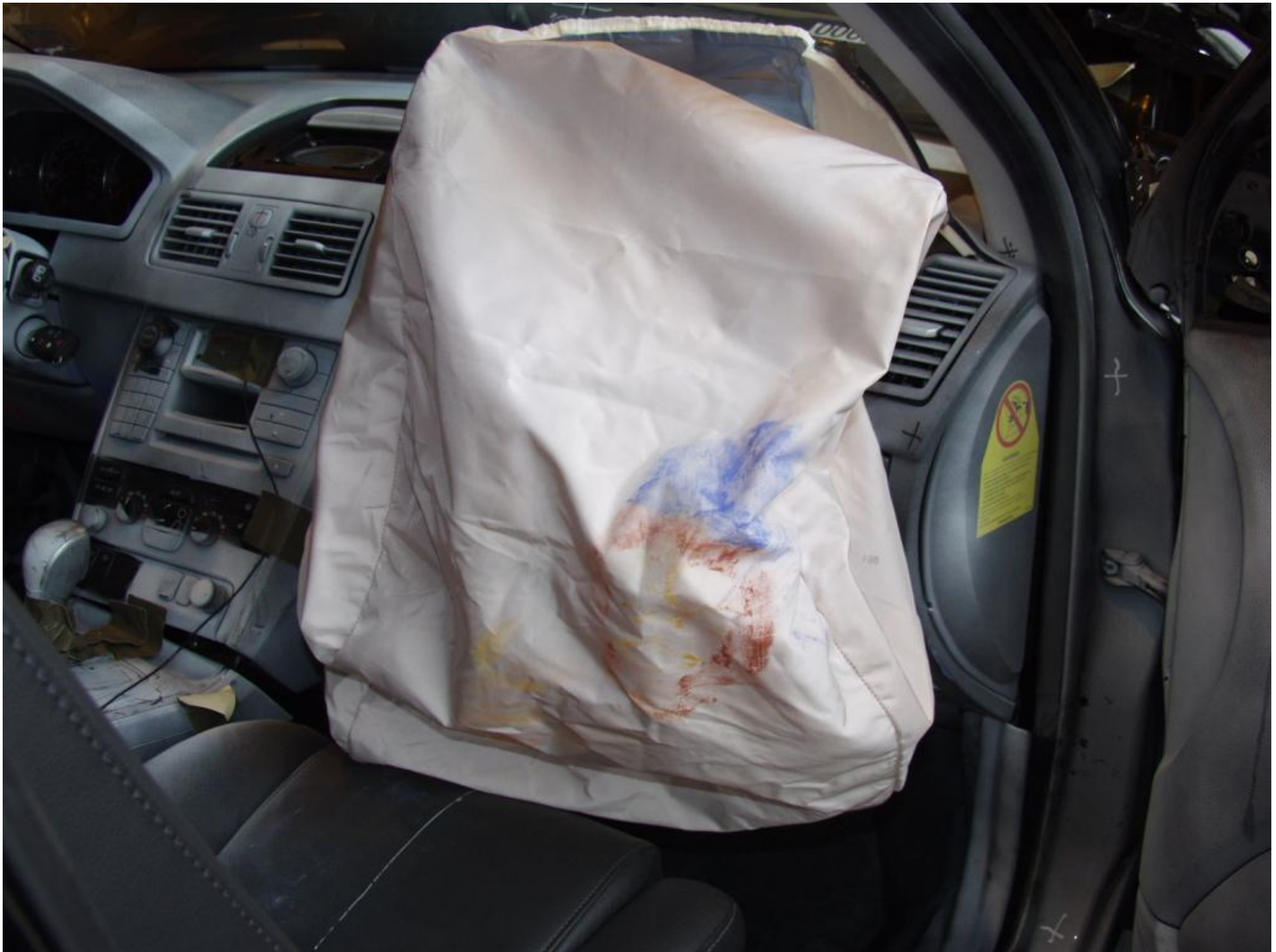
Figure A-57 POST-TEST PASSENGER CONTACT TO AIRBAG
