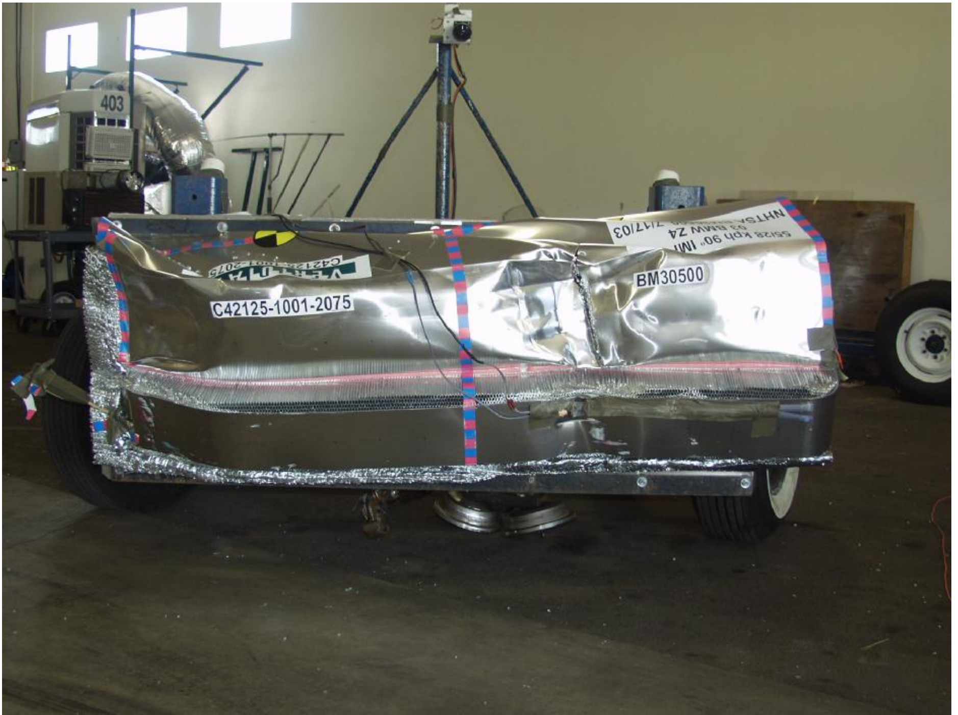
Figure A-16 POST-TEST FRONTAL VIEW OF IMPACTOR FACE
