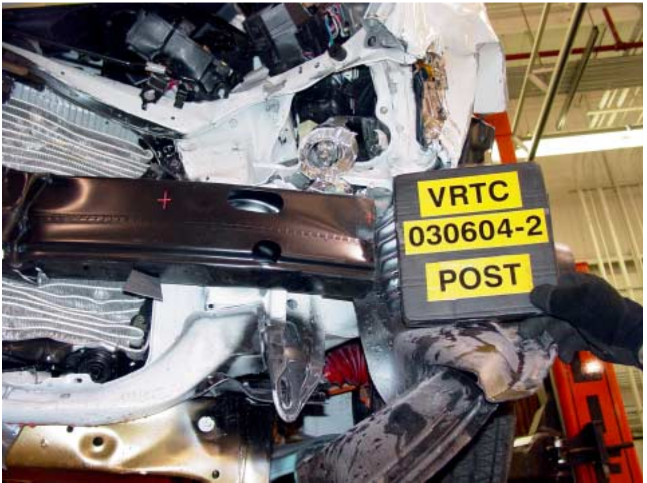
Figure A-79 Post-Test Bumper to Rail Attachment View
