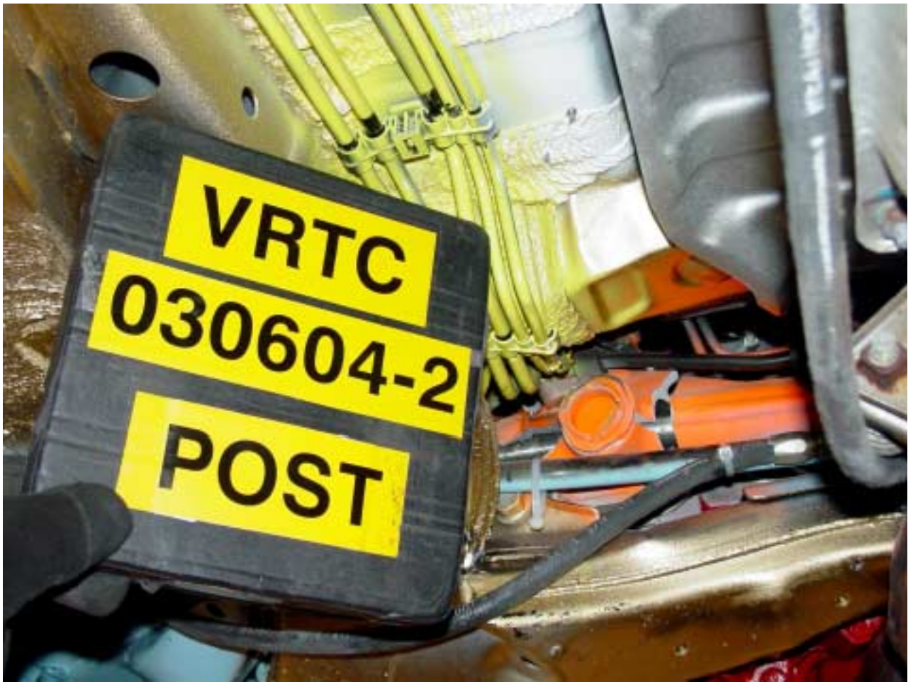
Figure A-89 Post-Test Vehicle Axle-Tube Damage View
