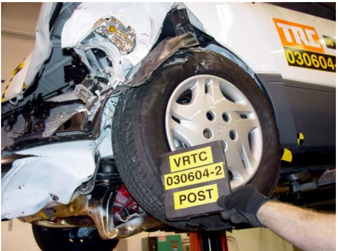
Figure A-80 Post-Test Wheel/Tire Deformation View
