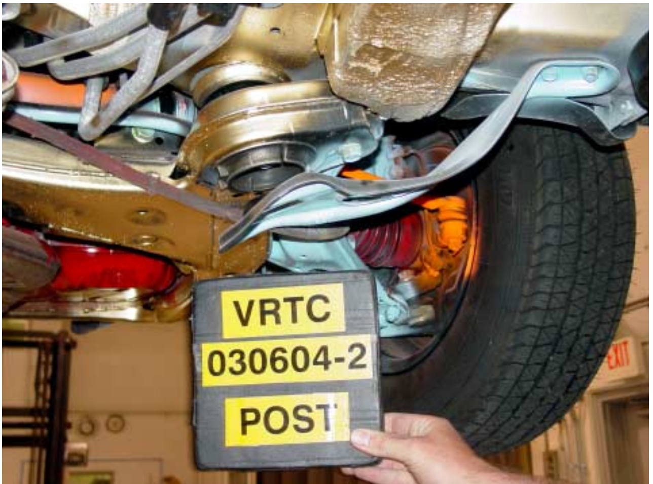
Figure A-86 Post-Test Vehicle Sub-Frame Damage - View 4
