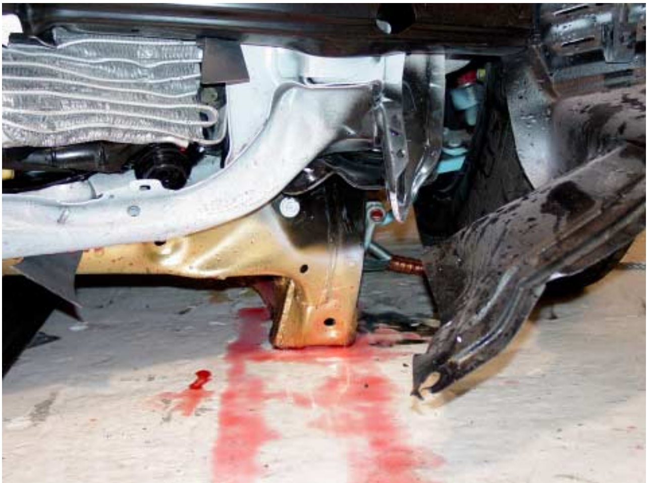
Figure A-84 Post-Test Vehicle Sub-Frame Damage - View 2
