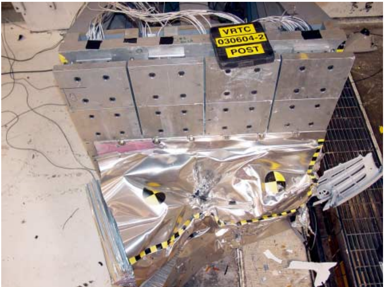
Figure A-48 Post-Test Overhead Barrier Face View
