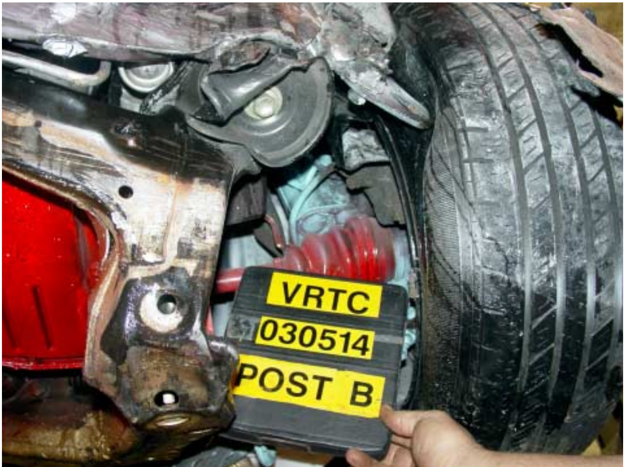
Figure A-123 Post-Test Bullet Vehicle Subframe Deformation - View 3
