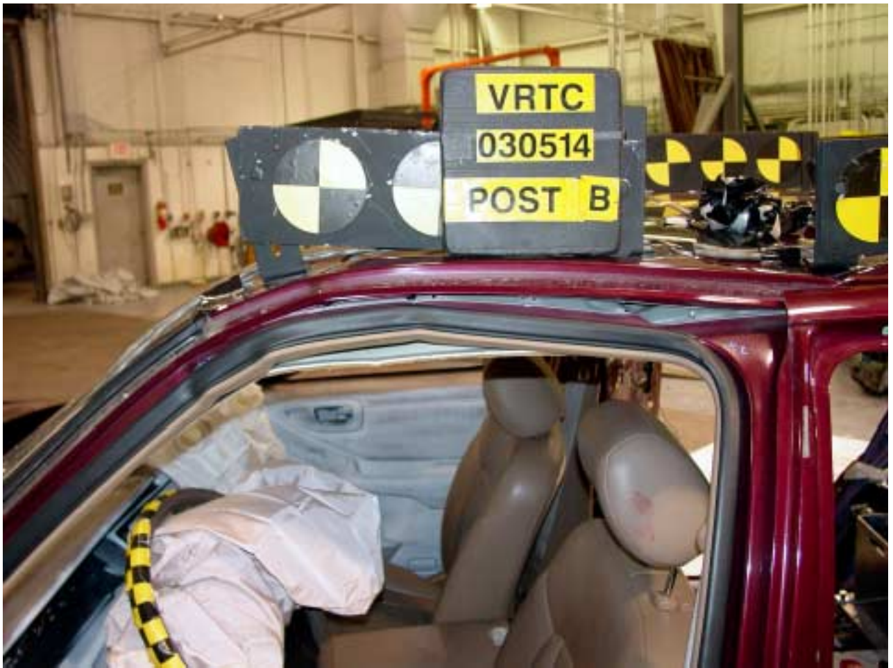
Figure A-117 Post-Test Bullet Vehicle Roof Deformation - View 1
