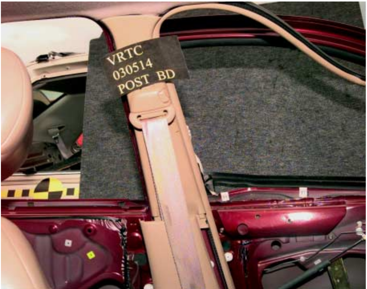
Figure A-98 Post-Test Bullet Vehicle Driver Dummy Head Contact – View 3
