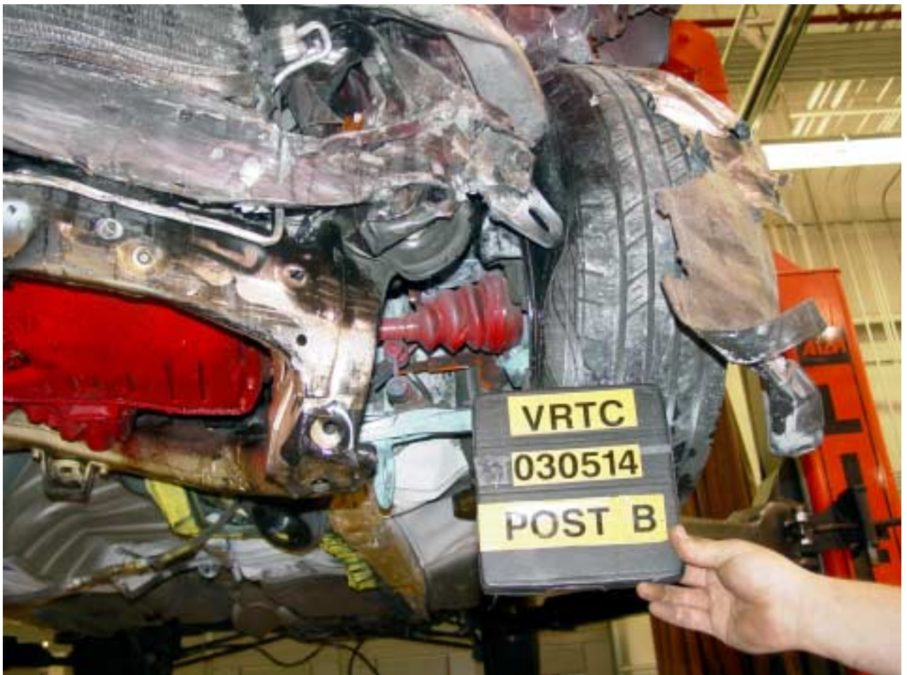
Figure A-128 Post-Test Bullet Vehicle Wheel Well View
