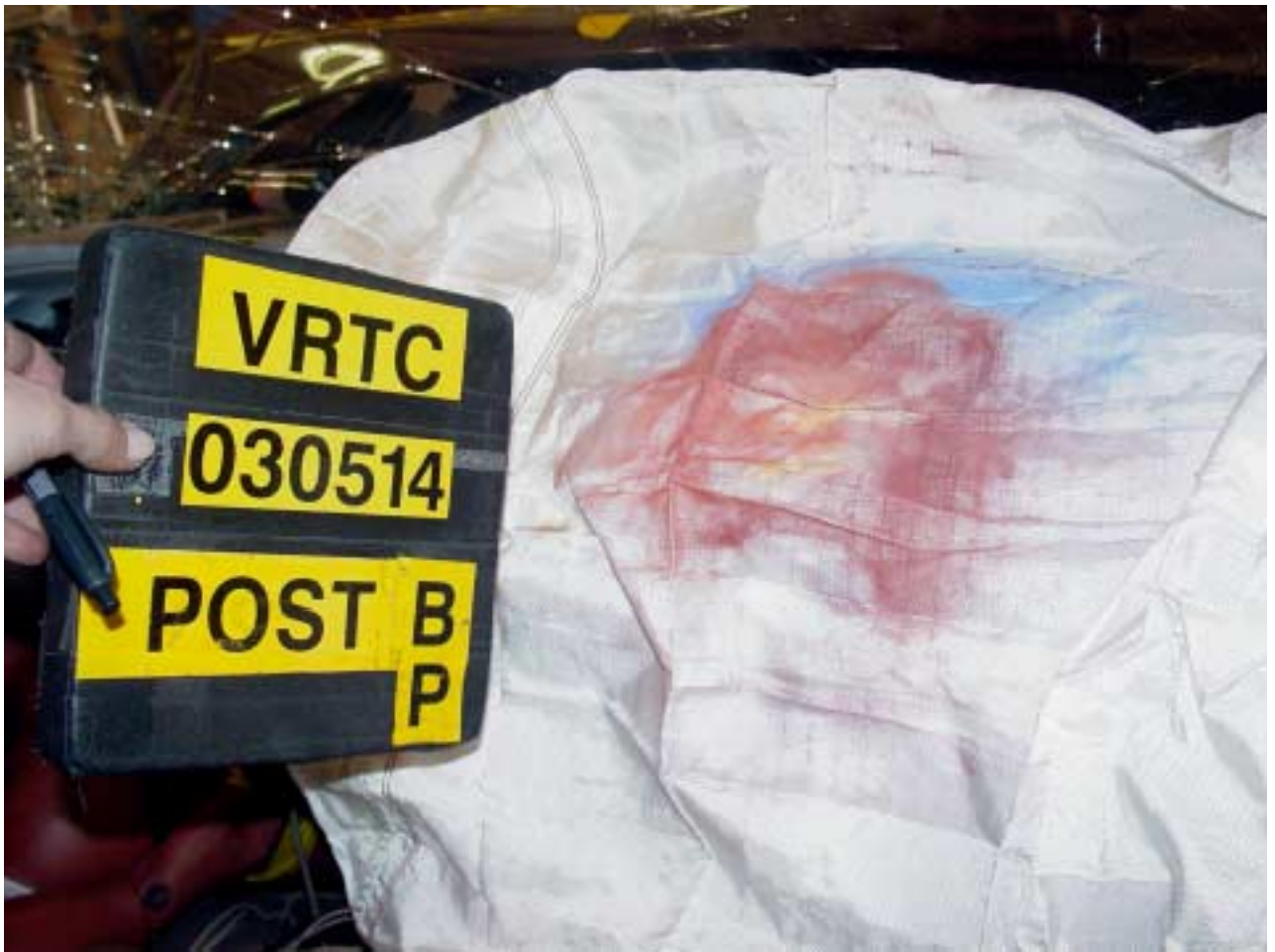
Figure A-104 Post-Test Bullet Vehicle Passenger Dummy Head Contact - View 2
