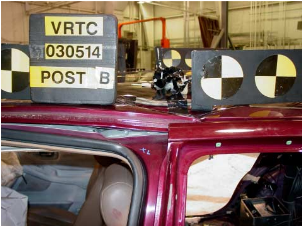
Figure A-118 Post-Test Bullet Vehicle Roof Deformation - View 2
