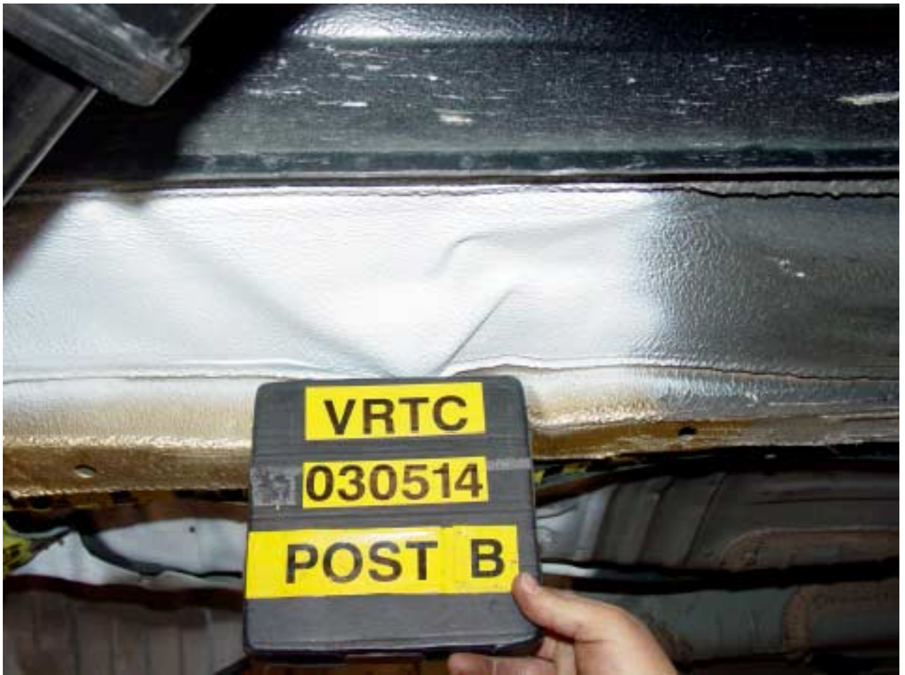
Figure A-125 Post-Test Bullet Vehicle Rail Deformation - View 1
