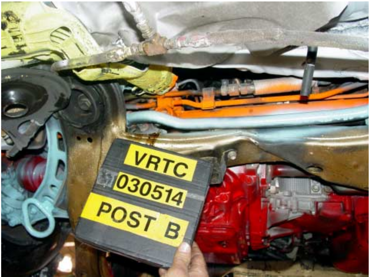
Figure A-121 Post-Test Bullet Vehicle Subframe Deformation - View 1
