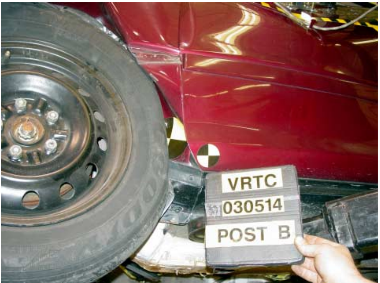
Figure A-124 Post-Test Bullet Vehicle Rocker Deformation View
