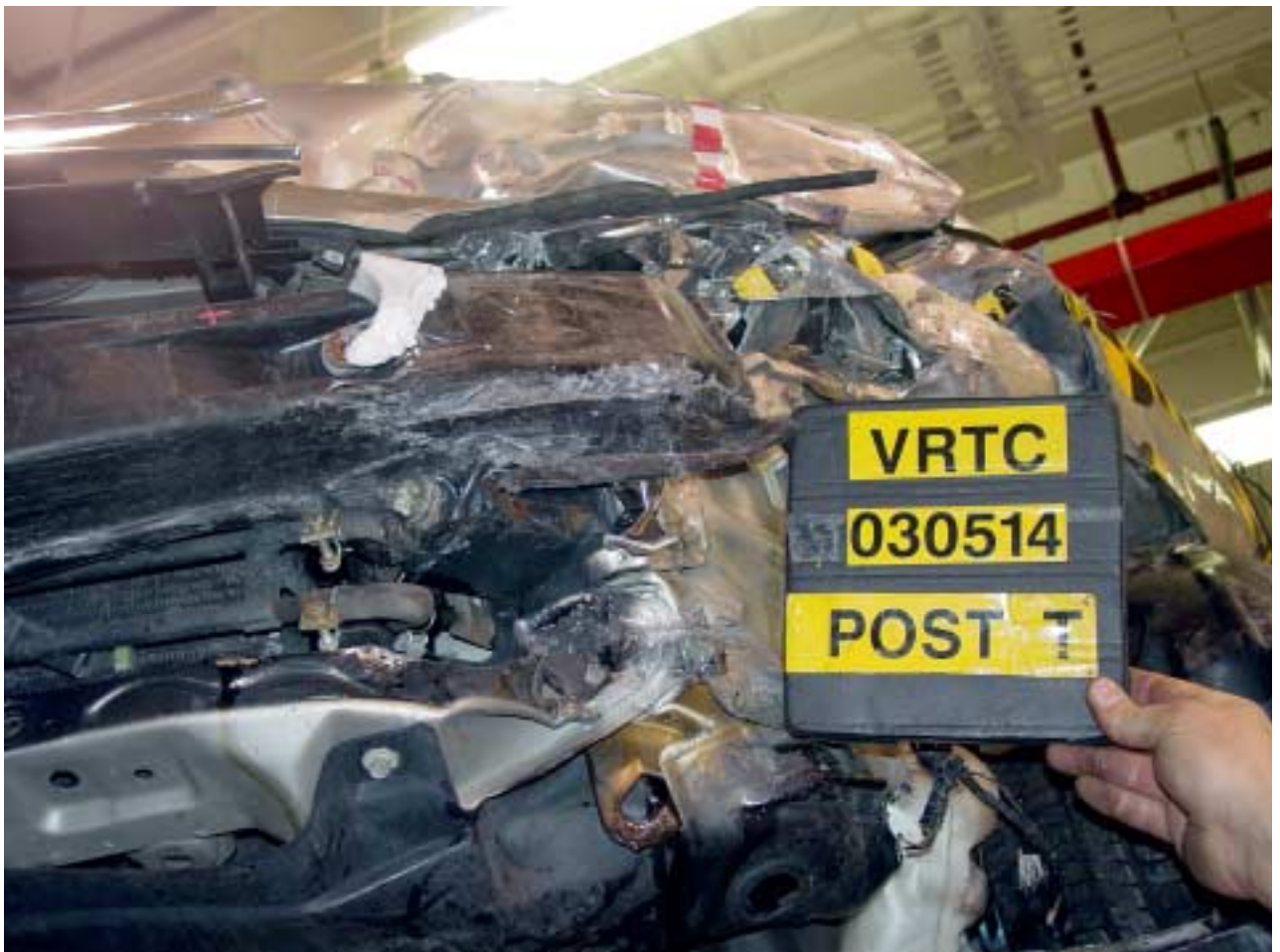
Figure A-113 Post-Test Target Vehicle Subframe Deformation View
