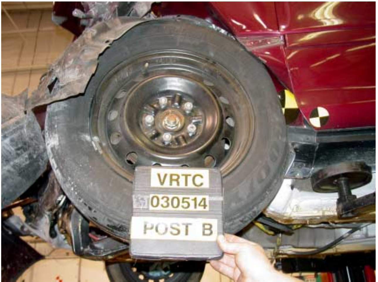
Figure A-127 Post-Test Bullet Vehicle Wheel Deformation View
