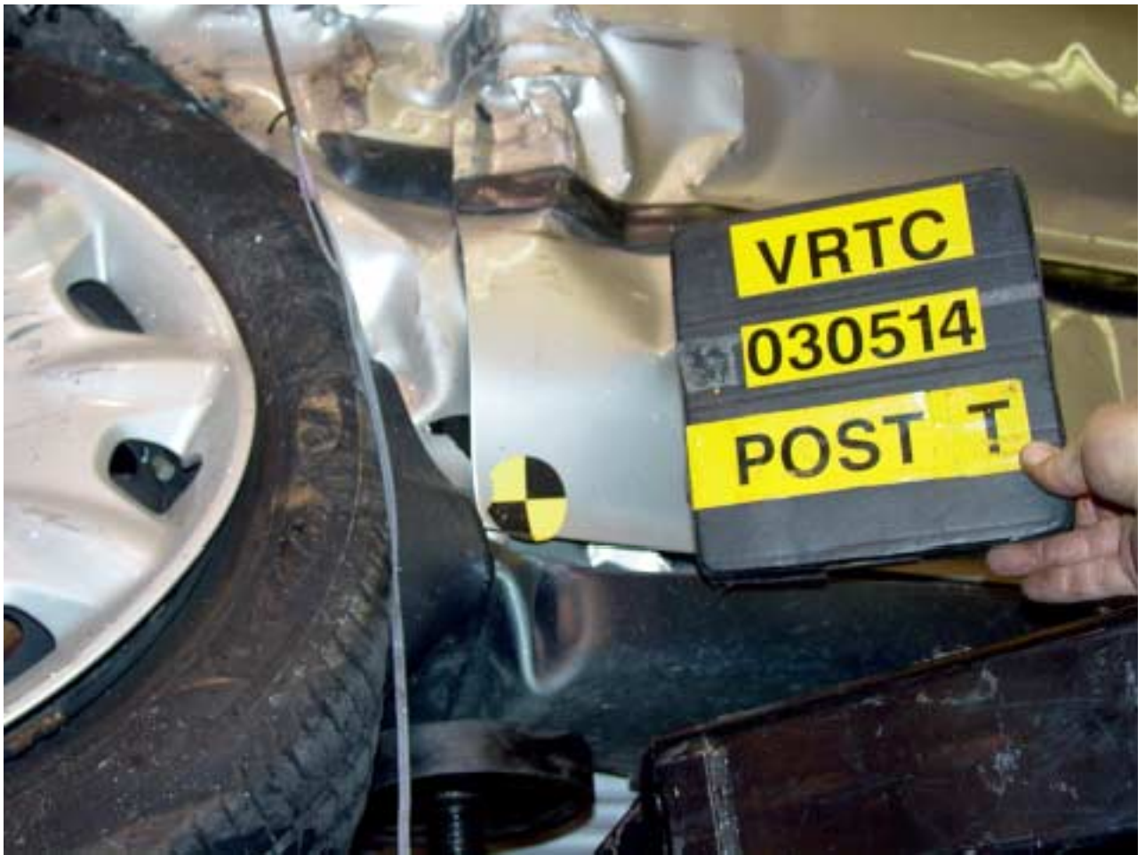
Figure A-112 Post-Test Target Vehicle Sill Deformation View
