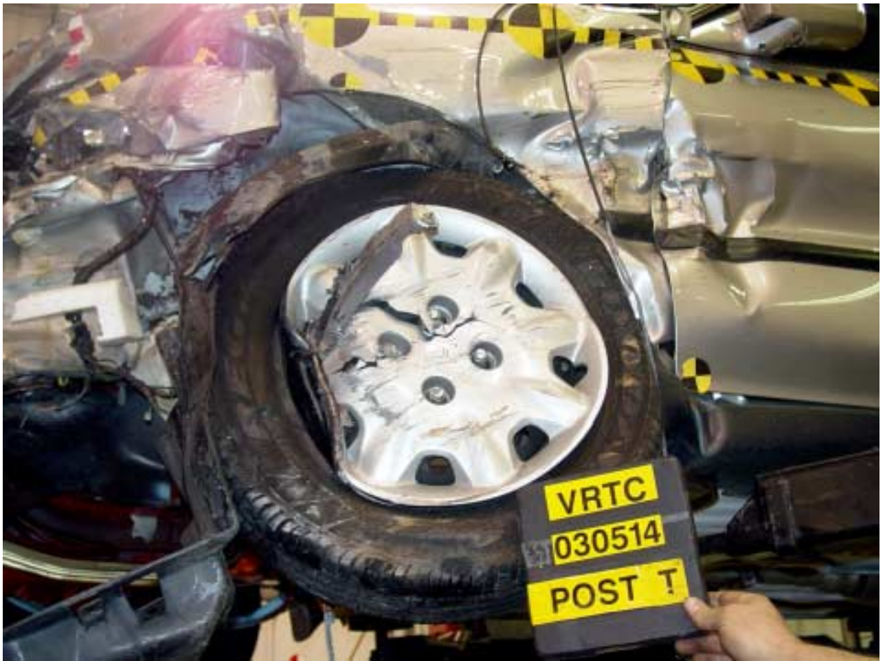
Figure A-114 Post-Test Target Vehicle Wheel Deformation View
