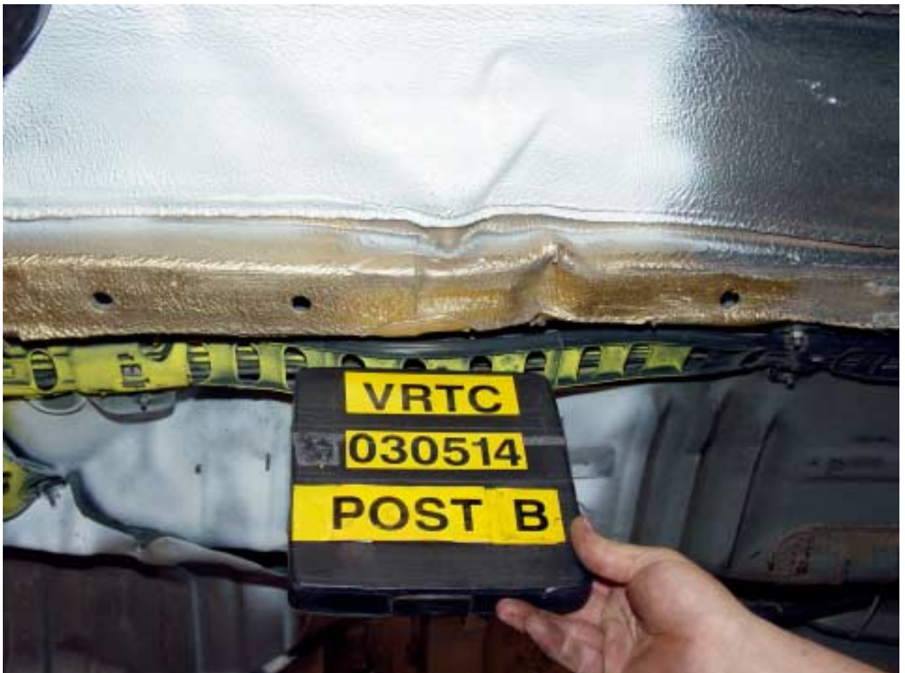
Figure A-126 Post-Test Bullet Vehicle Rail Deformation - View 2
