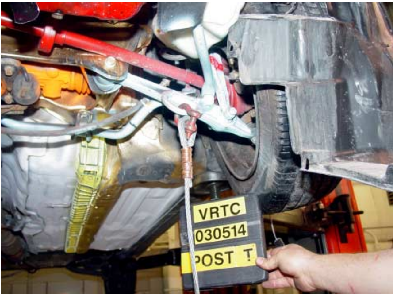
Figure A-120 Post-Test Target Vehicle Sway Bar - View 2
