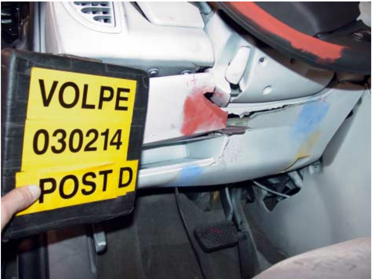
Figure A- 69 Post-Test Driver Dummy Knee Contact - View 2
