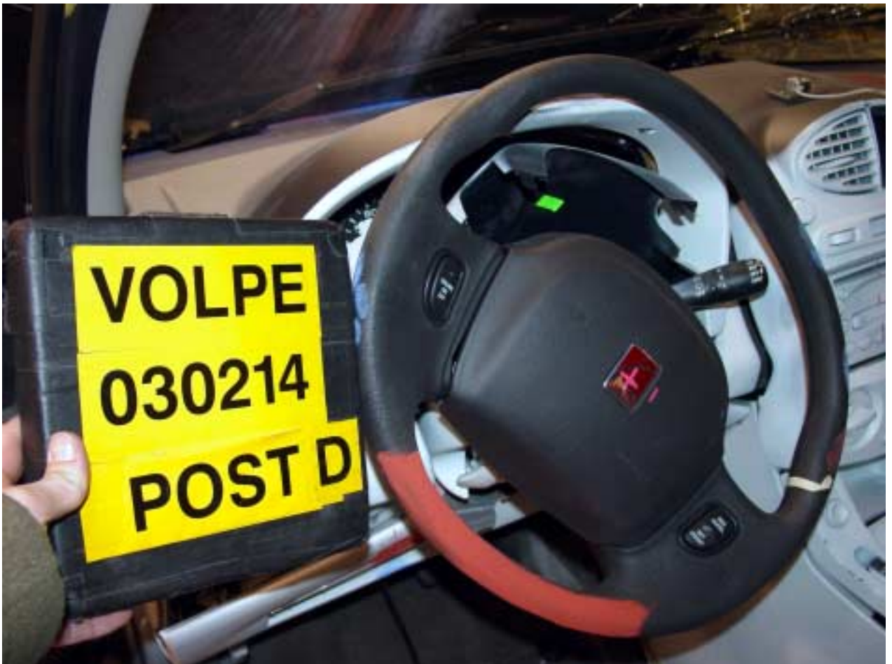
Figure A- 67 Post-Test Driver Dummy Abdomen Contact View
