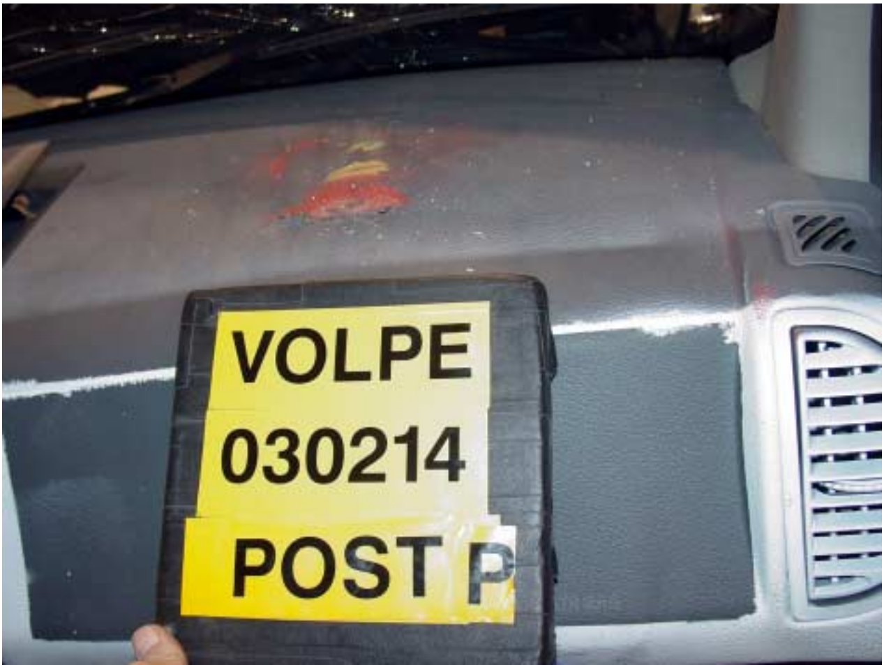
Figure A-73 Post-Test Passenger Dummy Head Contact - View 3
