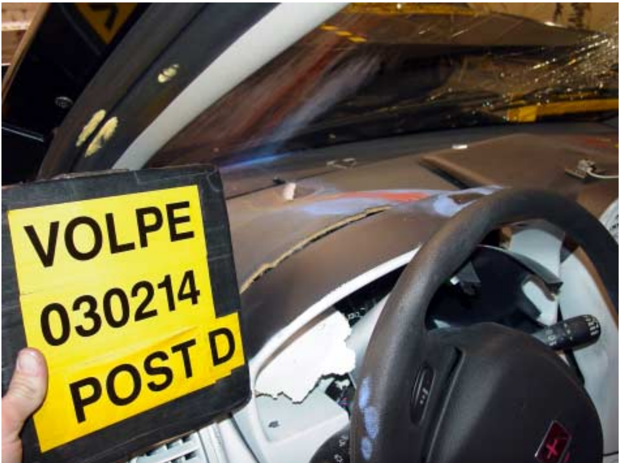
Figure A- 65 Post-Test Driver Dummy Head Contact - View 4
