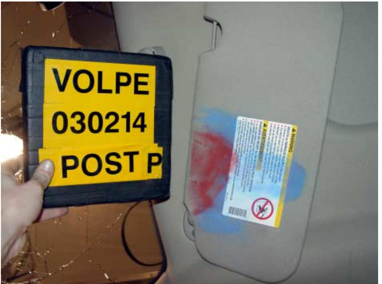
Figure A-74 Post-Test Passenger Dummy Head Contact - View 4
