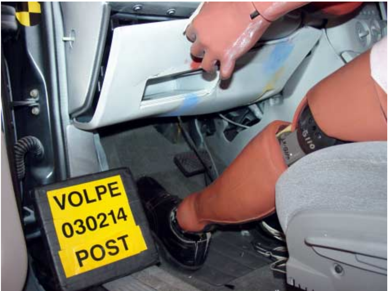
Figure A- 45 Post-Test Driver Dummy Leg Position View
