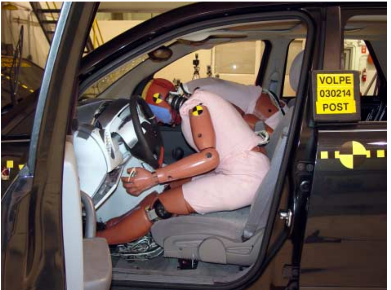
Figure A- 39 Post-Test Driver Dummy & Vehicle Interior - View 1
