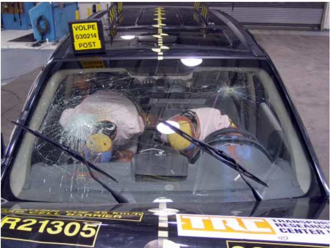
Figure A- 32 Post-Test Windshield View
