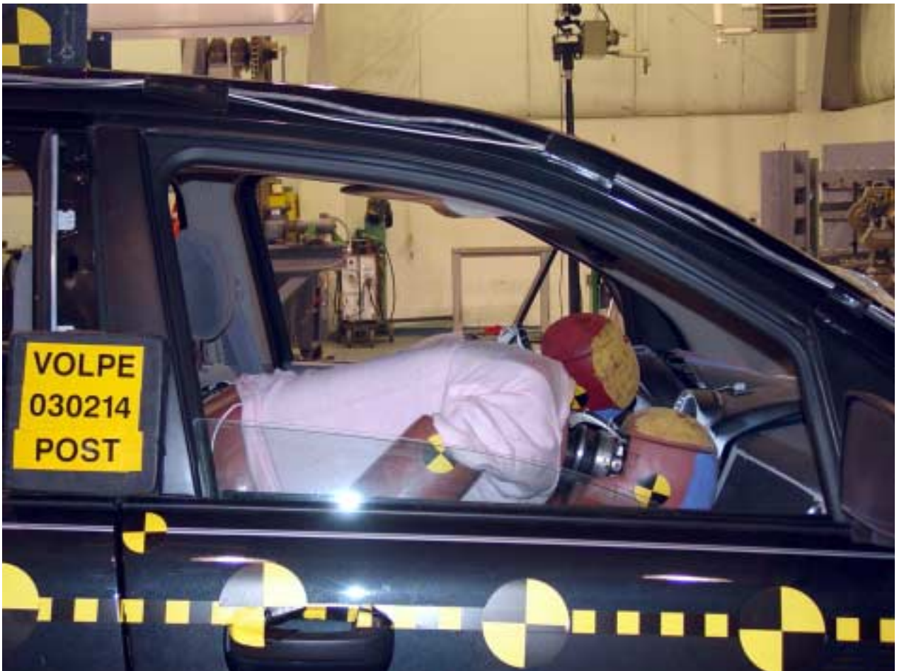
Figure A- 51 Post-Test Passenger Dummy Position - View 2
