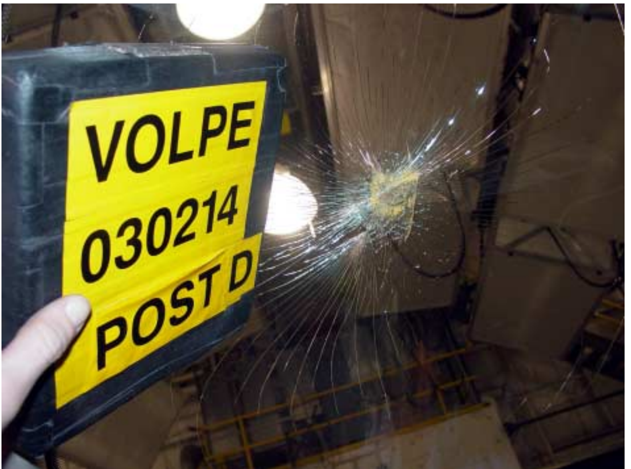
Figure A- 63 Post-Test Driver Dummy Head Contact - View 2
