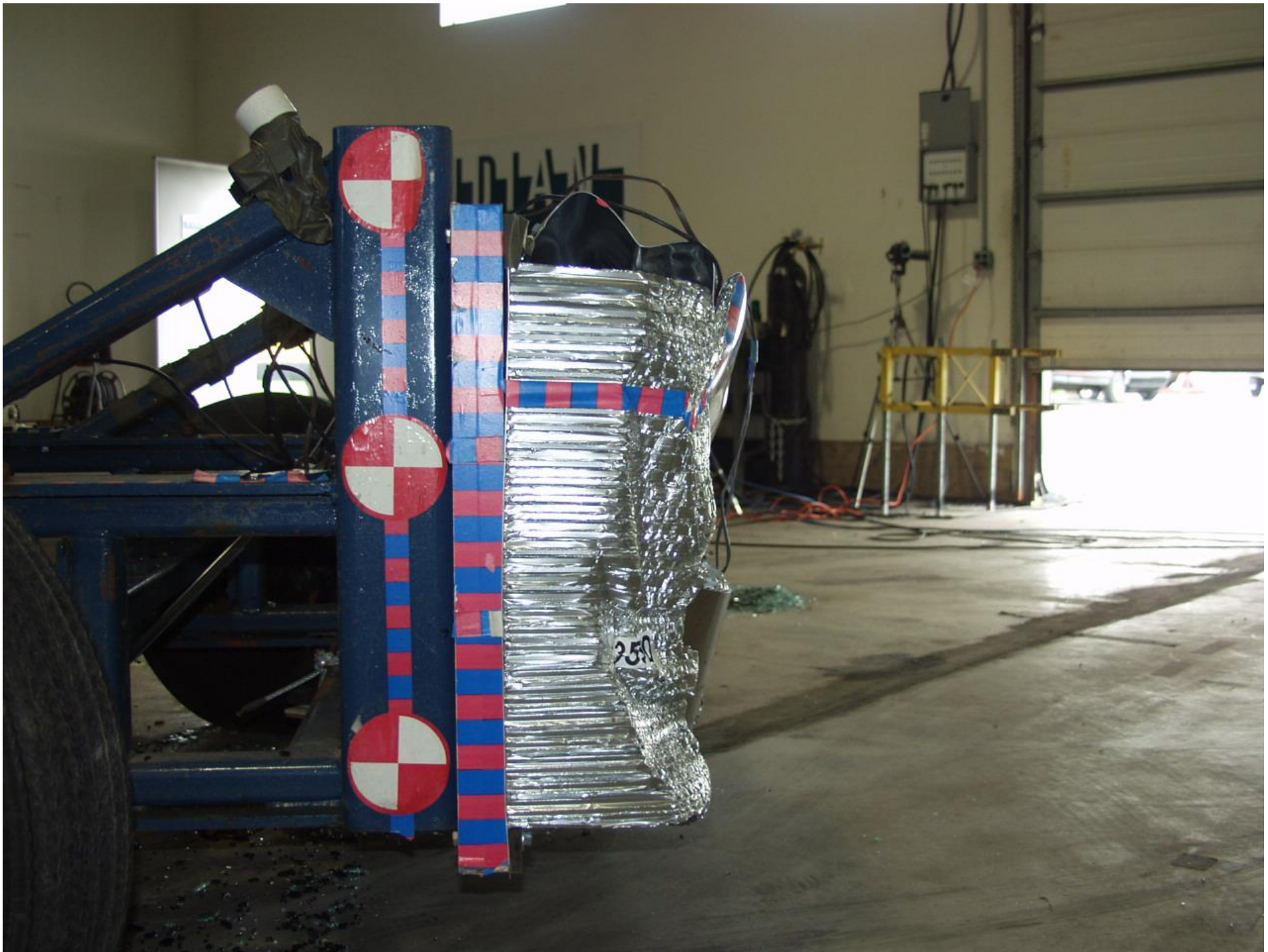
Figure A-20 POST-TEST RIGHT SIDE VIEW OF IMPACTOR FACE
