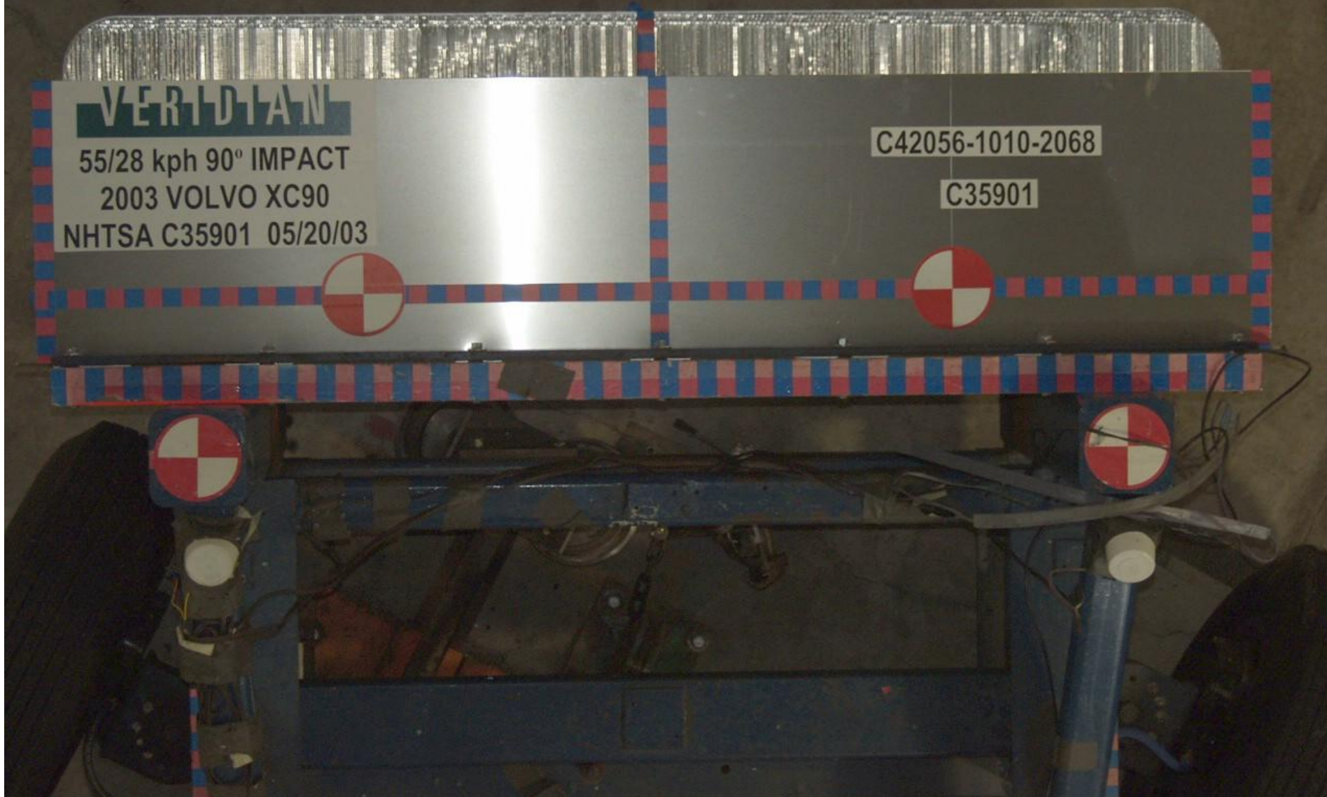
Figure A-21 PRE-TEST TOP VIEW OF IMPACTOR FACE
