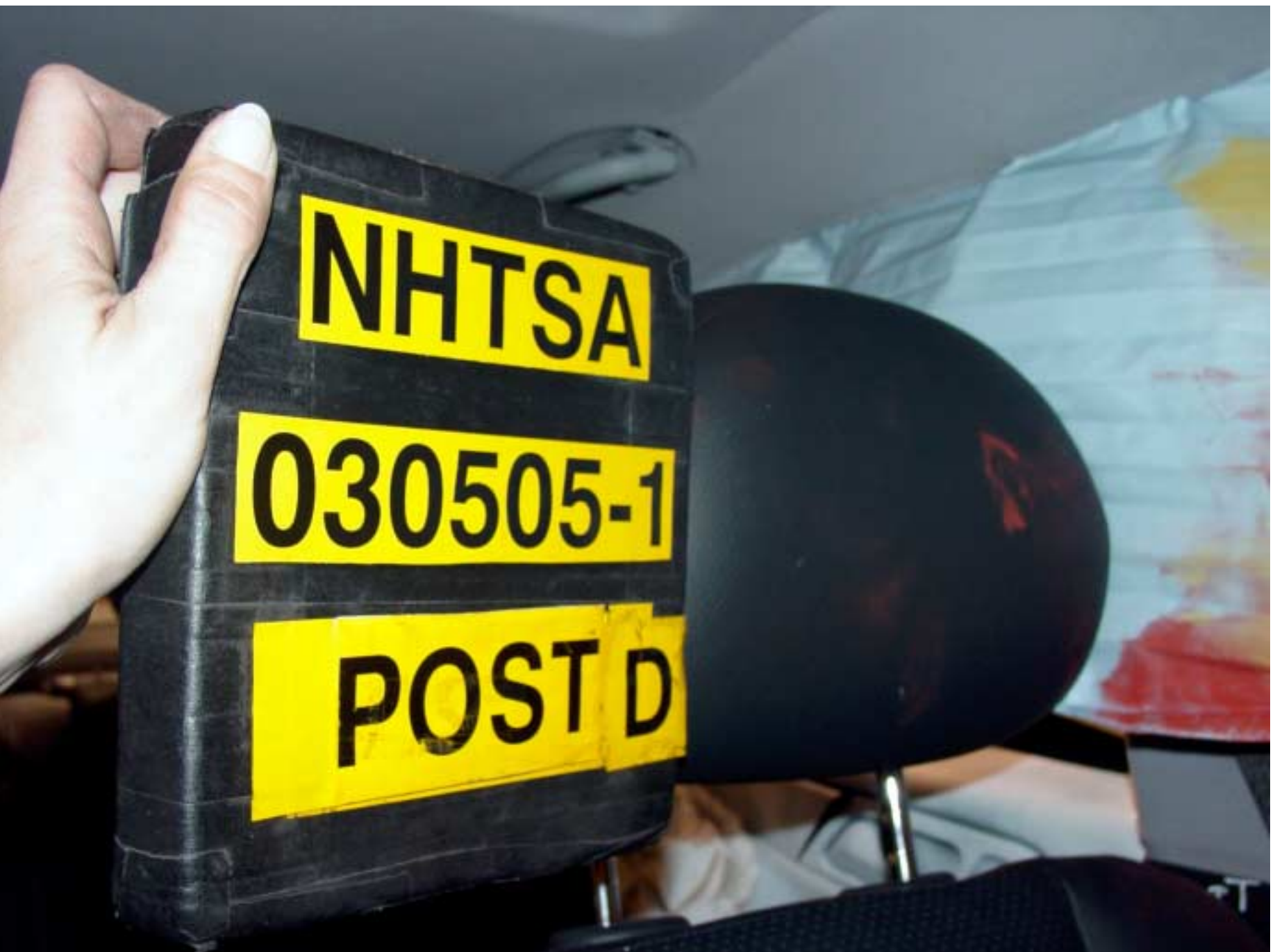
Figure A-34 Post-Test Front SID Contact – View 2
