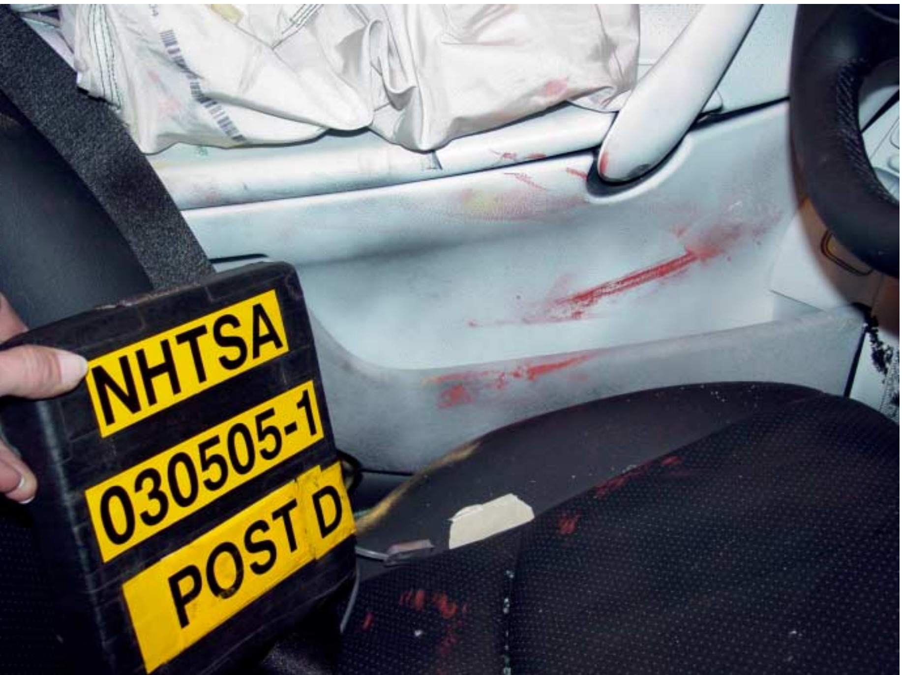
Figure A-36 Post-Test Front SID Contact – View 4
