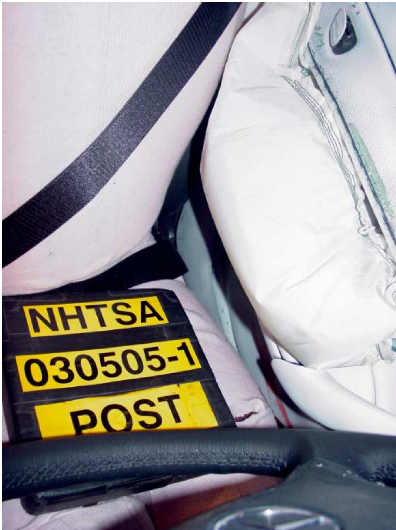
Figure A-25 Post-Test View of Front SID and Door Clearance
