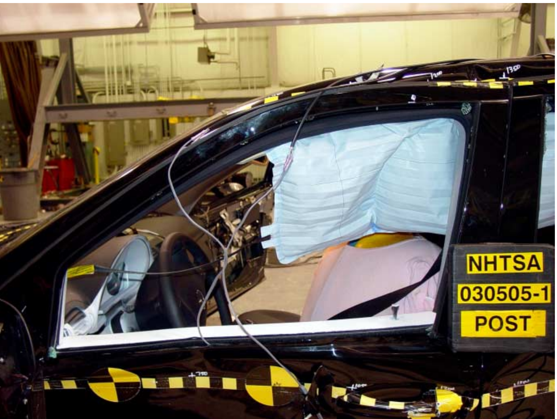
Figure A-22 Post-Test Left View of Front SID
