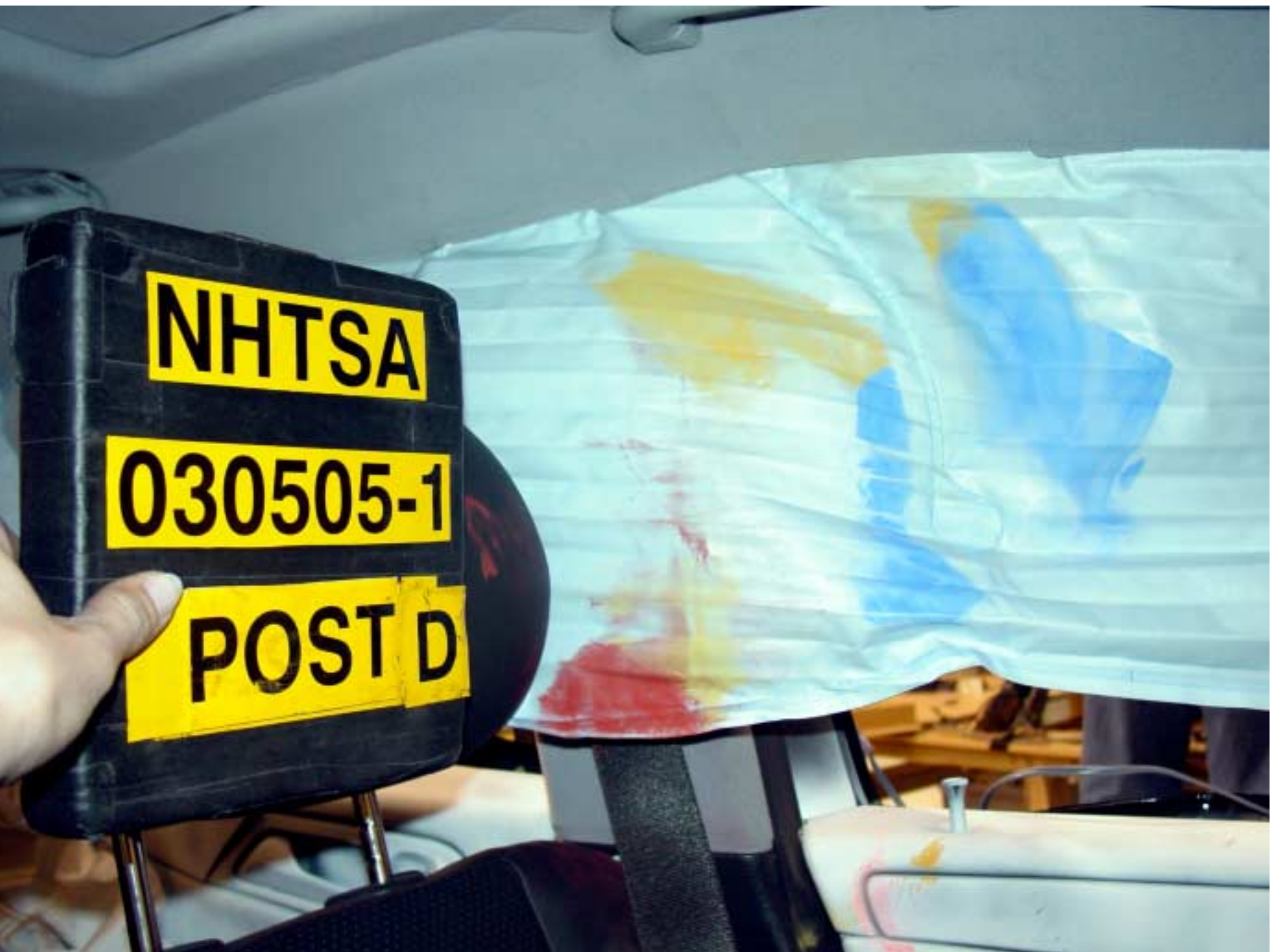
Figure A-33 Post-Test Front SID Contact – View 1
