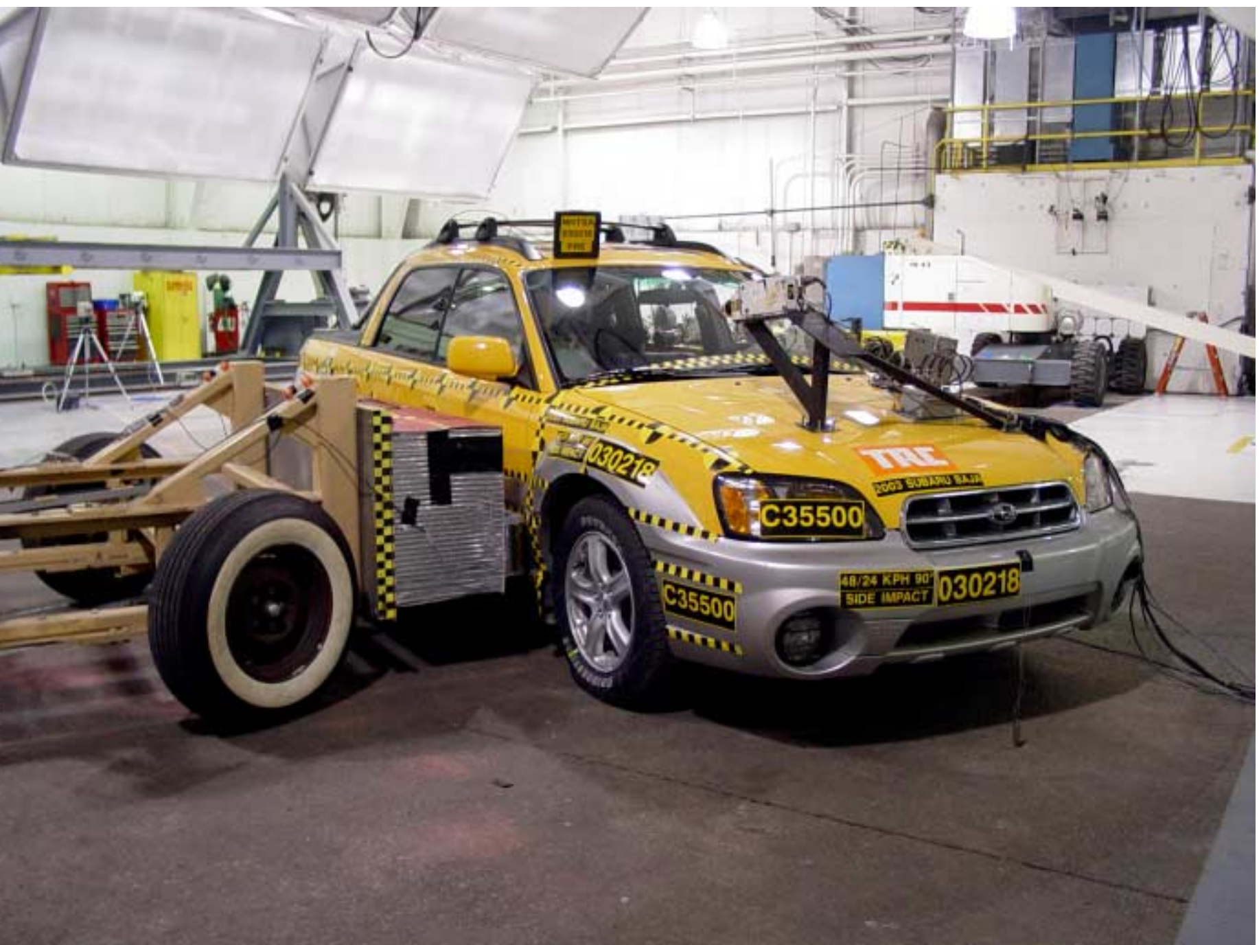
Figure A-43 Pre-Test Right Side View of MDB with Impactor Face in Position
