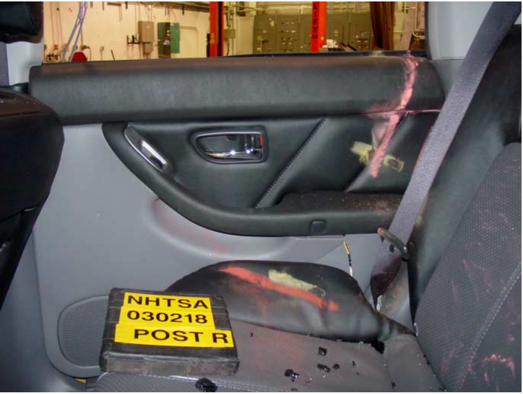
Figure A-36 Post-Test Interior of Rear Panel Showing SID Impact Locations
