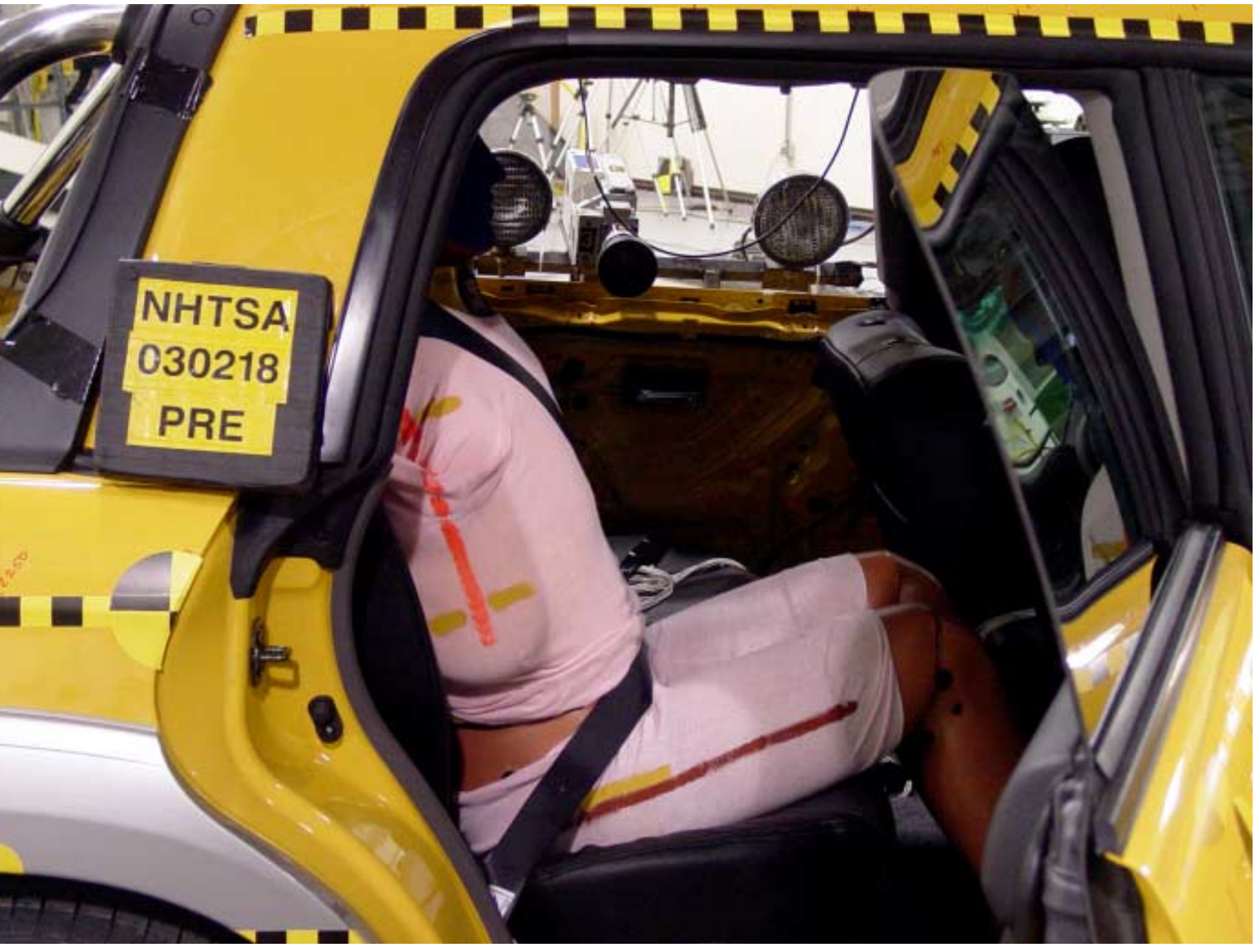
Figure A-27 Pre-Test Right View of Rear SID and Belt Position
