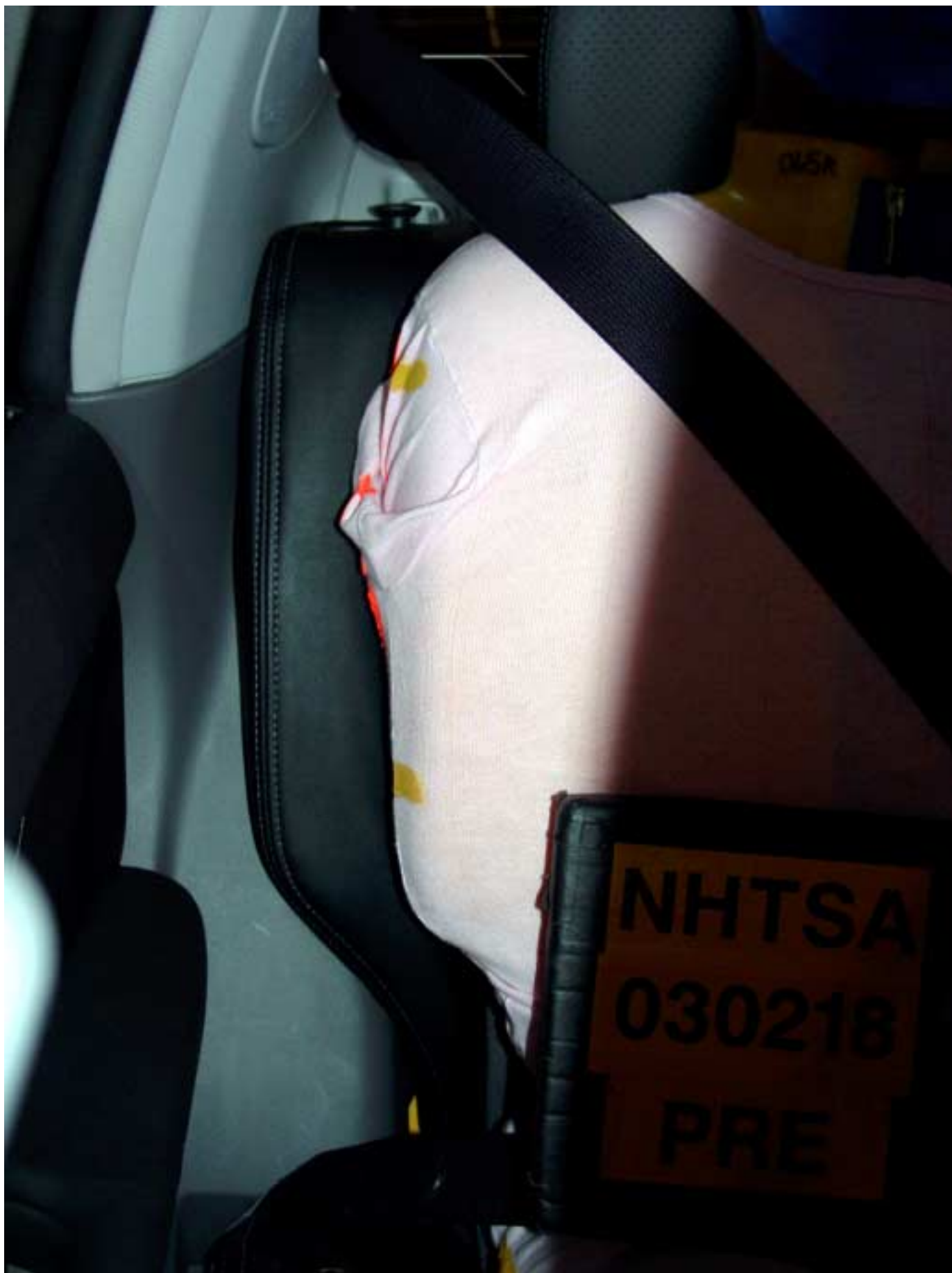
Figure A-28 Pre-Test Right View of Rear SID and Door Clearance
