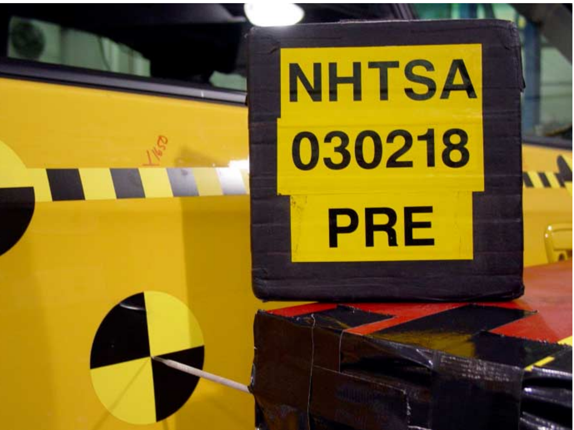
Figure A-44 Pre-Test Secondary Impact Point View
