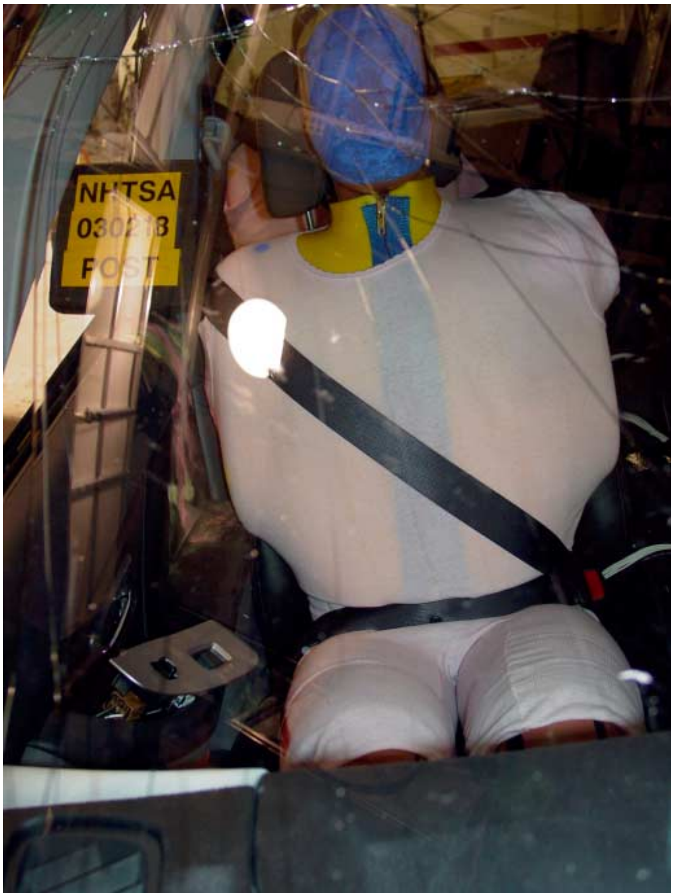
Figure A-25 Post-Test Right View of Front SID and Door Clearance
