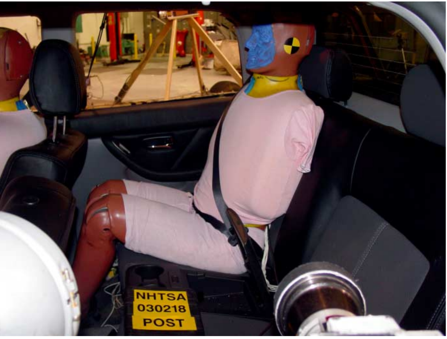
Figure A-21 Post-Test Left Occupant Compartment View of Rear SID
