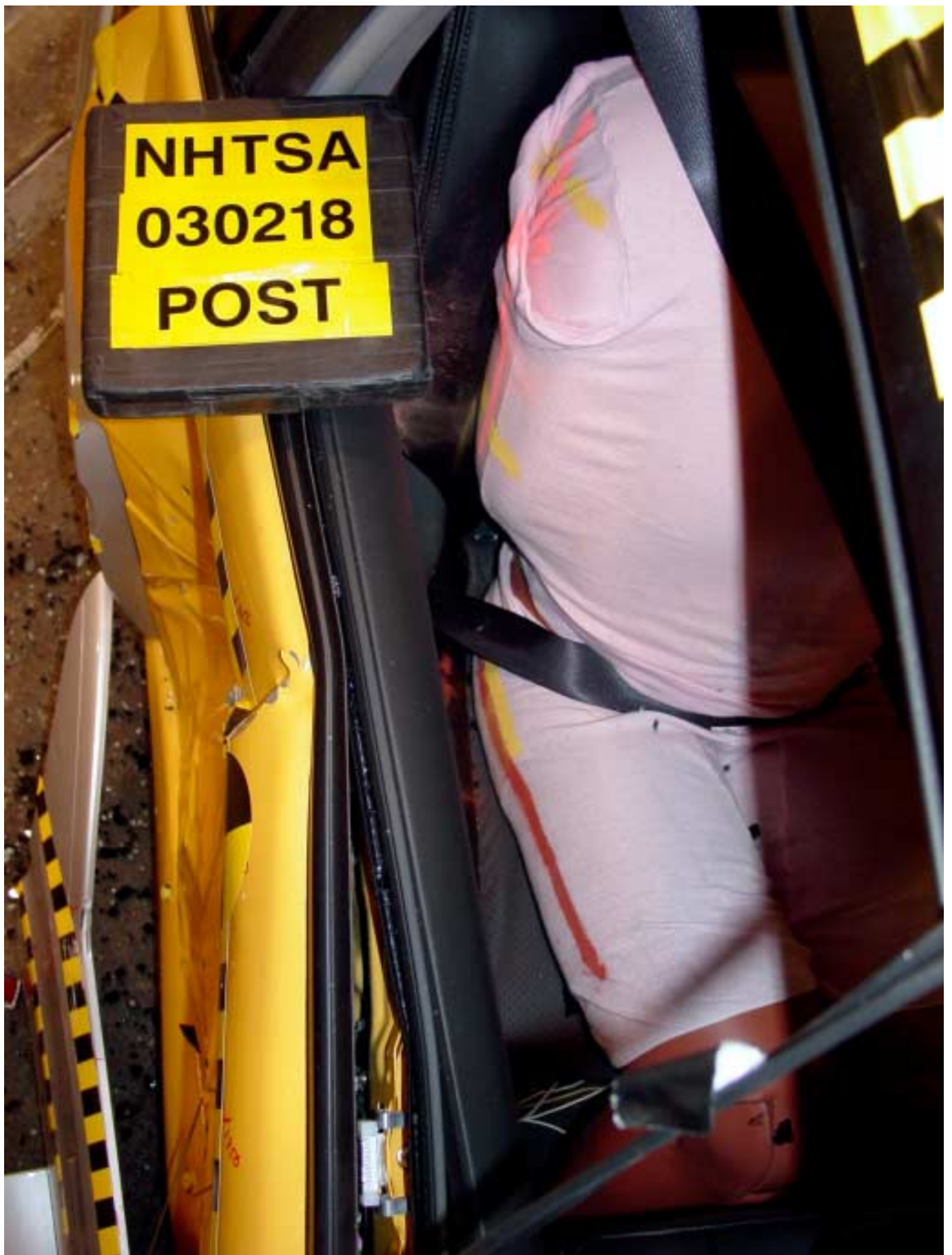
Figure A-29 Post-Test Right View of Rear SID and Door Clearance
