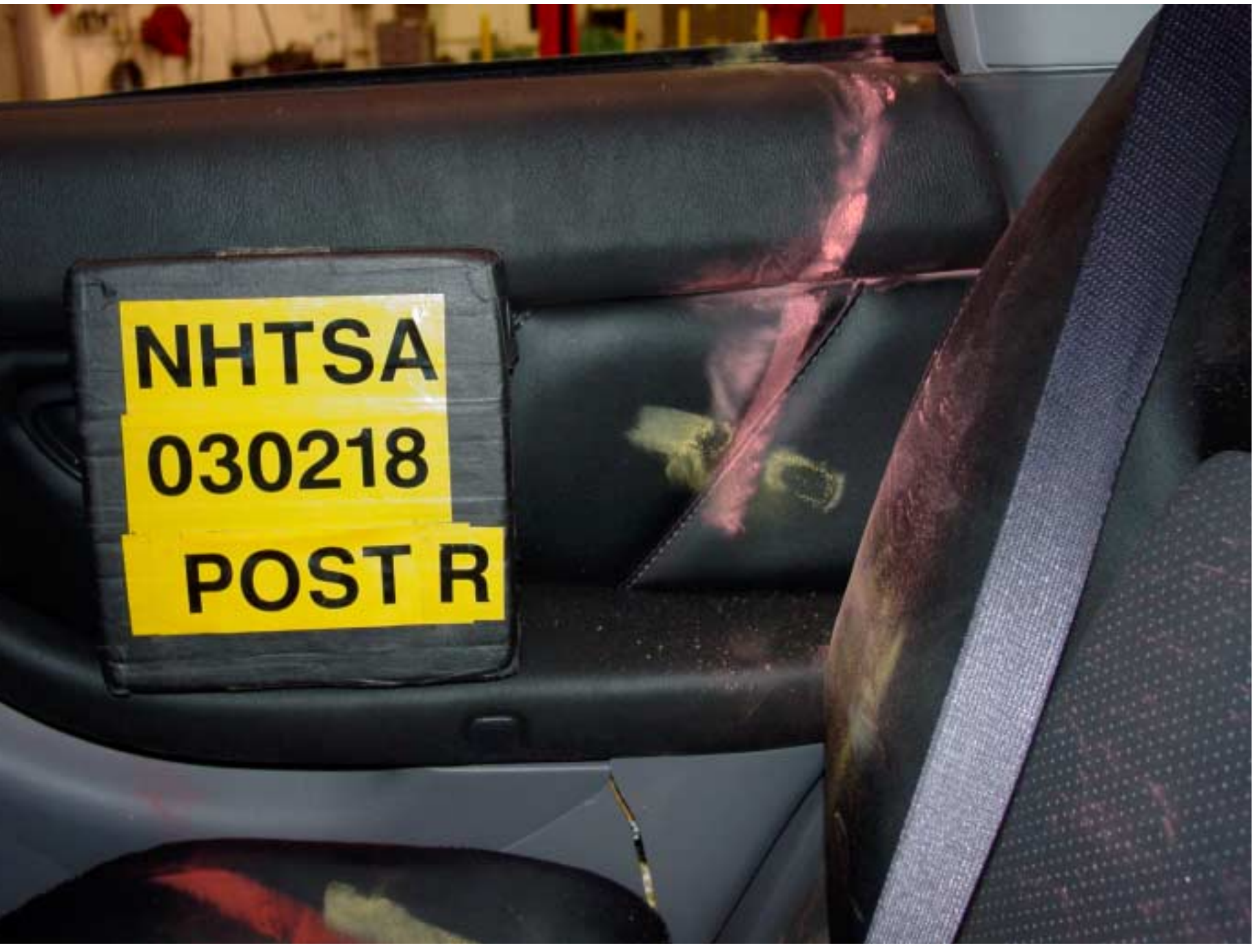
Figure A-37 Post-Test Rear SID Contact - View 1
