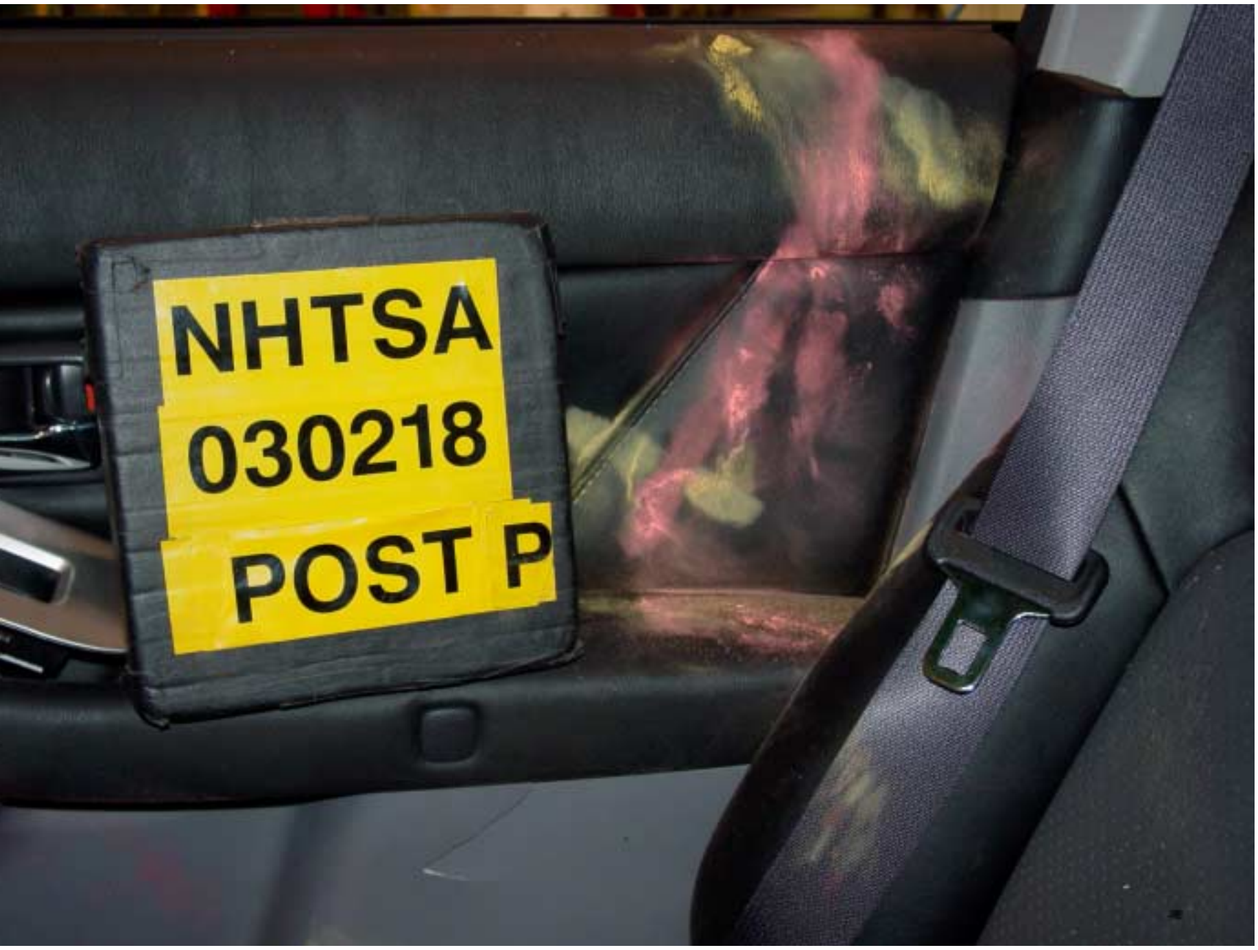
Figure A-32 Post-Test Front SID Contact - View 1
