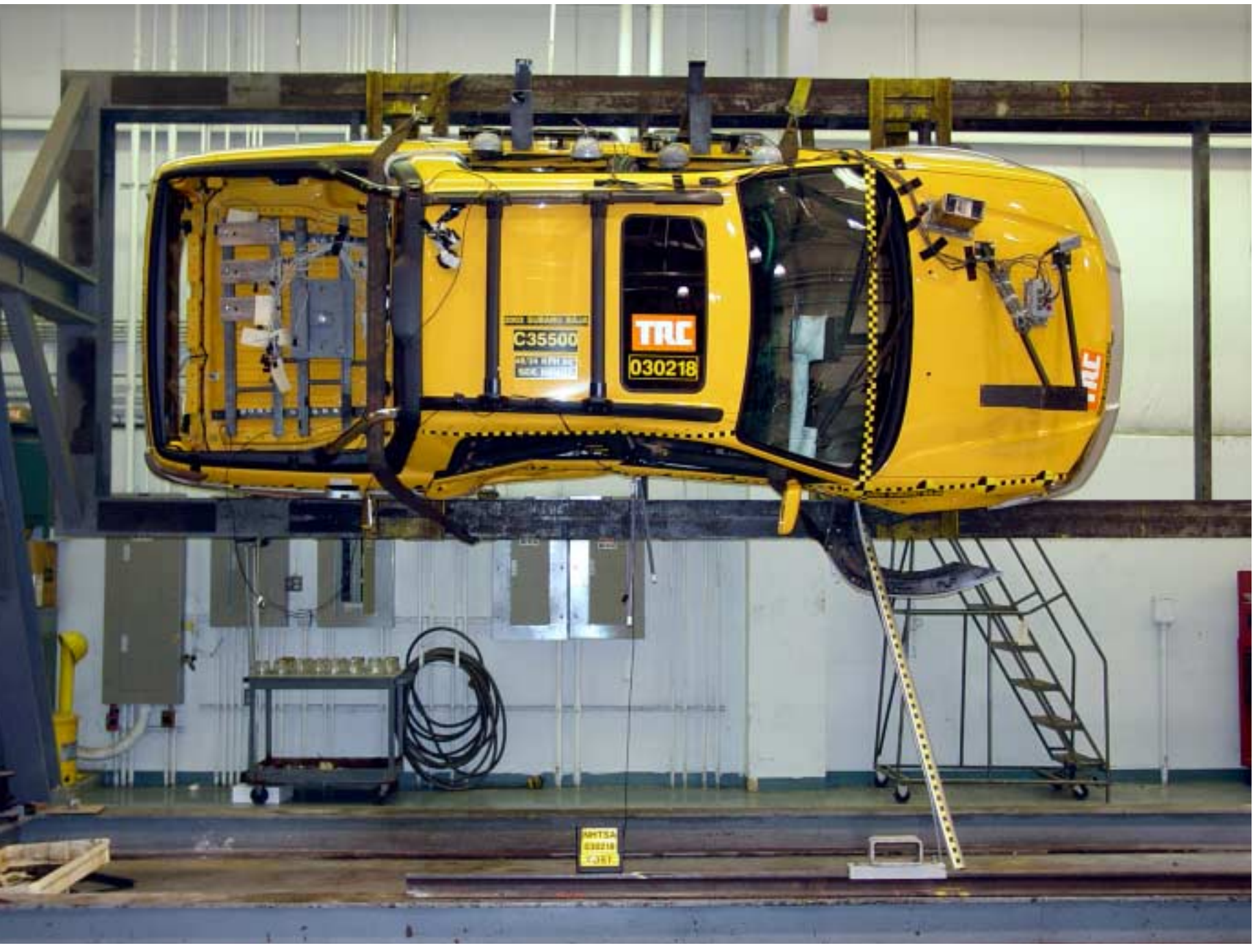
Figure A-51 FMVSS 301 Rollover View at 90°
