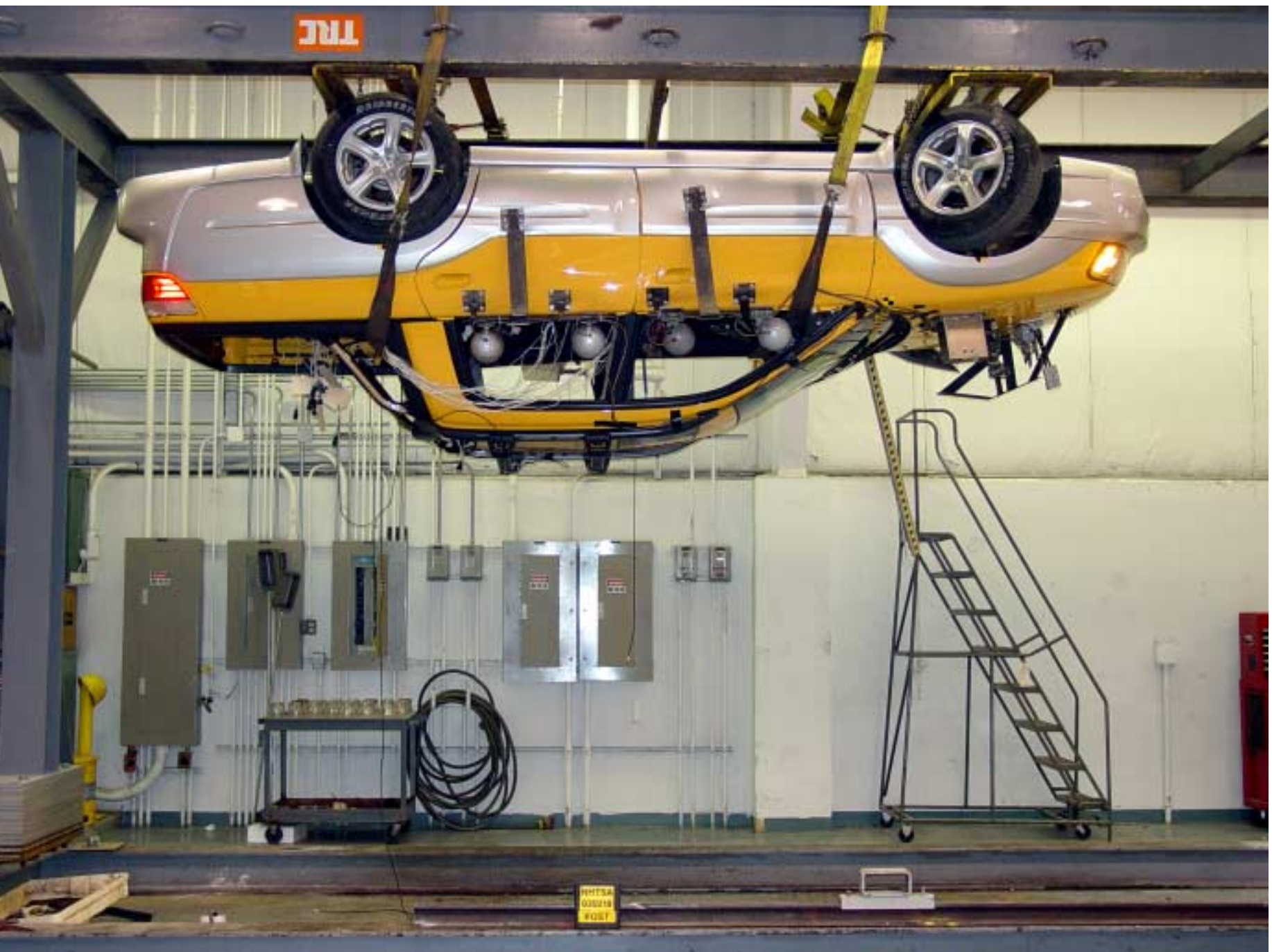
Figure A-52 FMVSS 301 Rollover View at 180°
