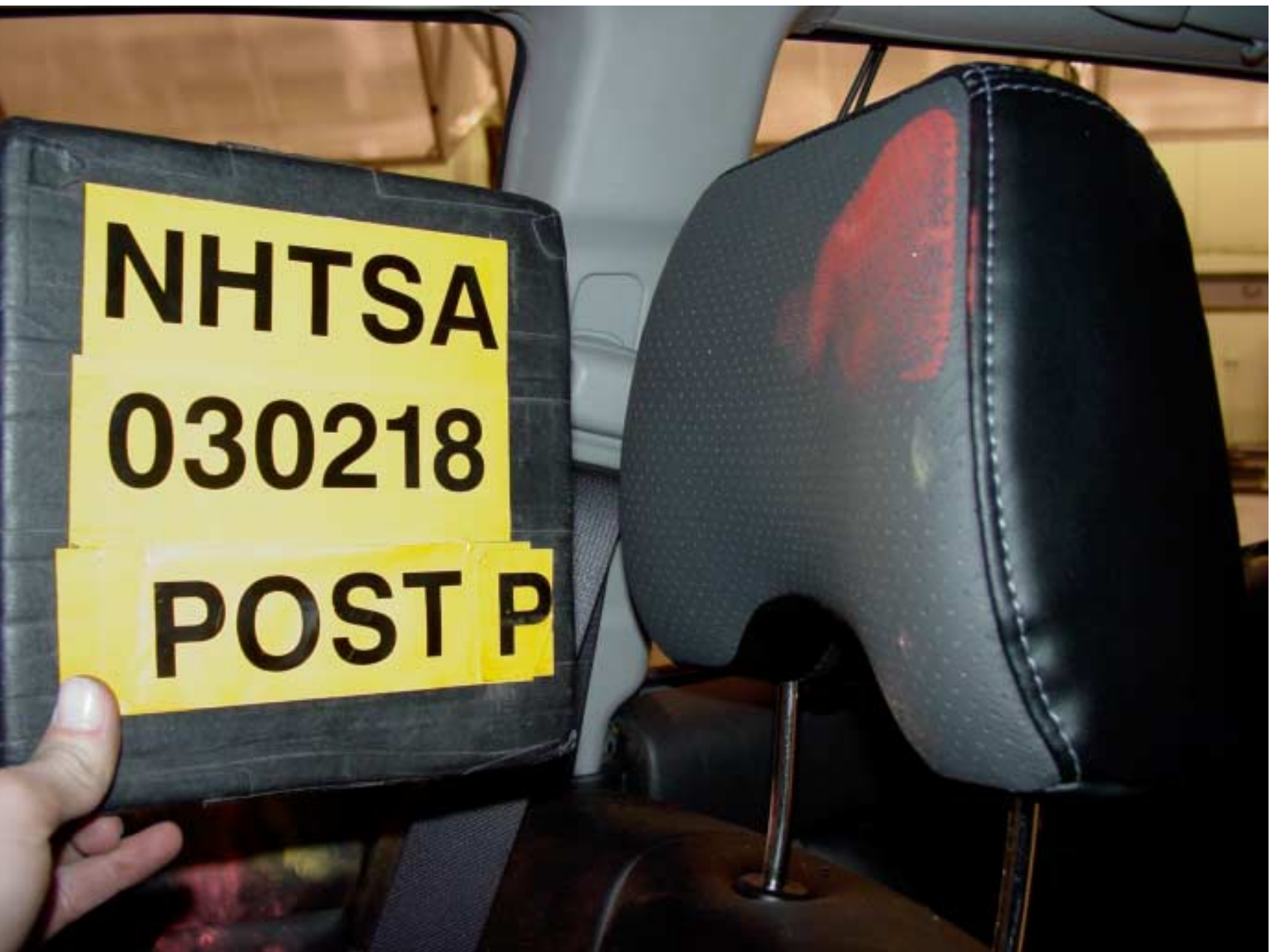
Figure A-33 Post-Test Front SID Contact - View 2
