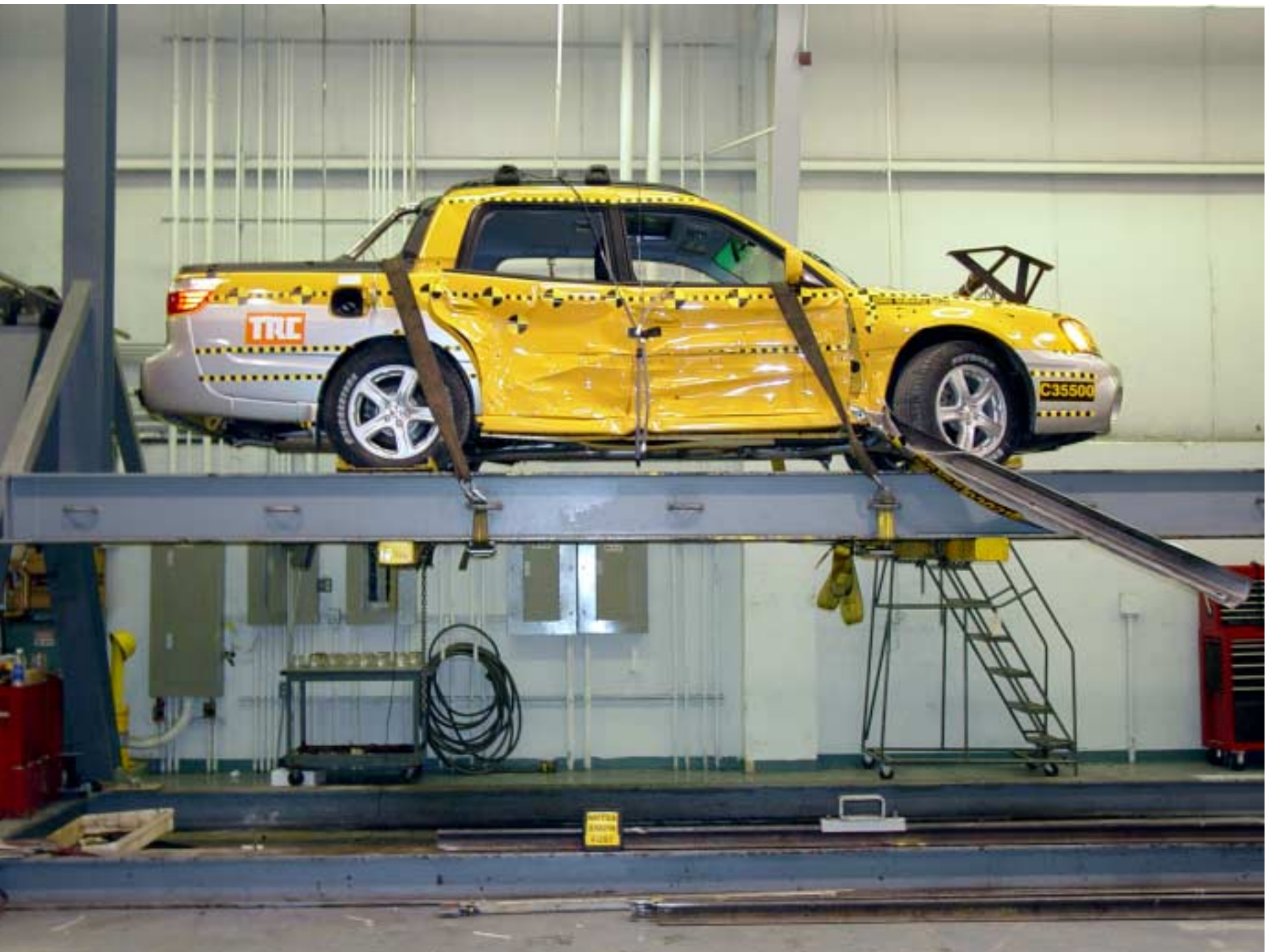
Figure A-54 FMVSS 301 Rollover View at 360°
