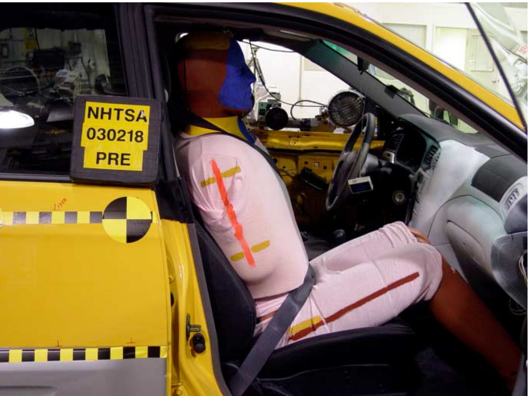
Figure A-23 Pre-Test Right View of Front SID and Belt Position
