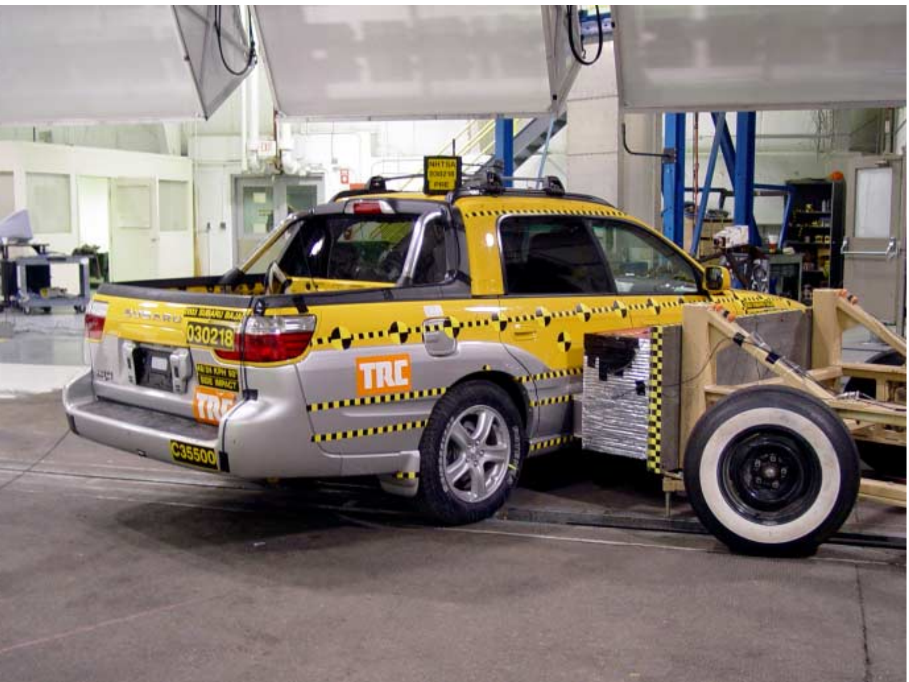
Figure A-40 Pre-Test Left Side View of MDB with Impactor Face in Position
