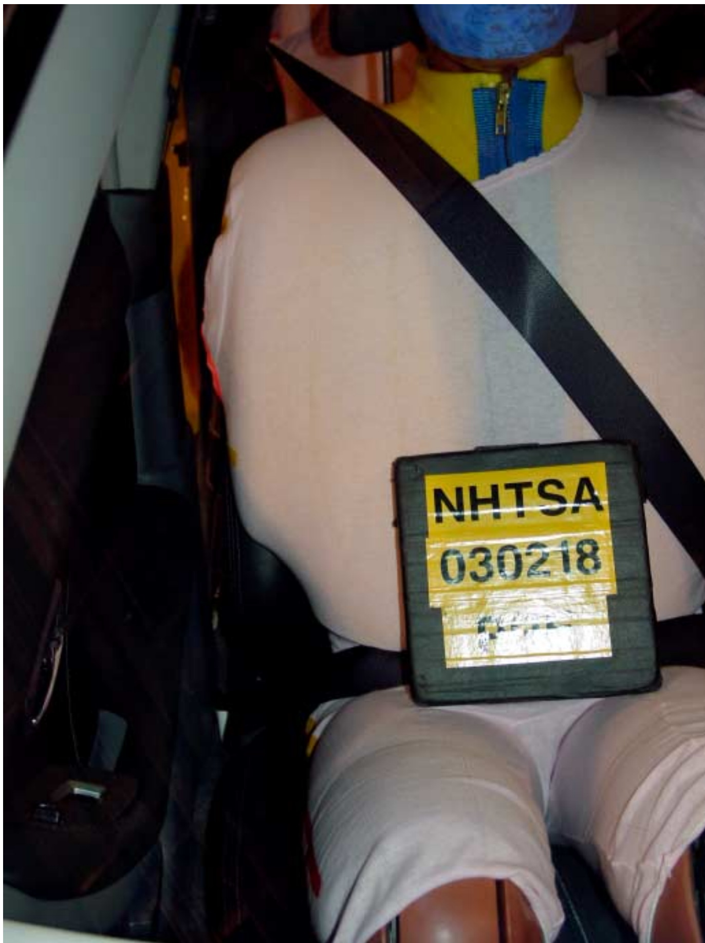
Figure A-24 Pre-Test Right View of Front SID and Door Clearance
