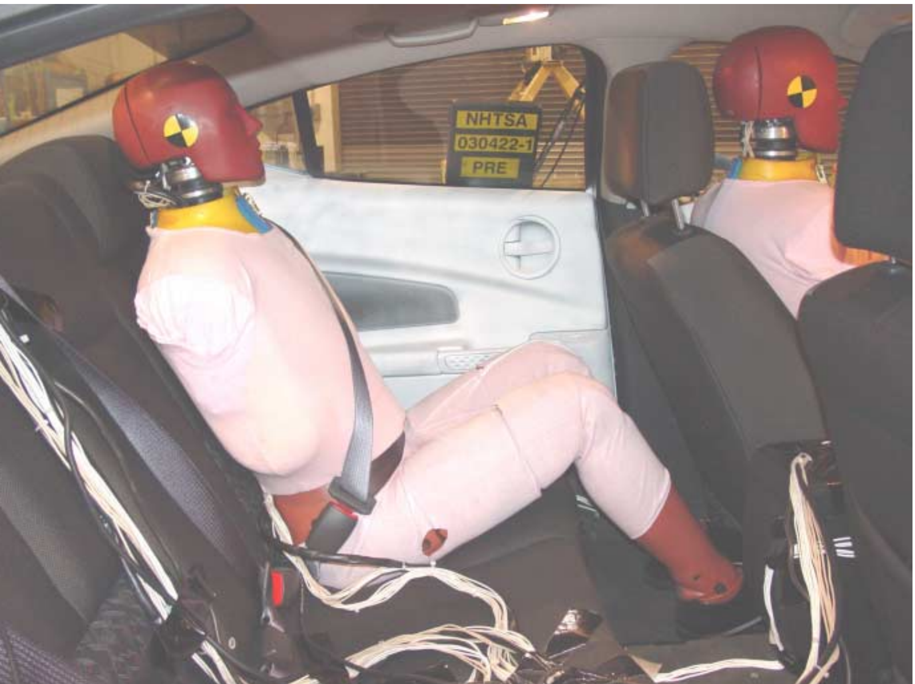
Figure A-20 Pre-Test Right Occupant Compartment View of Rear SID-H3
