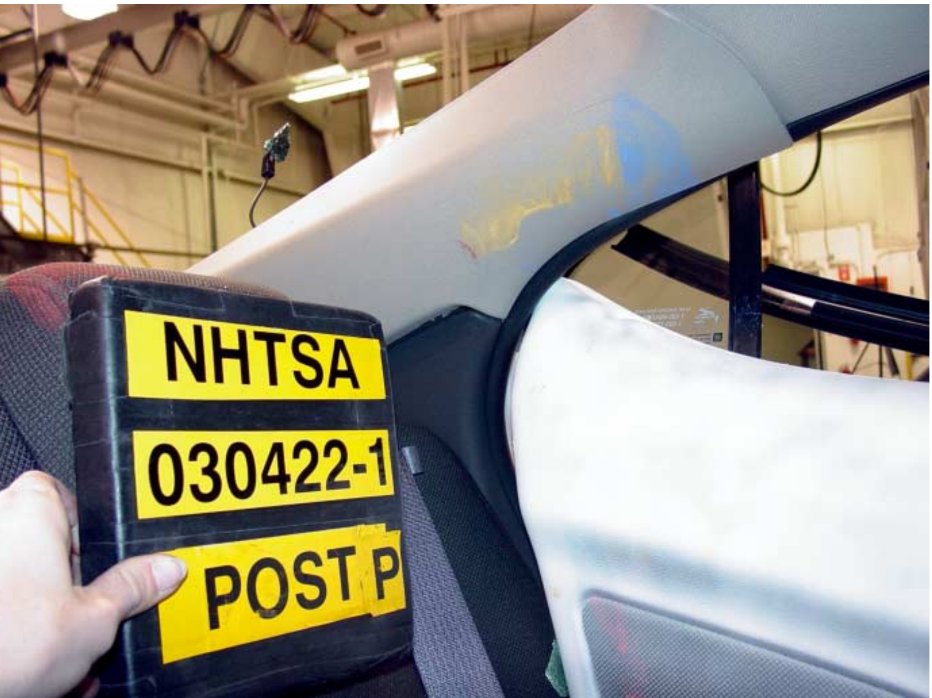
Figure A-39 Post-Test Rear SID-H3 Contact - View 3
