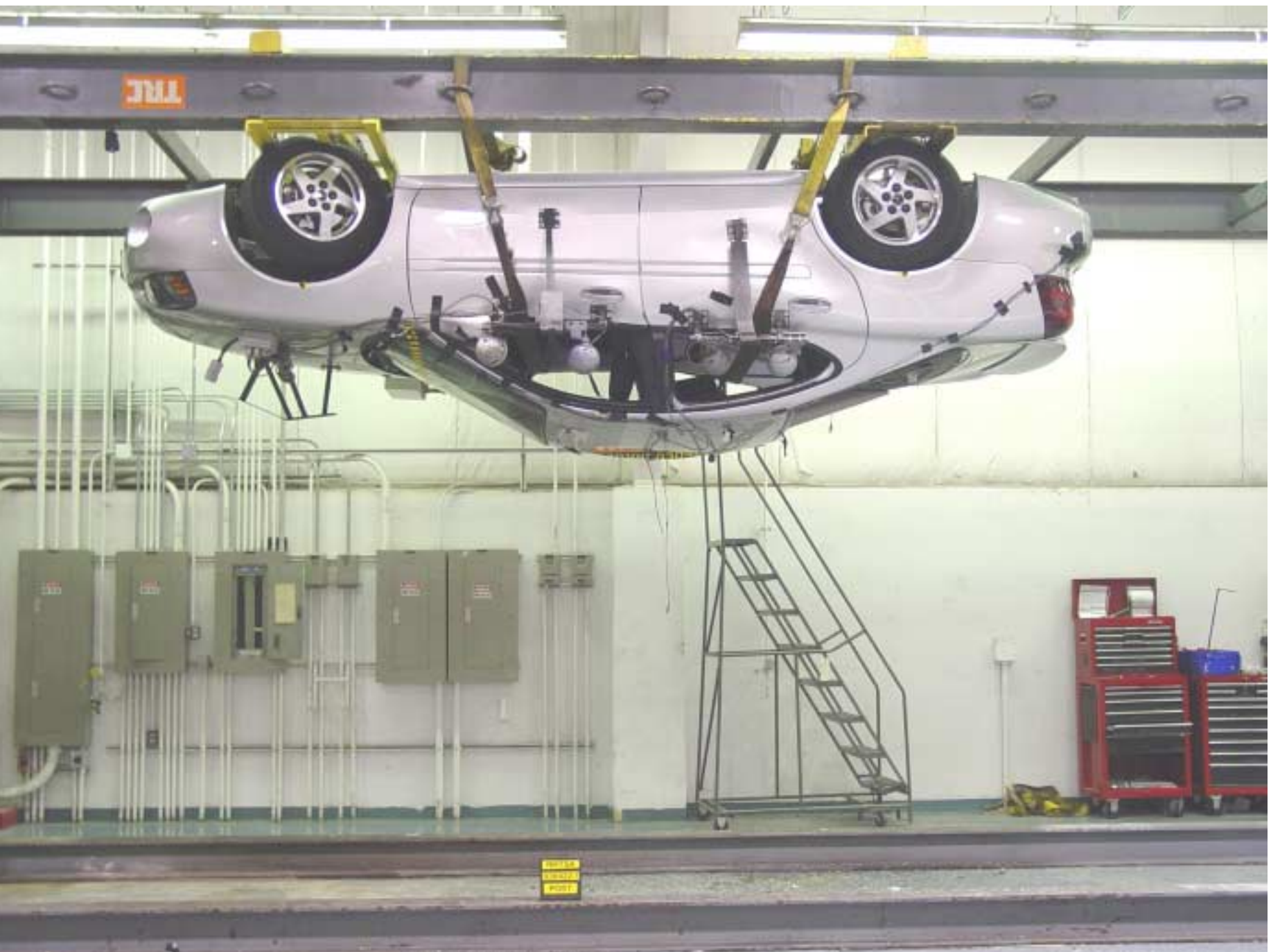
Figure A-53 FMVSS 301 Rollover View at 180°
