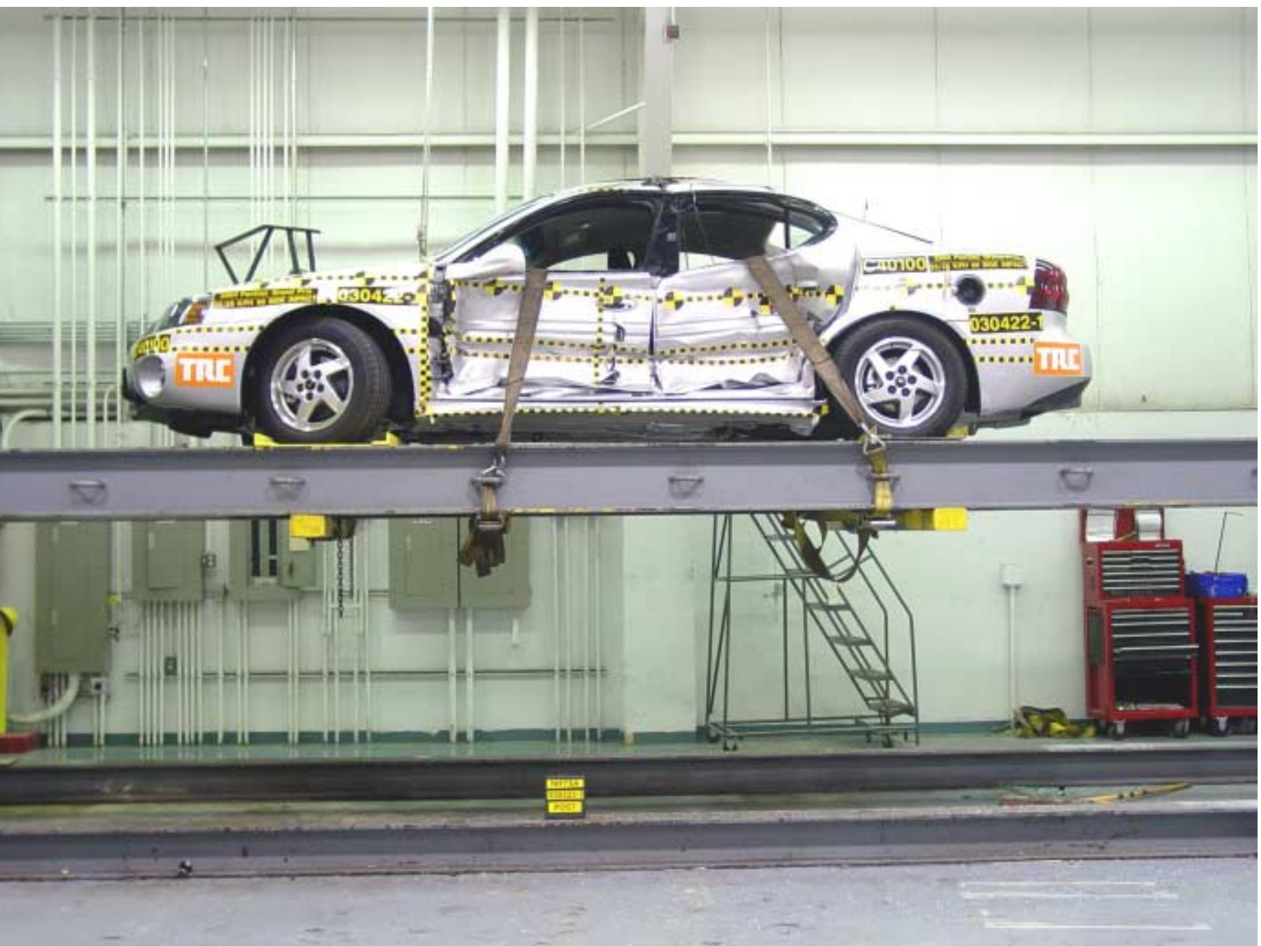
Figure A-55 FMVSS 301 Rollover View at 360°
