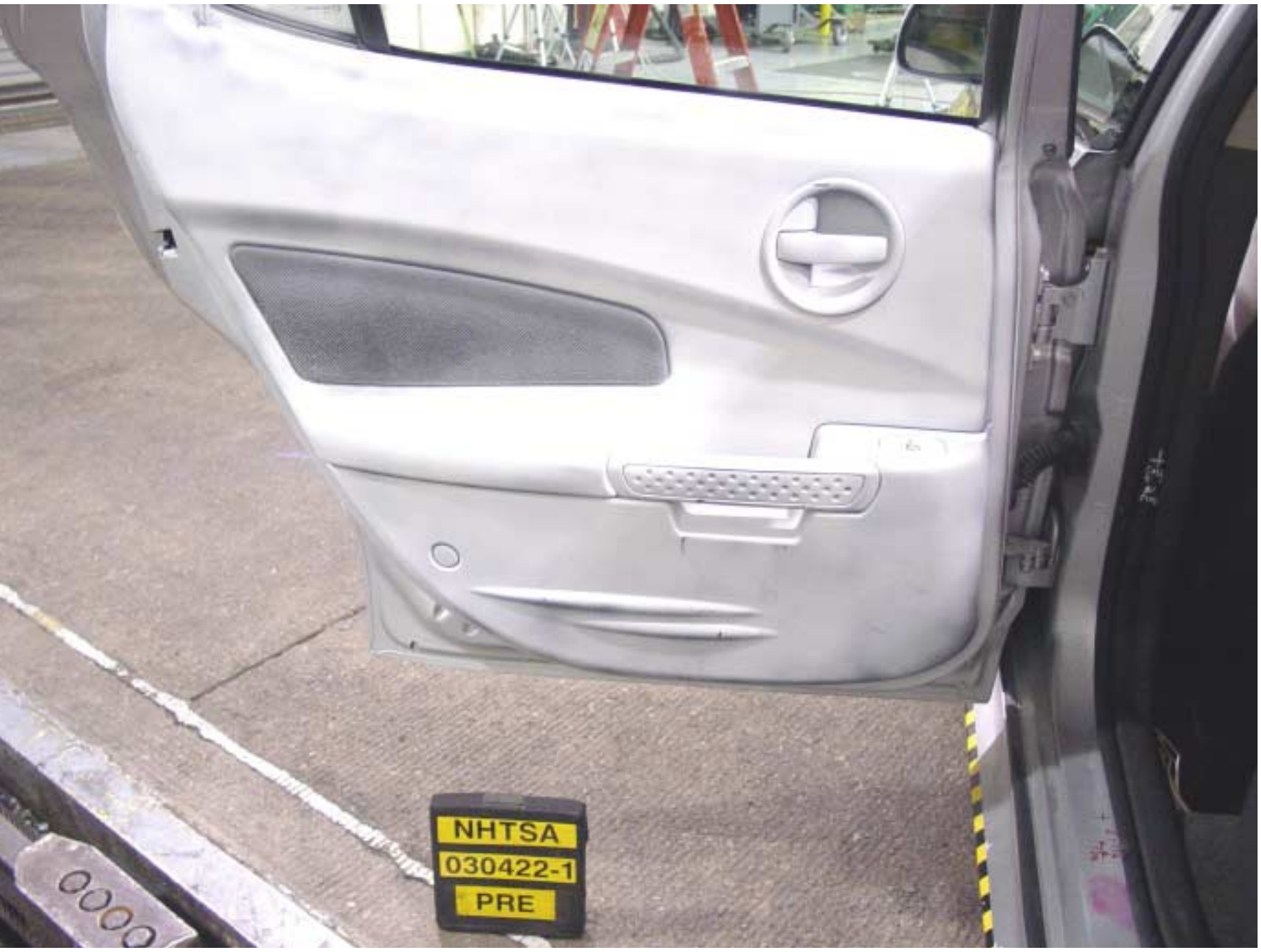
Figure A-35 Pre-Test Interior of Rear Door
