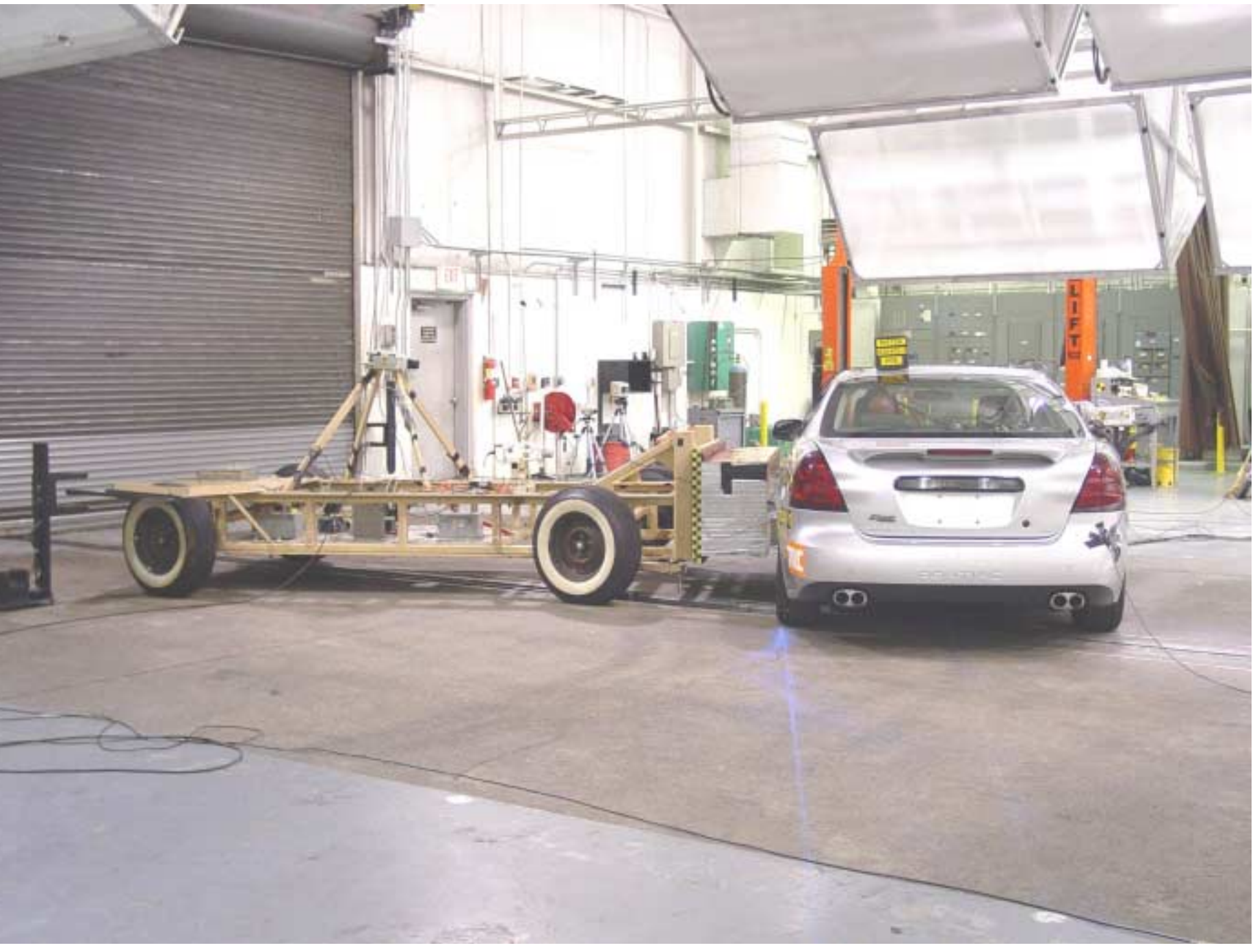
Figure A-44 Pre-Test Right Side View of MDB With Impactor Face in Position
