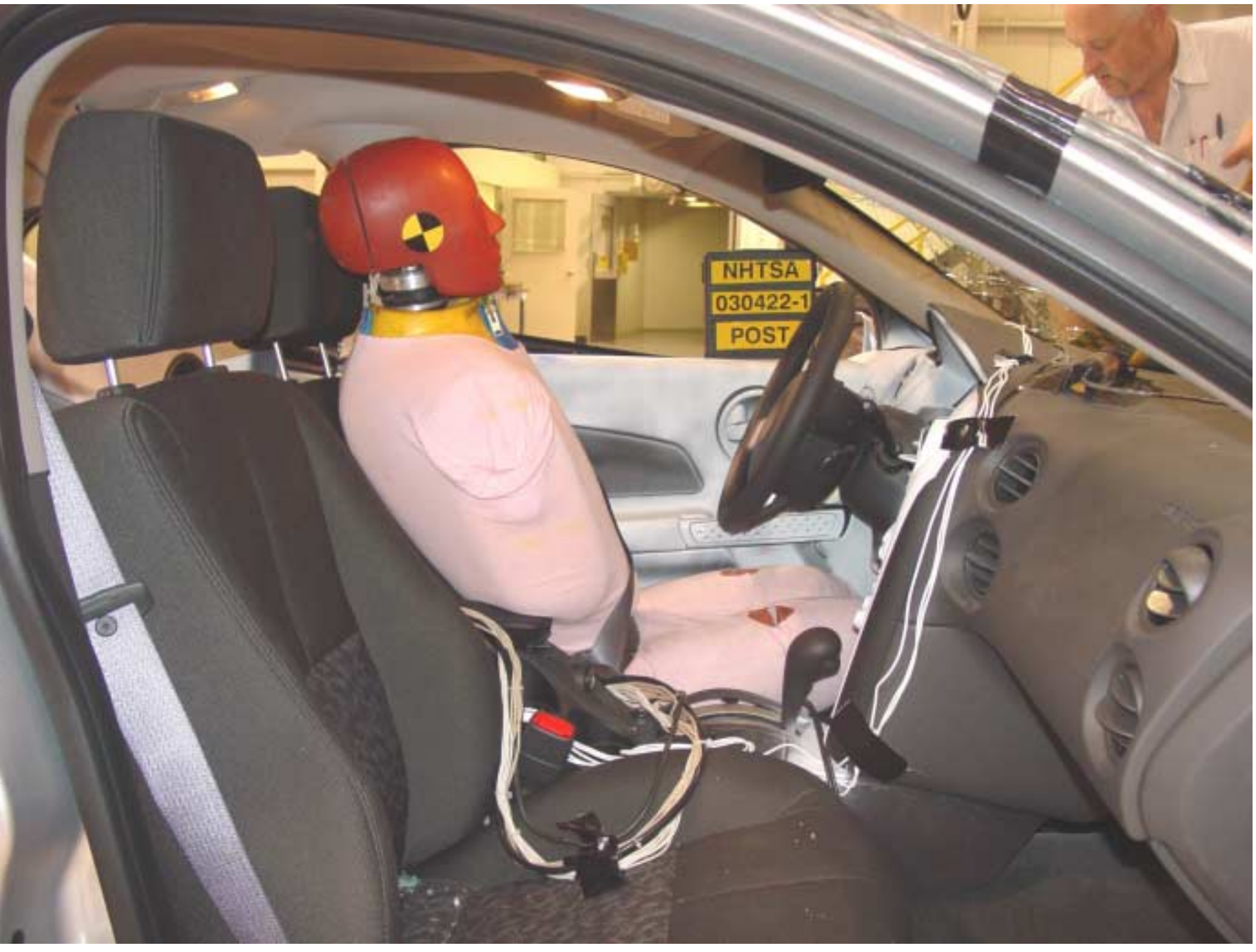
Figure A-19 Post-Test Right Occupant Compartment View of Front SID-H3
