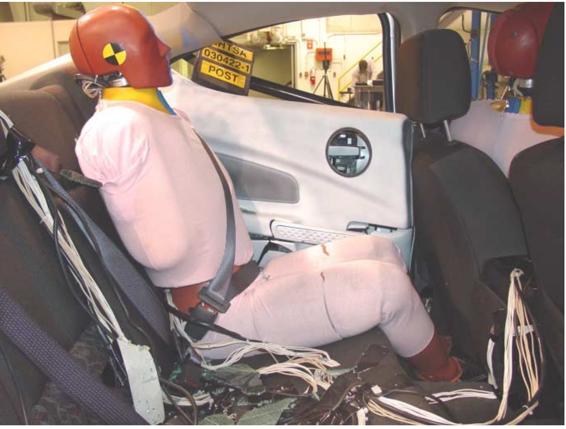
Figure A-21 Post-Test Right Occupant Compartment View of Rear SID-H3
