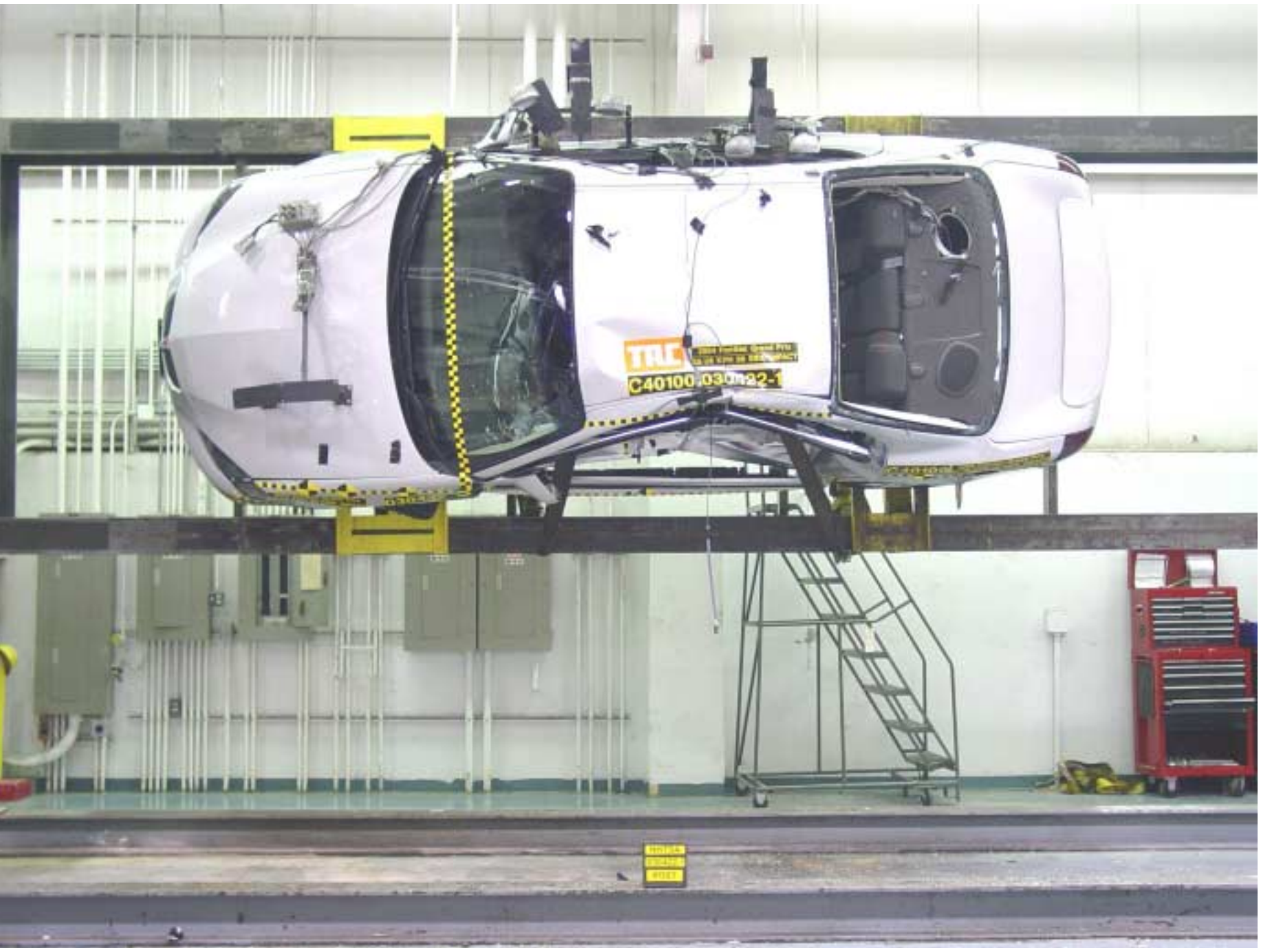
Figure A-52 FMVSS 301 Rollover View at 90°
