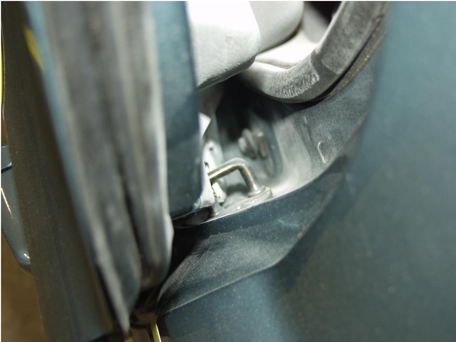
Figure A-47 POST TEST P4 DOOR LATCH/STRIKER
