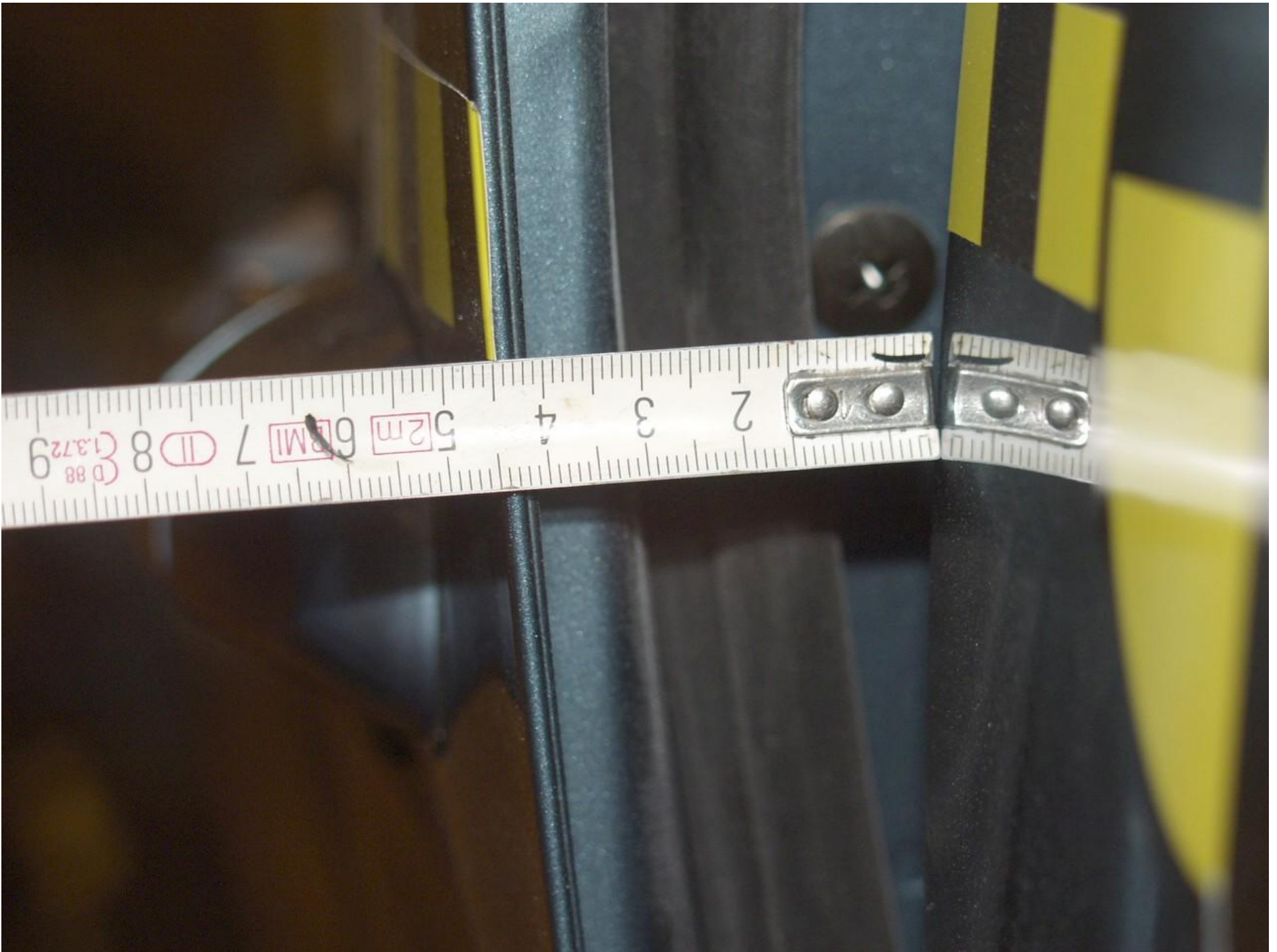
Figure A-48 POST TEST P4 DOOR TO BODY MEASUREMENT AT STRIKER HEIGHT
