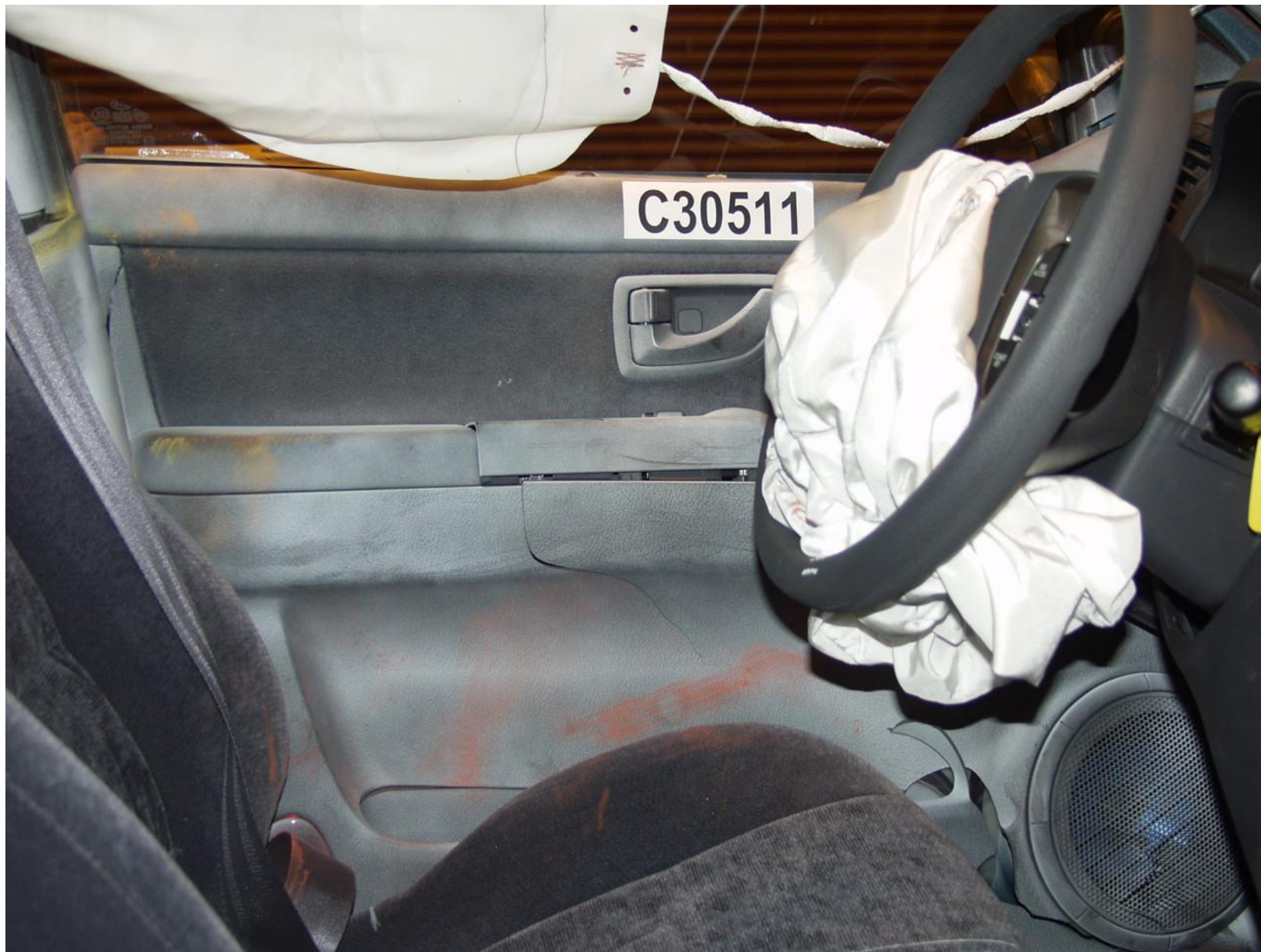
Figure A-34 POST-TEST INTERIOR OF FRONT DOOR SHOWING SID H3 IMPACT LOCATIONS
