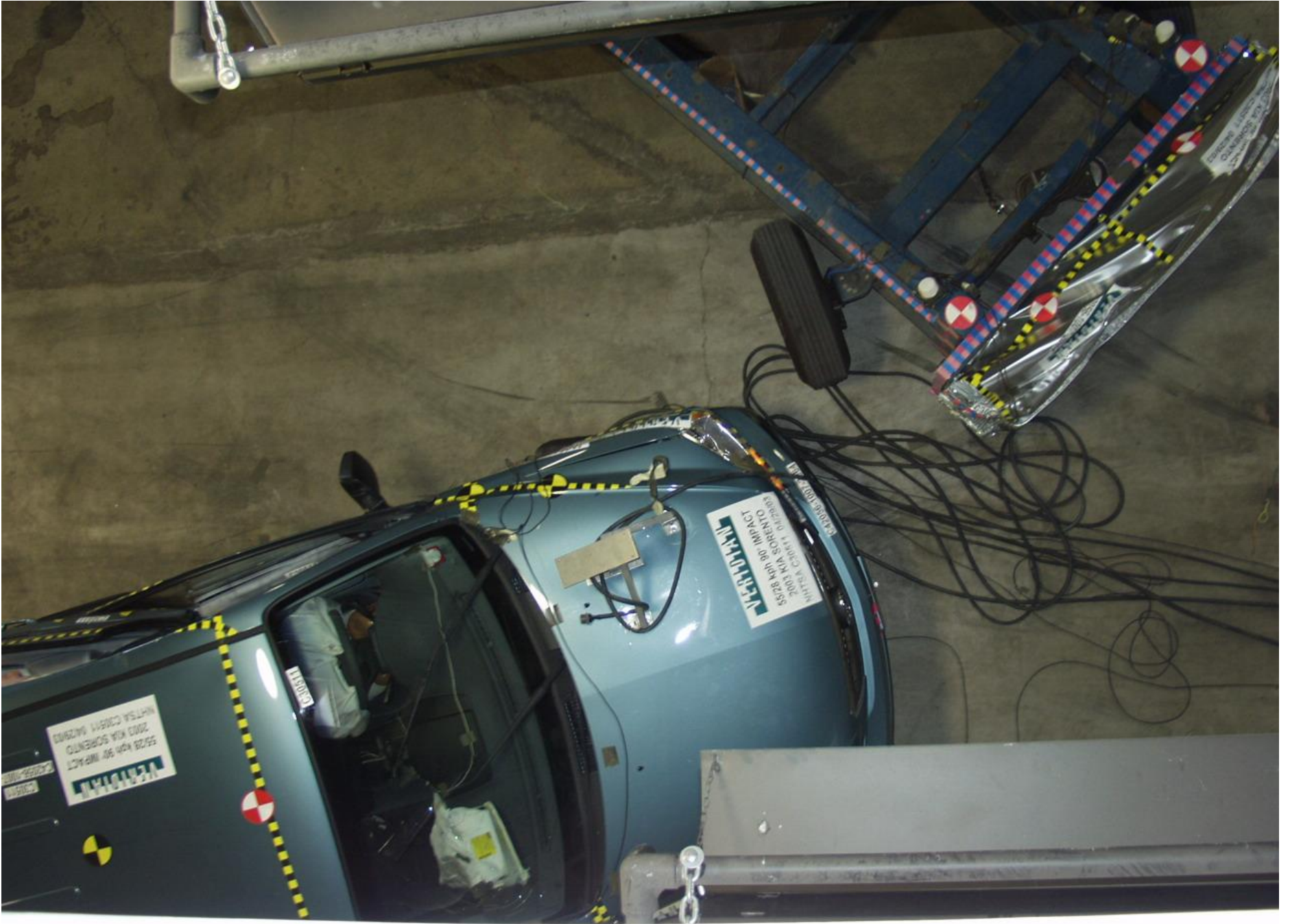
Figure A-24 POST-TEST OVERHEAD VIEW OF MDB AND VEHICLE
