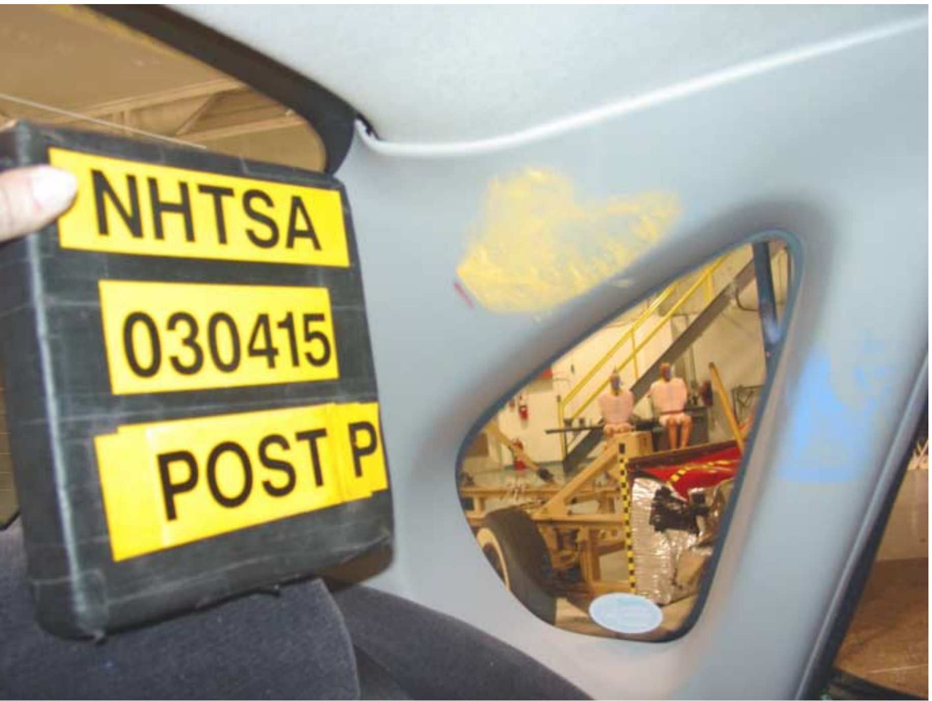
Figure A-42 Post-Test Rear SID H3 Contact - View 3
