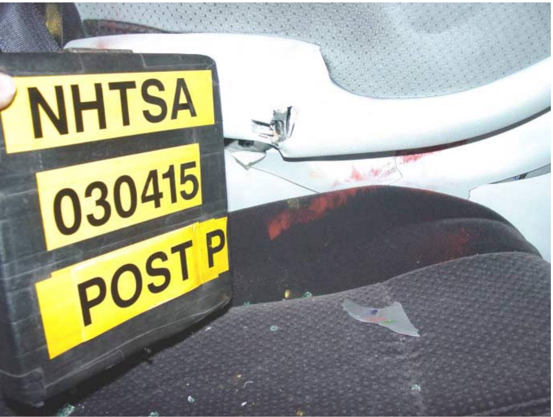
Figure A-40 Post-Test Rear SID H3 Contact - View 1
