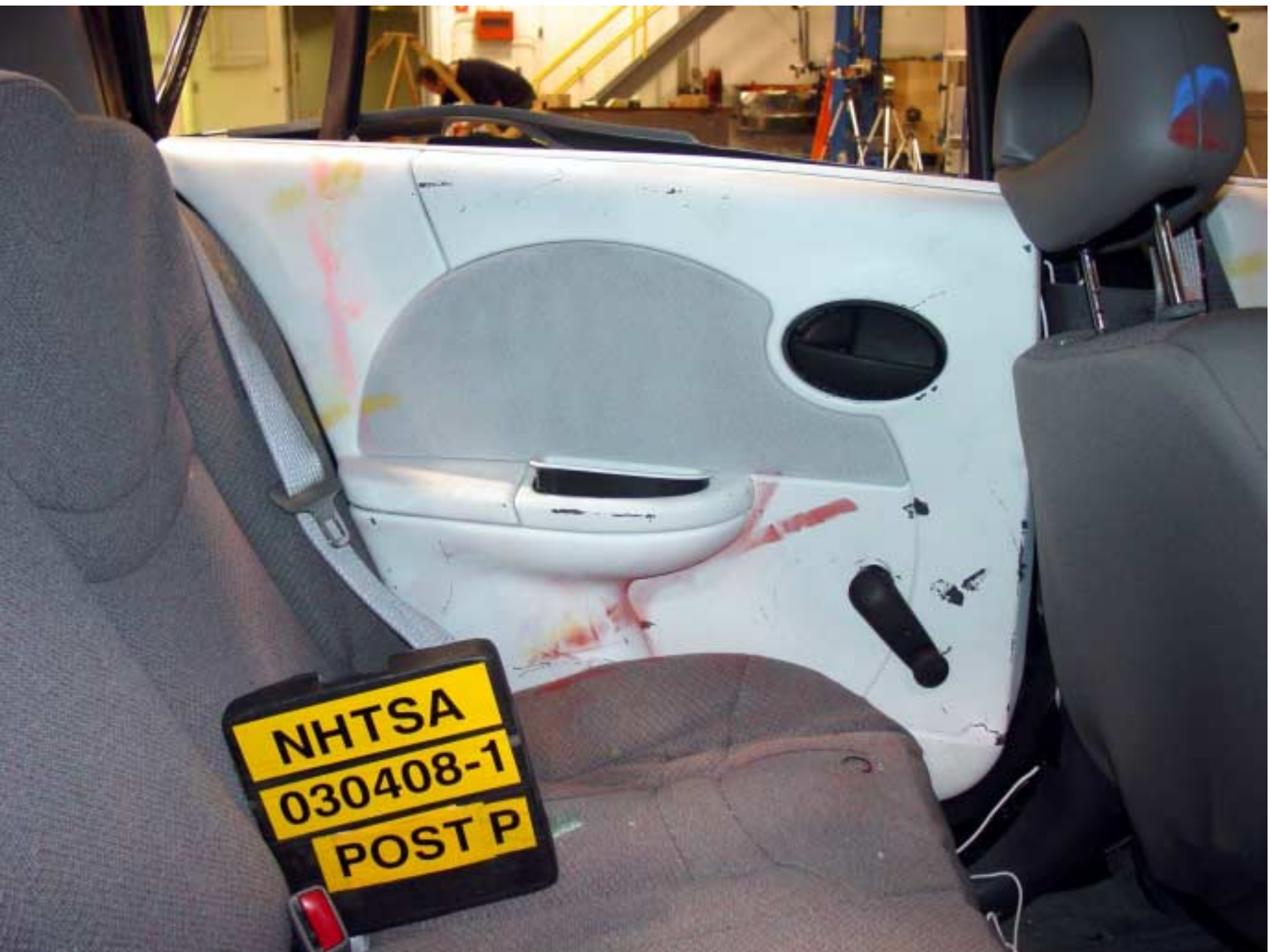
Figure A-38 Post-Test Interior of Rear Door Showing SID Impact Locations
