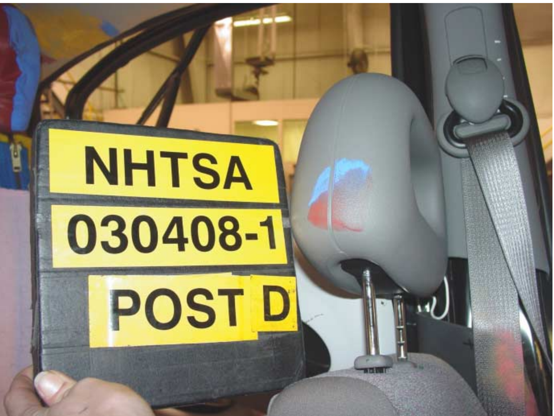
Figure A-36 Post-Test Front SID Contact - View 3
