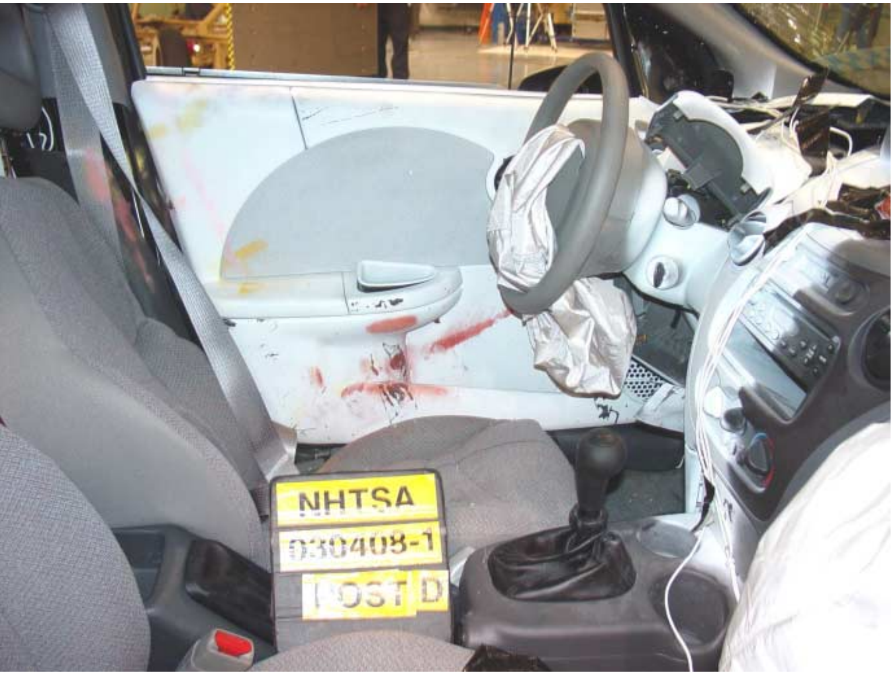
Figure A-33 Post-Test Interior of Front Door Showing SID Impact Locations
