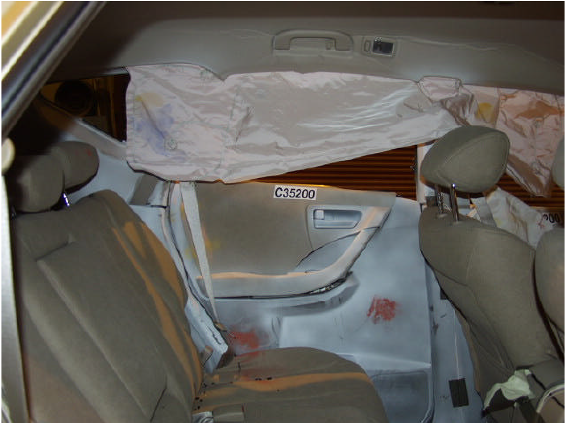
Figure A-36 POST-TEST INTERIOR OF REAR DOOR SHOWING SID H3 IMPACT LOCATIONS
