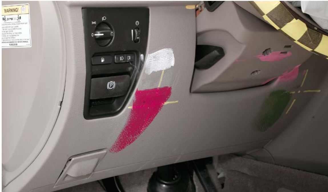
Figure 4 Dummy Left Knee/Shin Contacts, Postcrash — 2003 Volvo XC90
