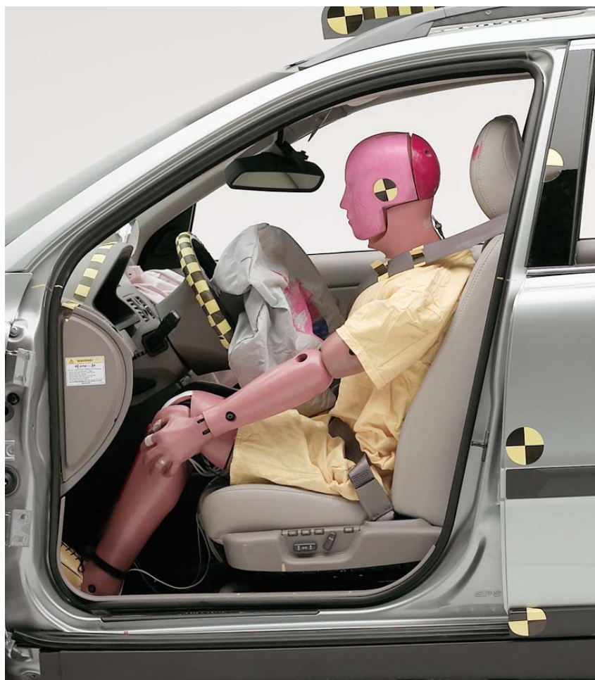
Figure 3 Dummy and Vehicle Interior, Postcrash — 2003 Volvo XC90
