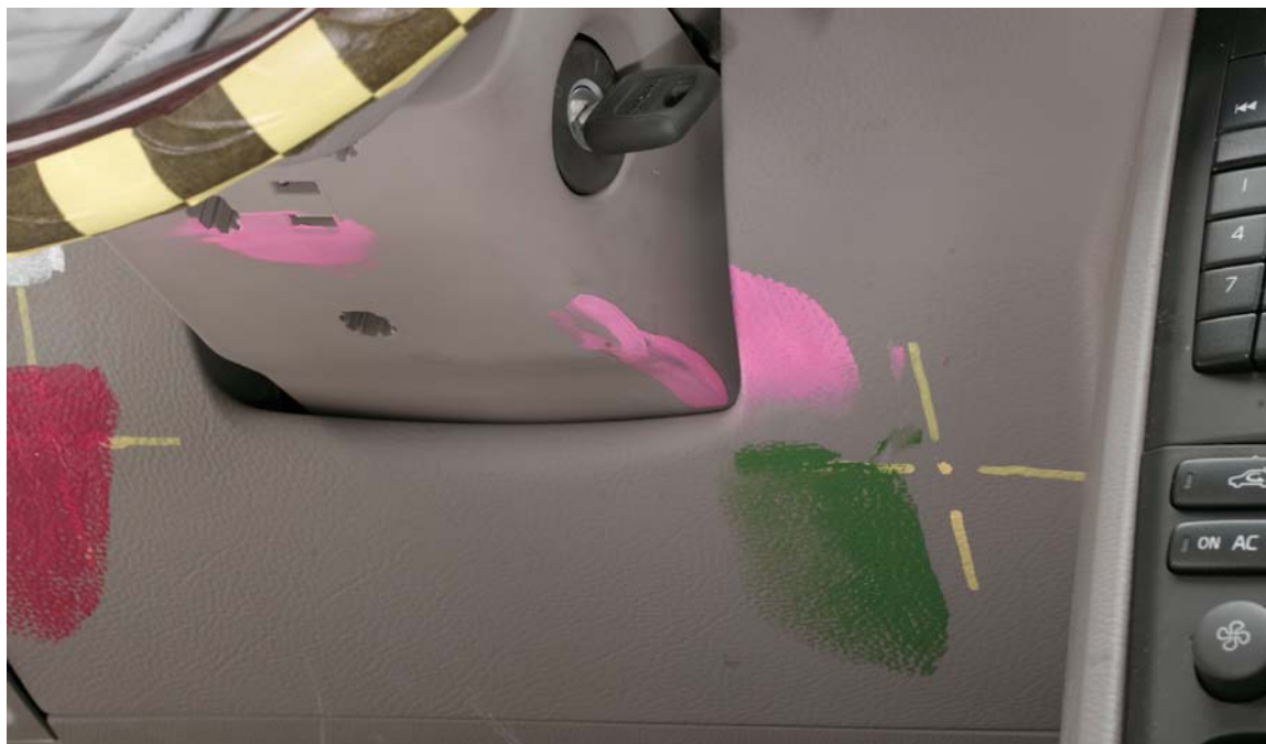
Figure 5 Dummy Right Knee/Shin Contacts, Postcrash — 2003 Volvo XC90
