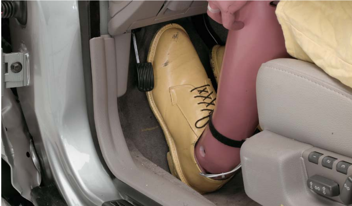
Figure 6 Dummy Feet Positions, Postcrash — 2003 Volvo XC90
