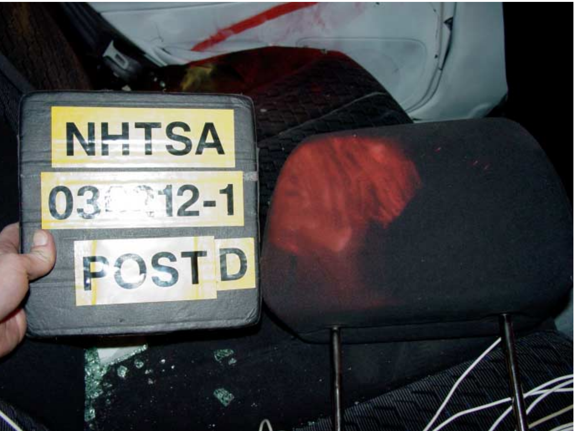
Figure A-32 Post-Test Front SID Contact
