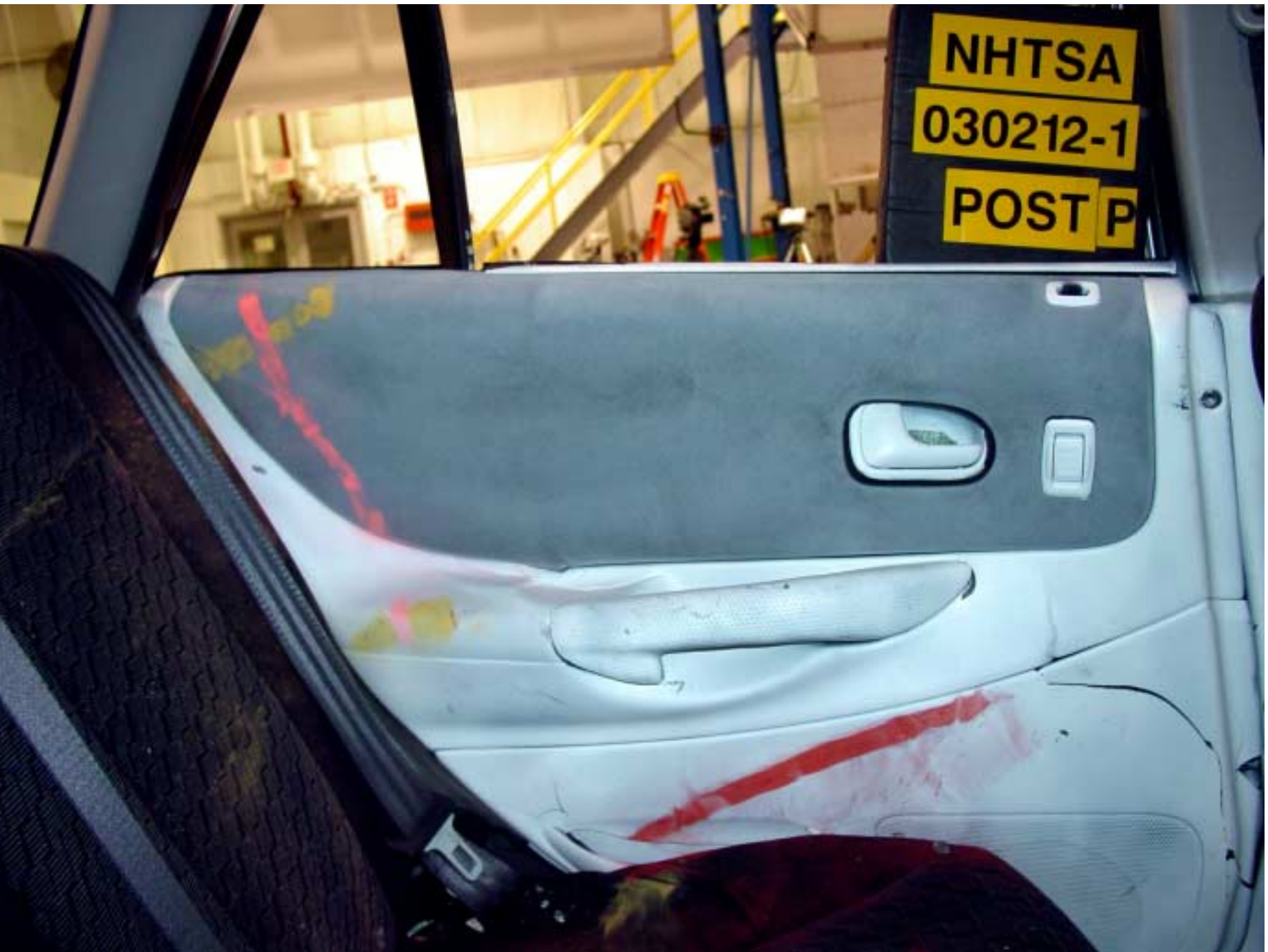
Figure A-34 Post-Test Interior of Rear Panel Showing SID Impact Locations
