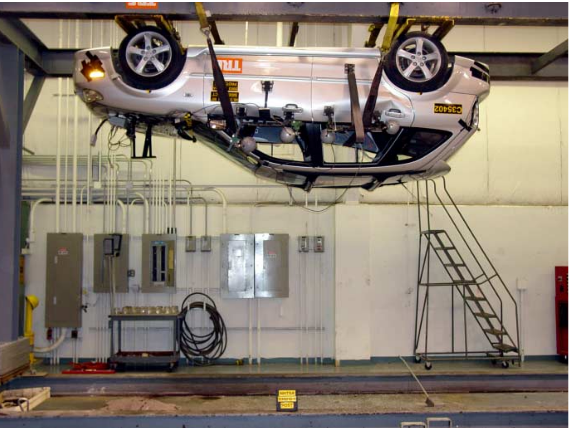
Figure A-49 FMVSS 301 Rollover View at 180°
