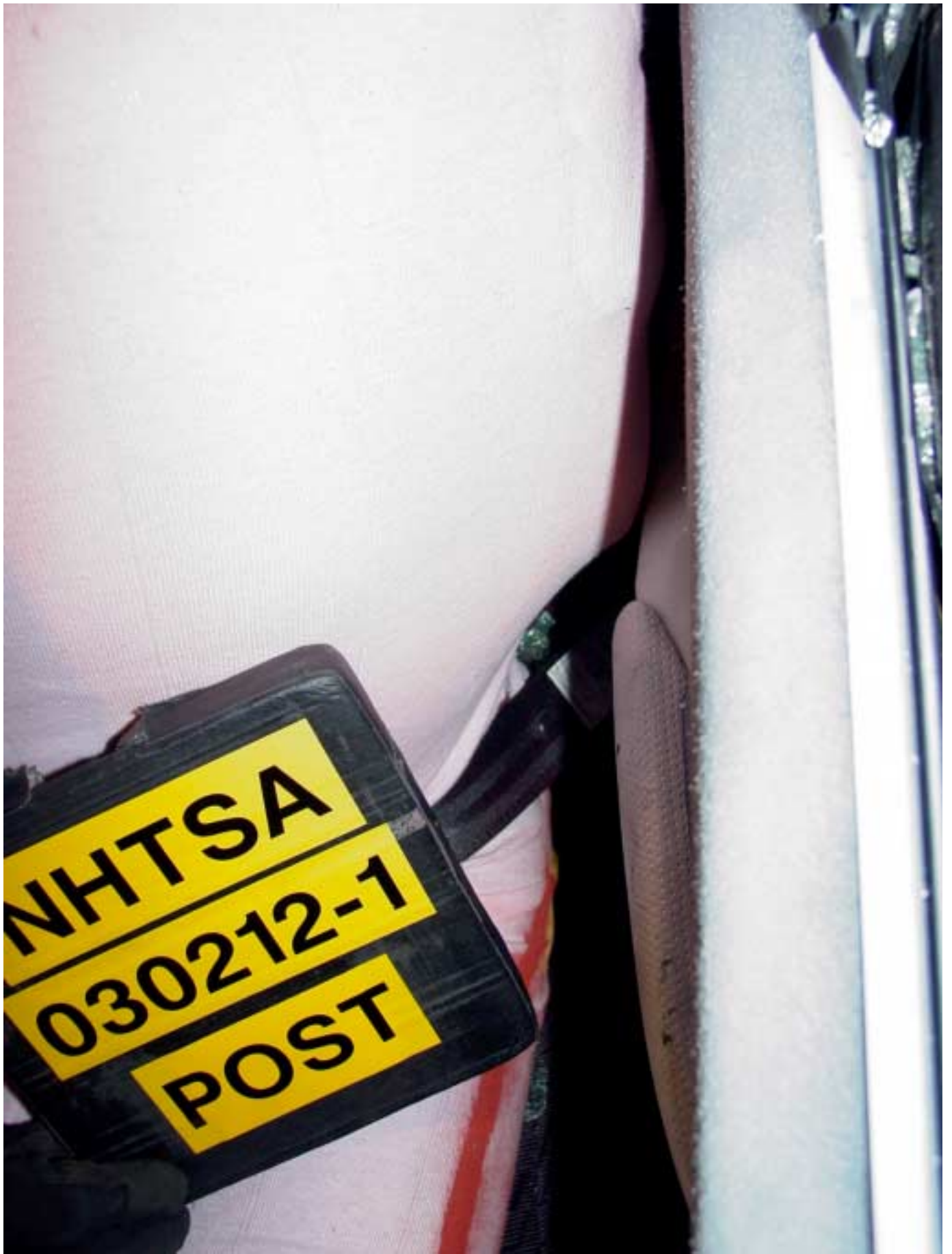
Figure A-29 Post-Test Left View of Rear SID and Door Clearance
