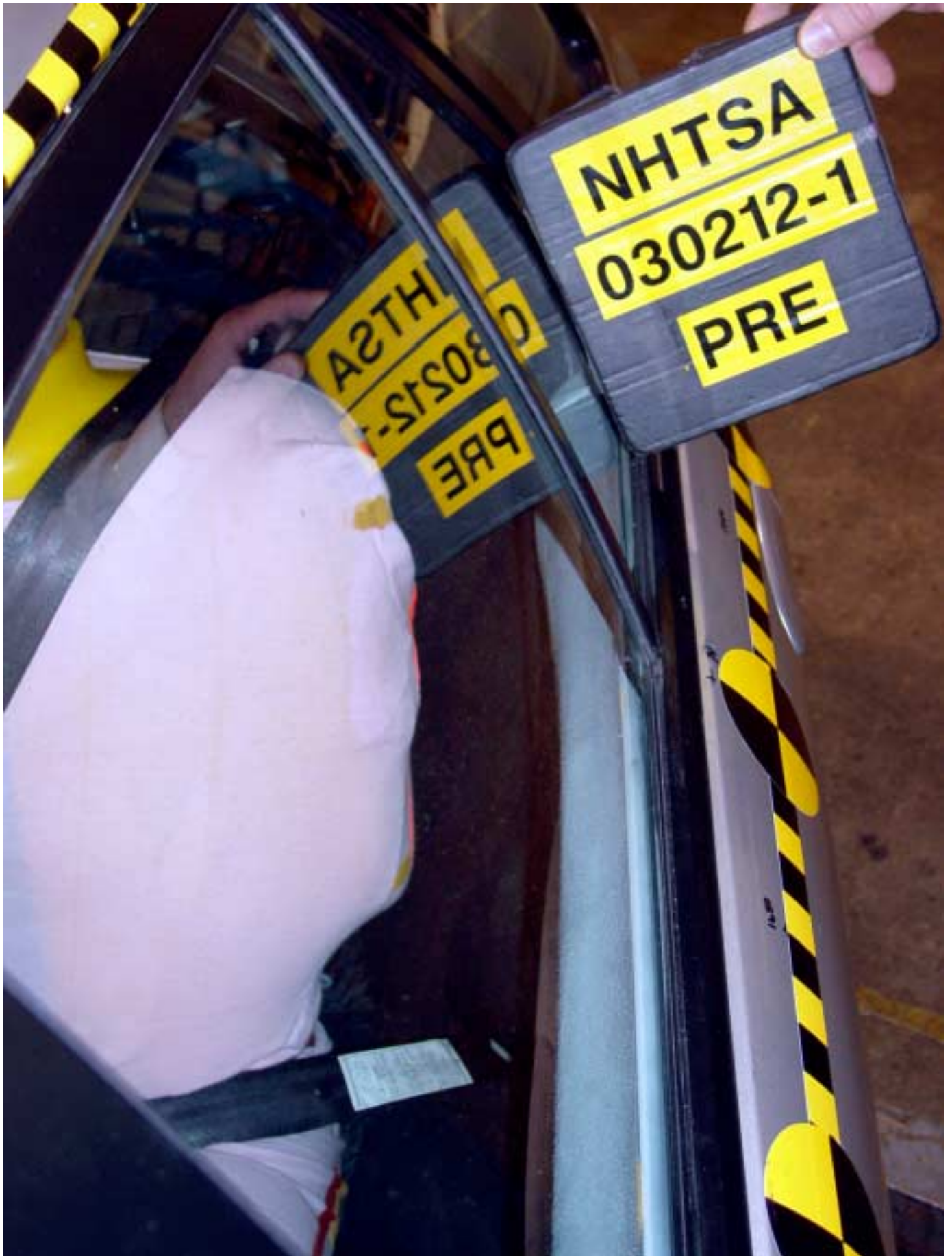
Figure A-28 Pre-Test Left View of Rear SID and Door Clearance
