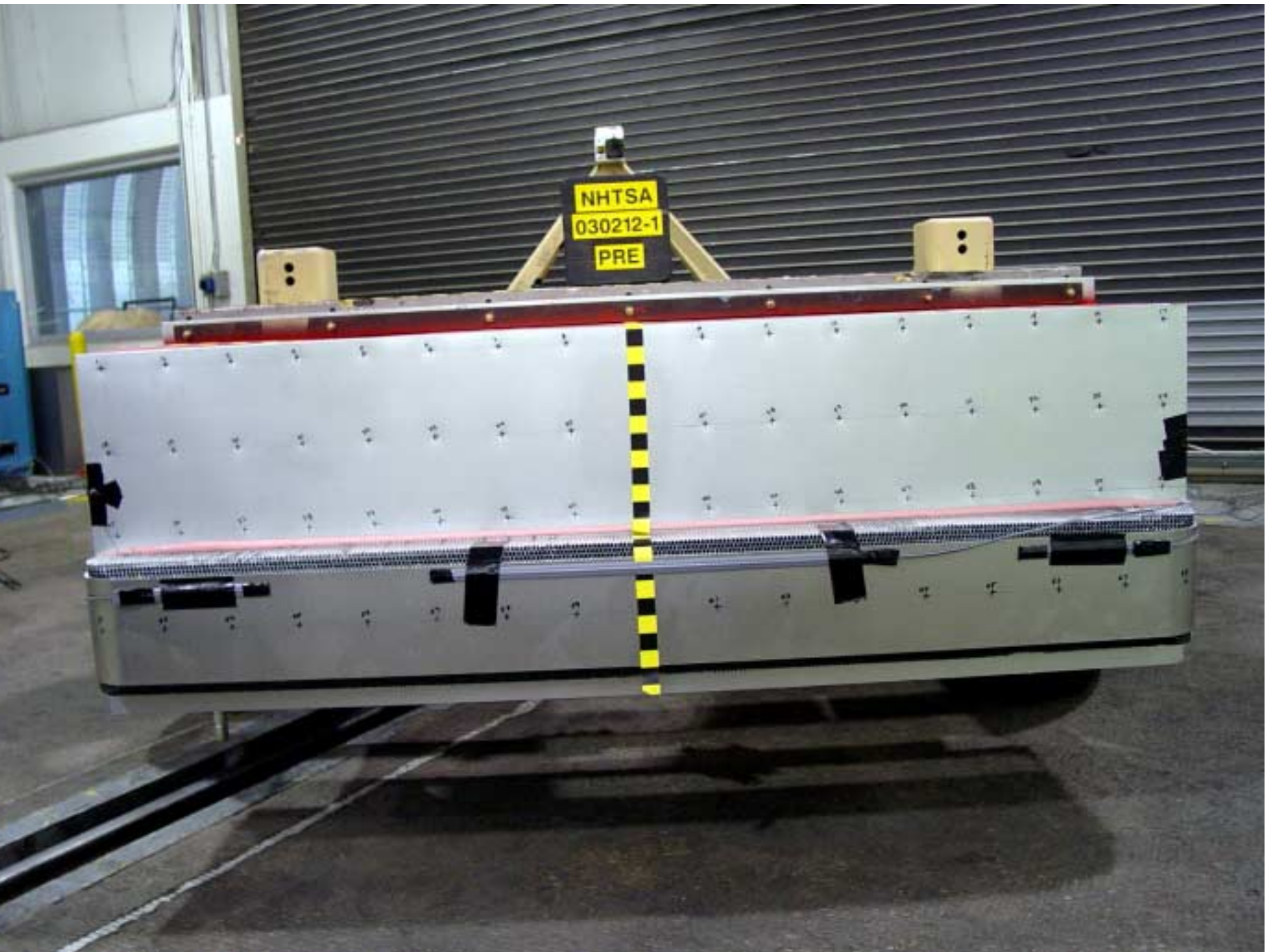
Figure A-15 Pre-Test View of MDB Showing Contact Switches in Place
