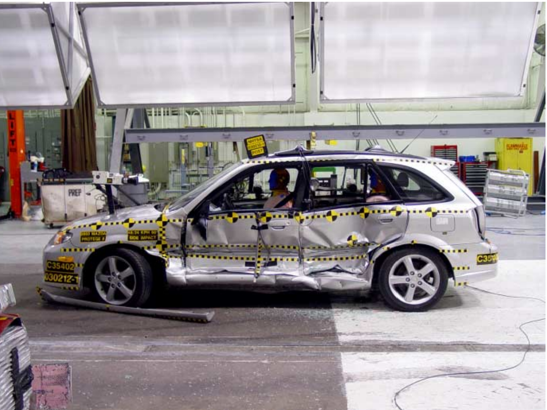
Figure A-4 Post-Test Impacted Side View of Test Vehicle
