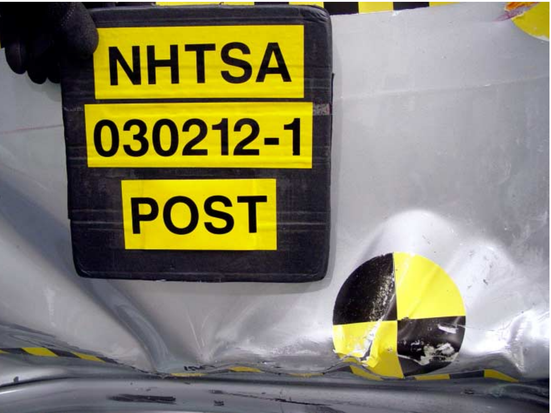
Figure A-42 Post-Test Secondary Impact Point View
