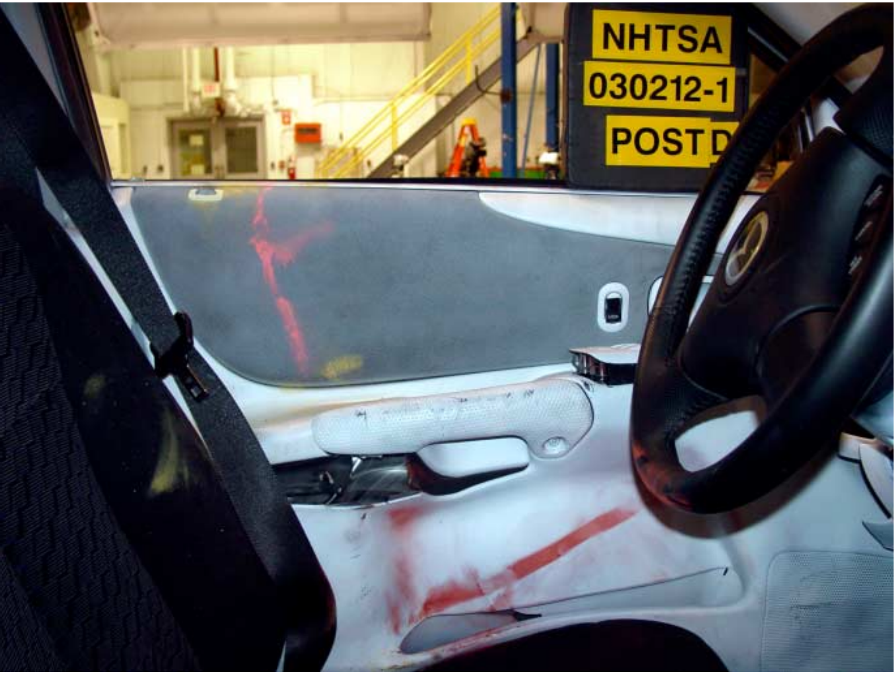
Figure A-31 Post-Test Interior of Front Door Showing SID Impact Locations
