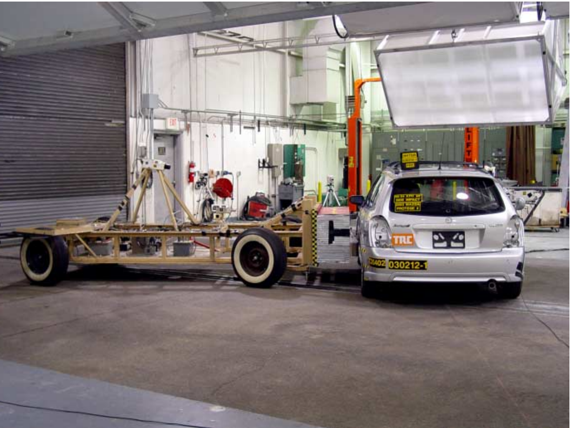
Figure A-40 Pre-Test Right Side View of MDB with Impactor Face in Position
