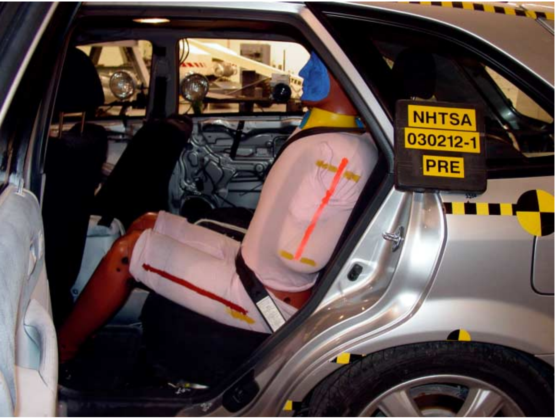
Figure A-27 Pre-Test Left View of Rear SID and Belt Position
