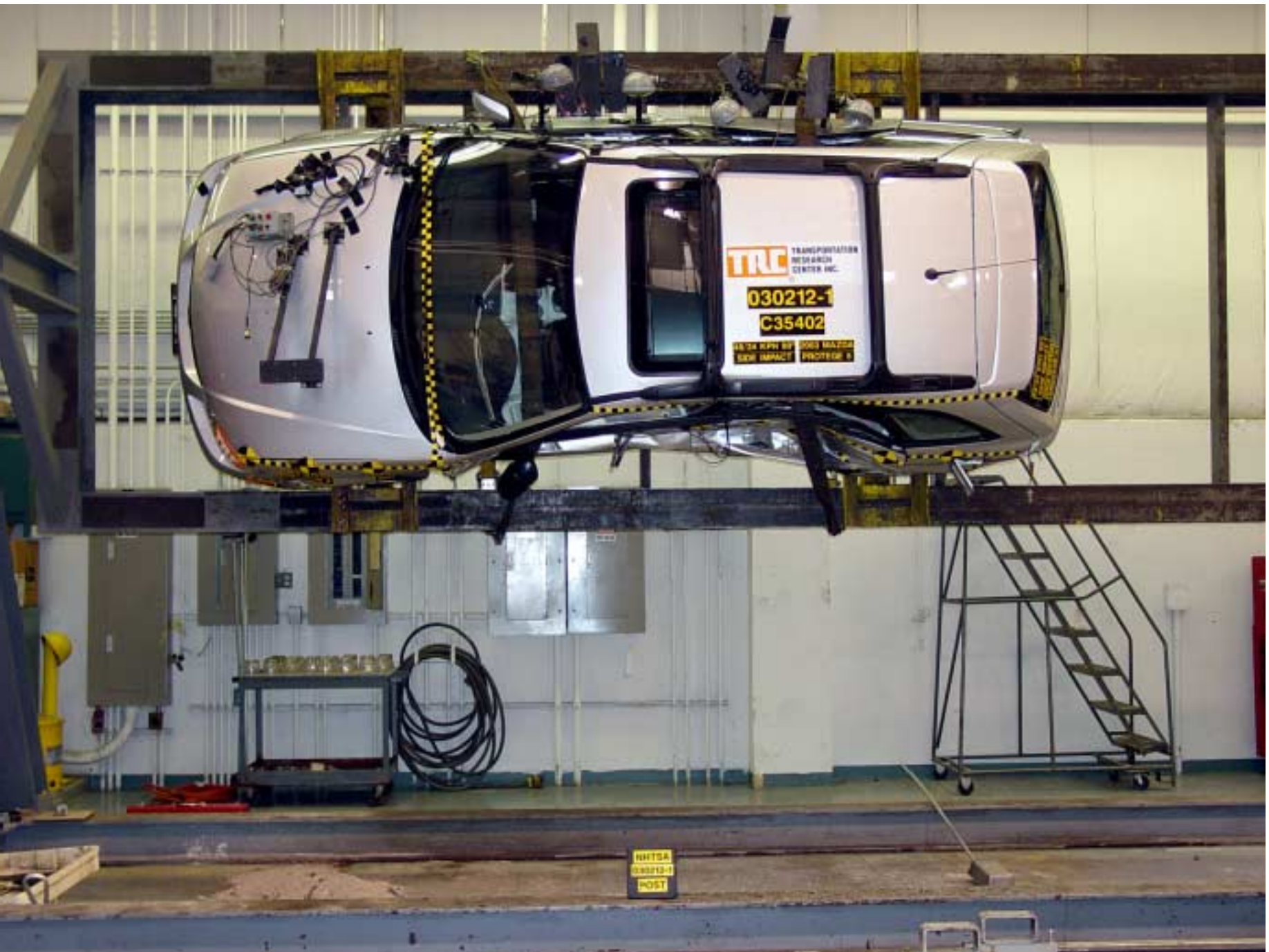
Figure A-48 FMVSS 301 Rollover View at 90°
