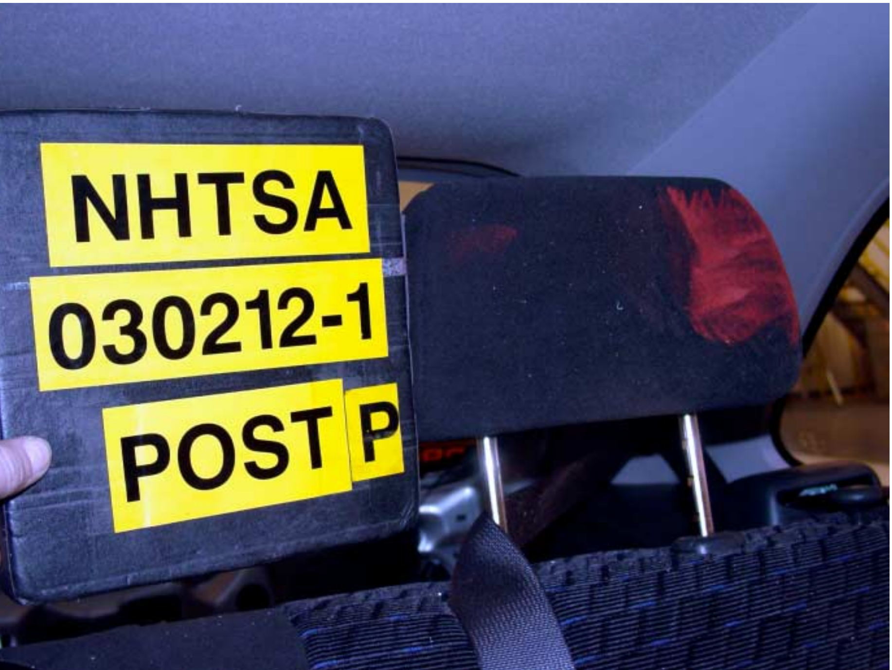
Figure A-36 Post-Test Rear SID Contact - View 2
