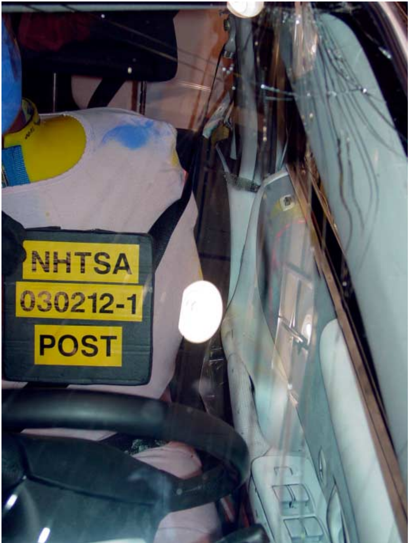
Figure A-25 Post-Test Left View of Front SID and Door Clearance
