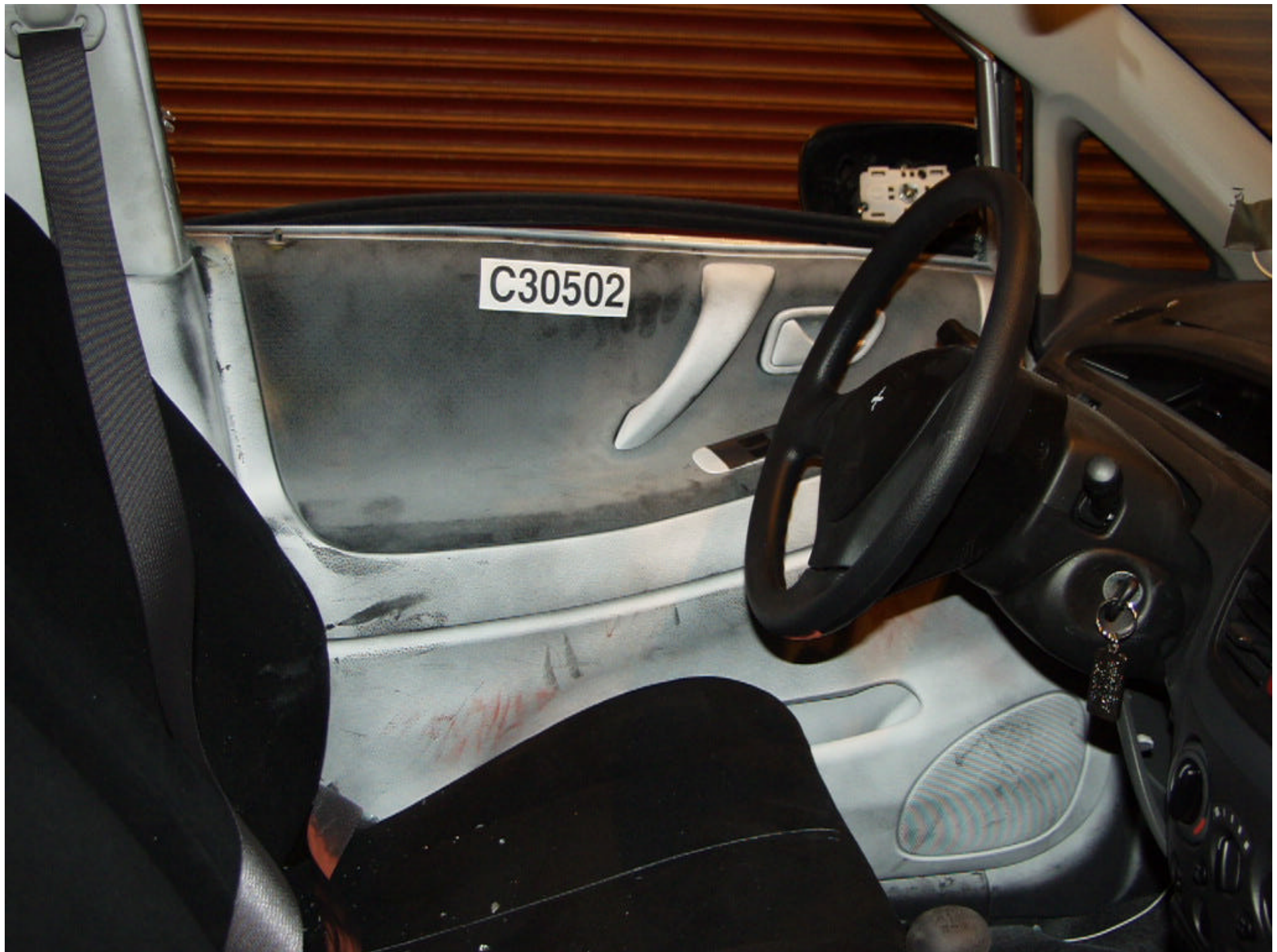
Figure A-26 POST-TEST INTERIOR OF FRONT DOOR SHOWING SID IMPACT LOCATIONS
