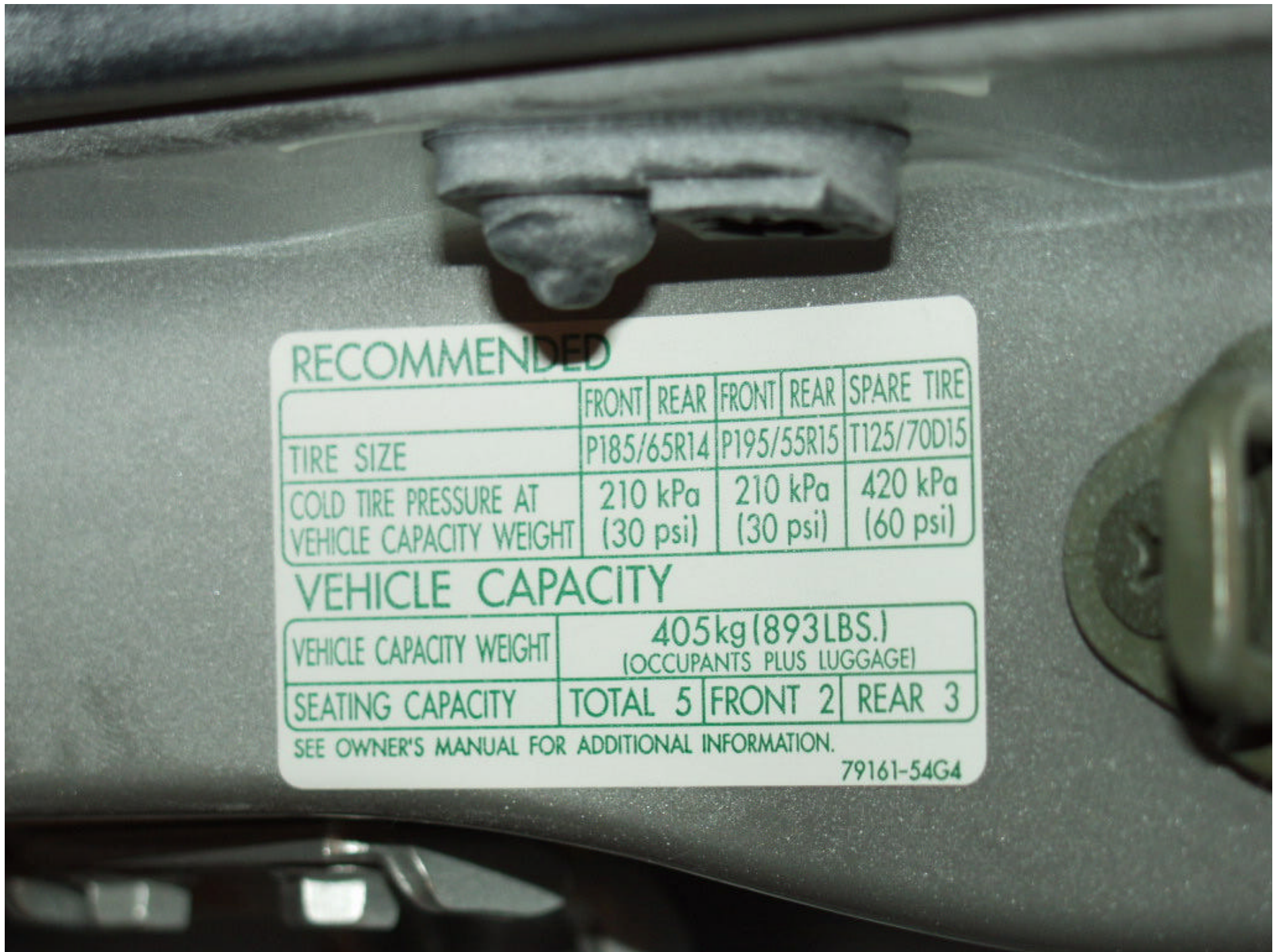
Figure A-33 CLOSE-UP VIEW OF VEHICLE'S TIRE PLACARD LABEL
