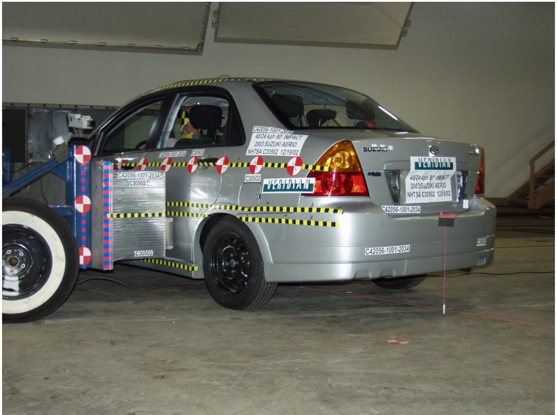
Figure A-30 PRE-TEST RIGHT SIDE VIEW OF MDB WITH IMPACTOR FACE IN POSITION
