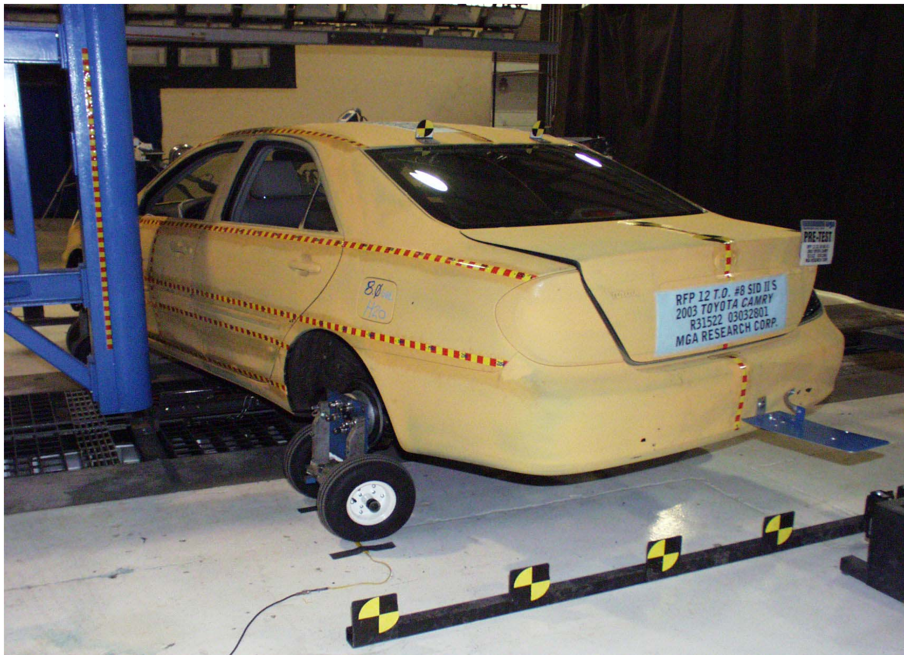
Pre-Test Vehicle Positioned Against Pole (right side)
