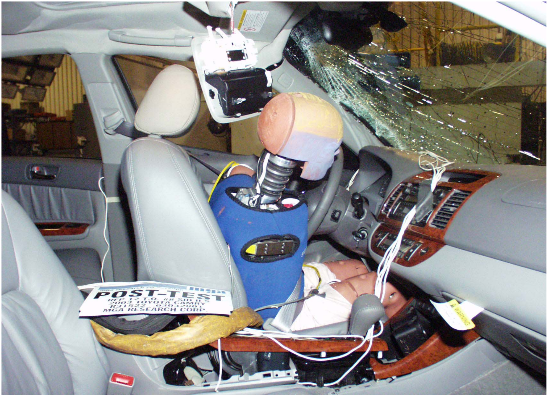
Post-Test Driver Dummy Right Side View
