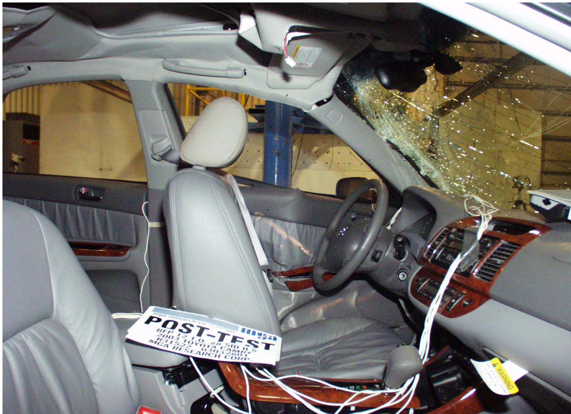
Post-Test Driver Dummy Contact
