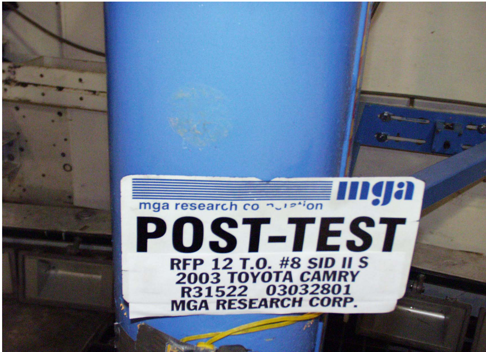
Dummy Head Contact With Pole
