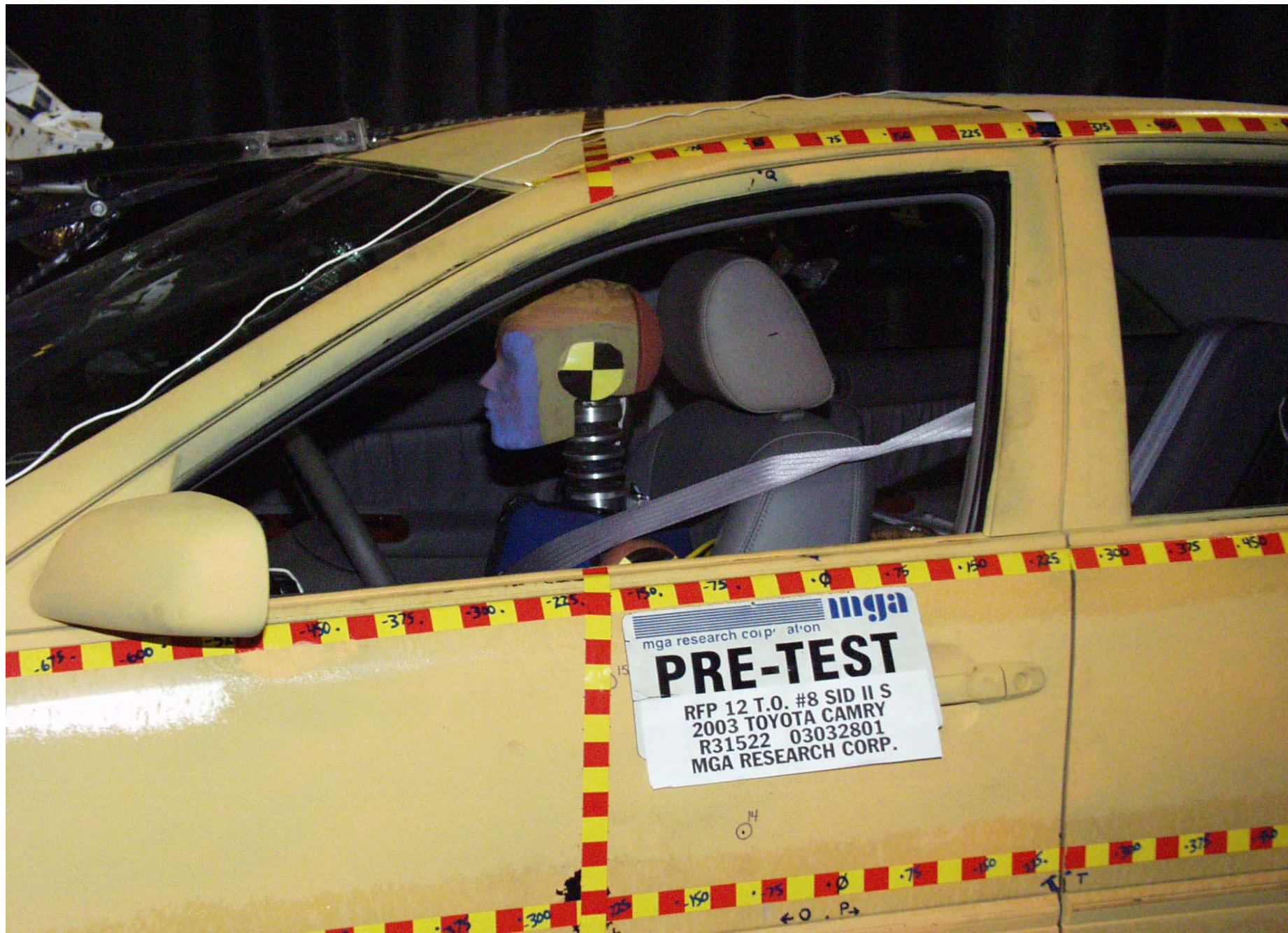
Pre-Test Driver Dummy Left Side View
