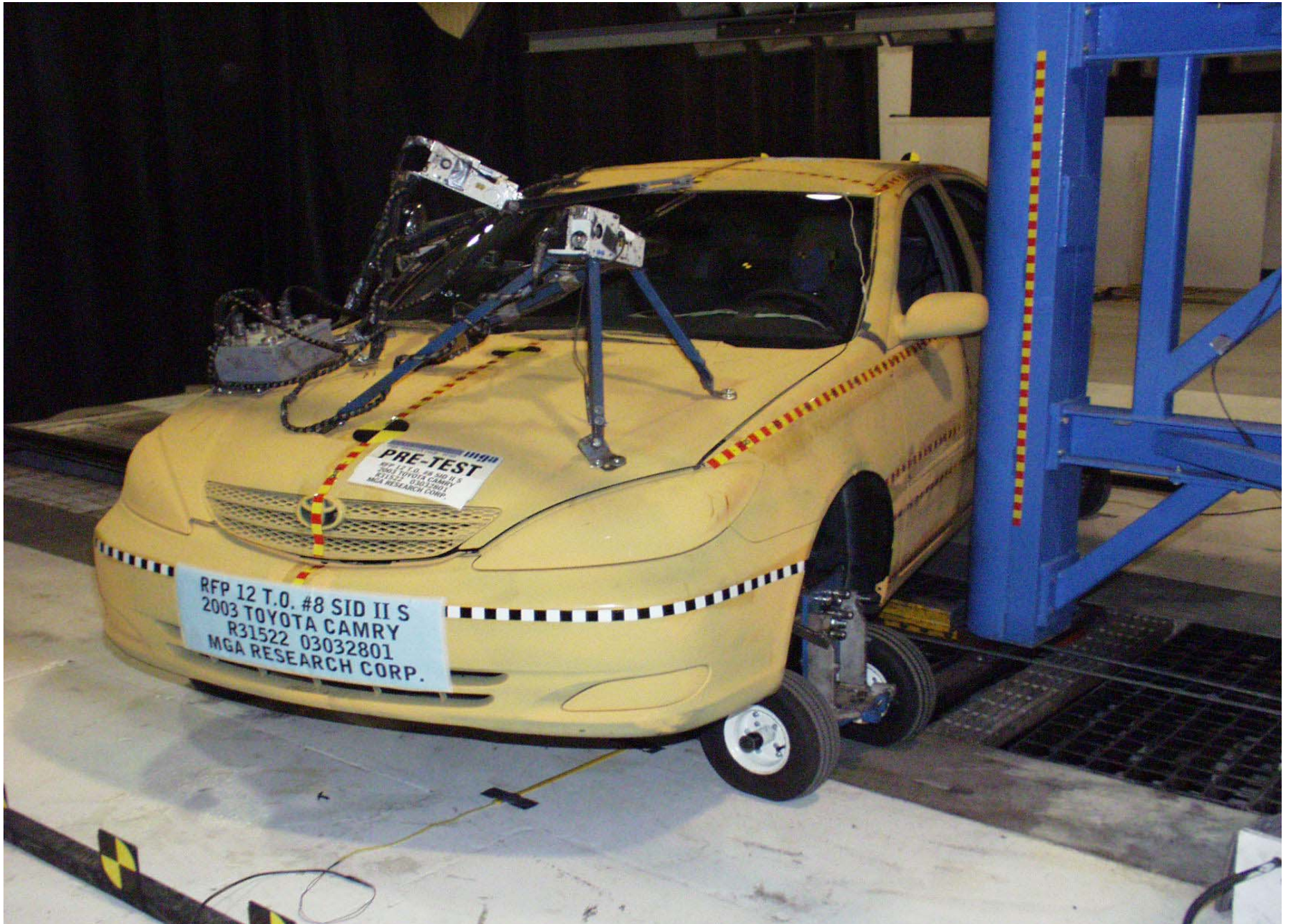
Pre-Test Vehicle Positioned Against Pole (left side)
