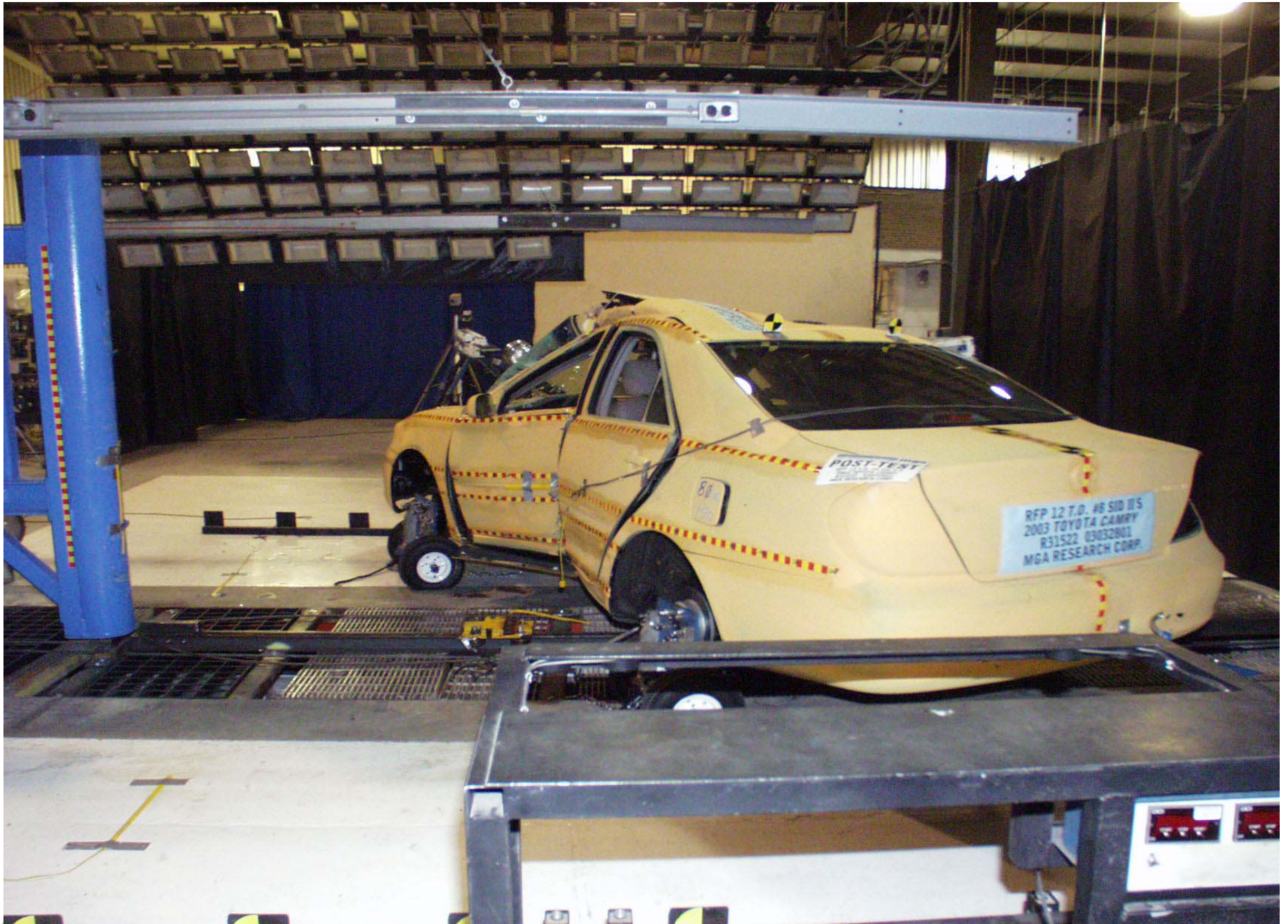
Post-Test Pole and Vehicle (right side)
