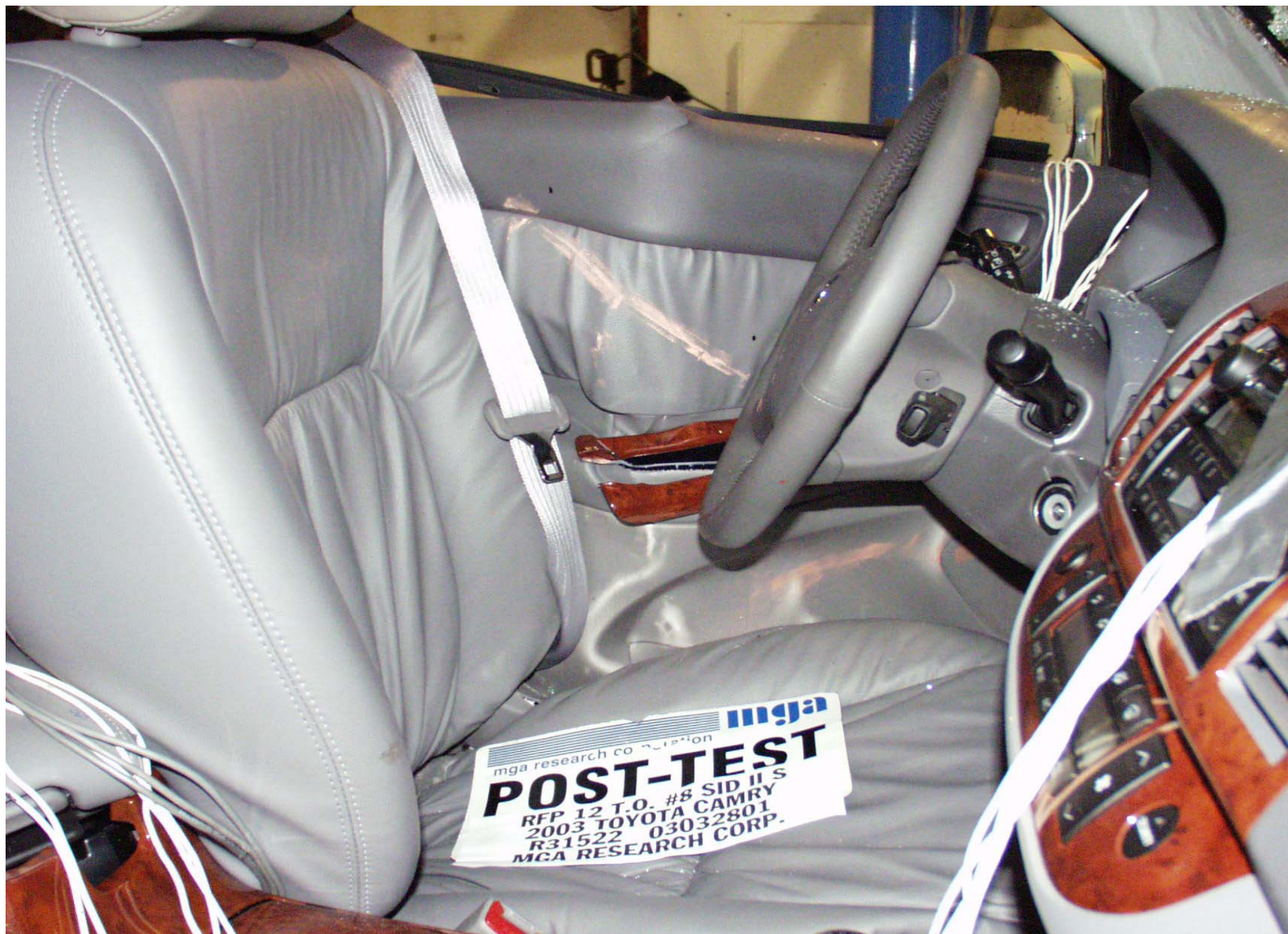
Post-Test Driver Dummy Lower Body Contact
