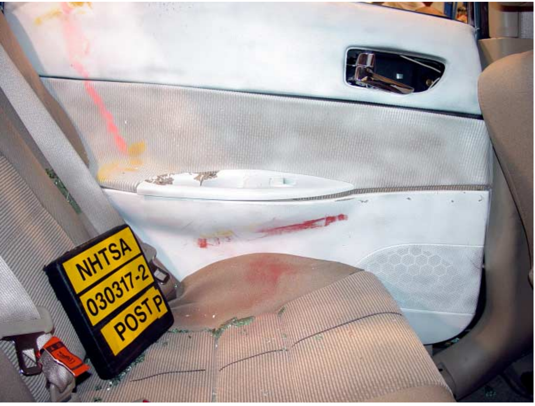
Figure A-39 Post-Test Interior of Rear Door Showing SID Impact Locations
