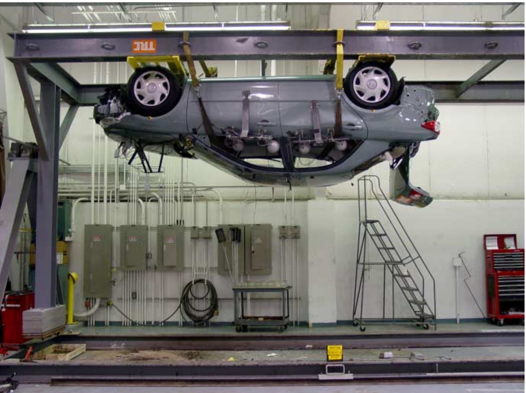
Figure A-55 FMVSS 301 Rollover View at 180°
