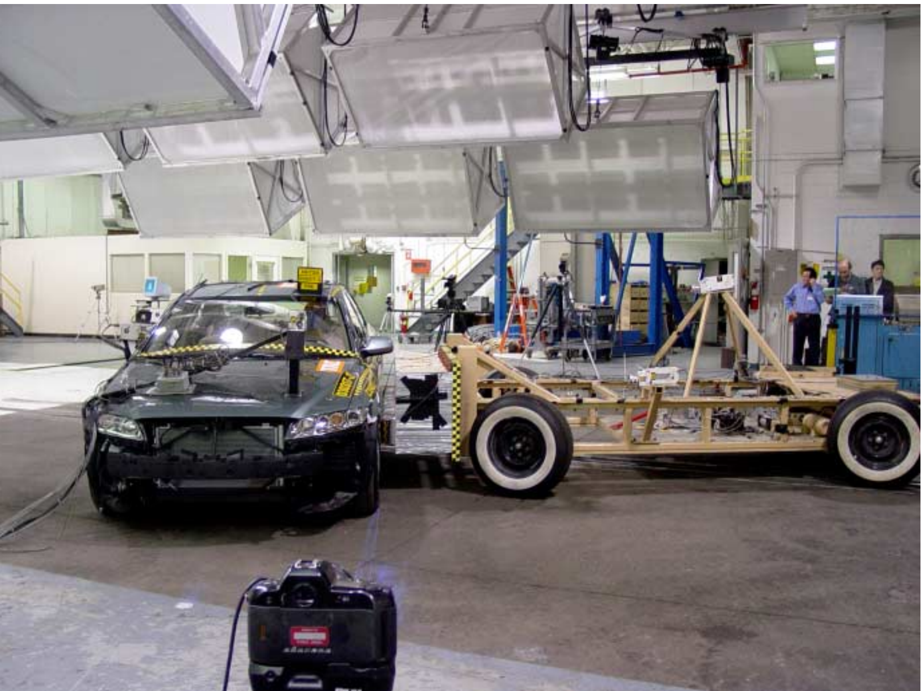
Figure A-43 Pre-Test Left Side View of MDB With Impactor Face in Position
