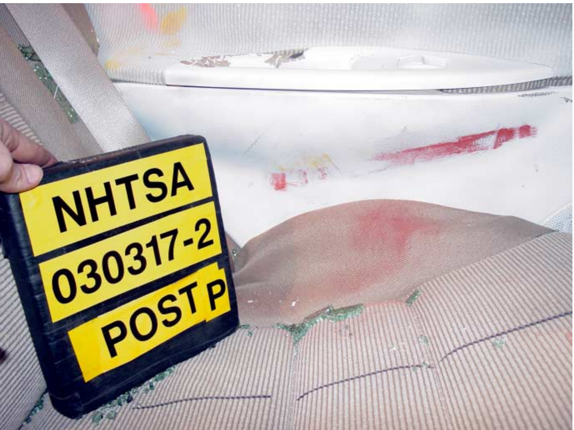
Figure A-42 Post-Test Rear SID Contact - View 3
