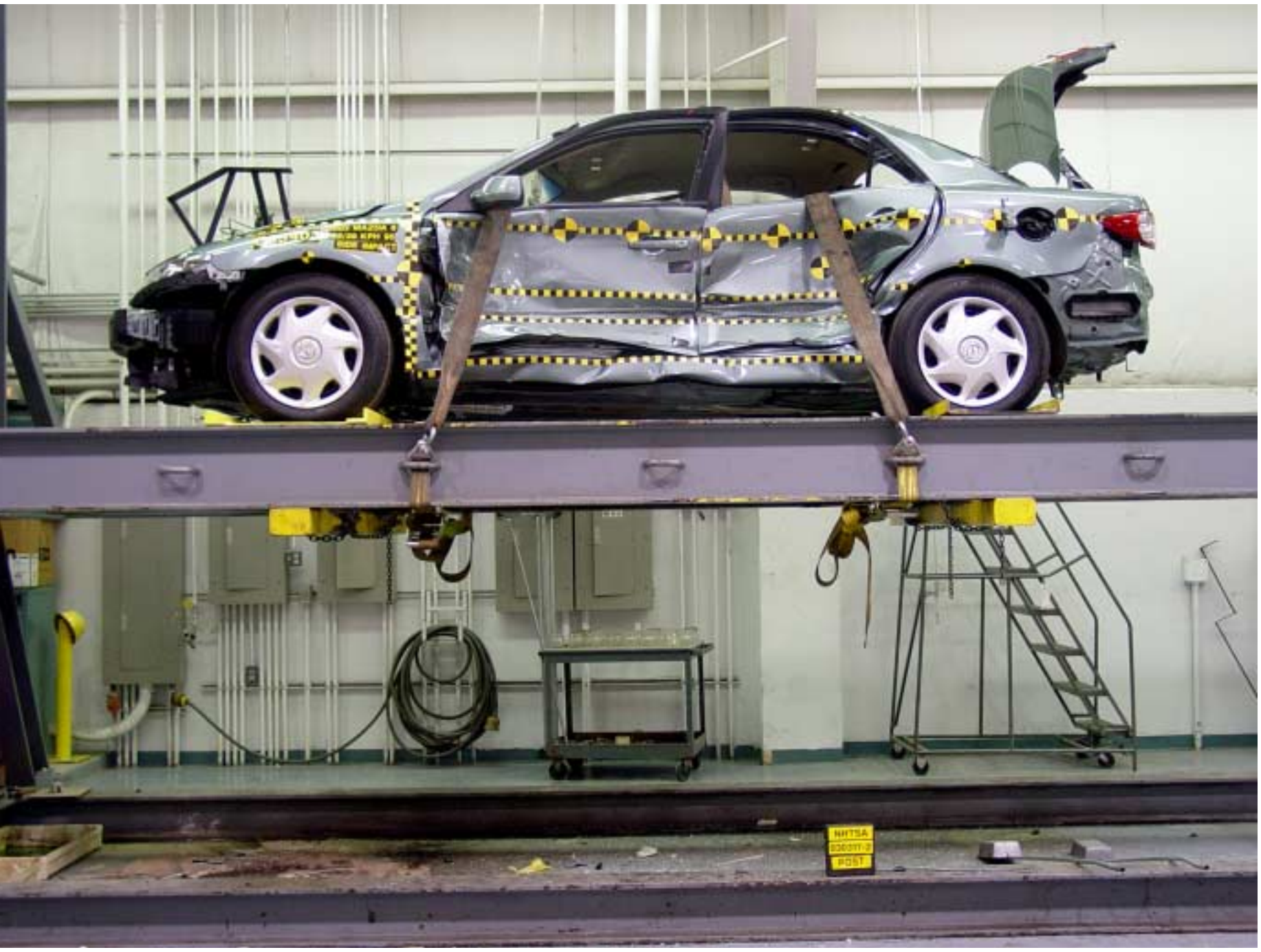
Figure A-57 FMVSS 301 Rollover View at 360°
