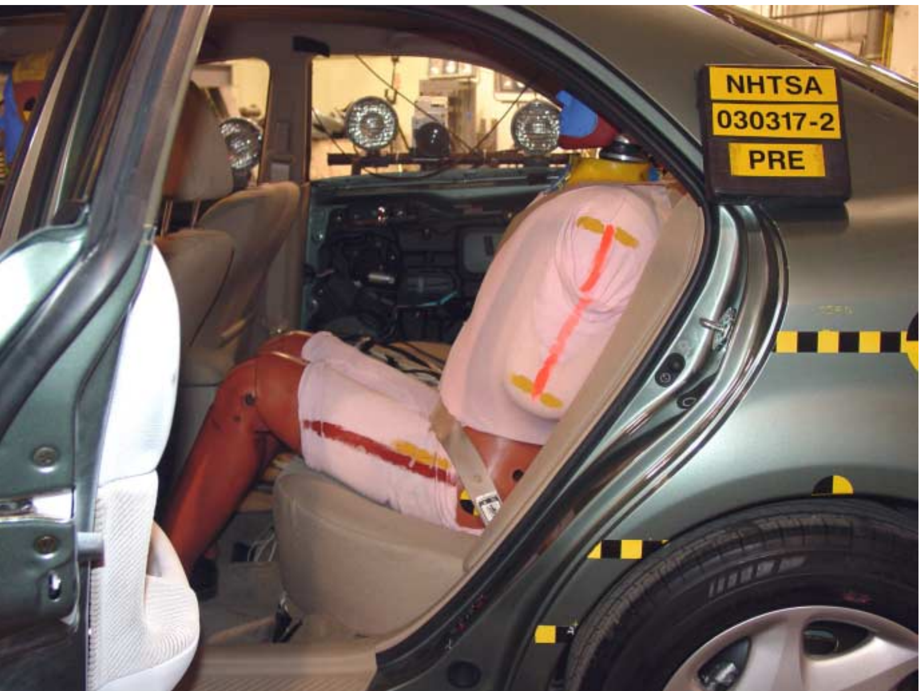
Figure A-29 Pre-Test Left of Rear SID and Belt Position
