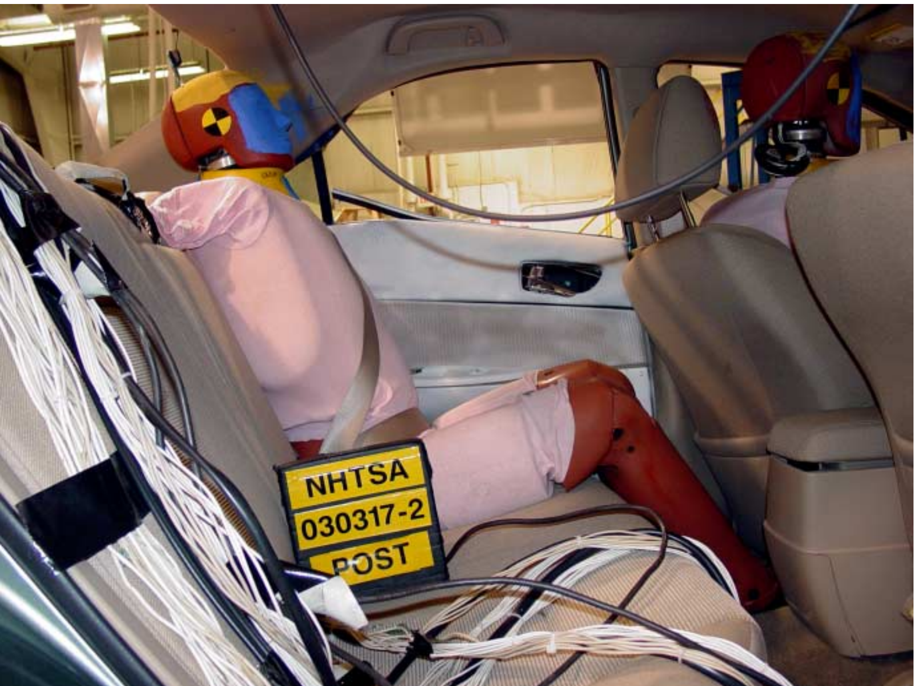
Figure A-21 Post-Test Right Occupant Compartment View of Rear SID
