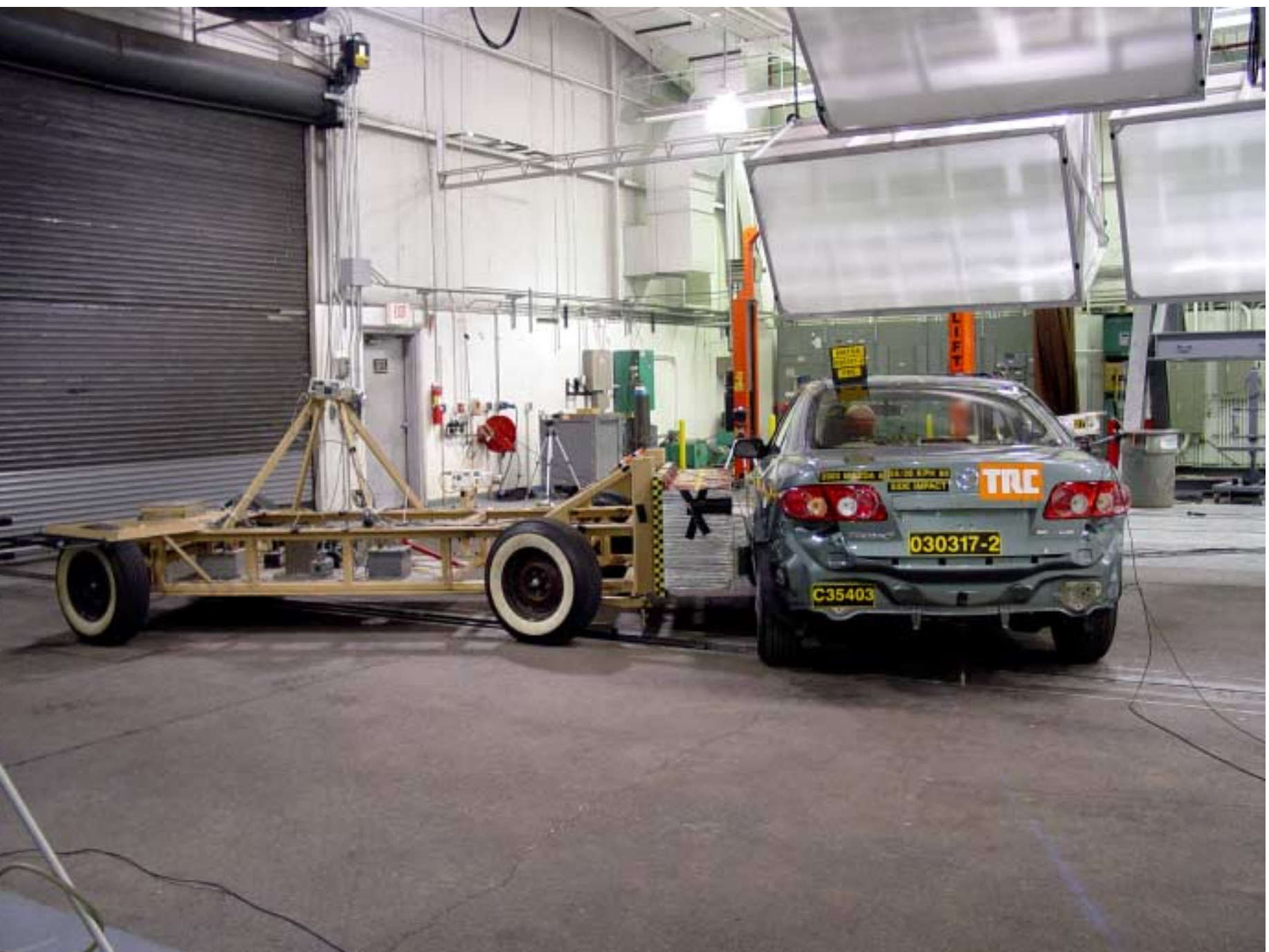
Figure A-46 Pre-Test Right Side View of MDB With Impactor Face in Position
