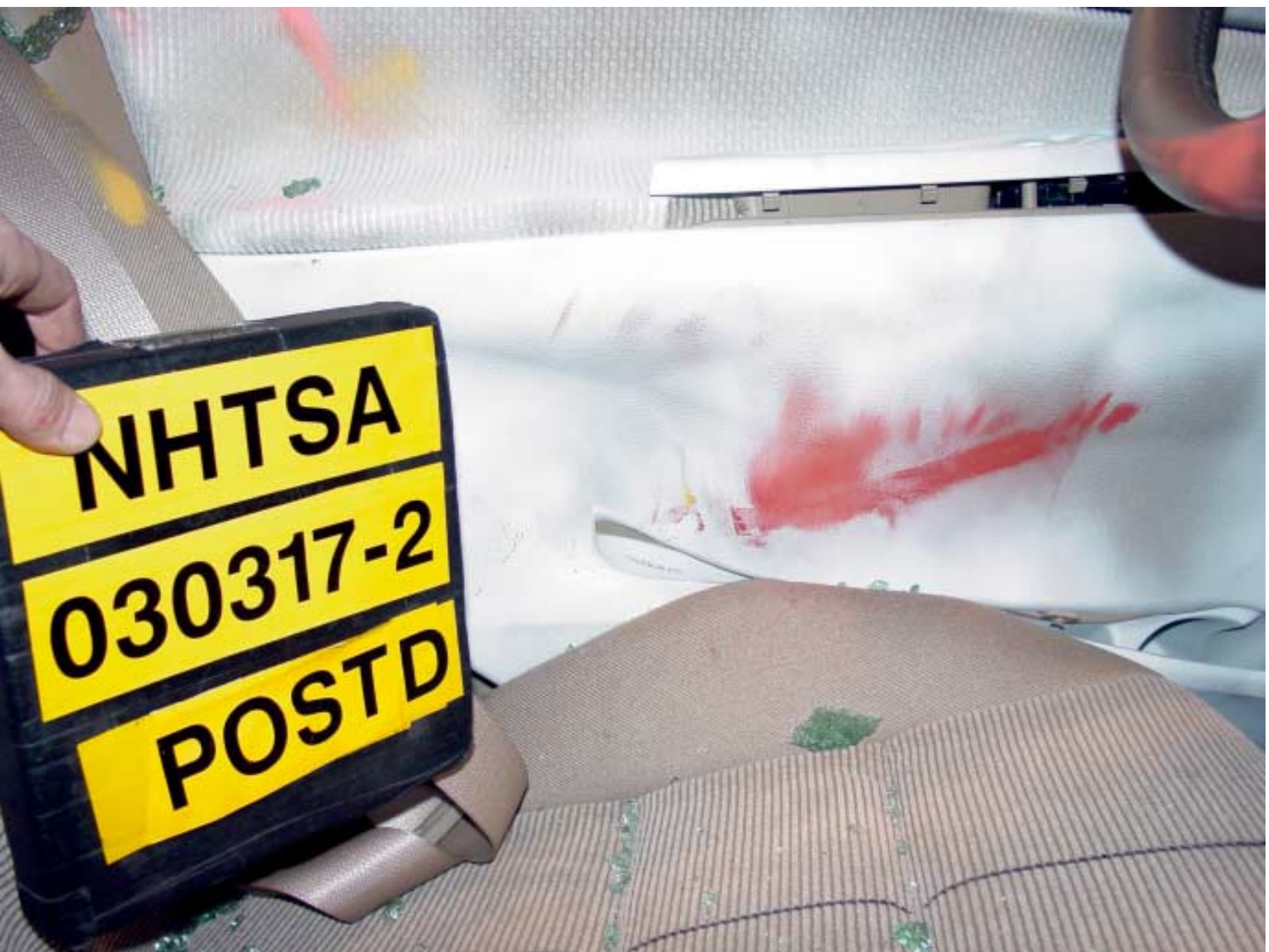
Figure A-35 Post-Test Front SID Contact – View 2
