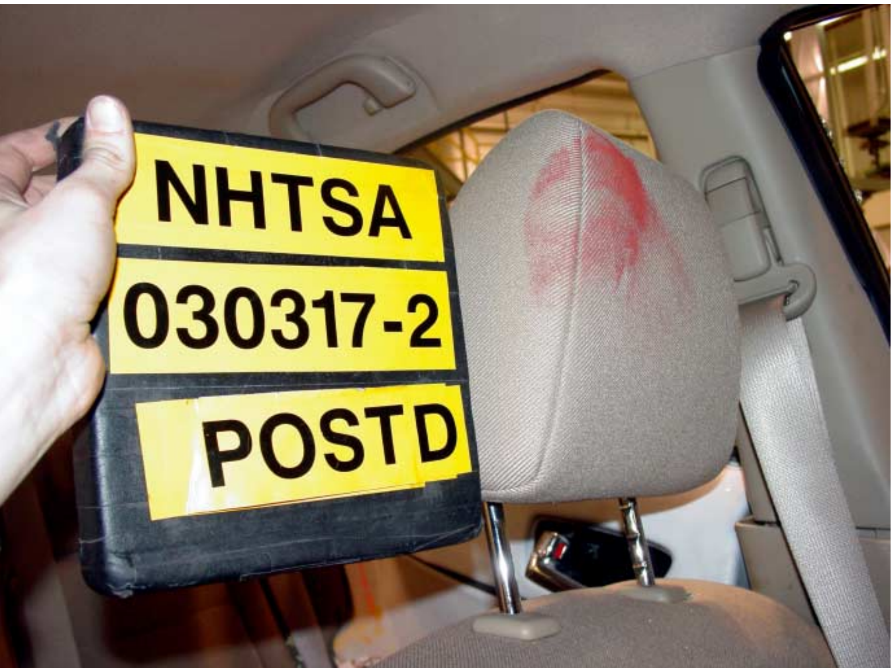
Figure A-34 Post-Test Front SID Contact – View 1
