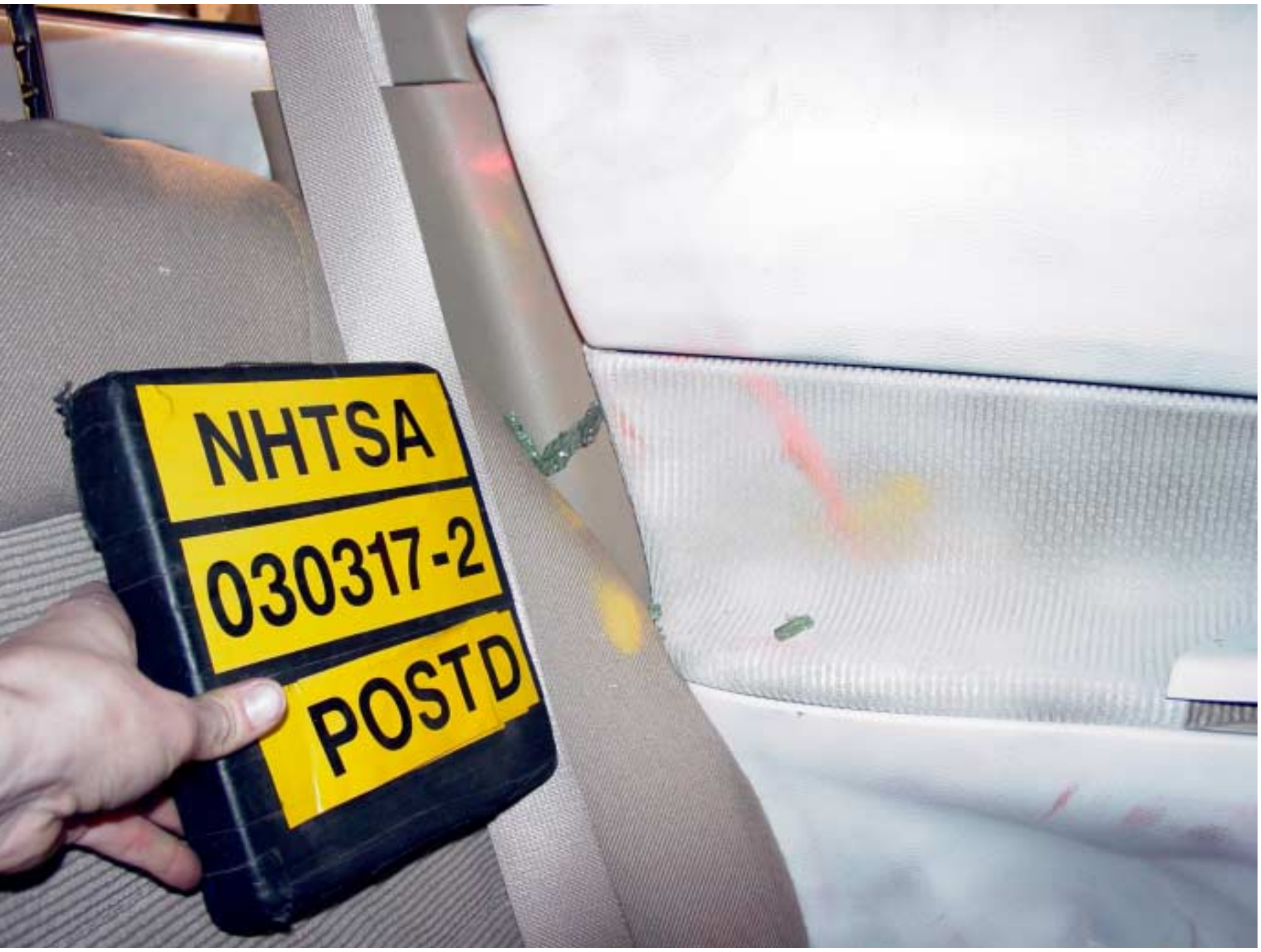
Figure A-36 Post-Test Front SID Contact – View 3
