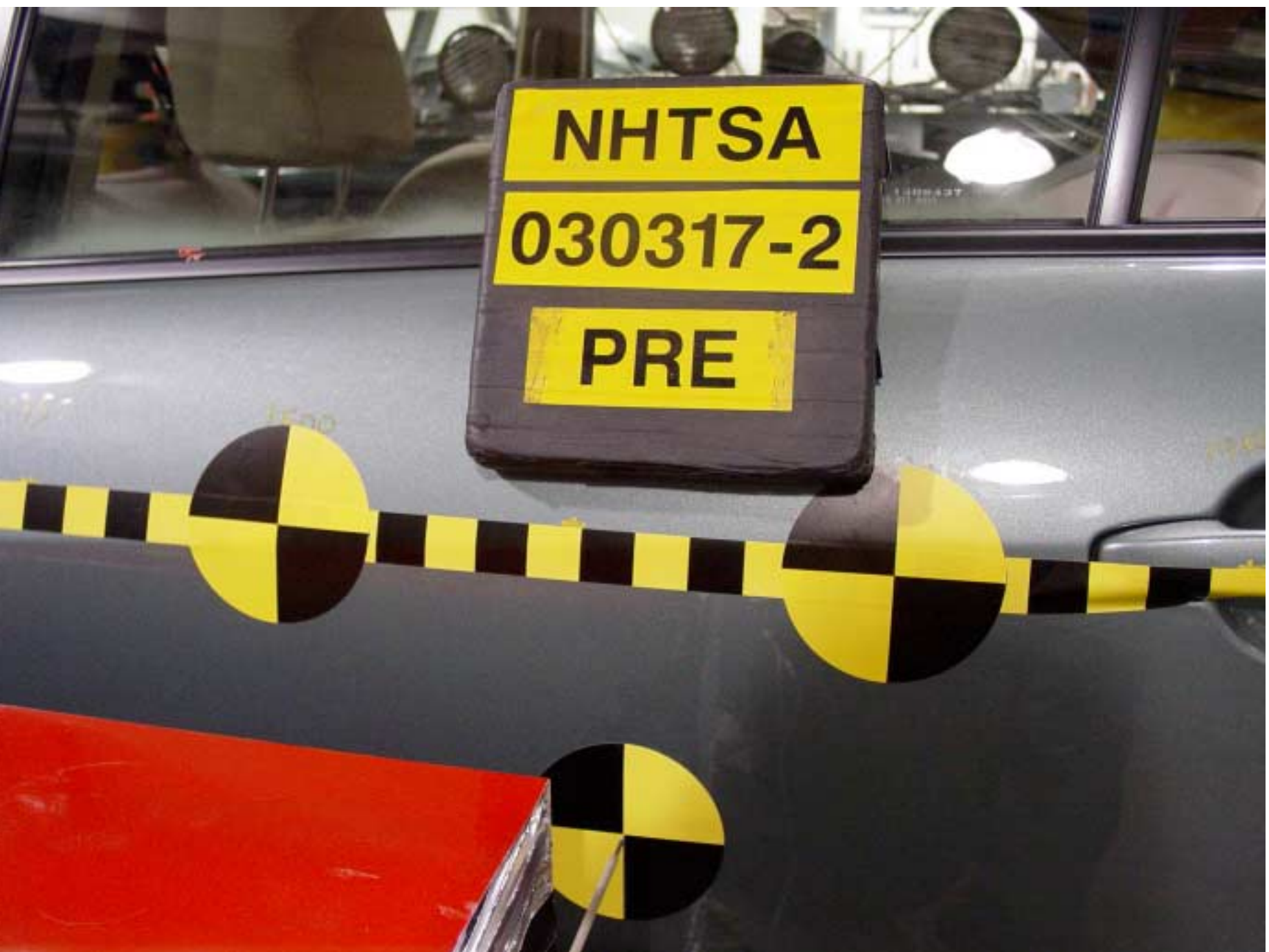
Figure A-47 Pre-Test Secondary Impact Point View
