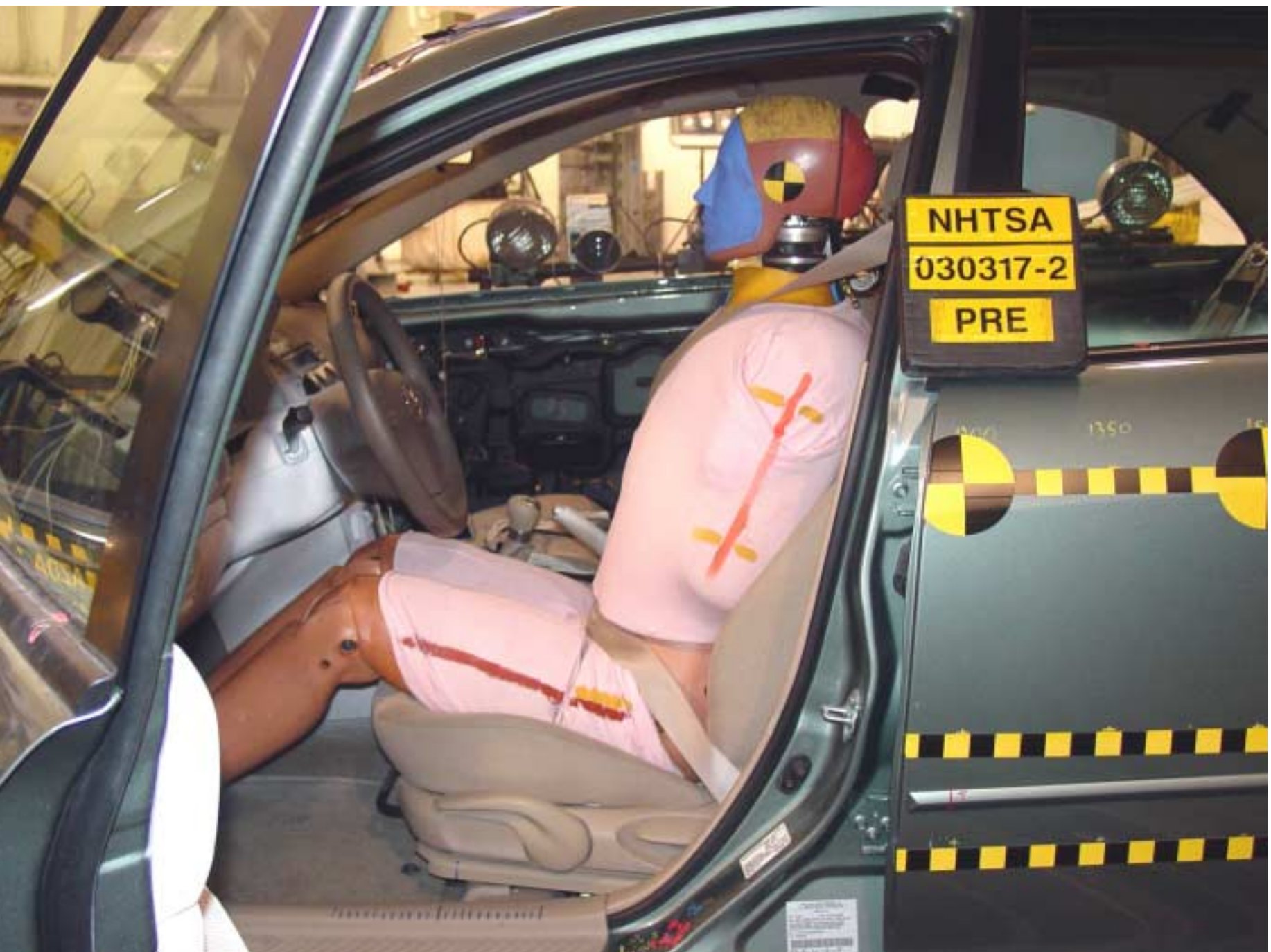
Figure A-24 Pre-Test Left View of Front SID and Belt Position
