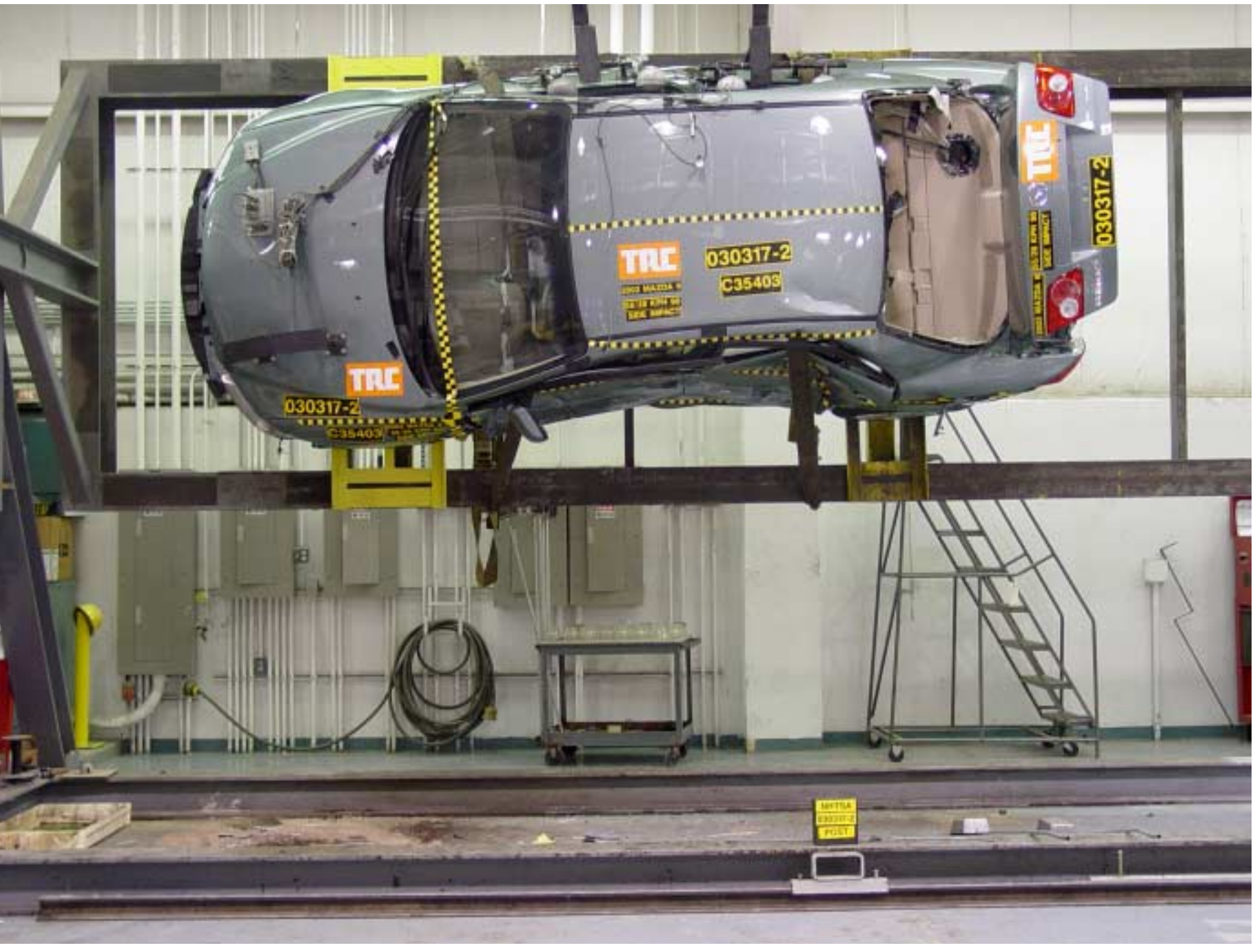
Figure A-54 FMVSS 301 Rollover View at 90°
