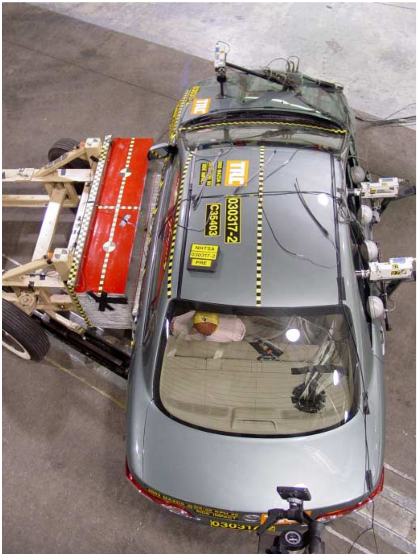
Figure A-16 Pre-Test Overhead View of MDB Aligned with Vehicle
