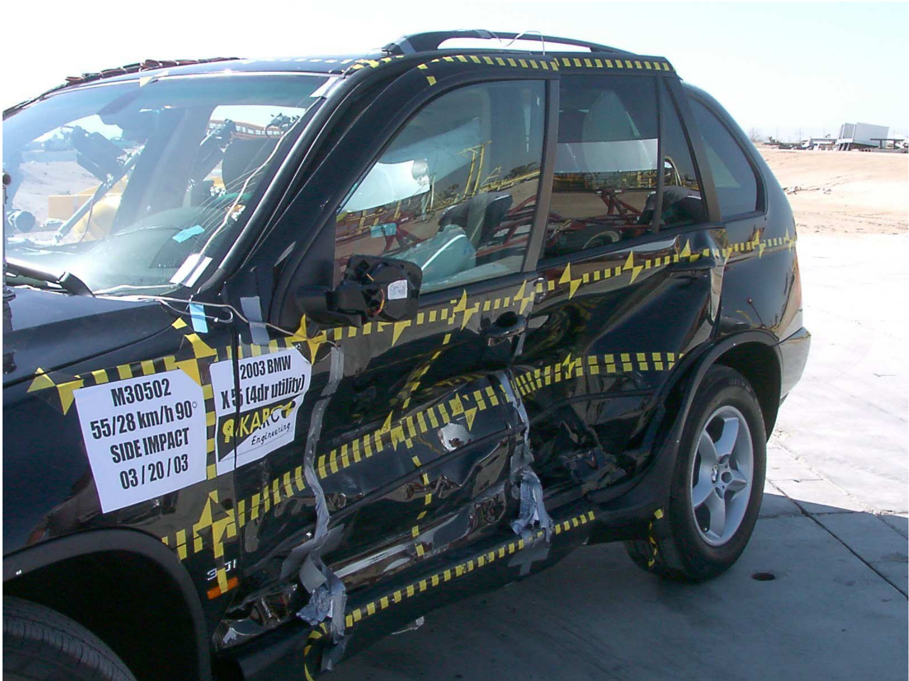
Figure A-22: Front ¾ View of Left Side Doors, Post-Test
