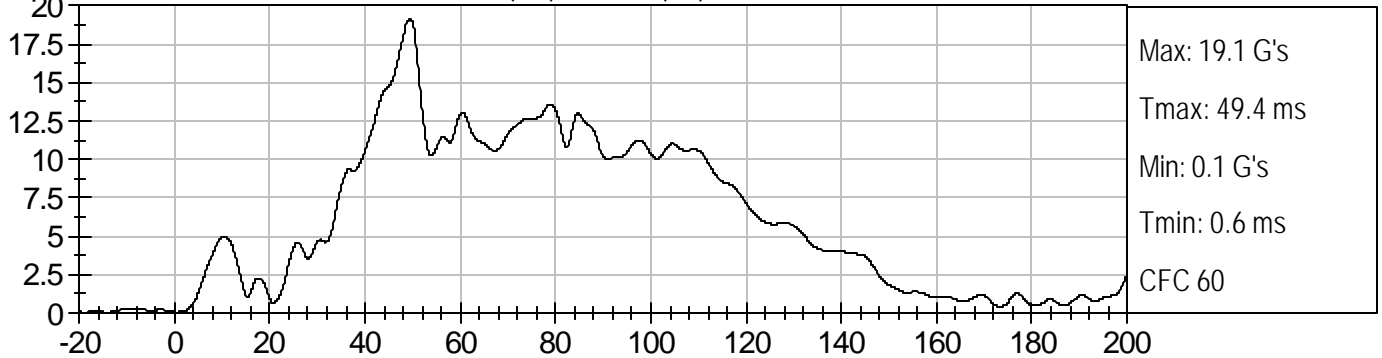
FLOORPAN @ REAR AXLE Resultant (G's) vs TIME (ms)
