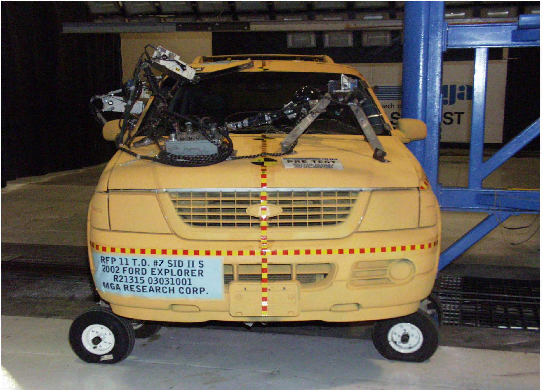
Pre-Test Vehicle Positioned Against Pole (left side)
