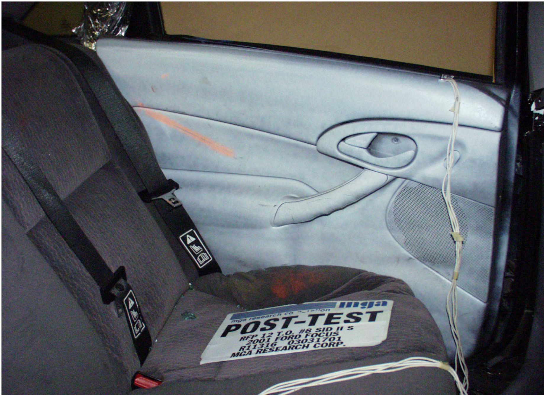
Post-Test Passenger Dummy Lower Body Contact
