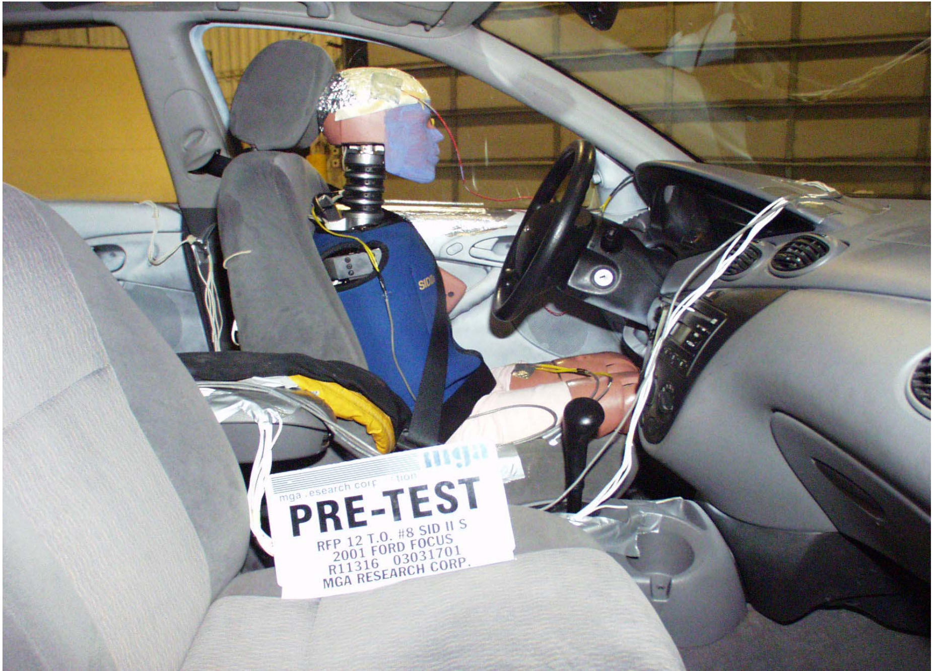
Pre-Test Driver Dummy Right Side View
