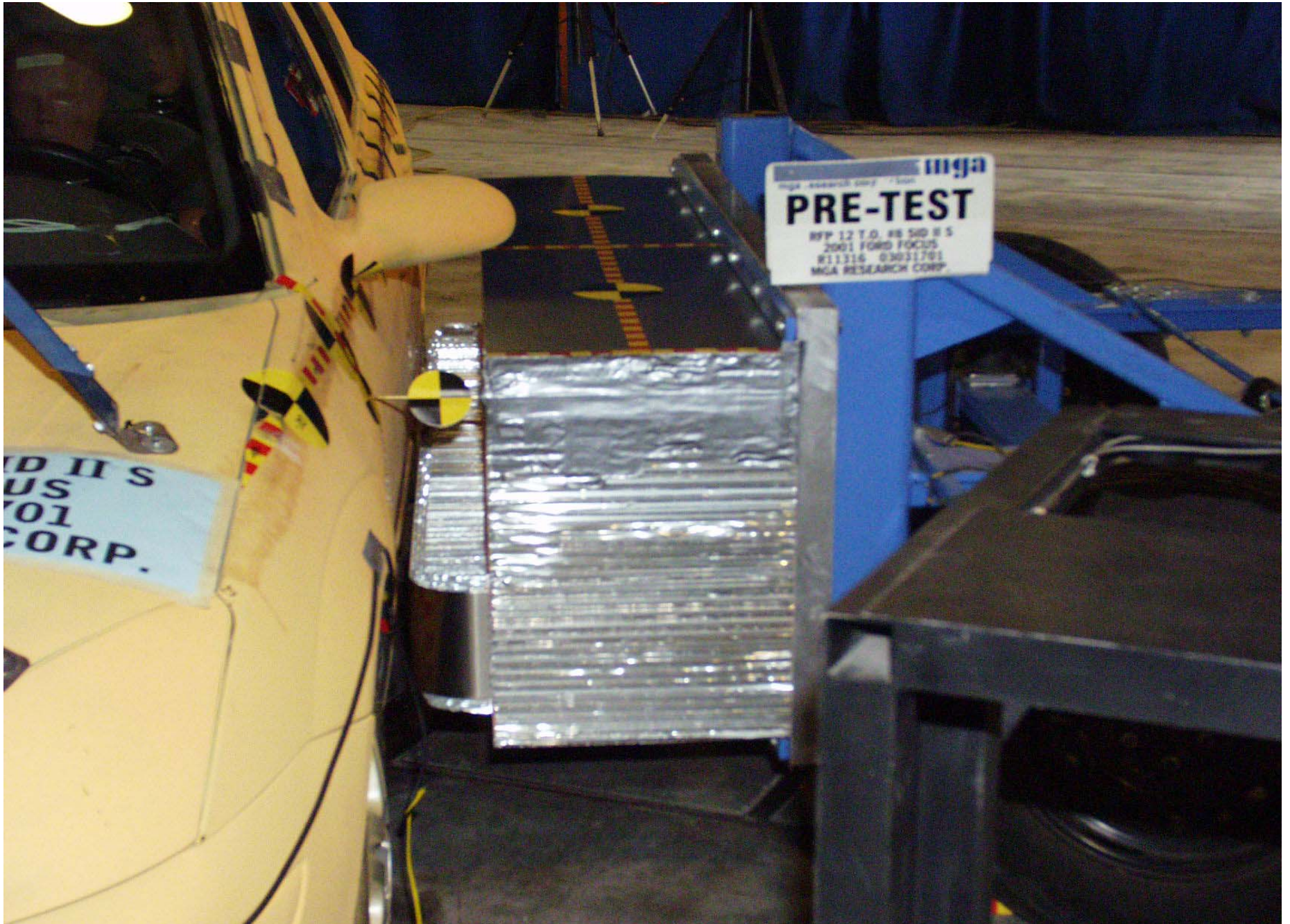
Pre-Test MDB Positioned Against Vehicle (left side)
