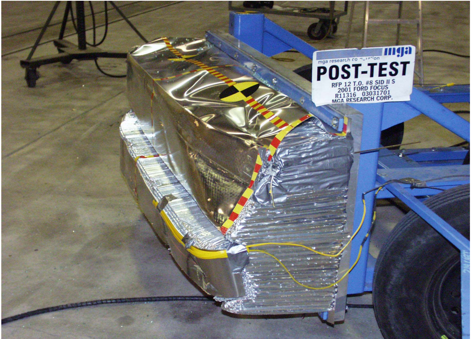
Post-Test MDB Left Side View
