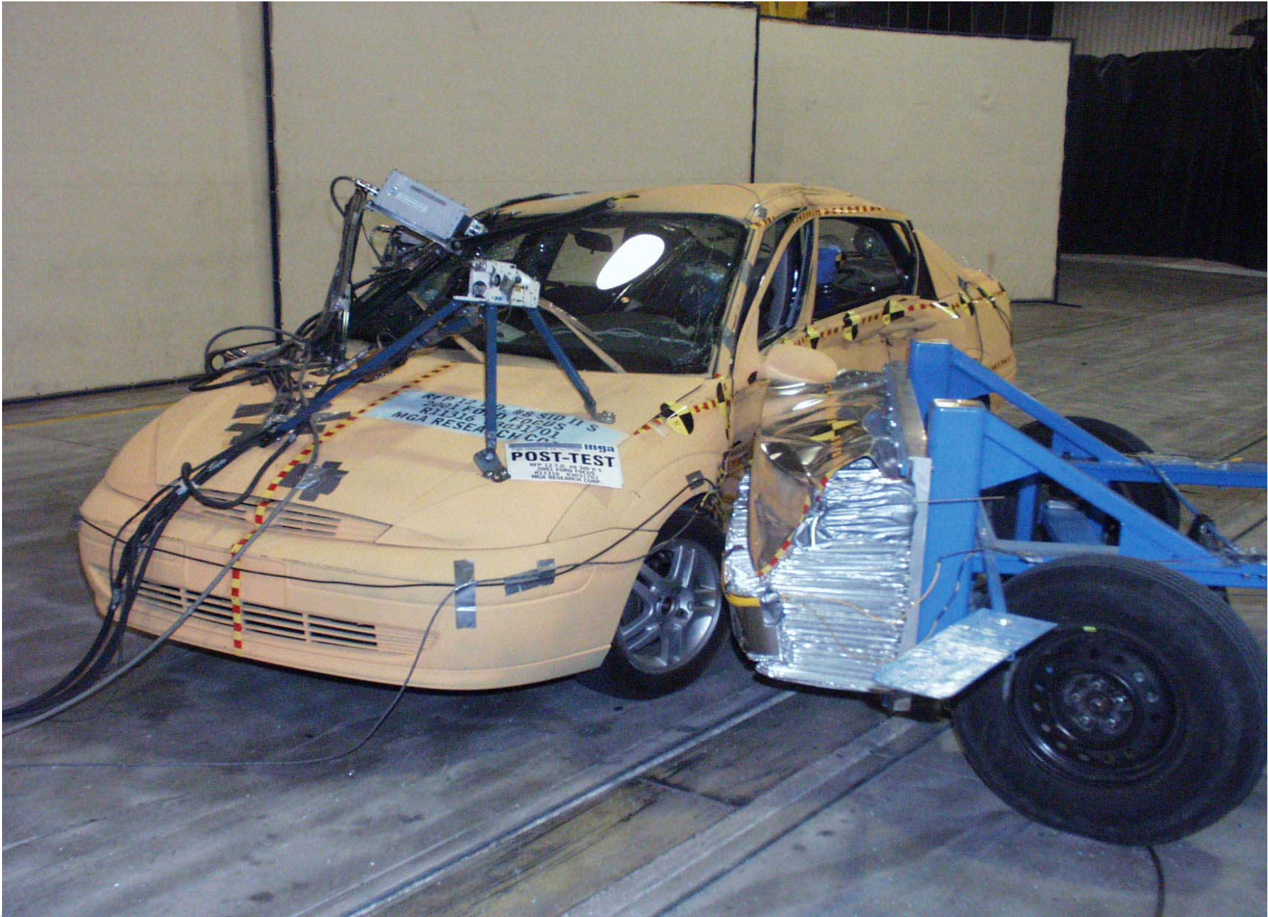
Post-Test MDB and Vehicle (left side)
