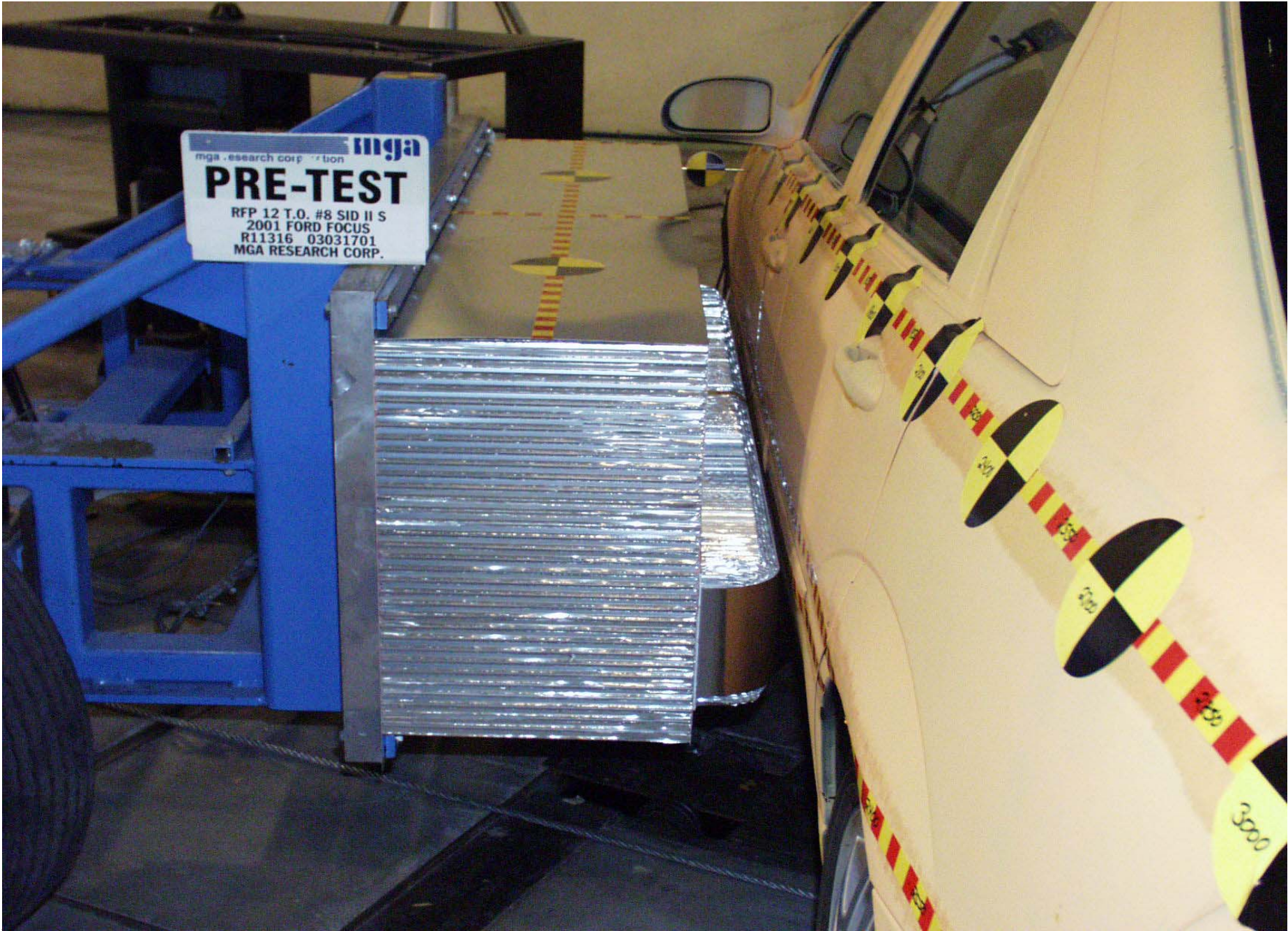
Pre-Test MDB Positioned Against Vehicle (right side)
