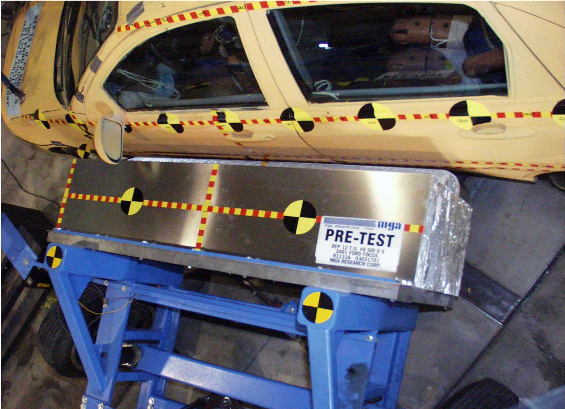
Pre-Test MDB Positioned Against Vehicle (overhead view)
