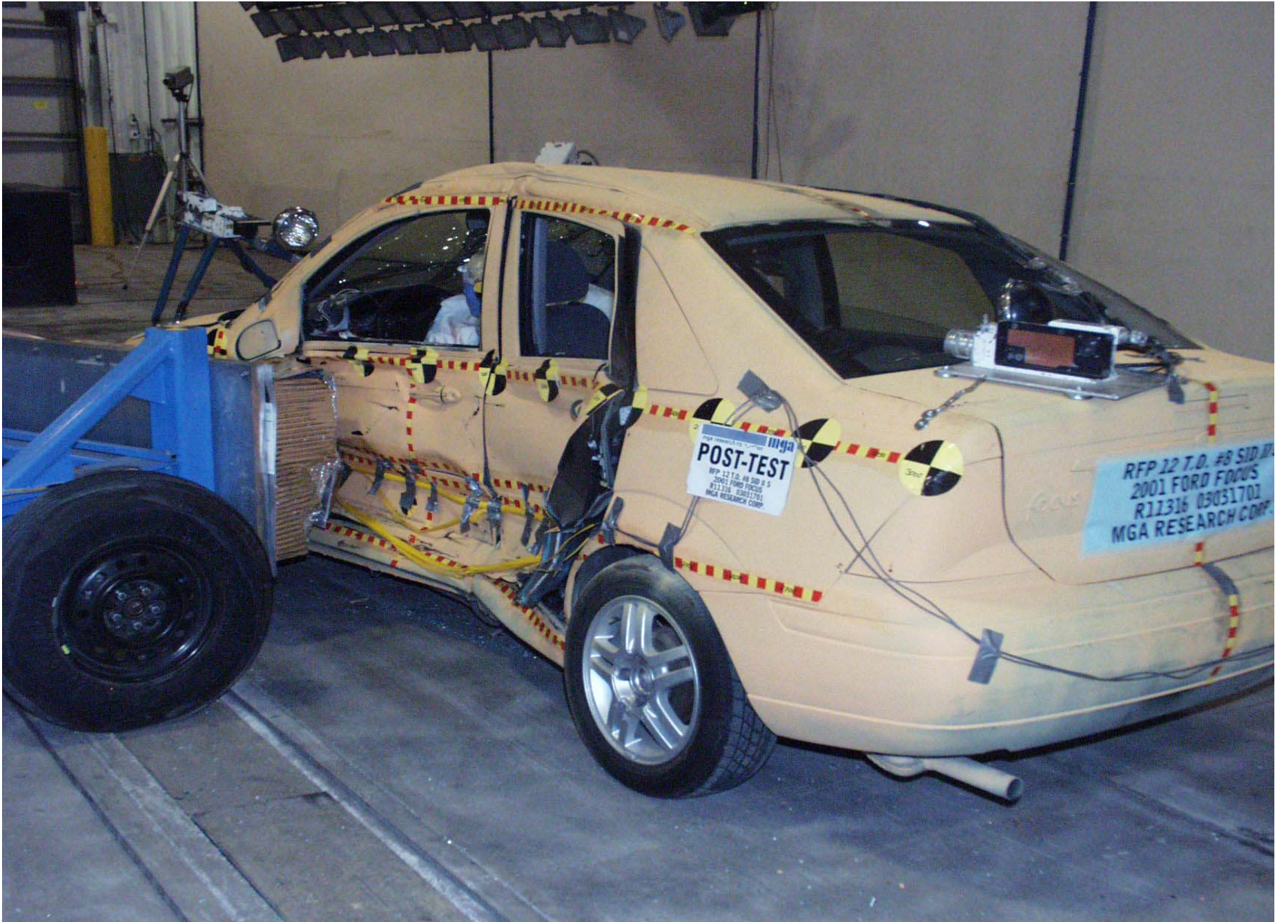
Post-Test MDB and Vehicle (right side)
