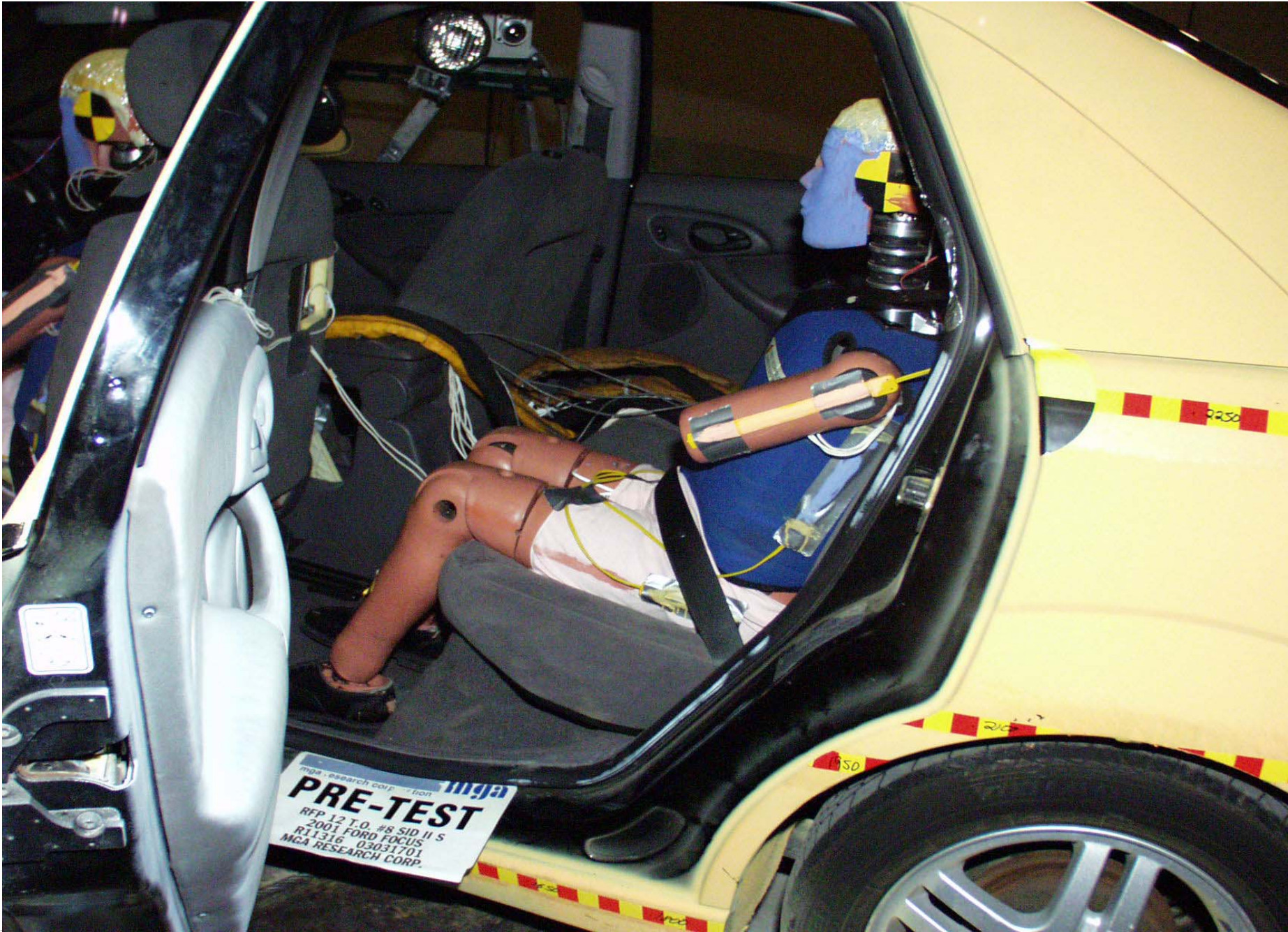
Pre-Test Passenger Dummy Left Side View (Door open)
