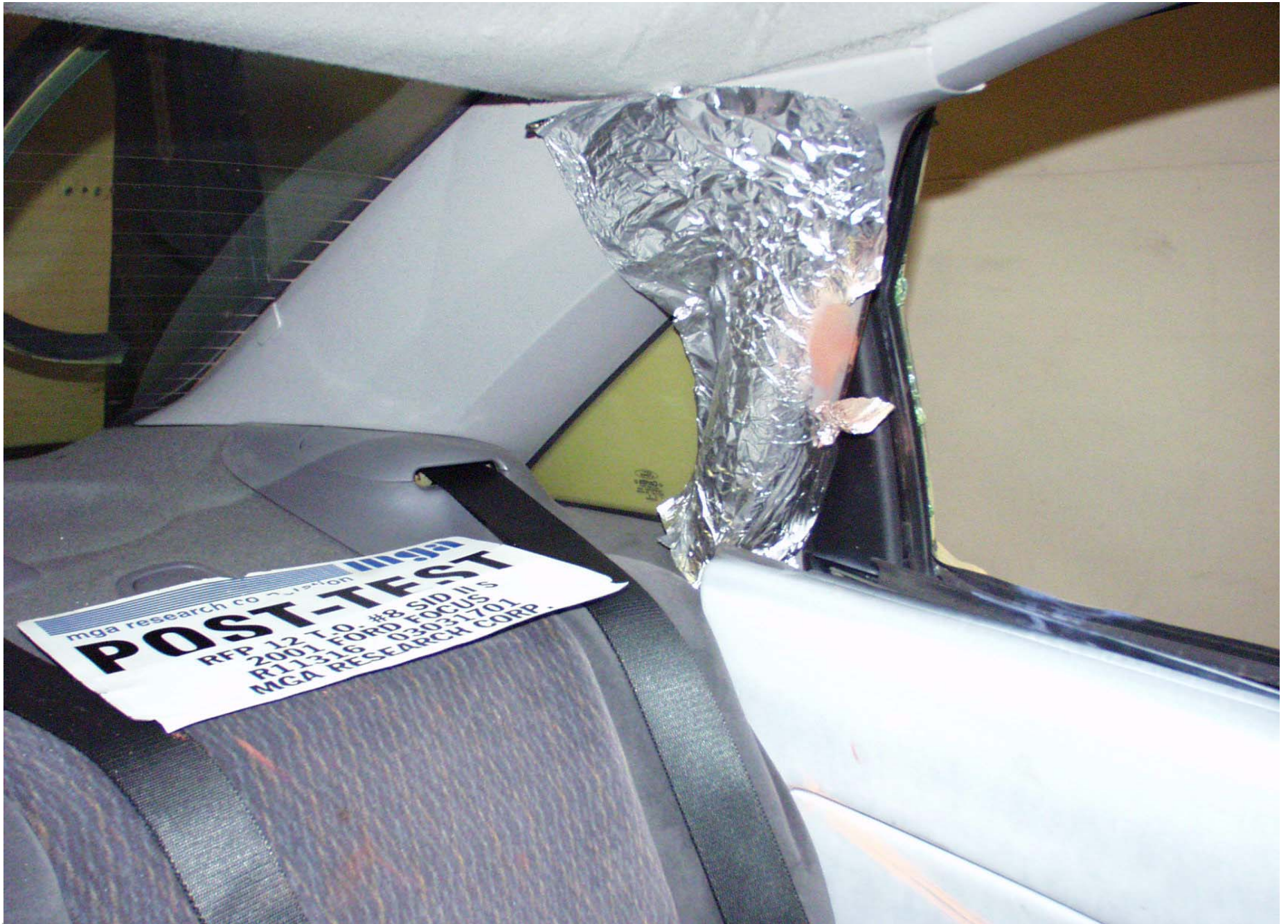
Post-Test Passenger Dummy Head Contact
