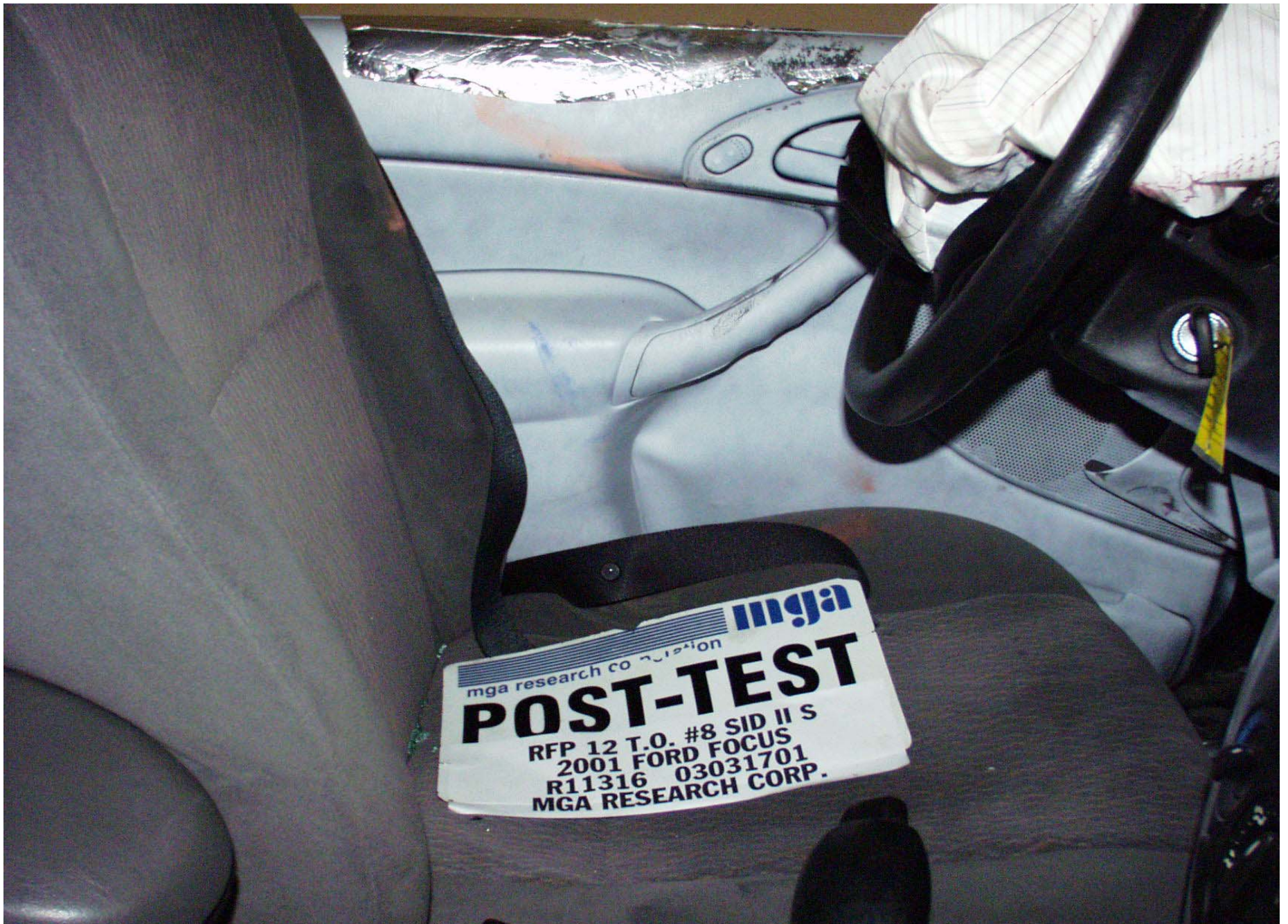
Post-Test Driver Dummy Lower Body Contact
