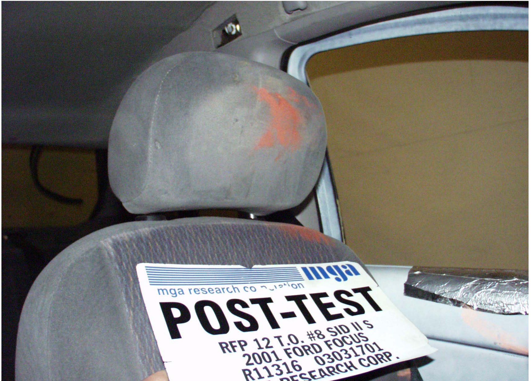
Post-Test Driver Dummy Head Contact
