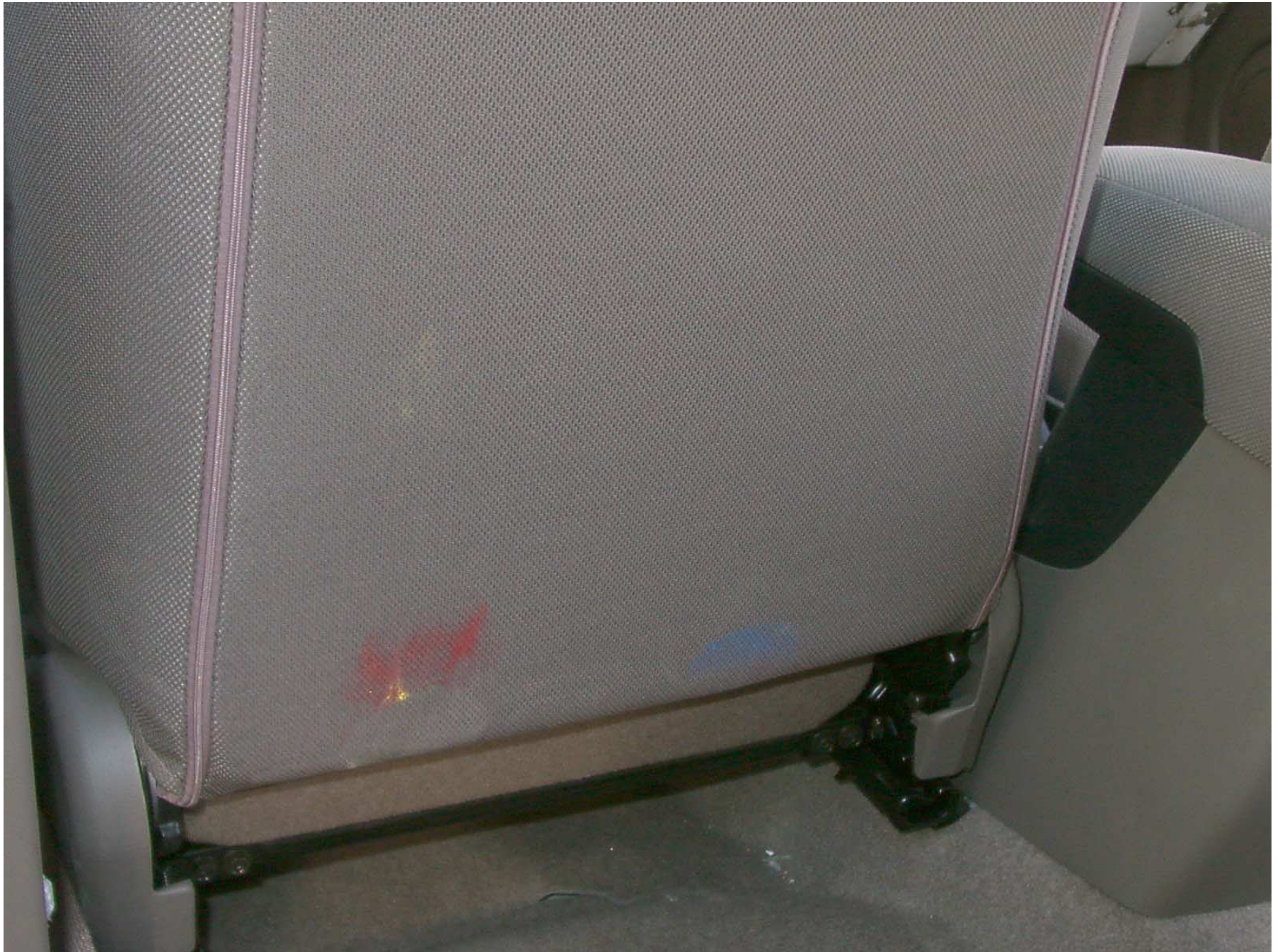
Figure F-32: Post-Test Position 4 Contact Point (Back of Left Front Seat)
