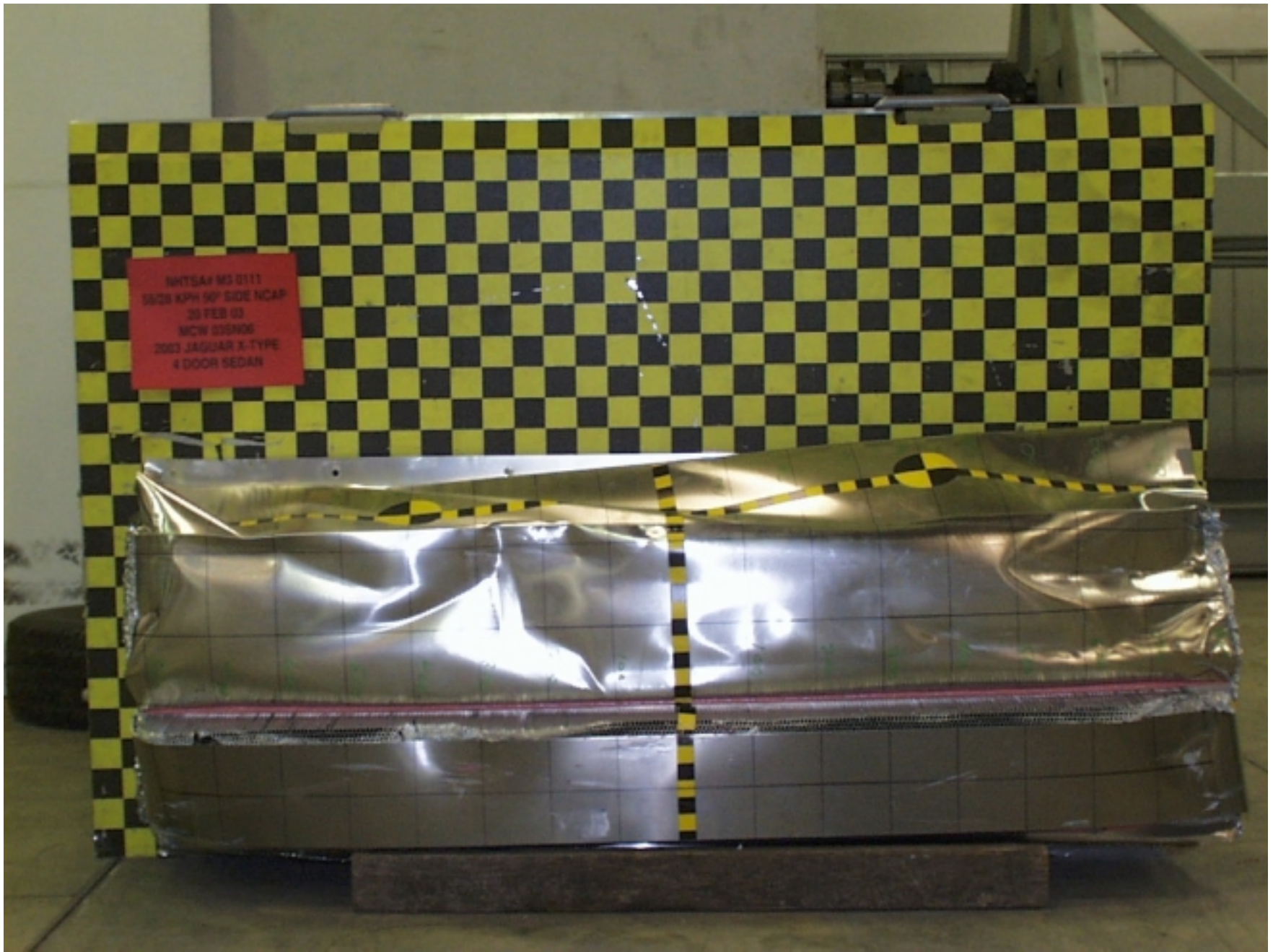
Figure A-50: POST-TEST ALUMINUM BARRIER FRONT
