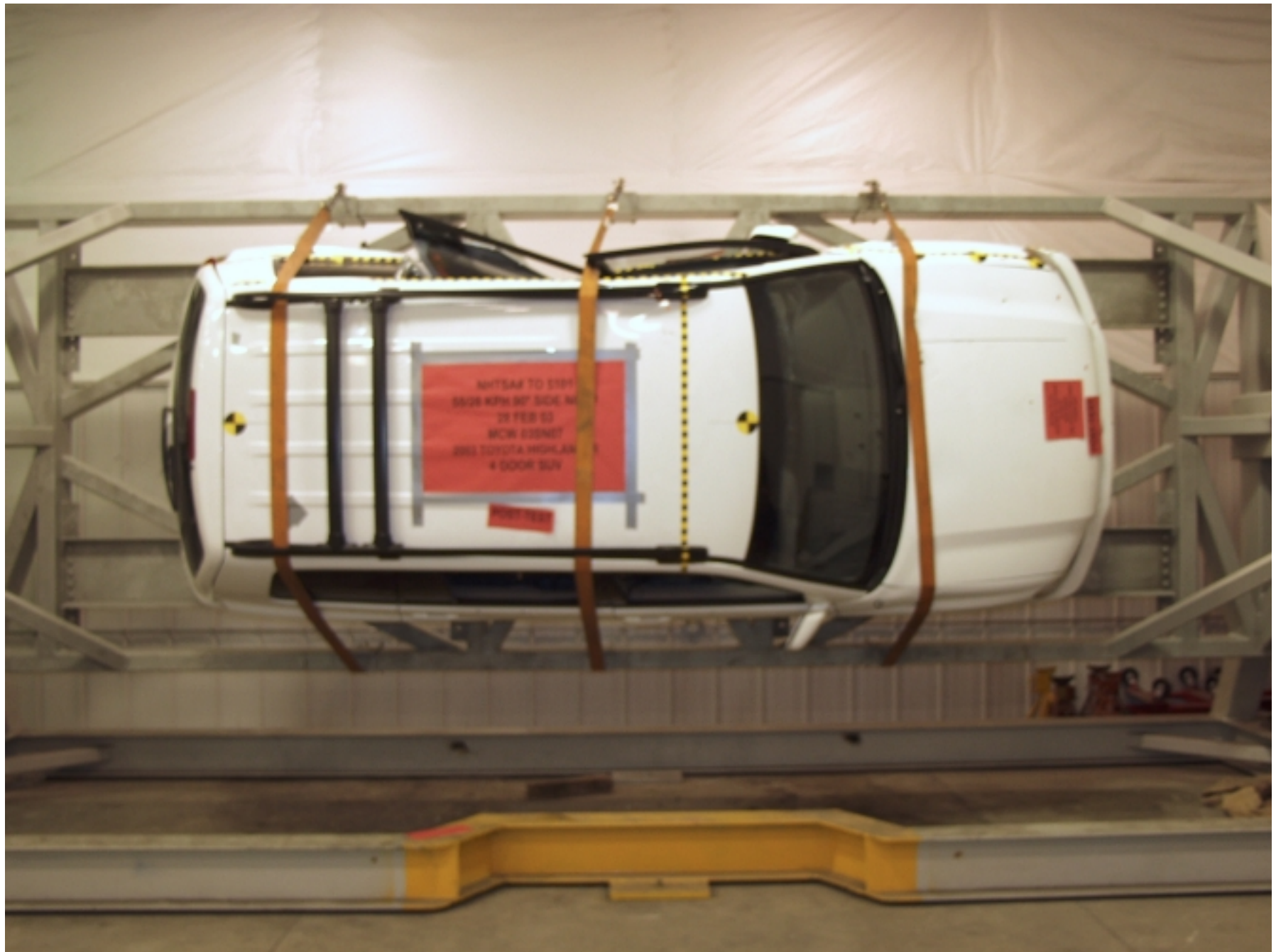
Figure A-47: ROLLOVER 270 DEGREES
