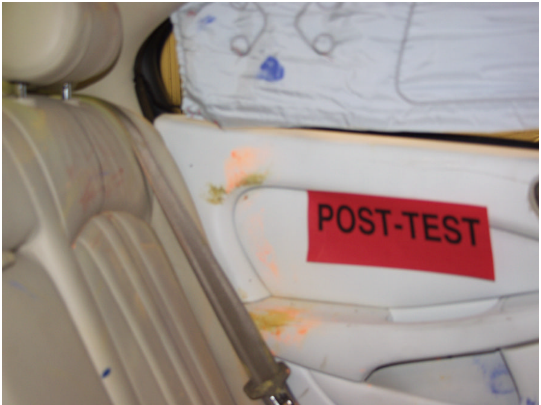
Figure A-28: POST-TEST INTERIOR OF REAR DOOR SHOWING SID H3 IMPACT LOCATIONS
