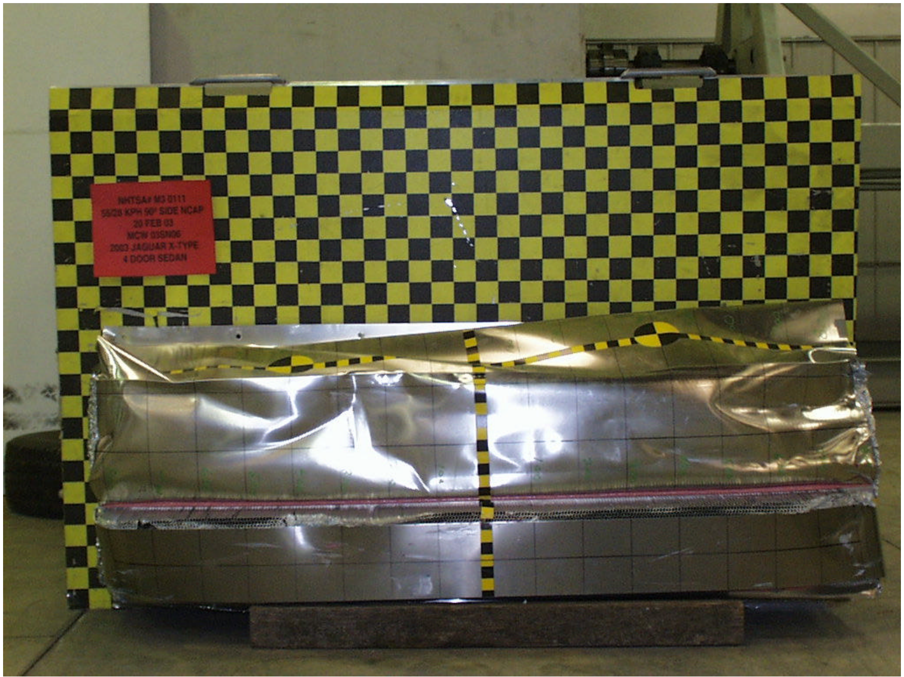
Figure A-46: POST-TEST ALUMINUM BARRIER FRONT
