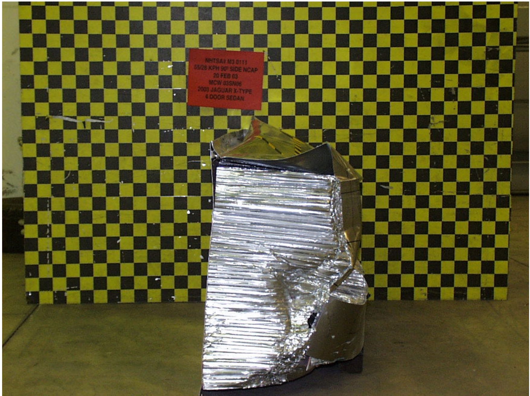
Figure A-50: POST-TEST ALUMINUM BARRIER RIGHT SIDE
