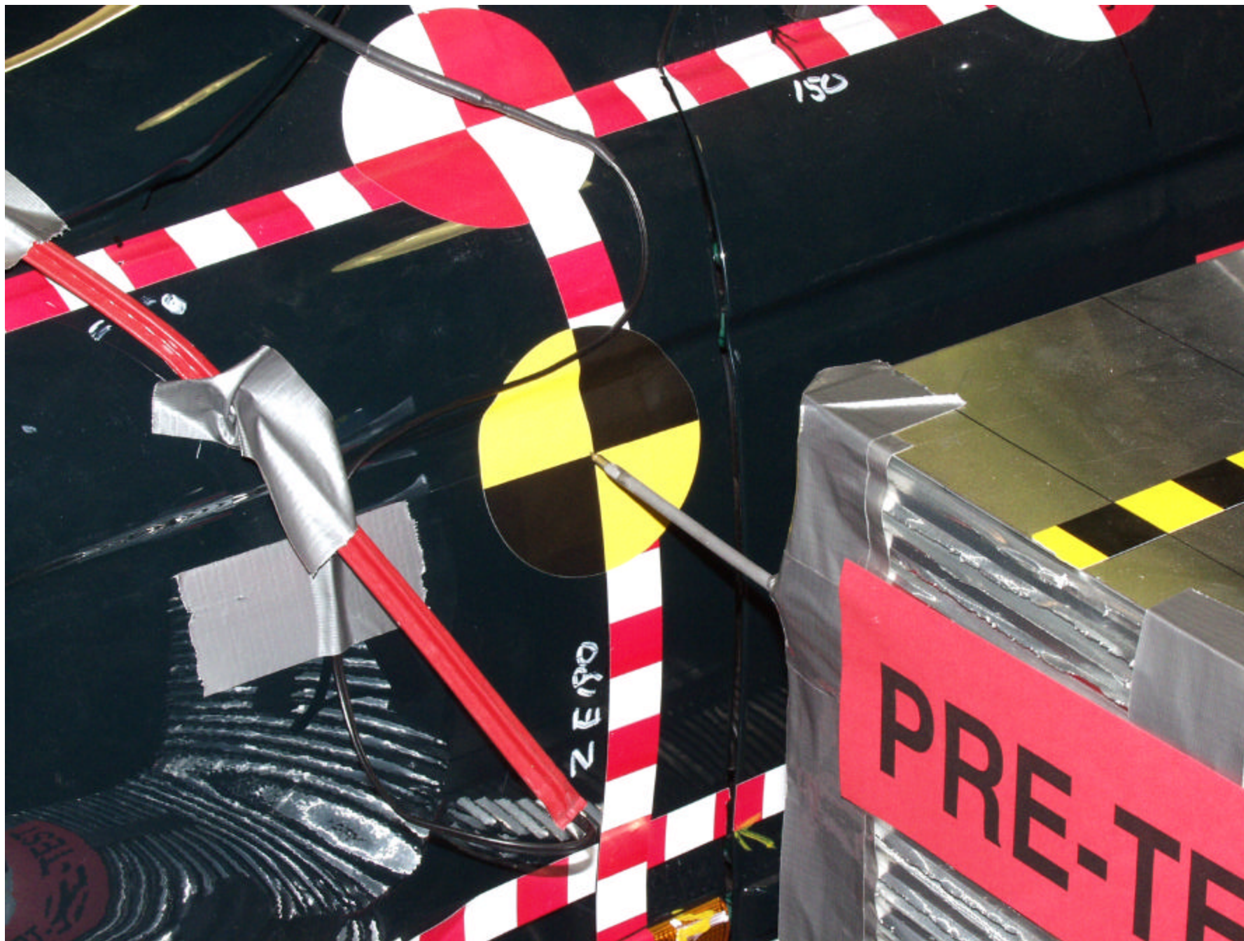
Figure A-35: PRE-TEST CLOSE-UP OF IMPACT POINT TARGET SHOWING WELDING ROD
