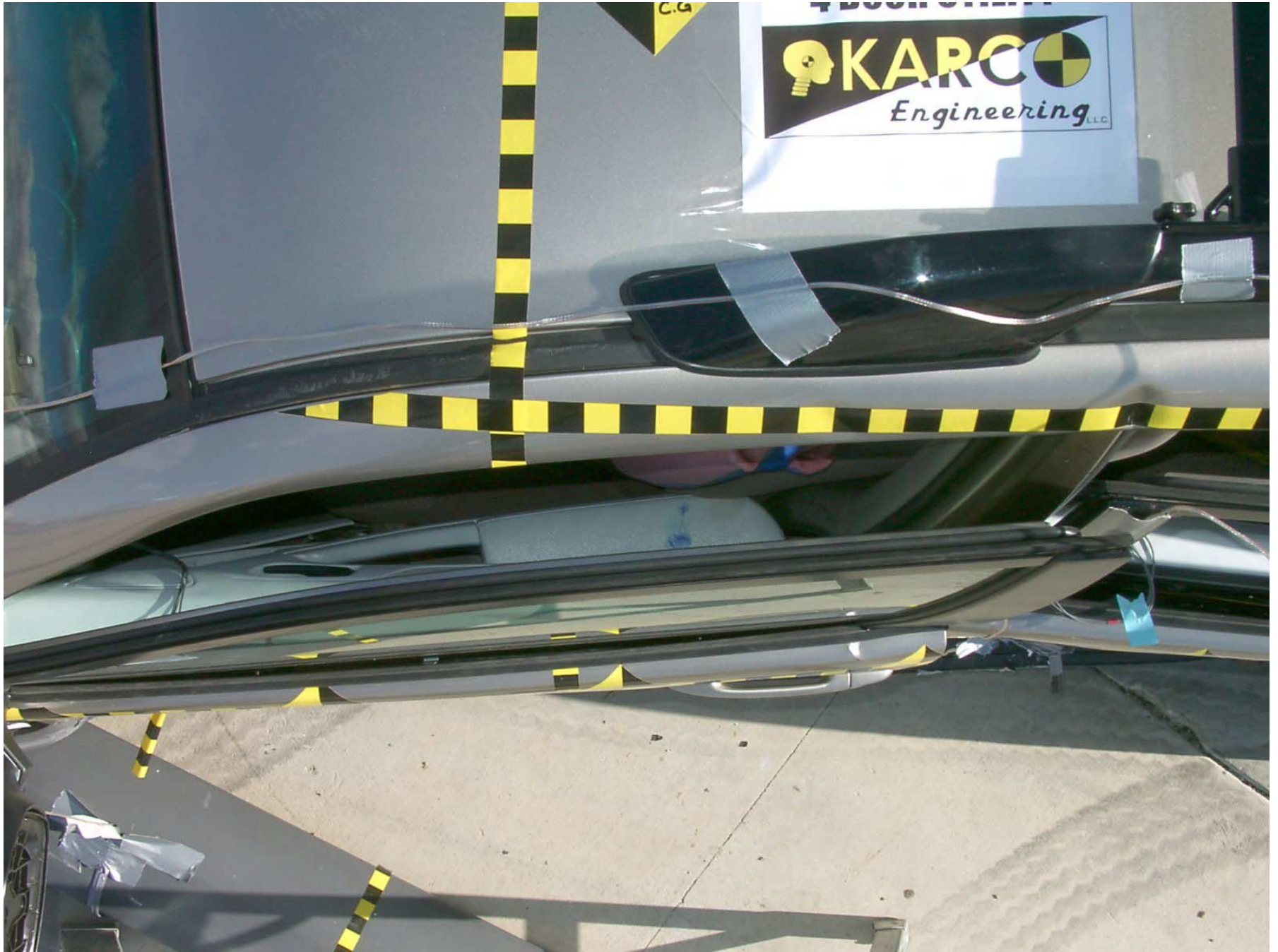
Figure A-29: Driver Dummy Clearance, Post-Test (Driver Door Unlatched Prior to Photo)
