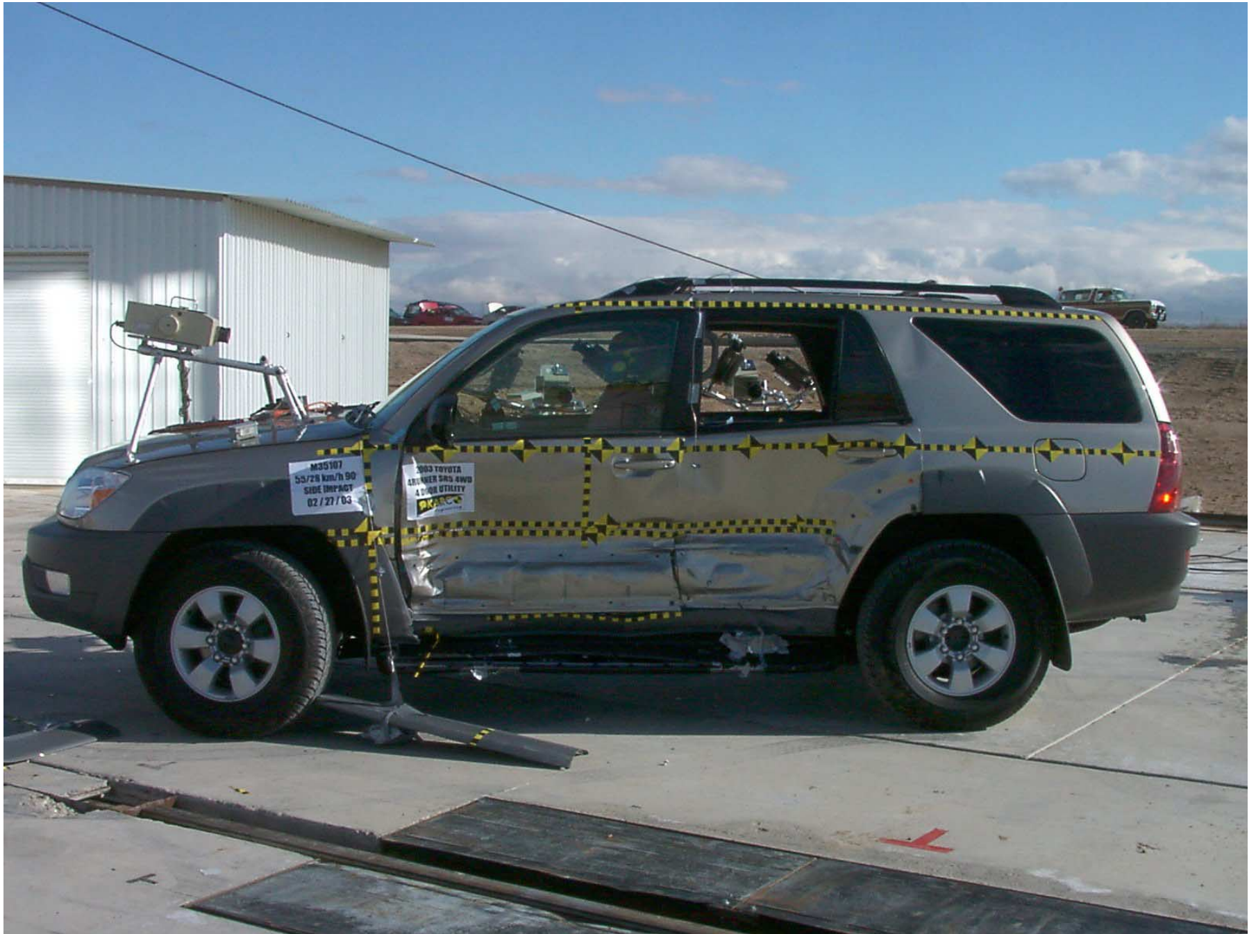
Figure A-10: Left (Impacted) Side View, Post-Test (Driver Door Unlatched Prior to Photo)
