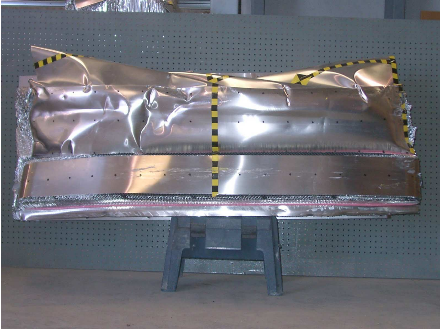
Figure A-44: Front View of Deformable Barrier, Post-Test
