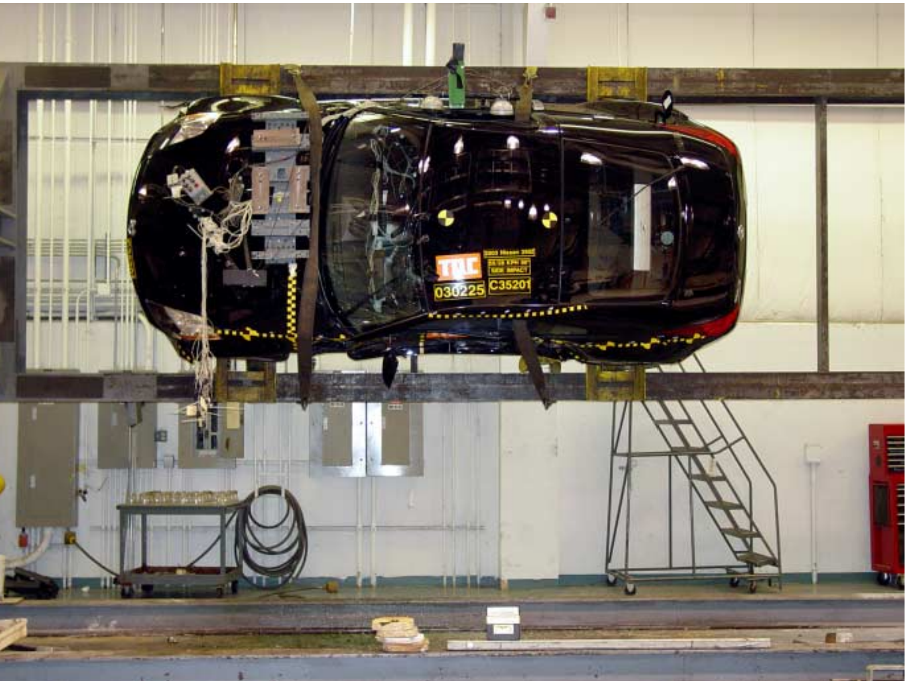
Figure A-41 FMVSS 301 Rollover View at 270°
