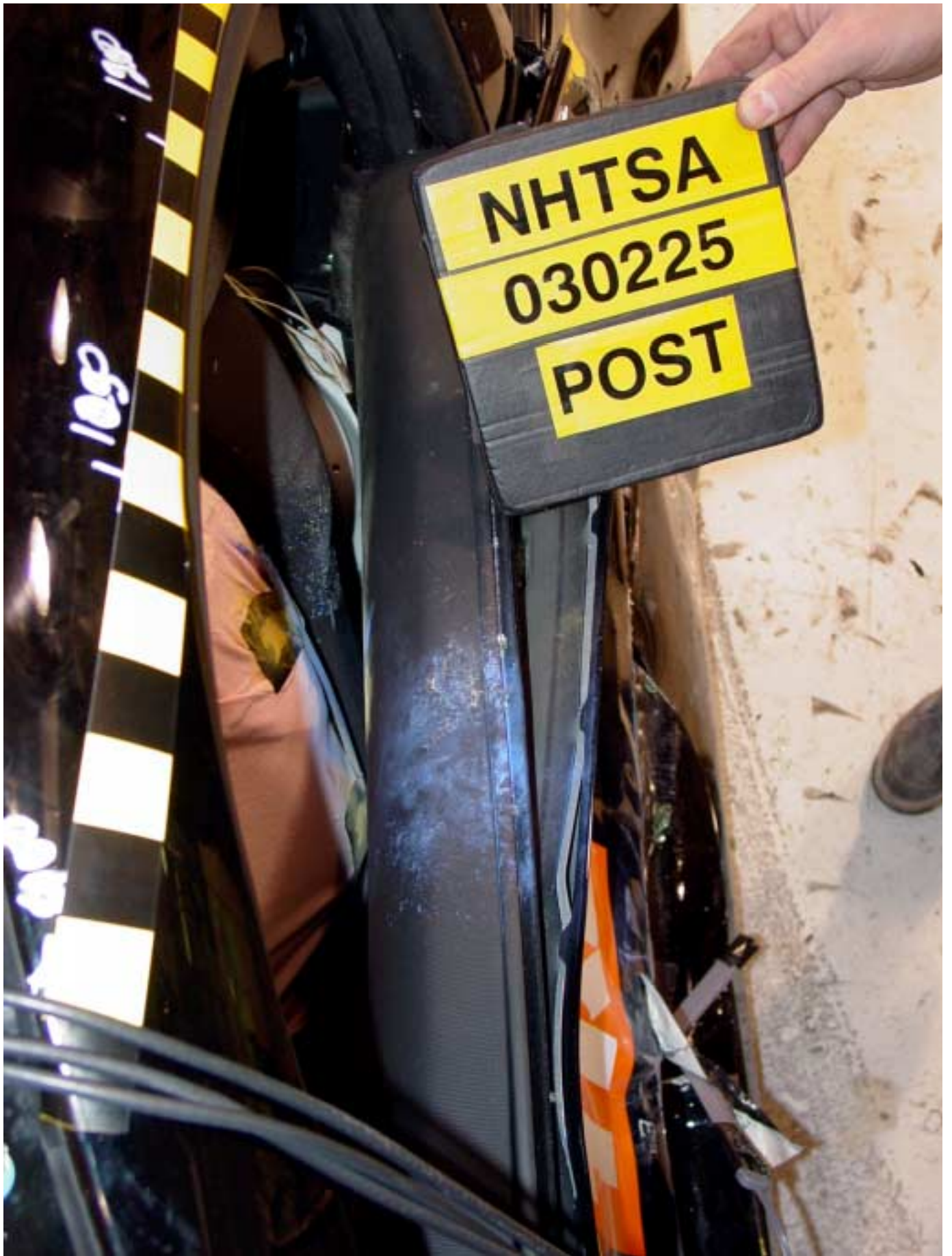
Figure A-27 Post-Test Front SID Contact - View 1
