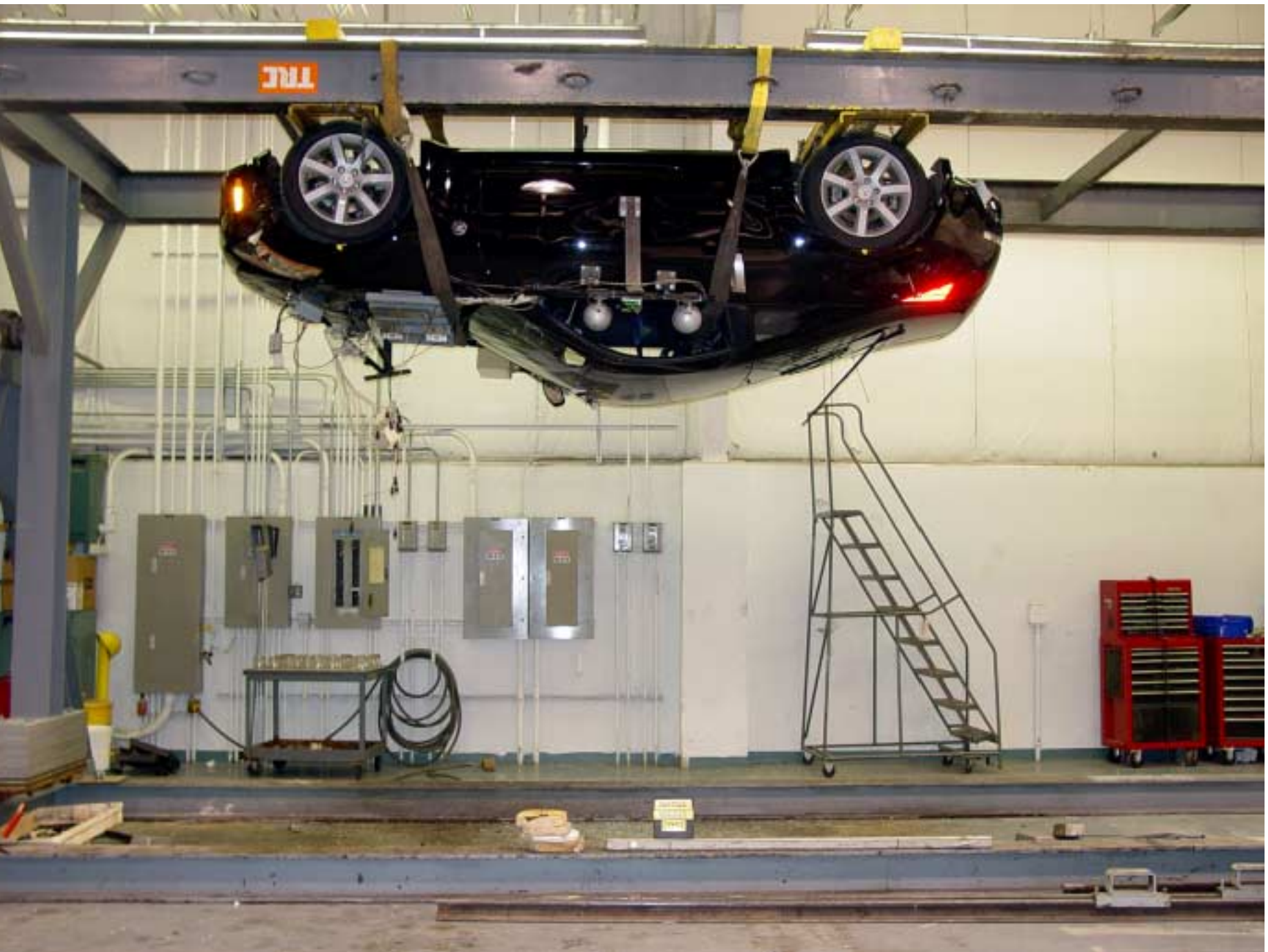
Figure A-40 FMVSS 301 Rollover View at 180°
