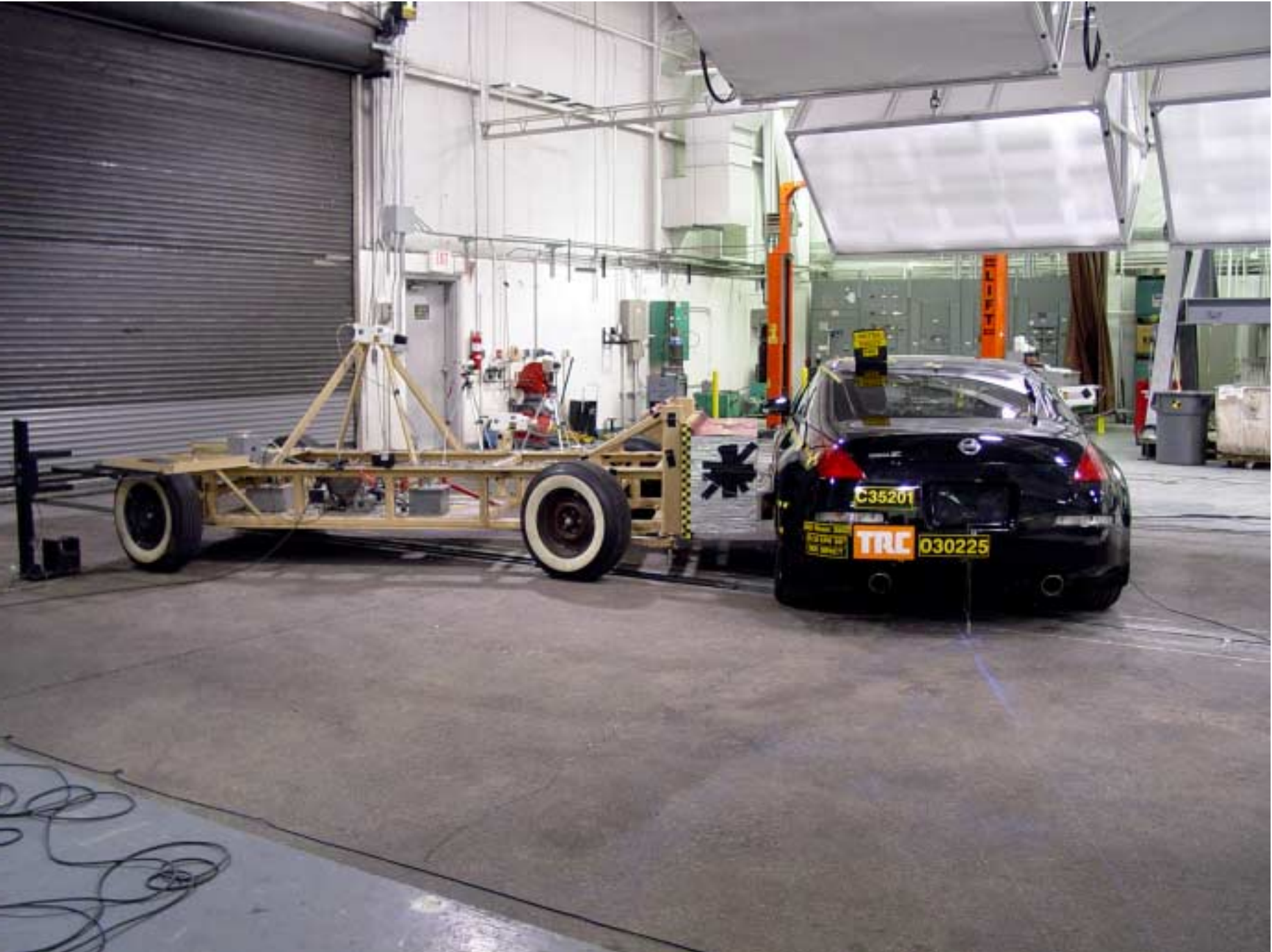
Figure A-32 Pre-Test Right Side View of MDB With Impactor Face in Position
