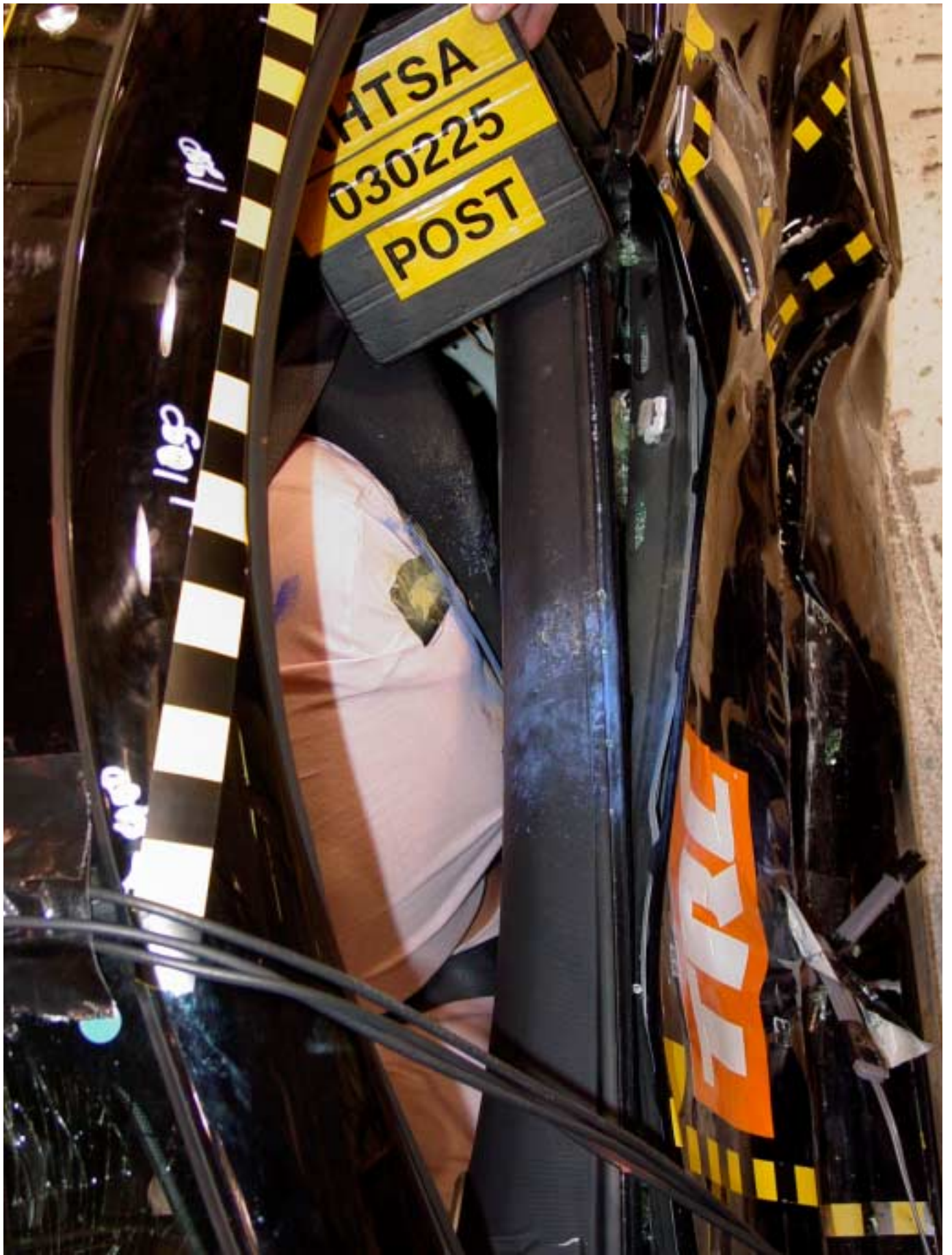
Figure A-24 Post-Test Left View of Front SID and Door Clearance
