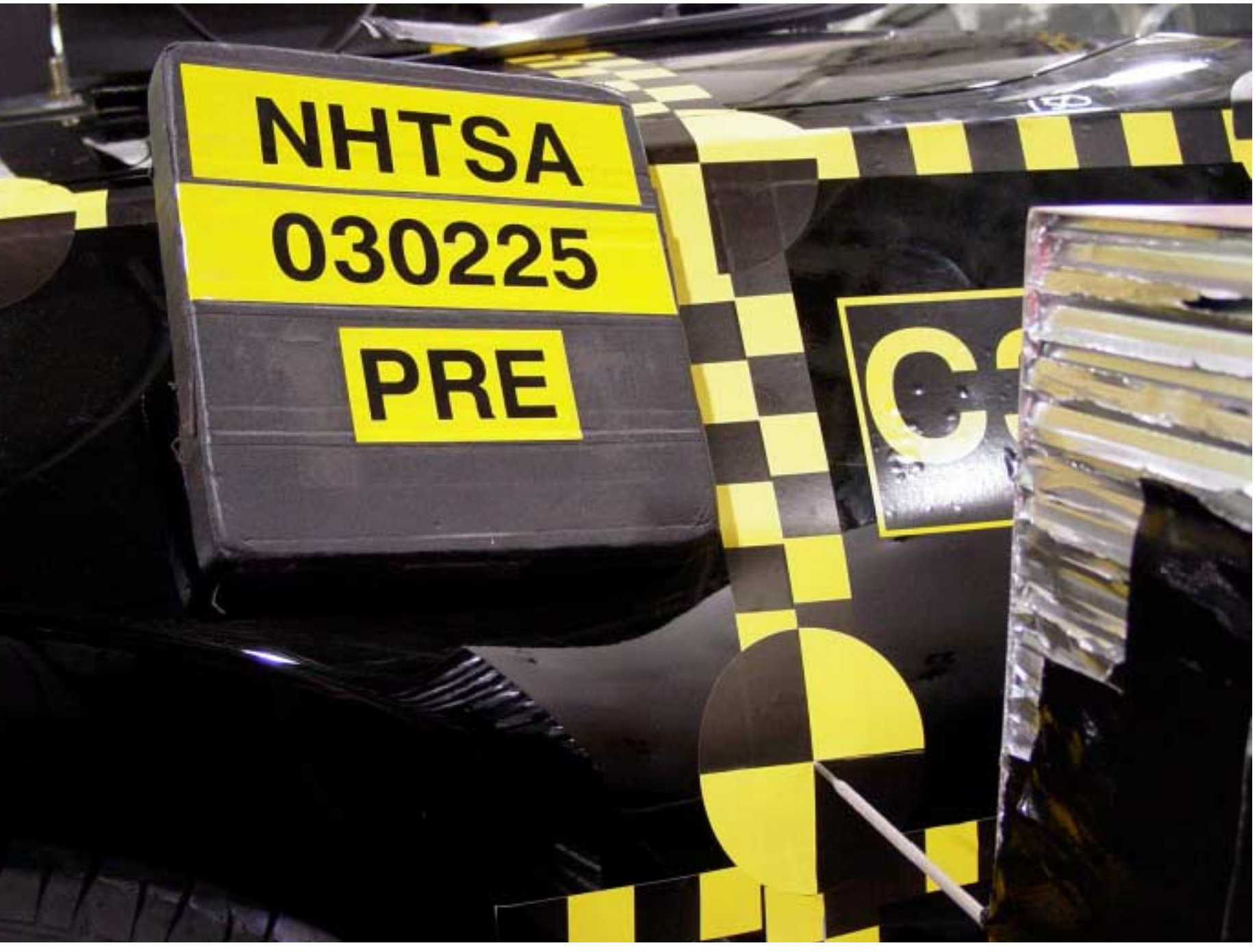
Figure A-30 Pre-Test Primary Impact Point View
