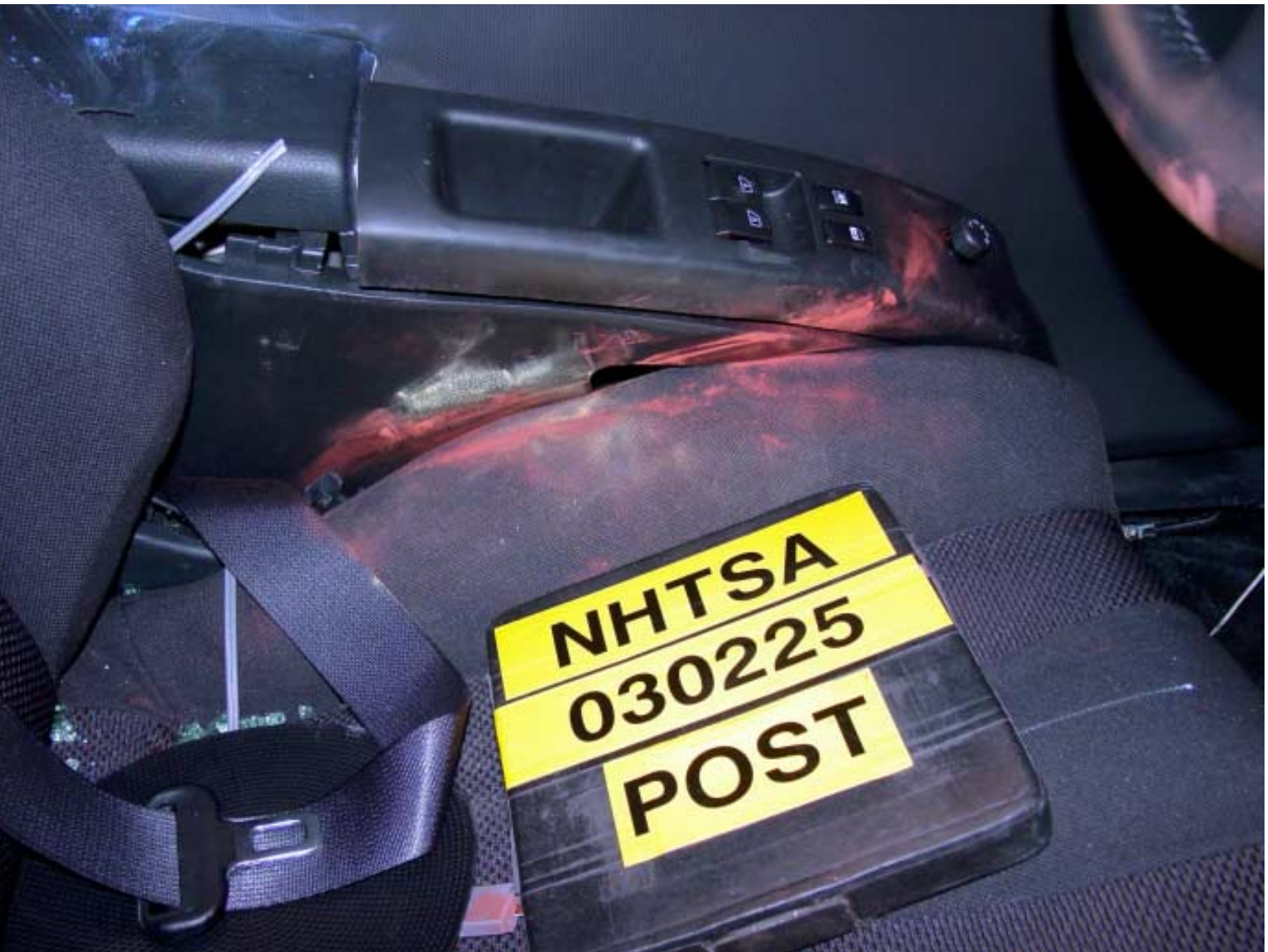
Figure A-28 Post-Test Front SID Contact - View 2
