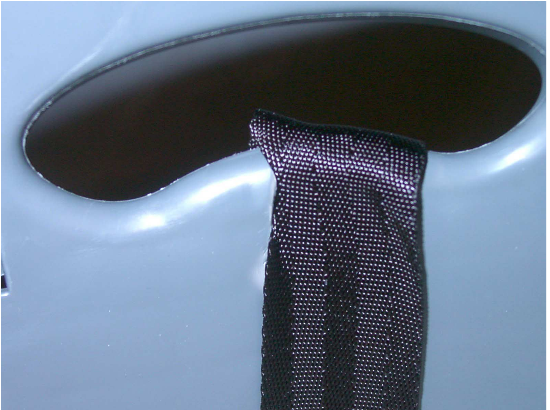
Figure F2-34: Post-Test Damage to Position 3 CRS (Front View of Tether Strap)
