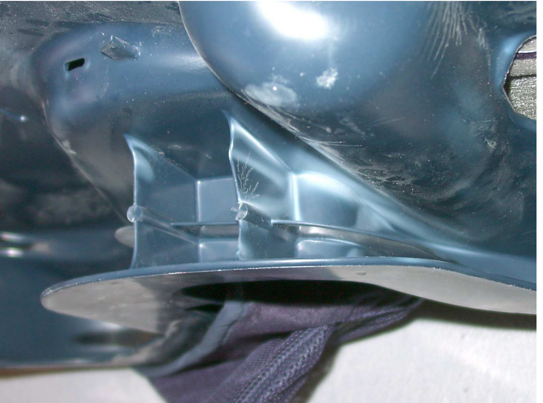
Figure F2-35: Post-Test Damage to Position 3 CRS (Left Side)
