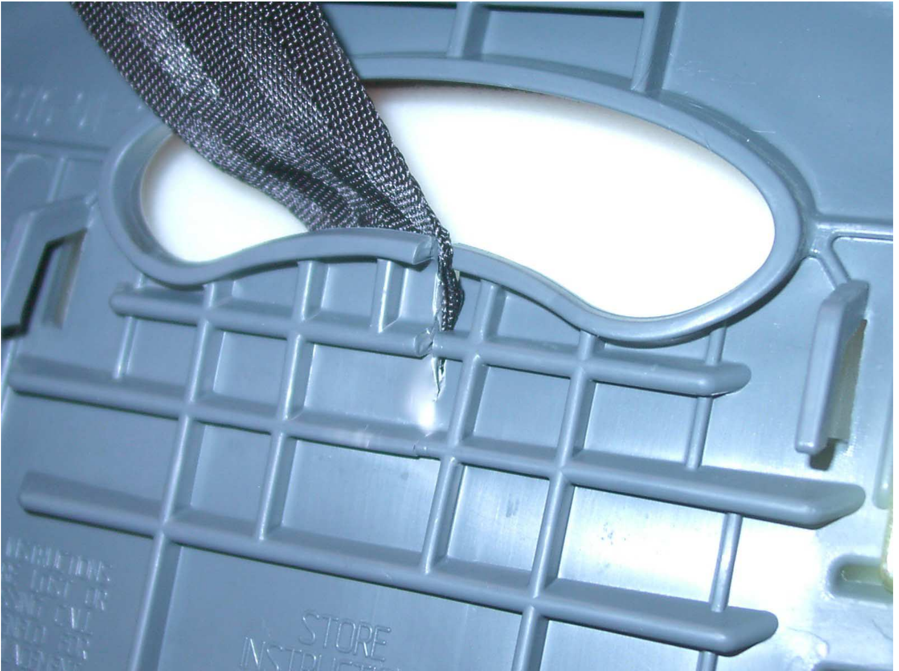
Figure F2-33: Post-Test Damage to Position 3 CRS (Rear View of Tether Strap)
