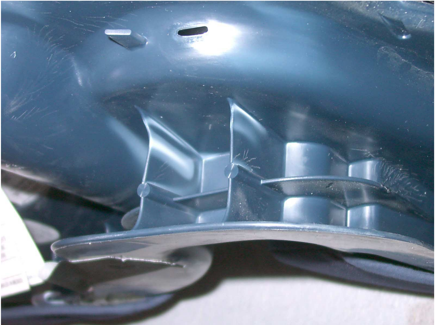
Figure F2-36: Post-Test Damage to Position 3 CRS (Right Side)
