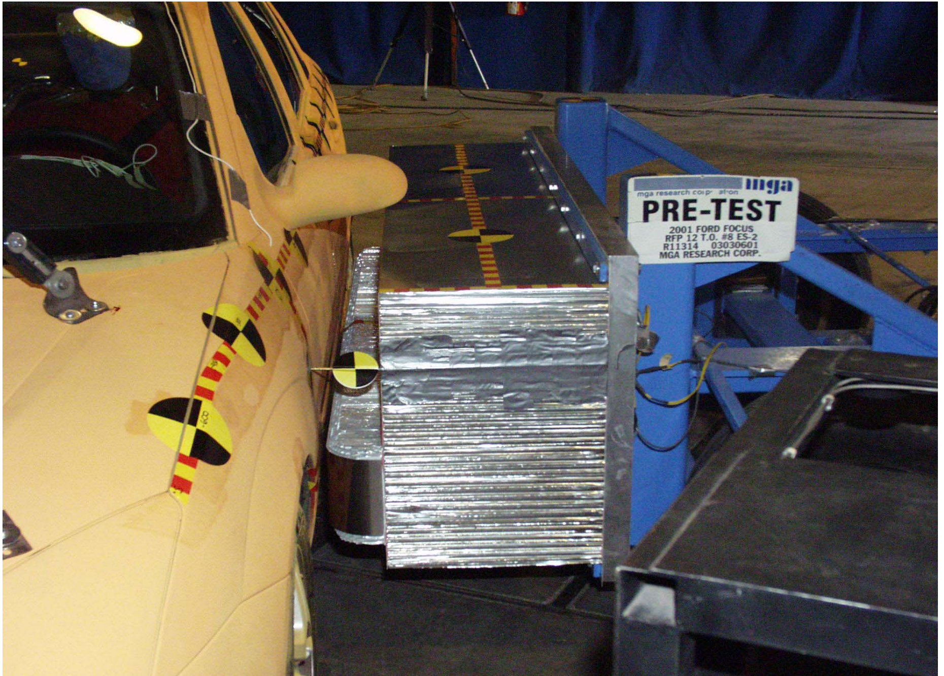
Pre-Test MDB Positioned Against Vehicle (left side)
