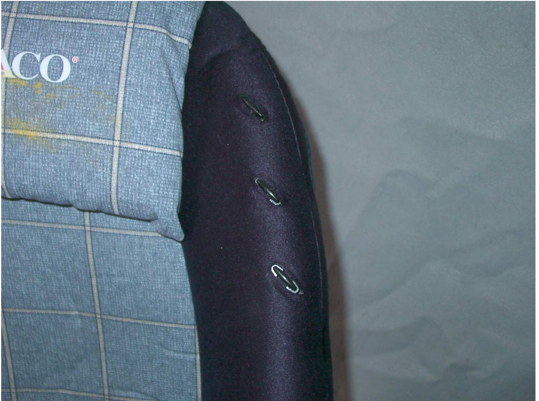
Figure F-33: Post-Test Position 4 Child Seat Damage
