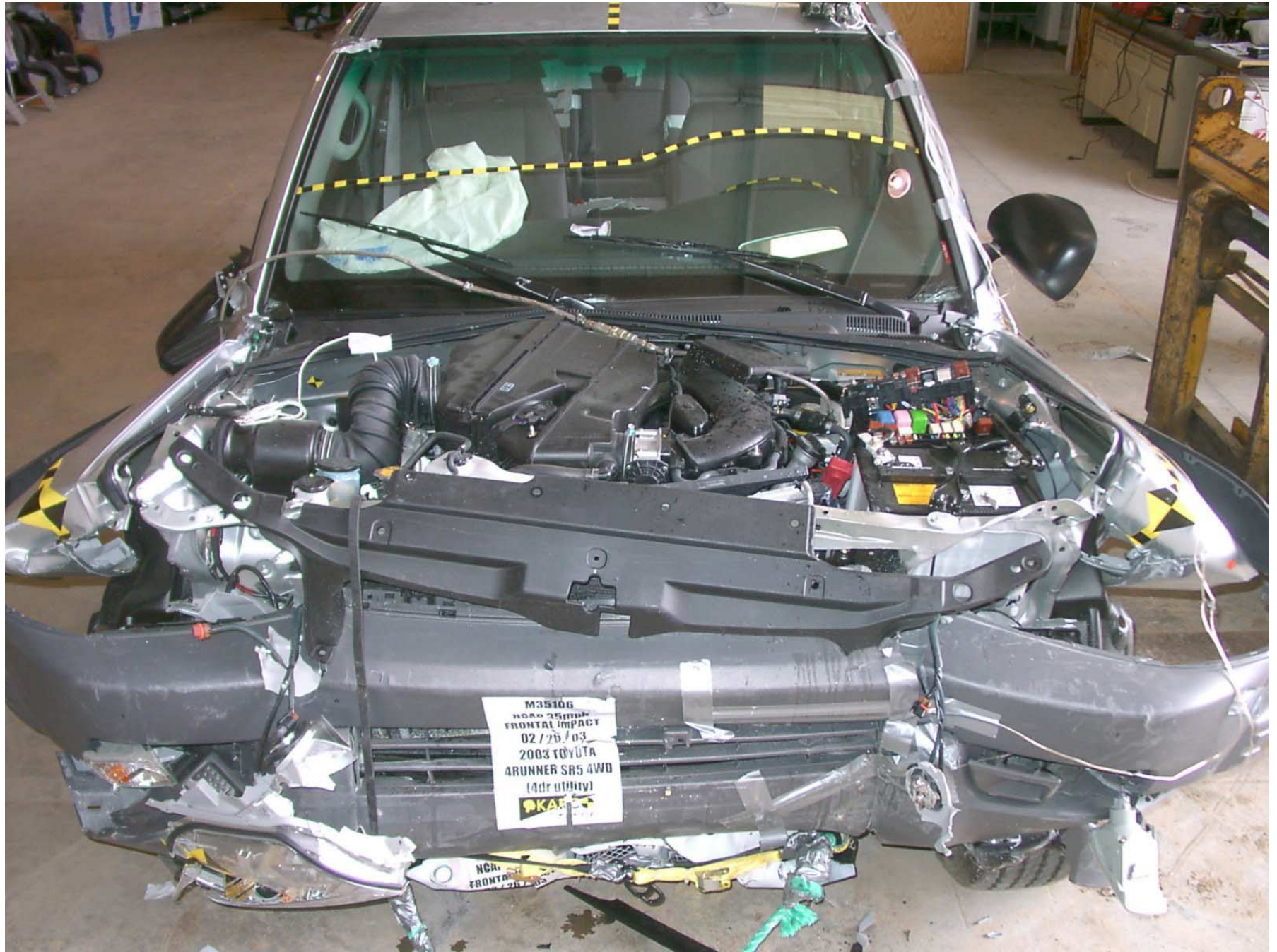
Figure A-21: Post-Test Engine Compartment
