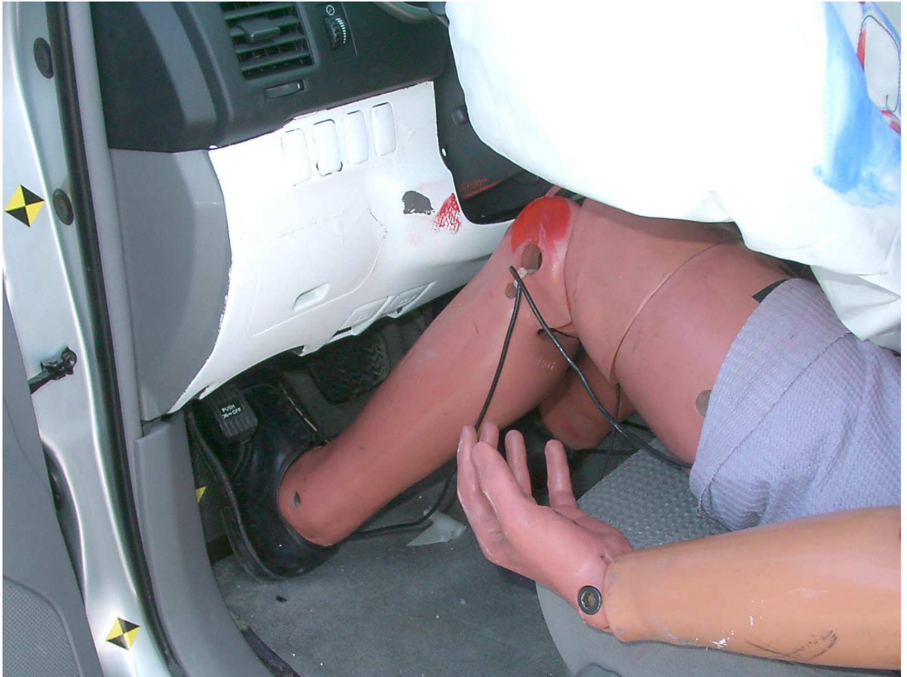
Figure A-37: Post-Test Driver Dummy Feet
