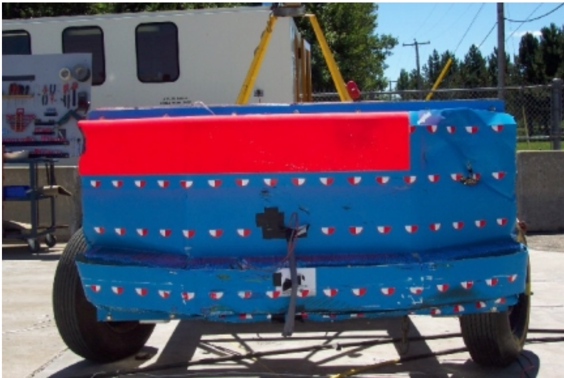
Front view of the deformable face, pre-test.
