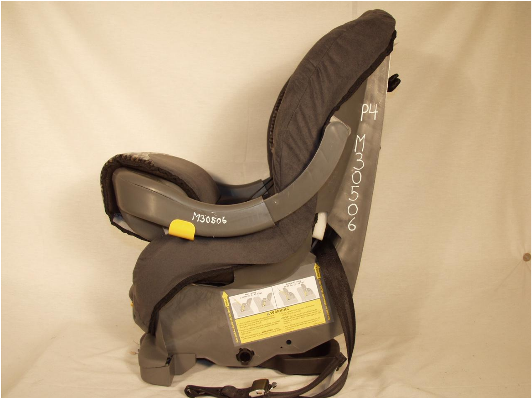
Figure 3-15: PRE-TEST LEFT SIDE VIEW OF POSITION 4 CRS
