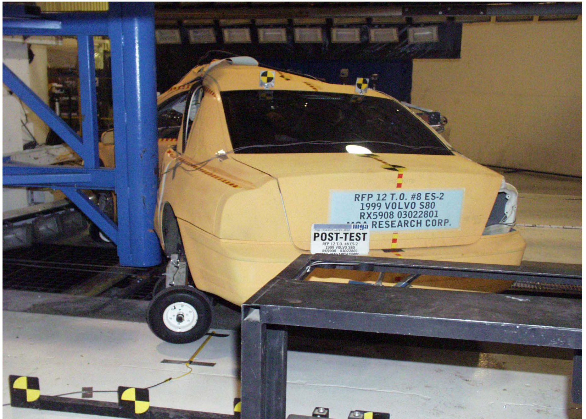
Post-Test Vehicle Positioned Against Pole (right side)
