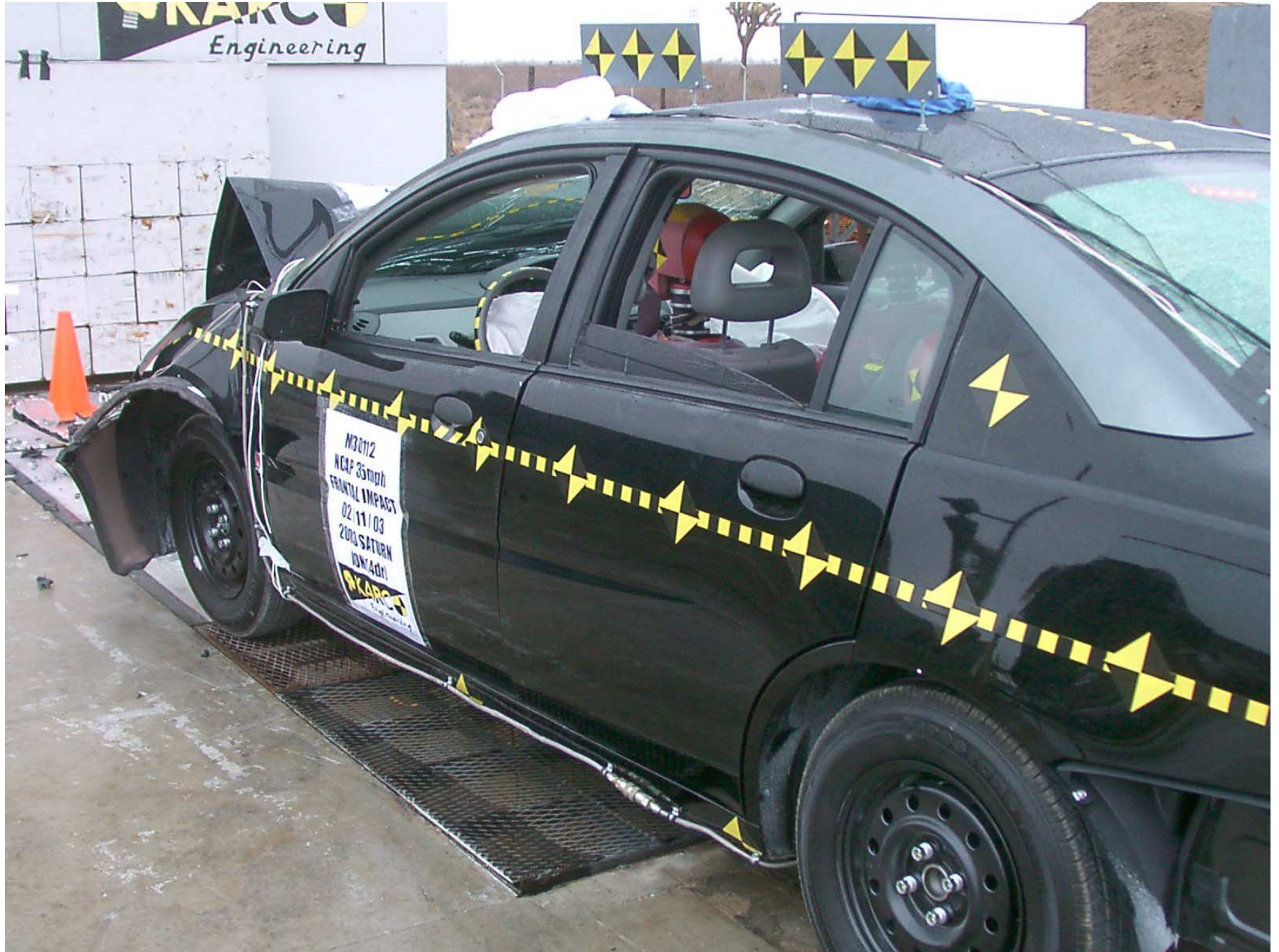
Figure A-16: Left Rear ¾ View of Doors After Impact
