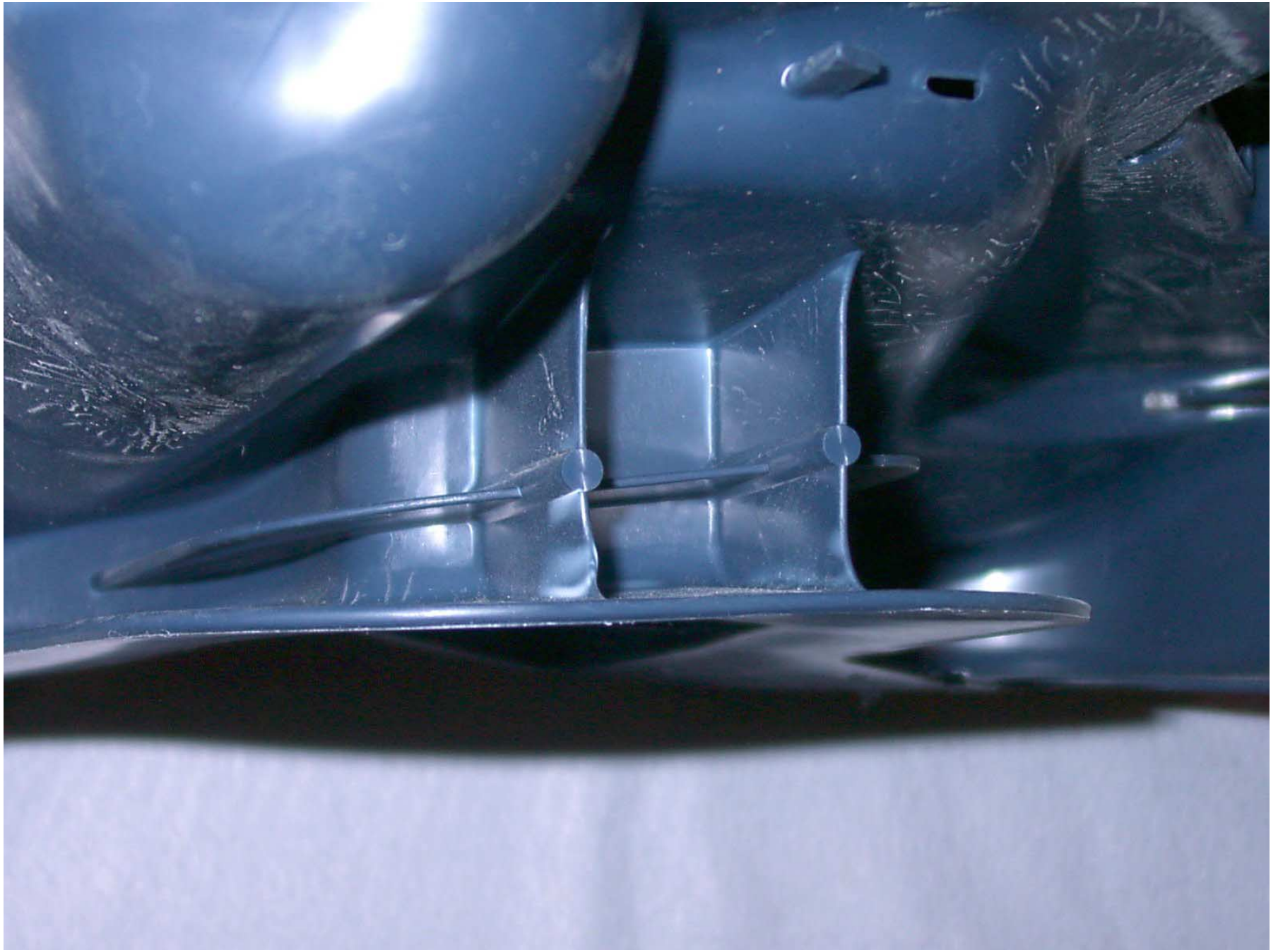
Figure F-34: Post-Test Position 4 Child Seat, Damage to Right Side (Underside View)
