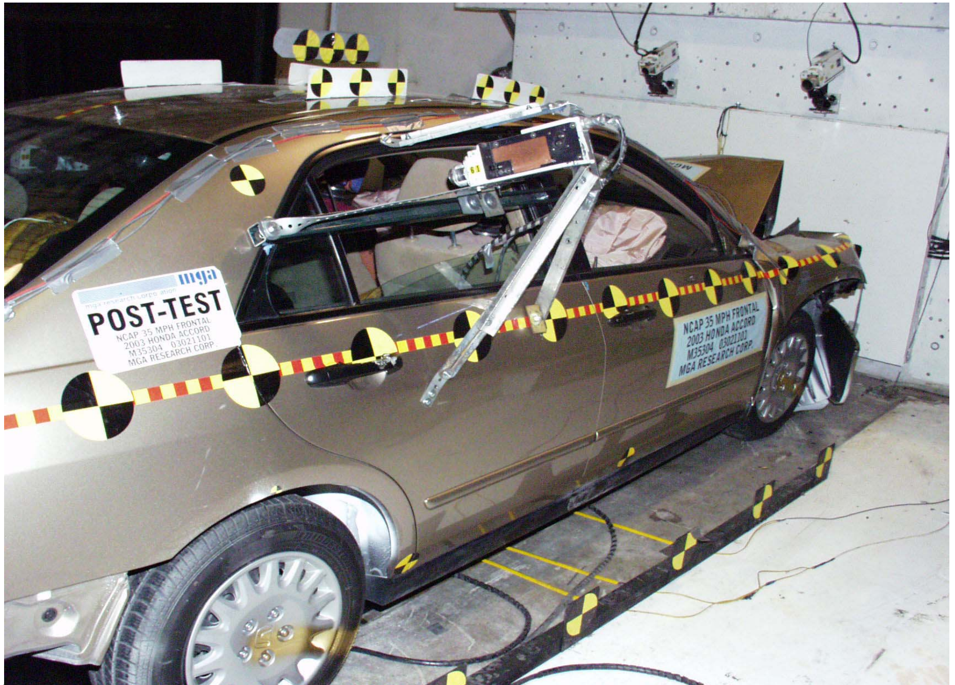
Post-Test Right Rear Three-Quarter View of Doors After Impact
