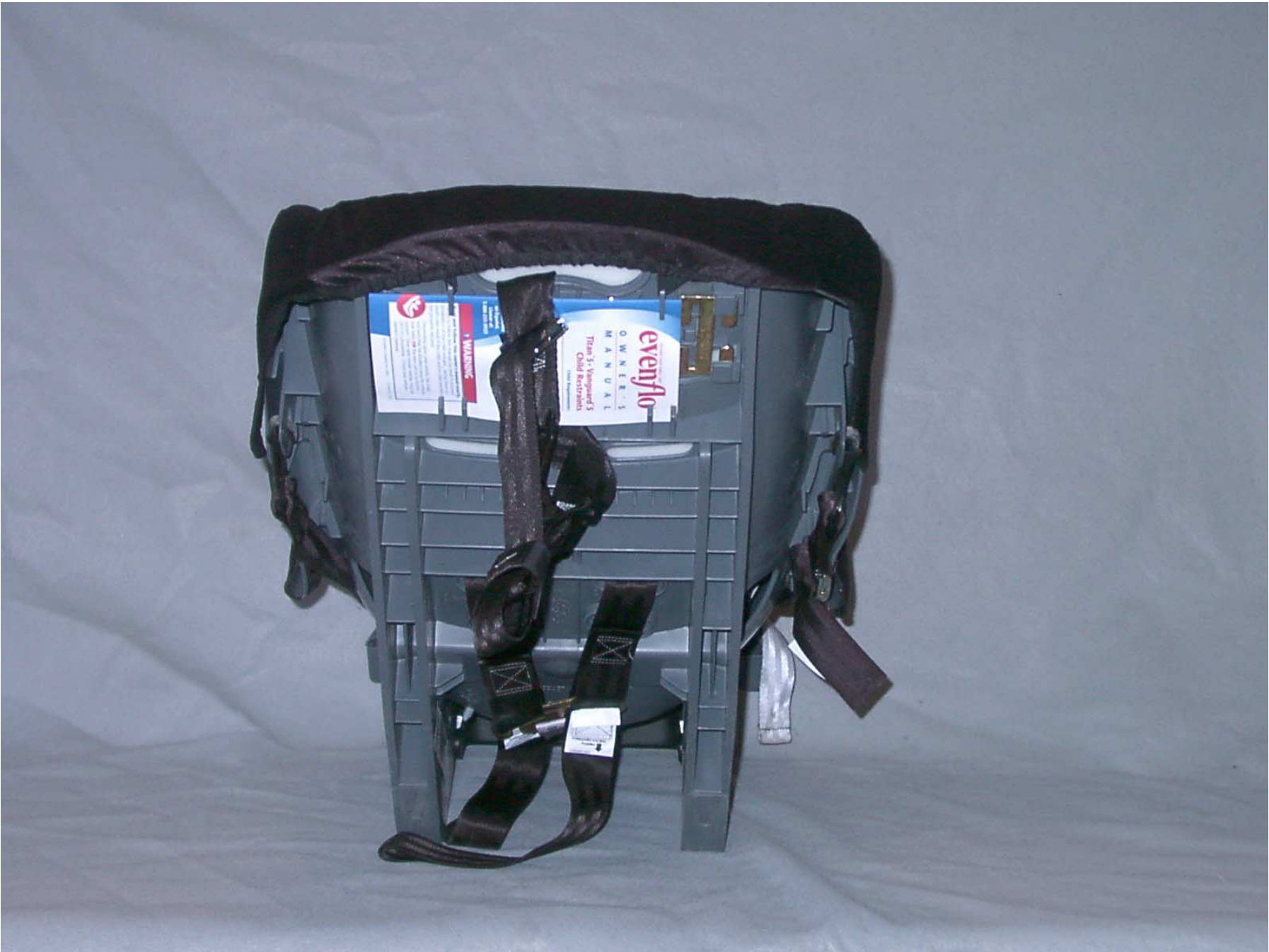
Figure F-19: Pre-Test Rear View of Position 4 CRS
