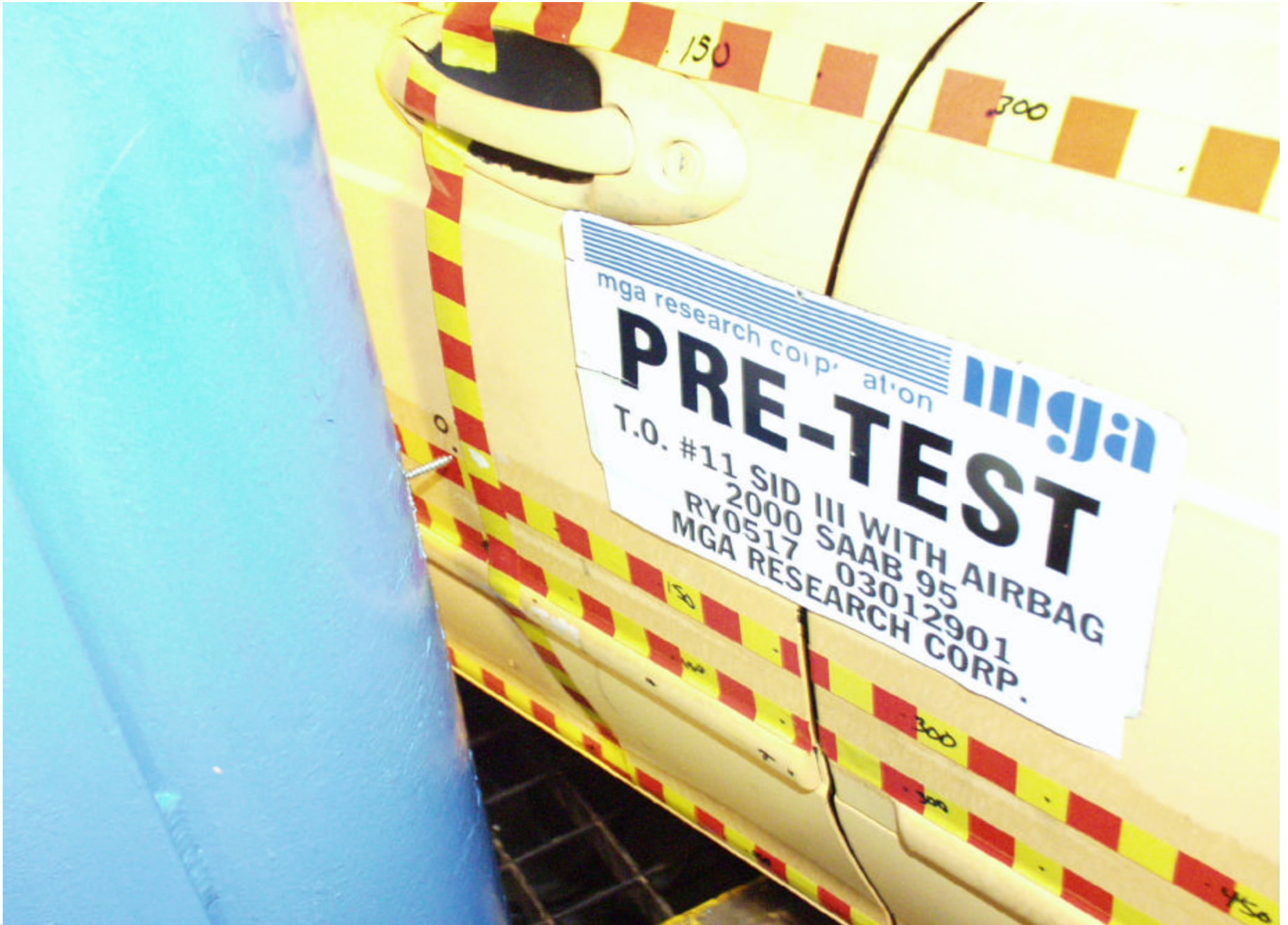
Pre-Test Impact Point on Vehicle
