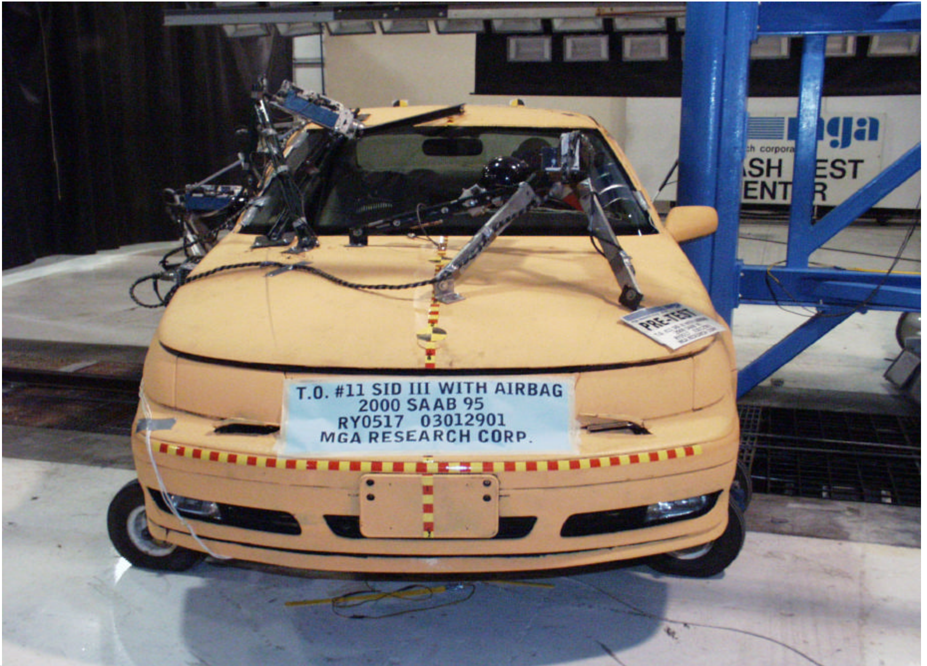
Pre-Test Vehicle Positioned Against Pole (right side)
