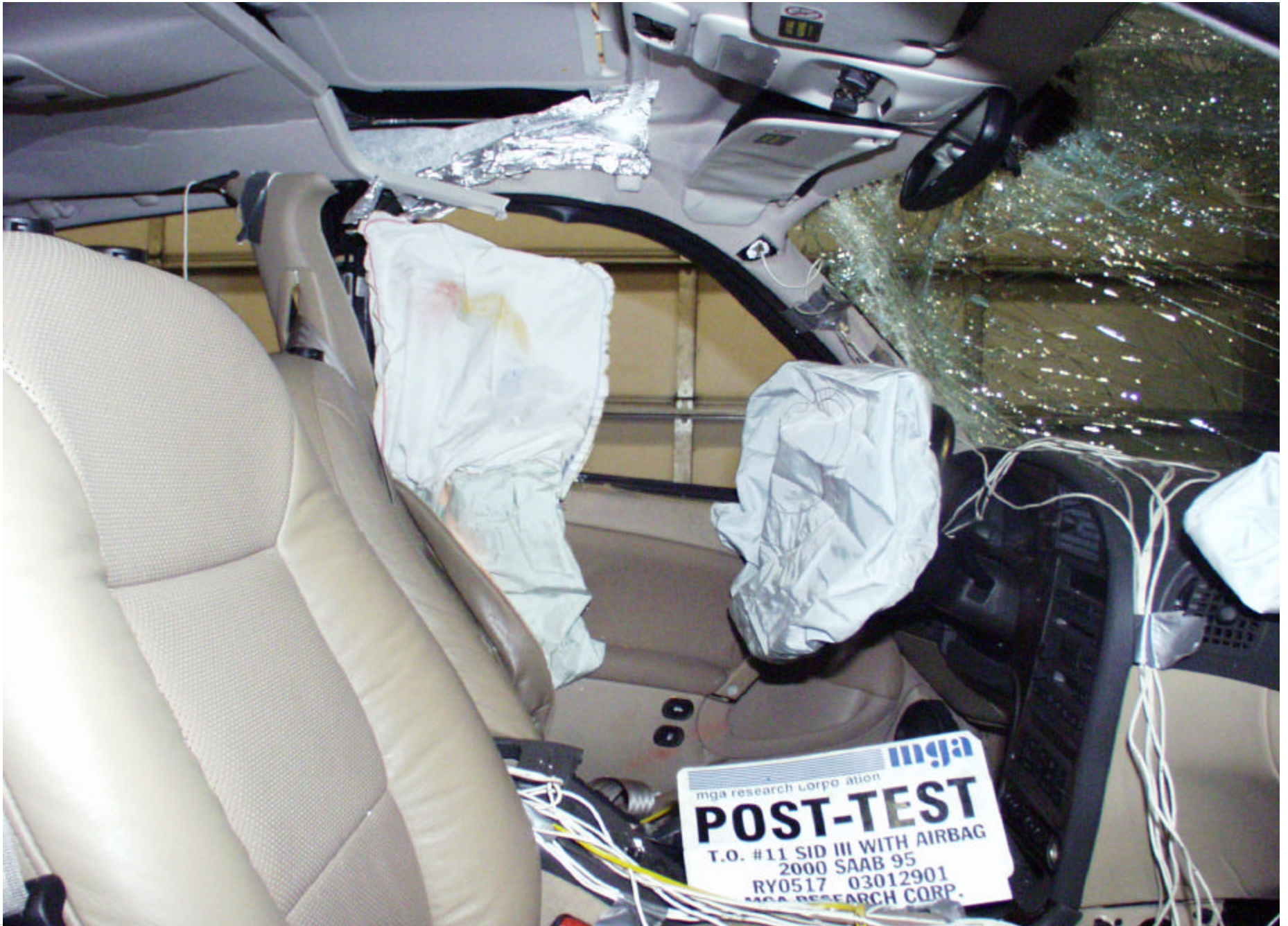
Post-Test Driver Dummy Head Contact
