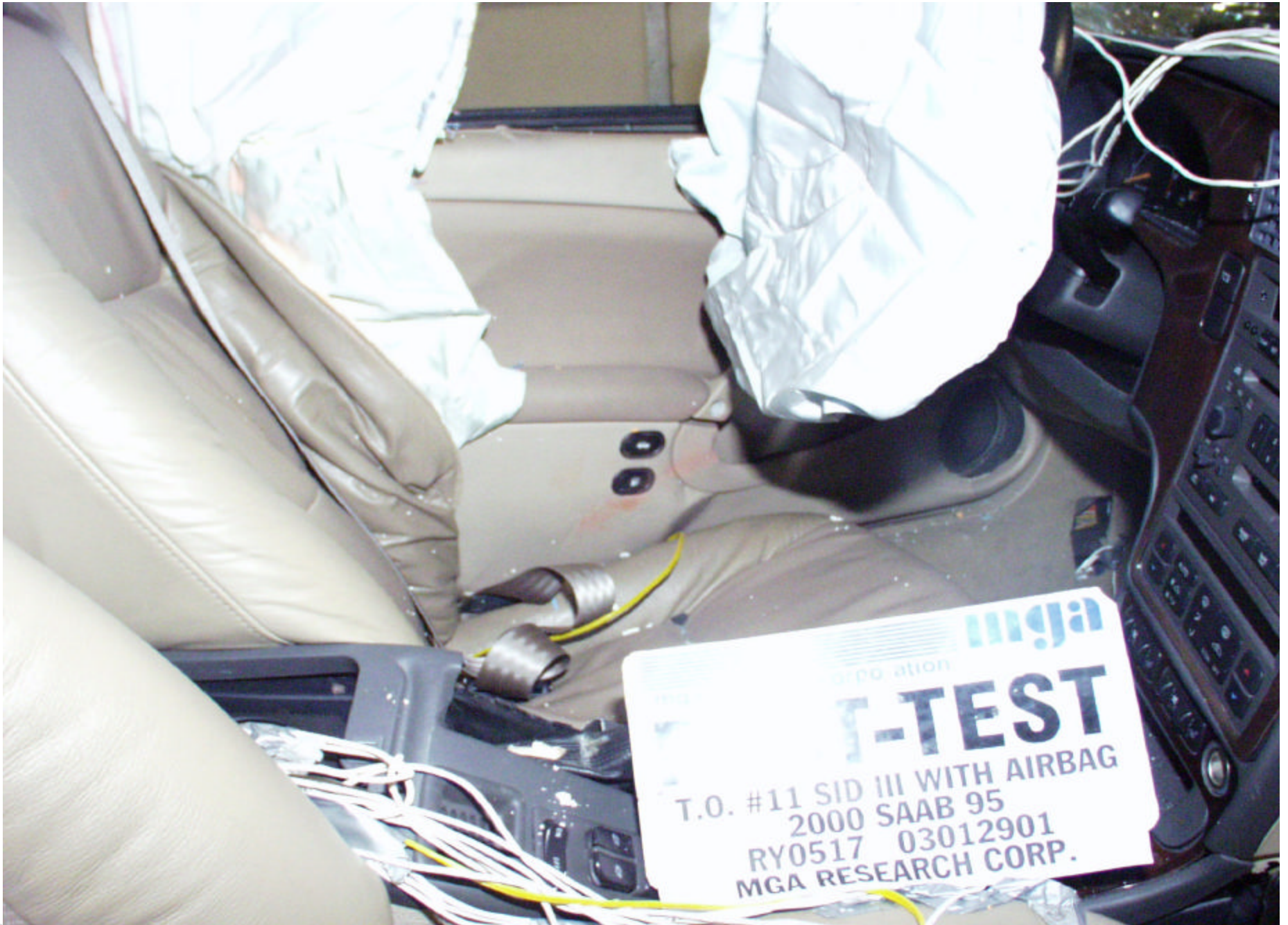
Post-Test Driver Dummy Lower Body Contact
