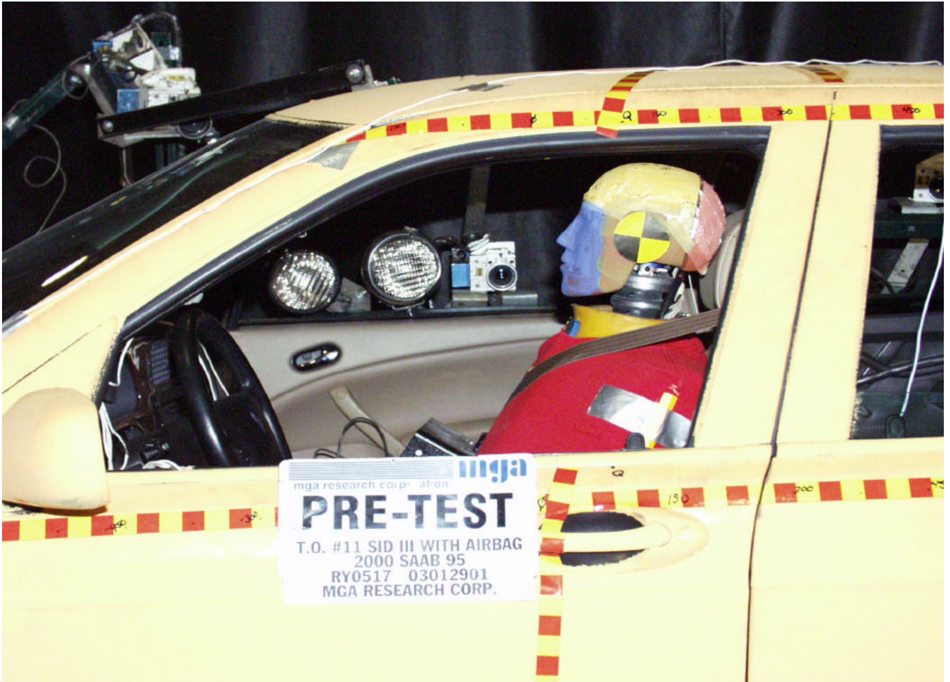
Pre-Test Driver Dummy Left Side View
