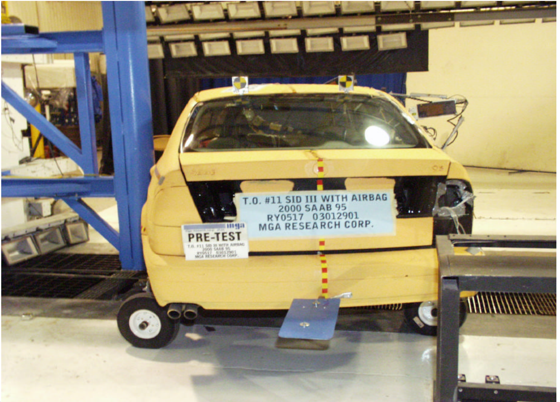
Pre-Test Vehicle Positioned Against Pole (left side)
