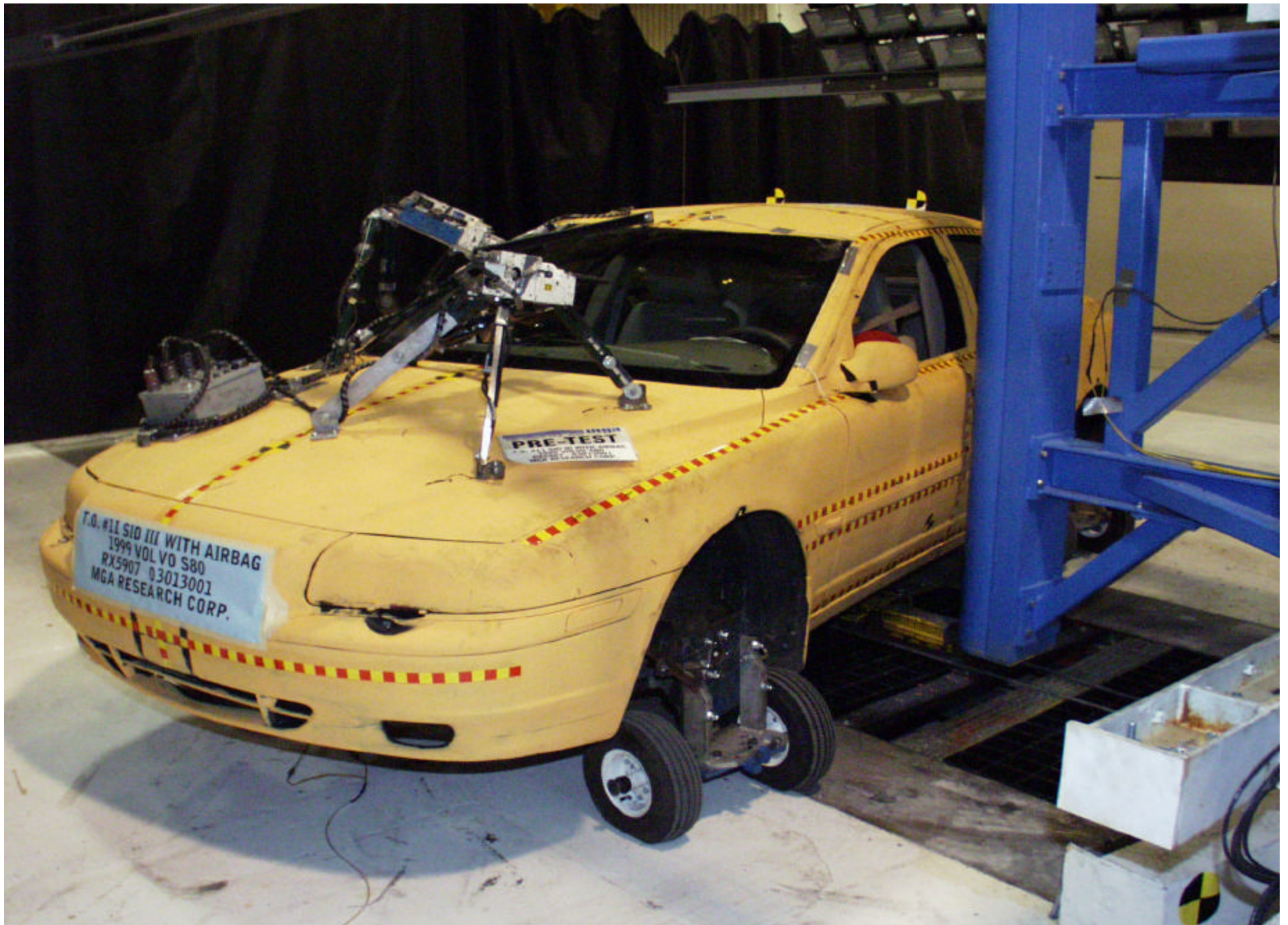
Pre-Test Vehicle Positioned Against Pole (right side)
