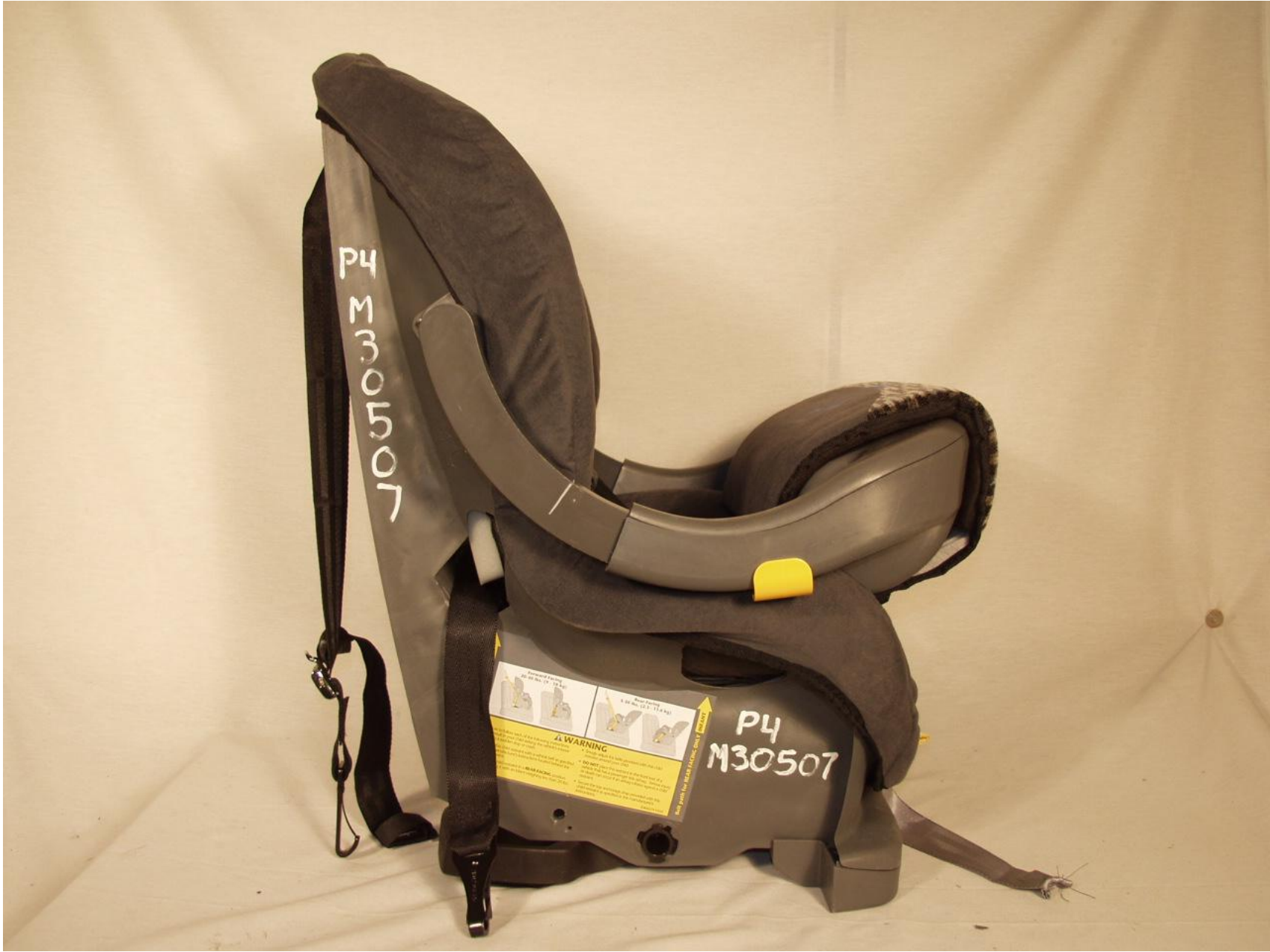
Figure 3-18: POST-TEST RIGHT SIDE VIEW OF POSITION 4 CRS
