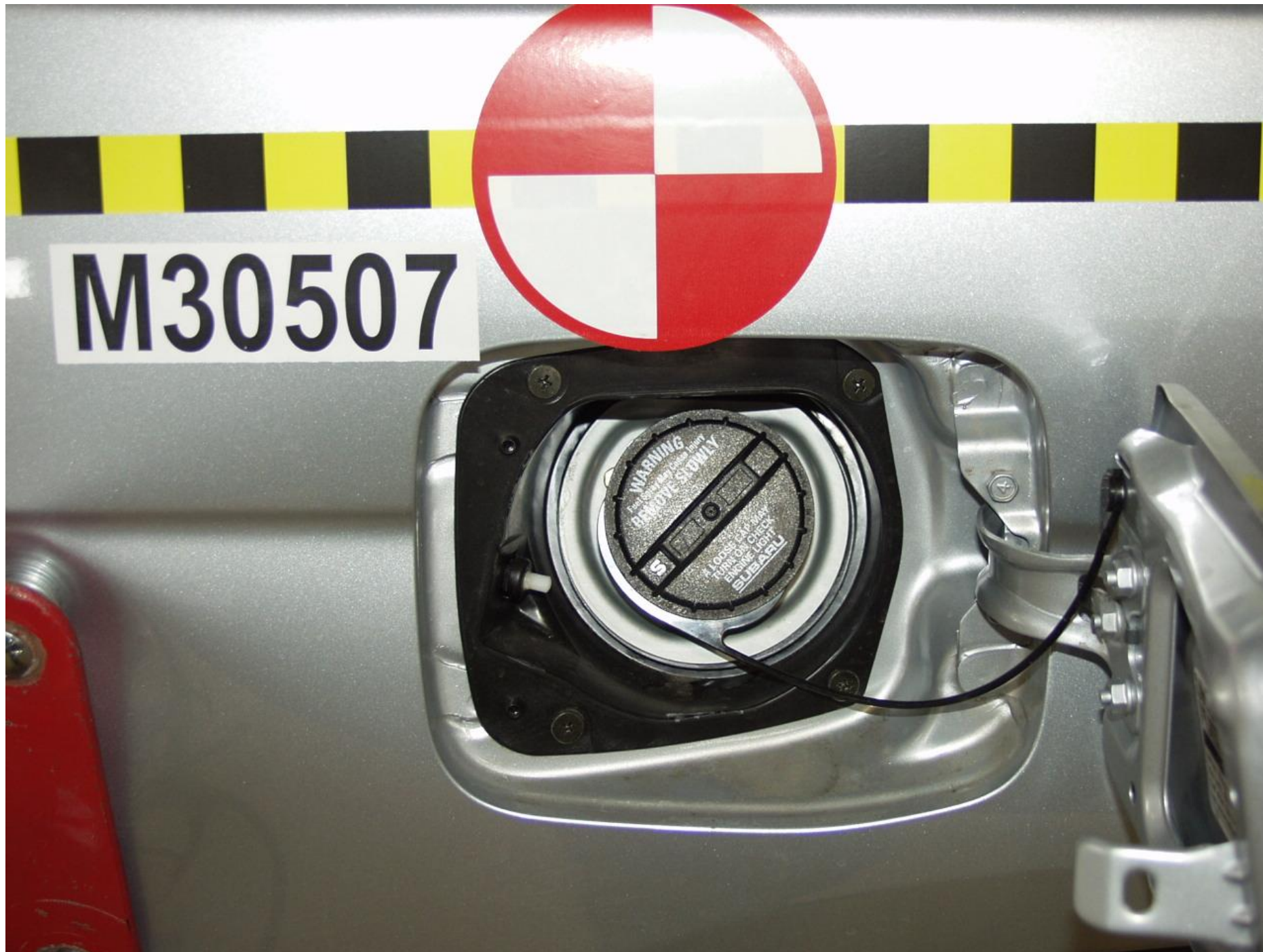
Figure A-23 POST-TEST FUEL CAP VIEW
