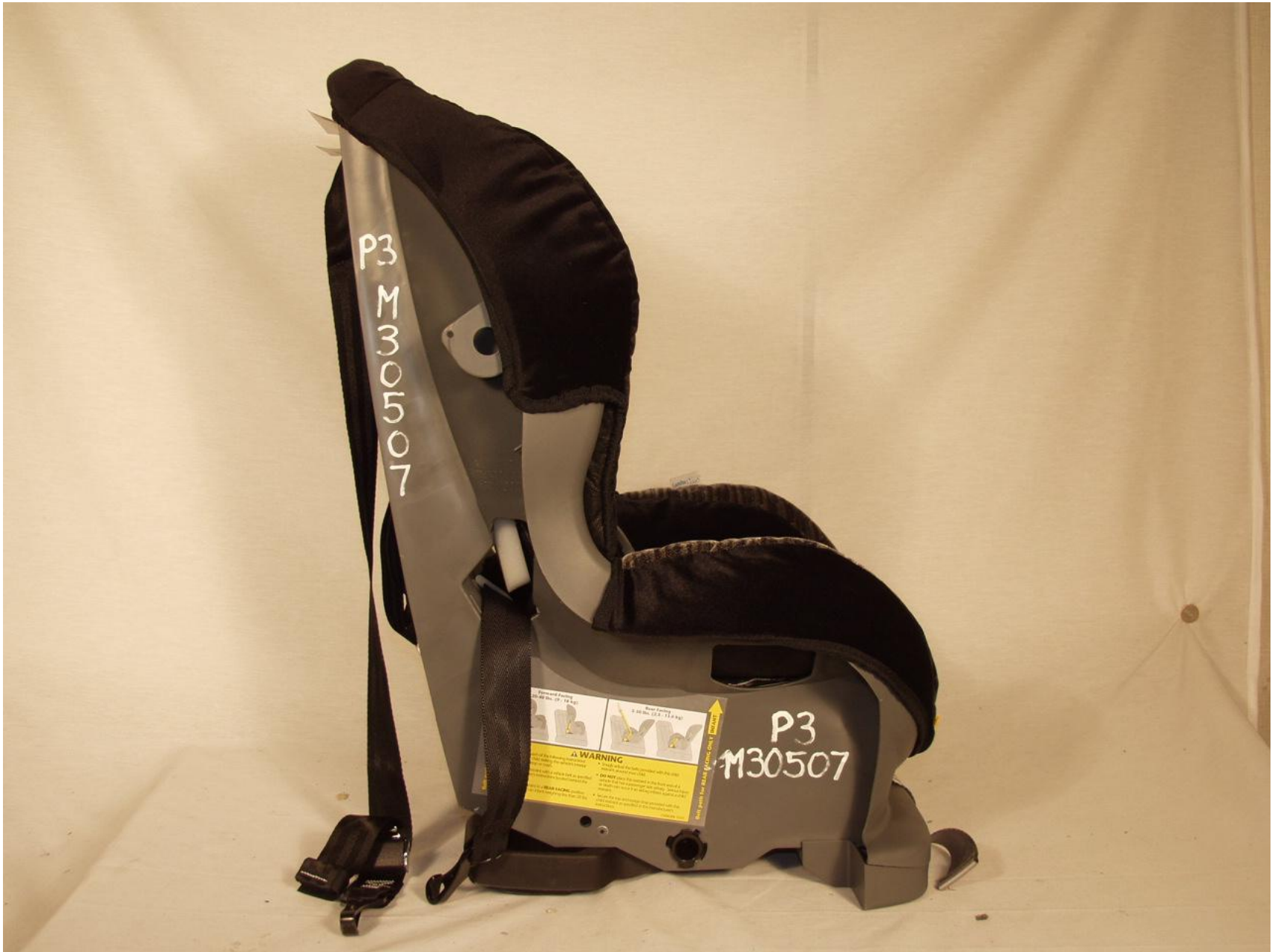
Figure 3-8: PRE-TEST RIGHT SIDE VIEW OF POSITION 3 CRS
