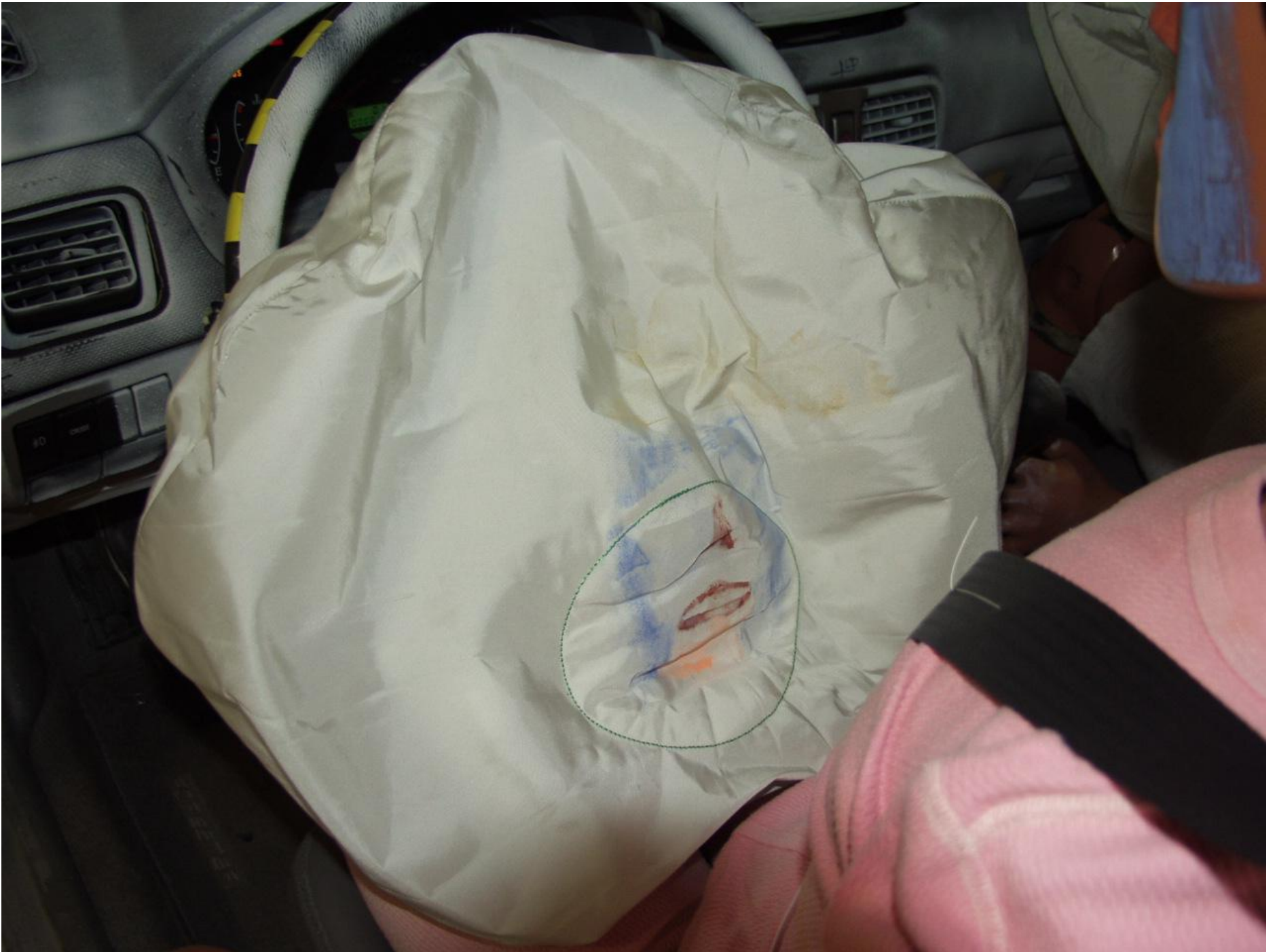
Figure A-43 POST-TEST DRIVER CONTACT TO AIRBAG
