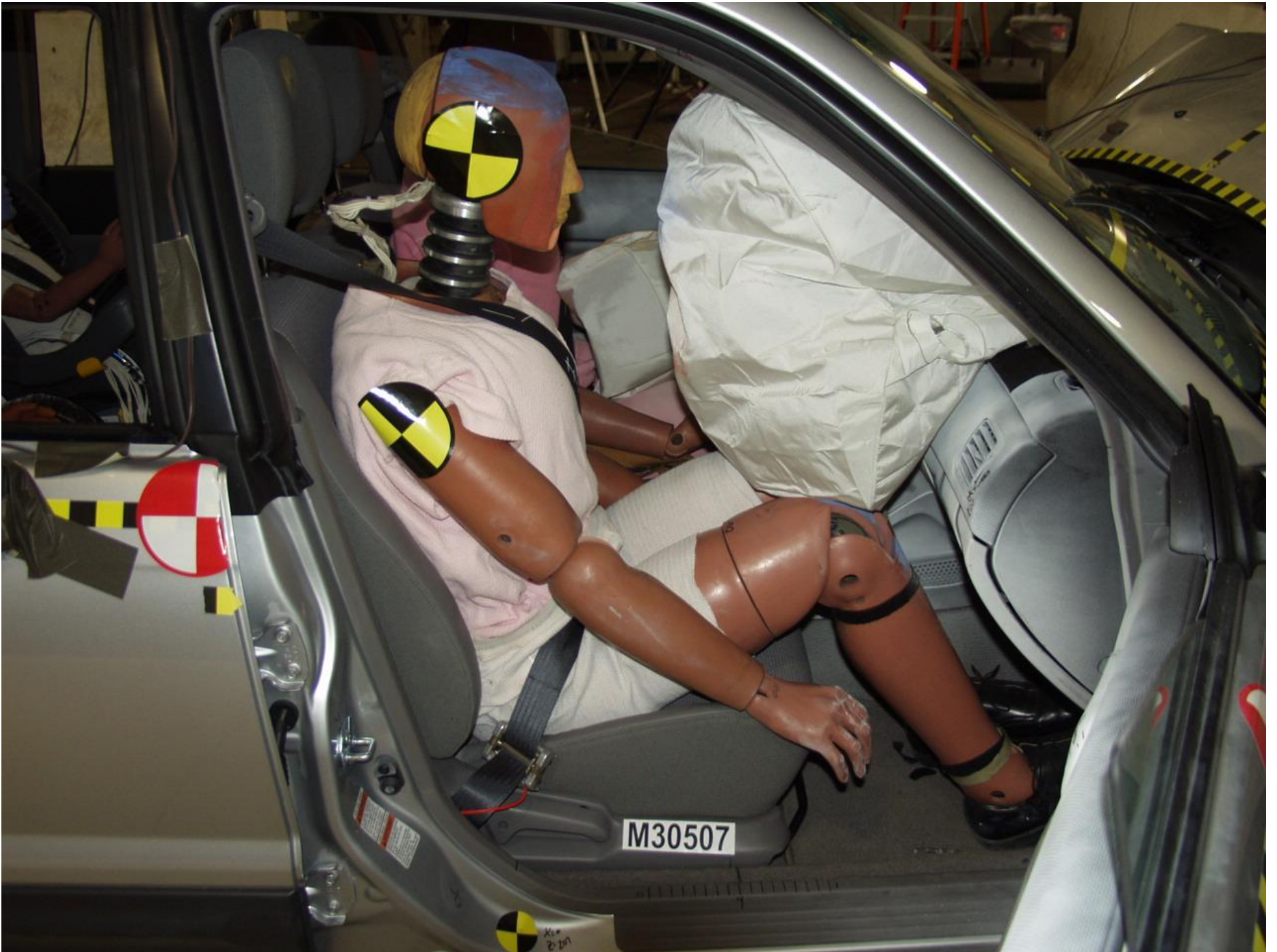
Figure A-49 POST-TEST PASSENGER AND INTERIOR VIEW
