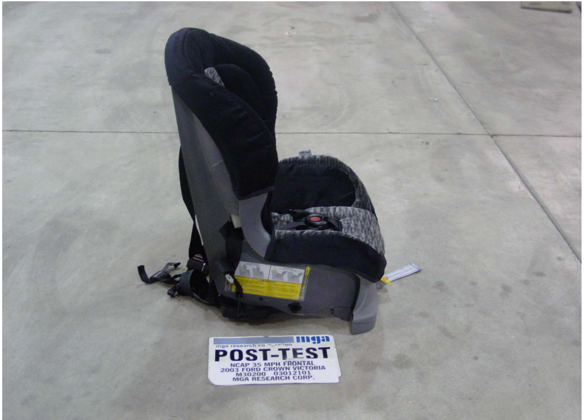
Post-Test Right Side View of Position 3 CRS
