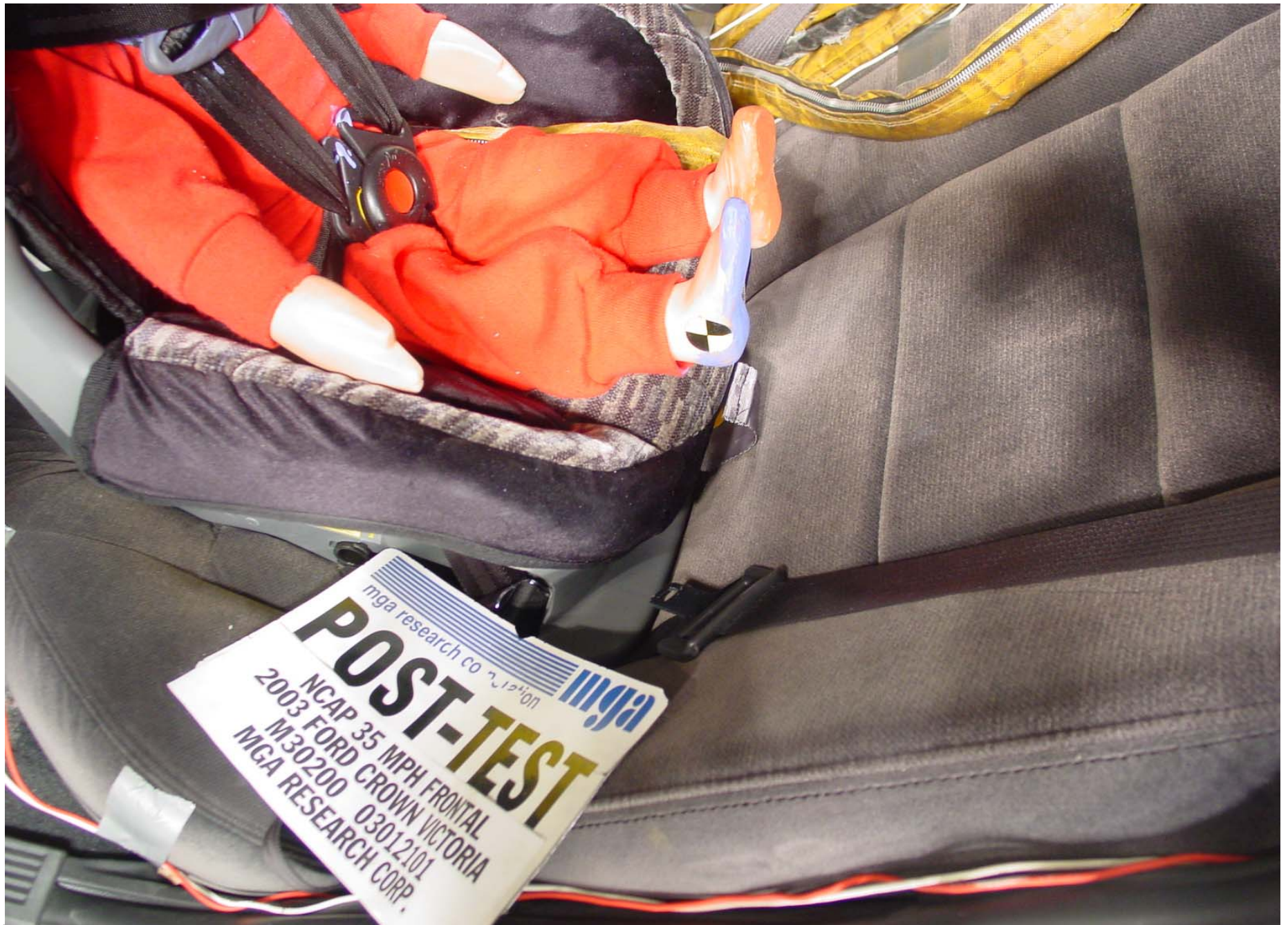
Post-Test Position 4 Feet Contact
