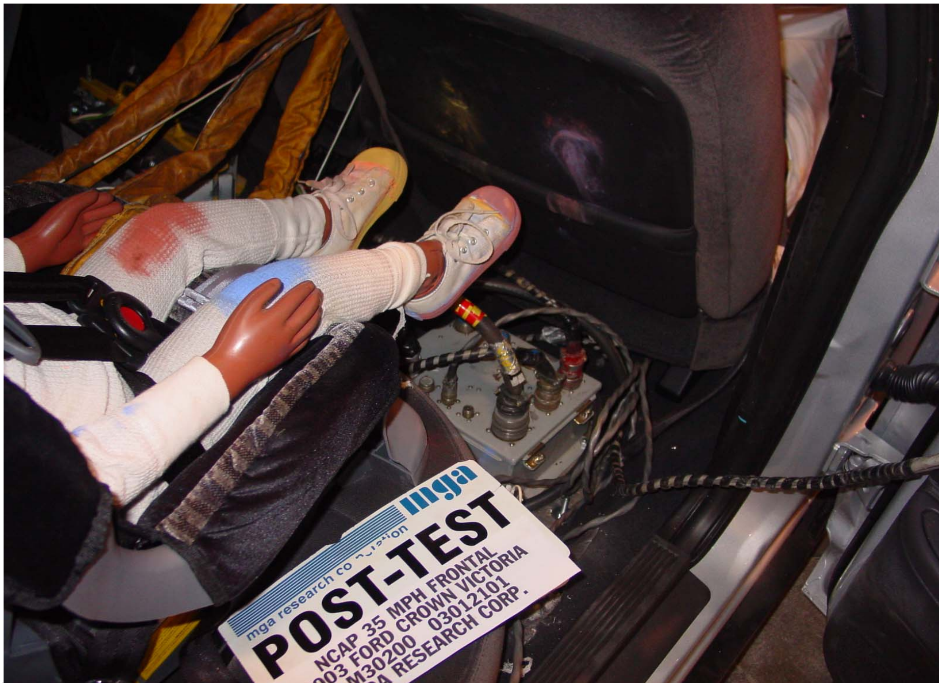
Post-Test Position 3 Feet Contact
