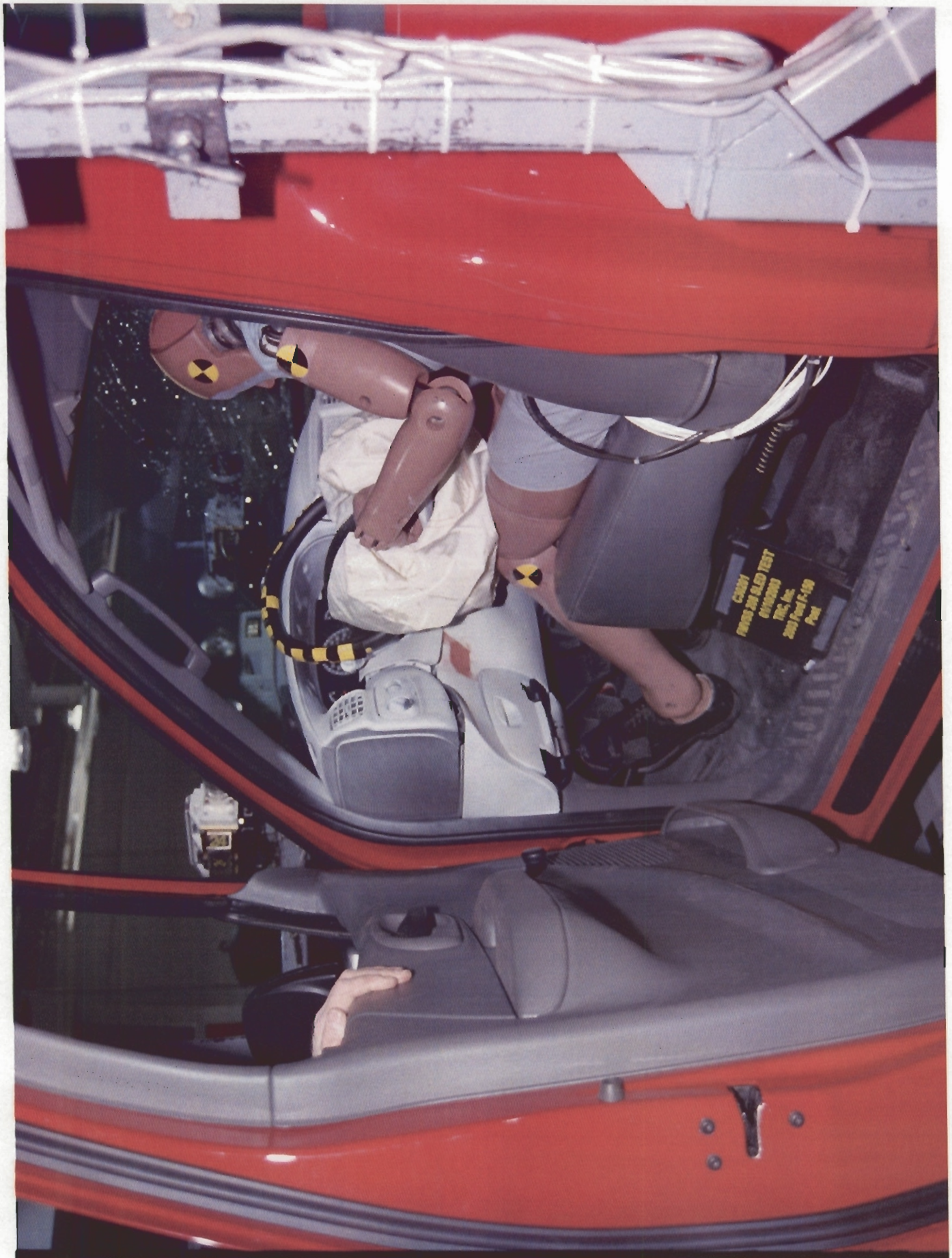
Figure A-12. Post-Test Driver Dummy Position View with Door Open - View 2
