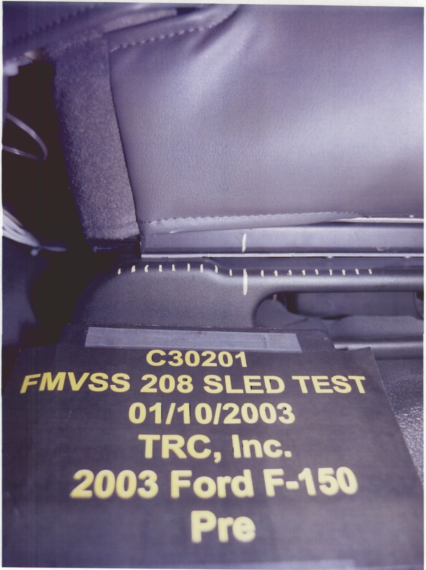
Figure A-21. Pre-Test Passenger Seat Track Position View
