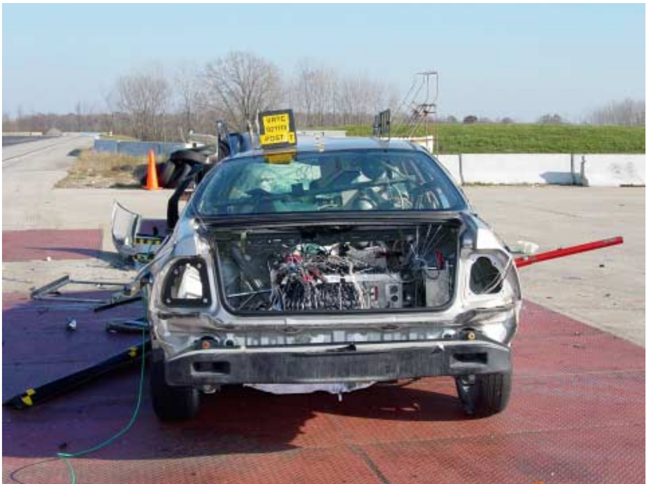
Figure A-11 Post-Test Target Vehicle Rear View
