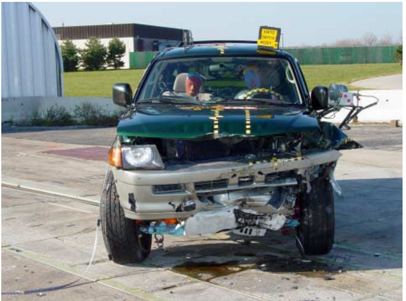
Figure A-23 Post-Test Bullet Vehicle Front View
