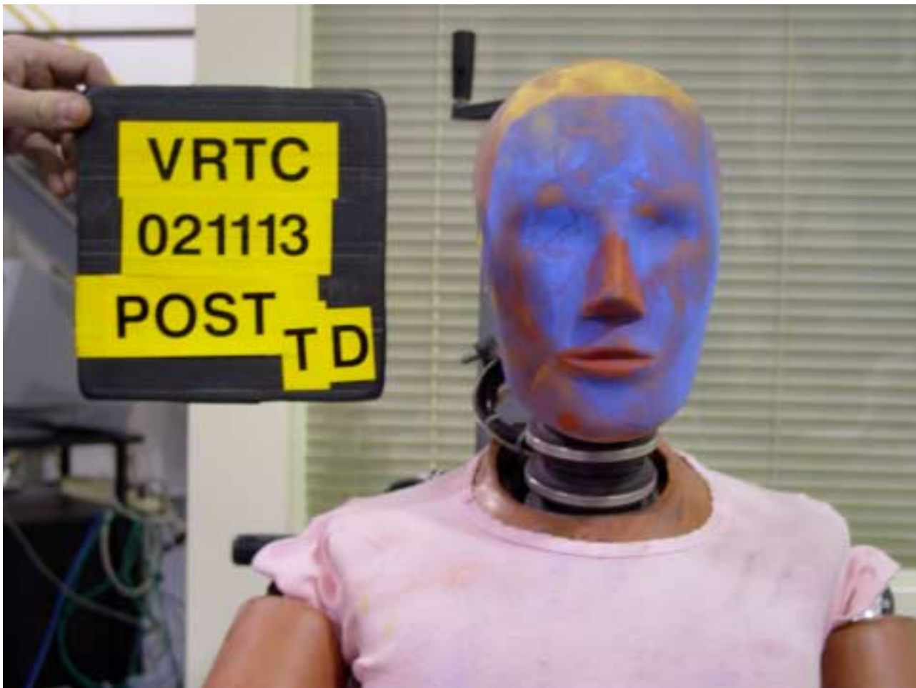
Figure A-68 Post-Test Target Vehicle Driver Dummy Head Contact - View 1
