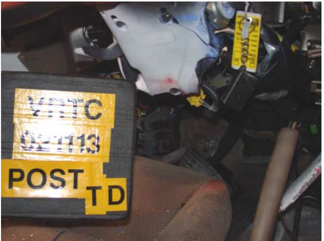
Figure A-76 Post-Test Target Vehicle Driver Dummy Knee Contact - View 2
