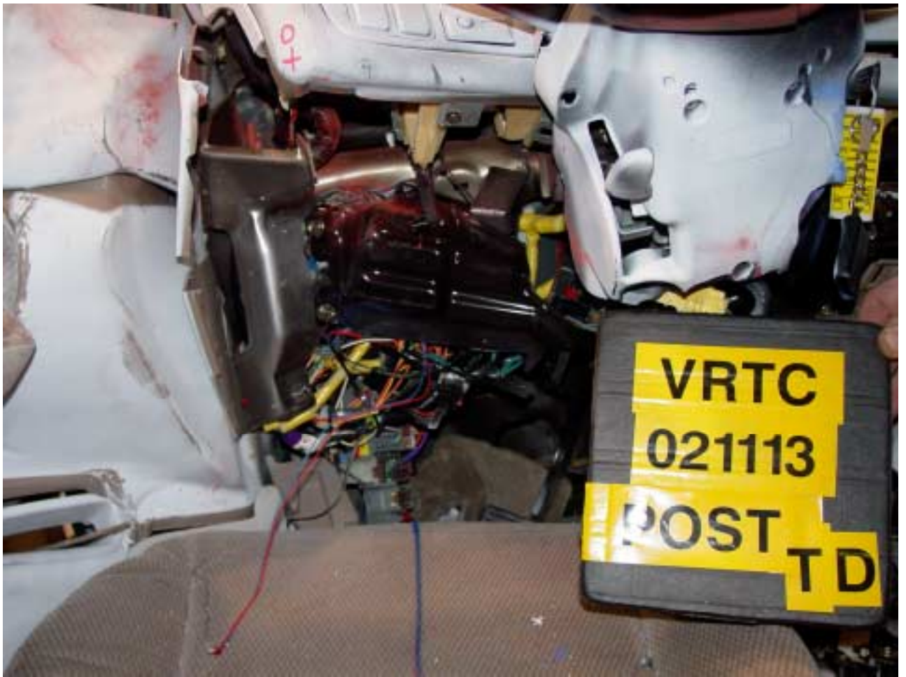
Figure A-77 Post-Test Target Vehicle Driver Dummy Knee Contact - View 3
