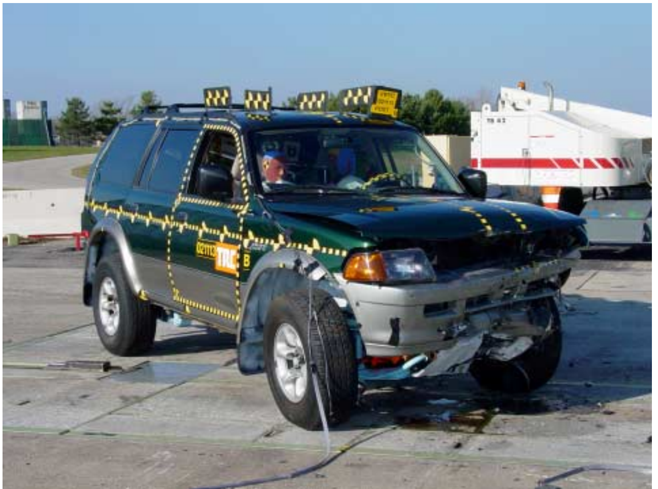
Figure A-35 Post-Test Bullet Vehicle Right Front View
