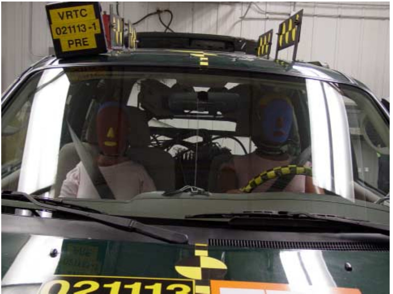
Figure A-49 Pre-Test Bullet Vehicle Driver and Passenger Dummies through Windshield View
