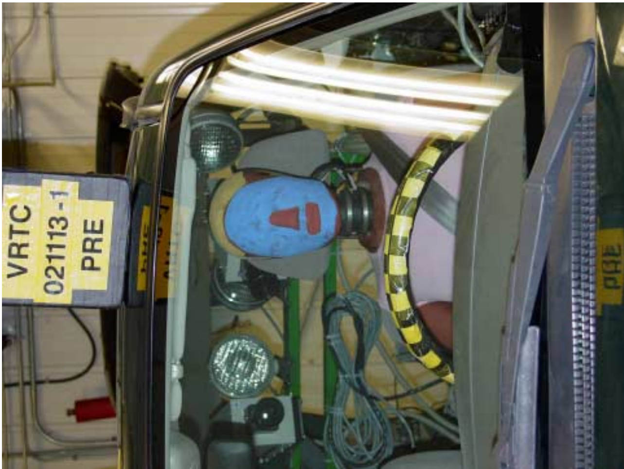
Figure A-51 Pre-Test Bullet Vehicle Driver Dummy - View 1
