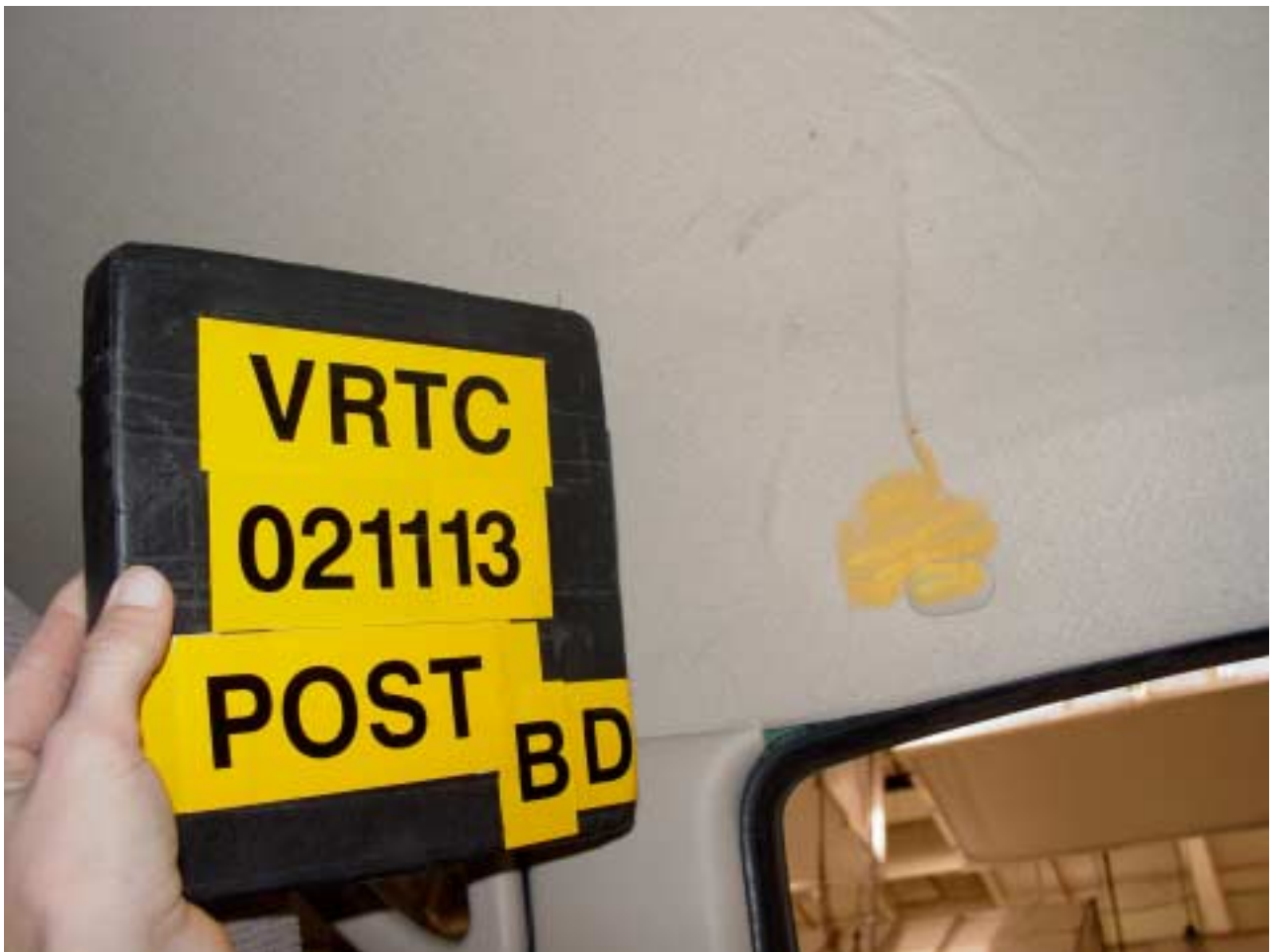
Figure A-81 Post-Test Bullet Vehicle Driver Dummy Head Contact - View 3
