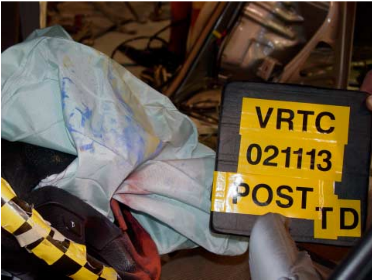
Figure A-73 Post-Test Target Vehicle Driver Dummy Head Contact - View 6
