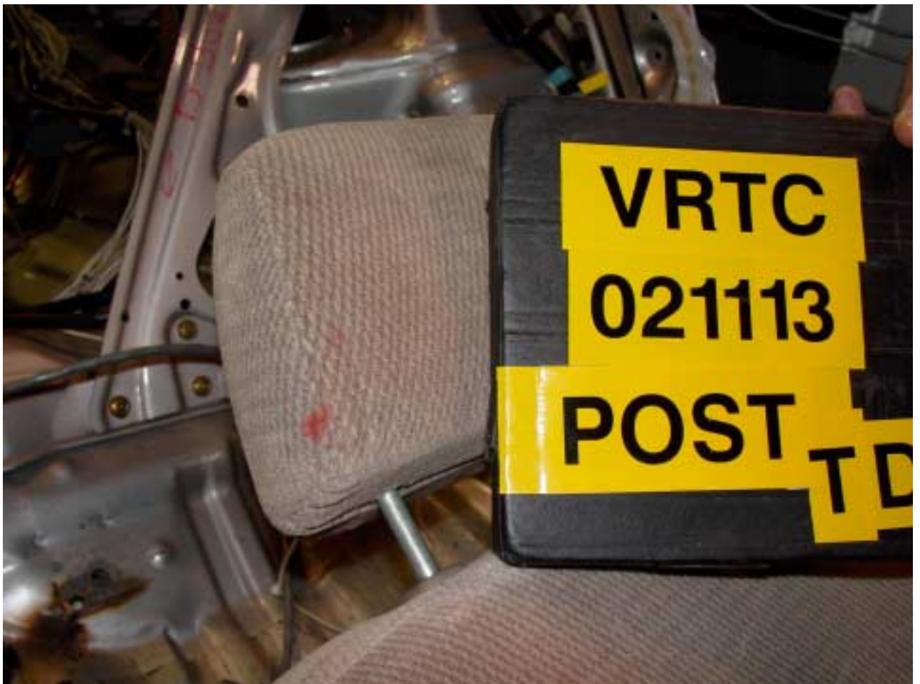
Figure A-74 Post-Test Target Vehicle Driver Dummy Head Contact - View 7
