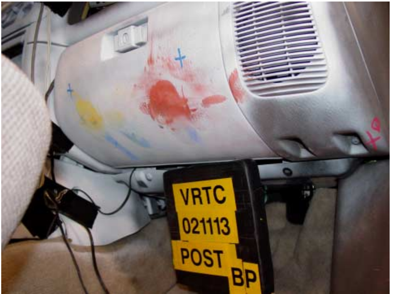
Figure A-88 Post-Test Bullet Vehicle Passenger Dummy Knee Contact - View 2
