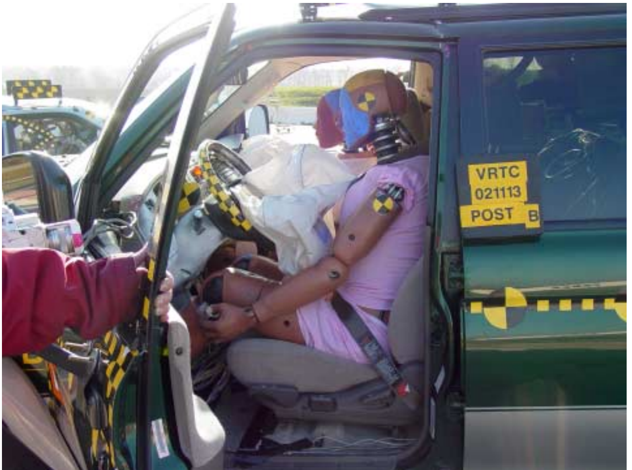
Figure A-56 Post-Test Bullet Vehicle Driver Dummy - View 3
