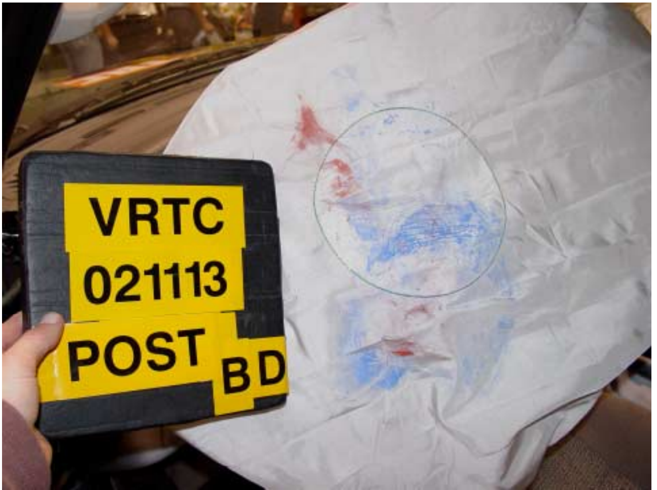
Figure A-80 Post-Test Bullet Vehicle Driver Dummy Head Contact - View 2
