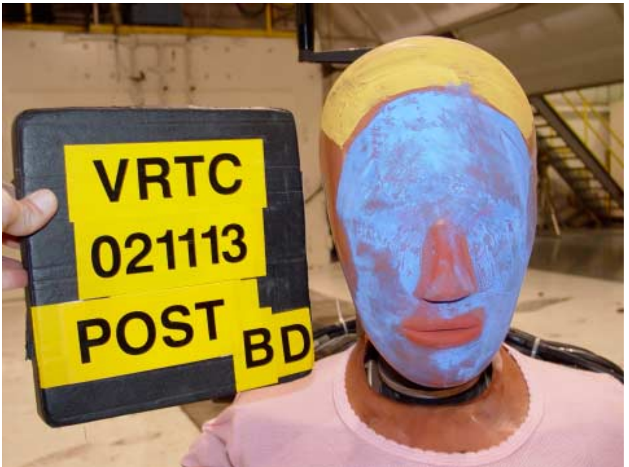
Figure A-79 Post-Test Bullet Vehicle Driver Dummy Head Contact - View 1
