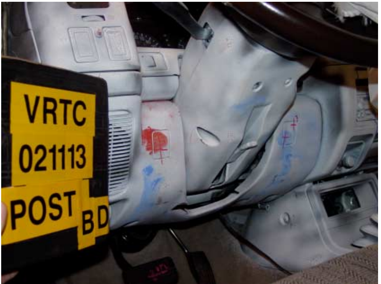
Figure A-83 Post-Test Bullet Vehicle Driver Dummy Knee Contact - View 2
