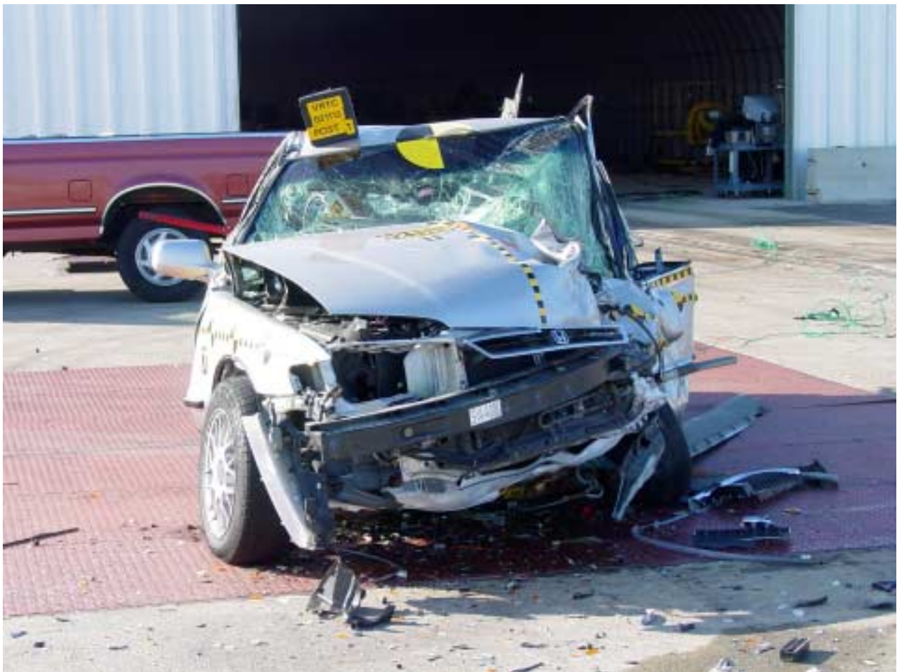
Figure A-4 Post-Test Target Vehicle Front View
