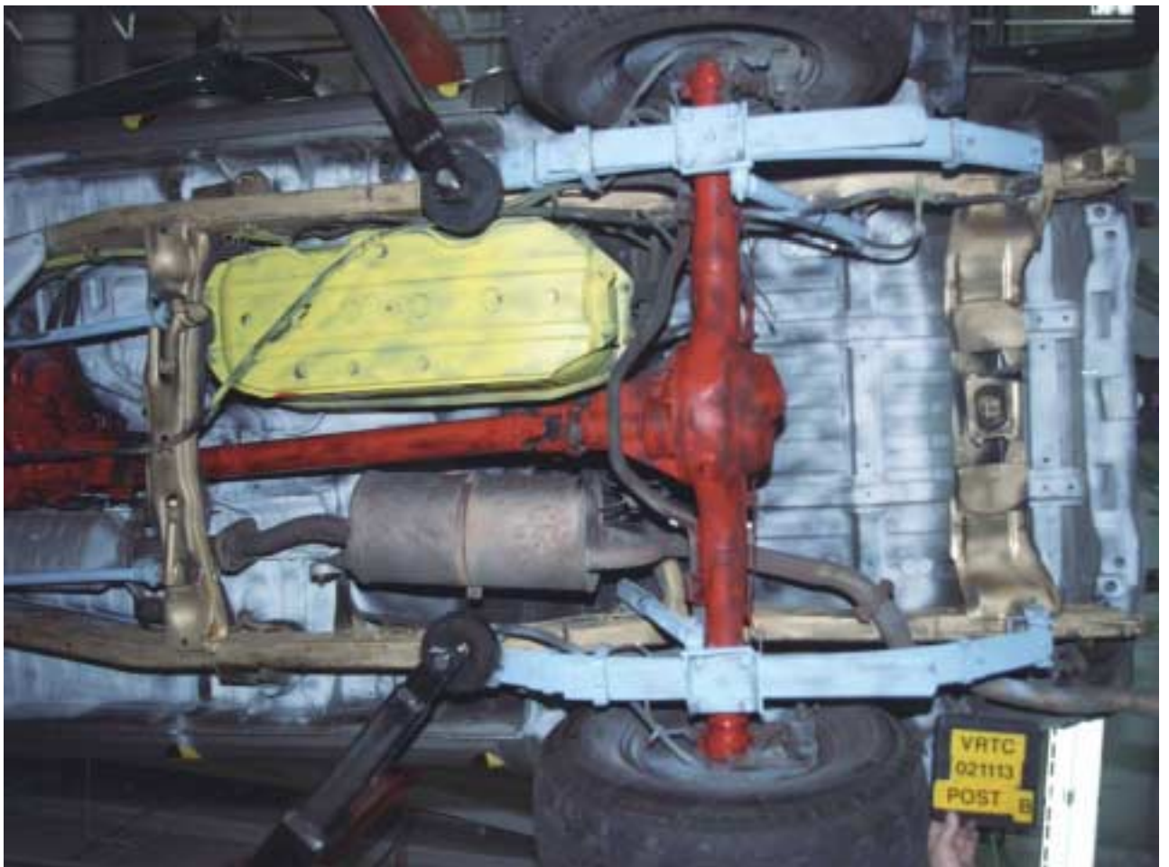
Figure A-40 Post-Test Bullet Vehicle Rear Underbody View
