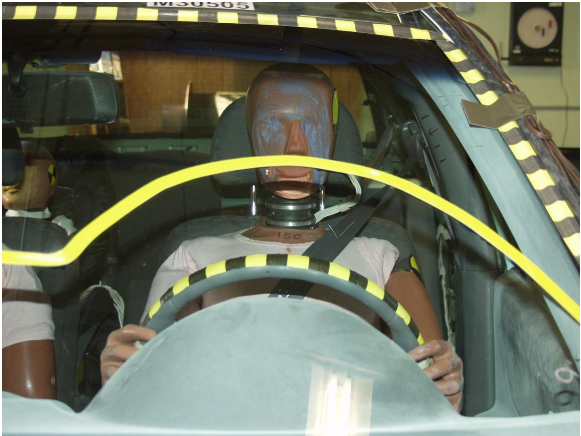
Figure A-30 PRE-TEST DRIVER HEAD LOCATION
