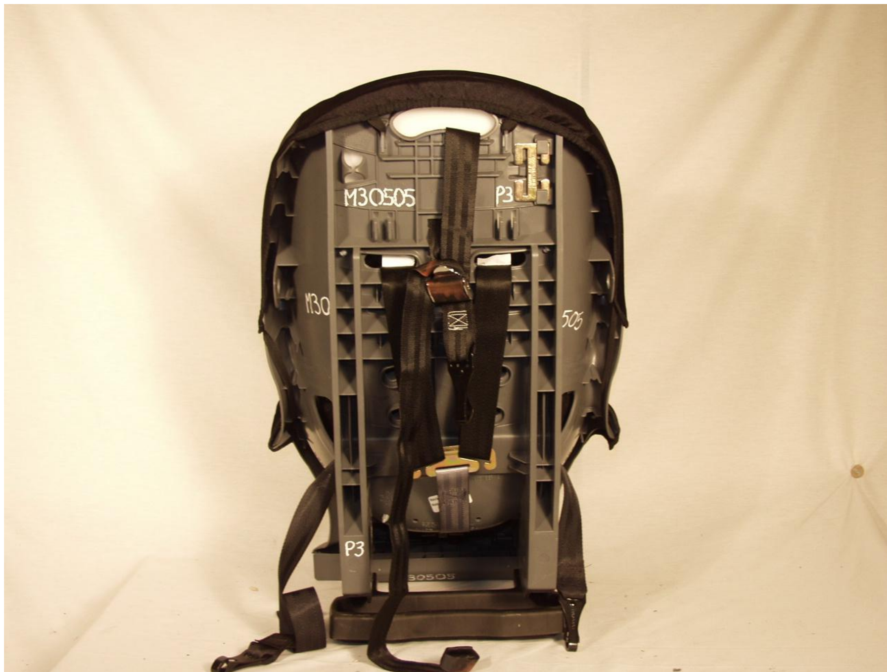
Figure 3-5: POST-TEST REAR VIEW OF POSITION 3CRS
