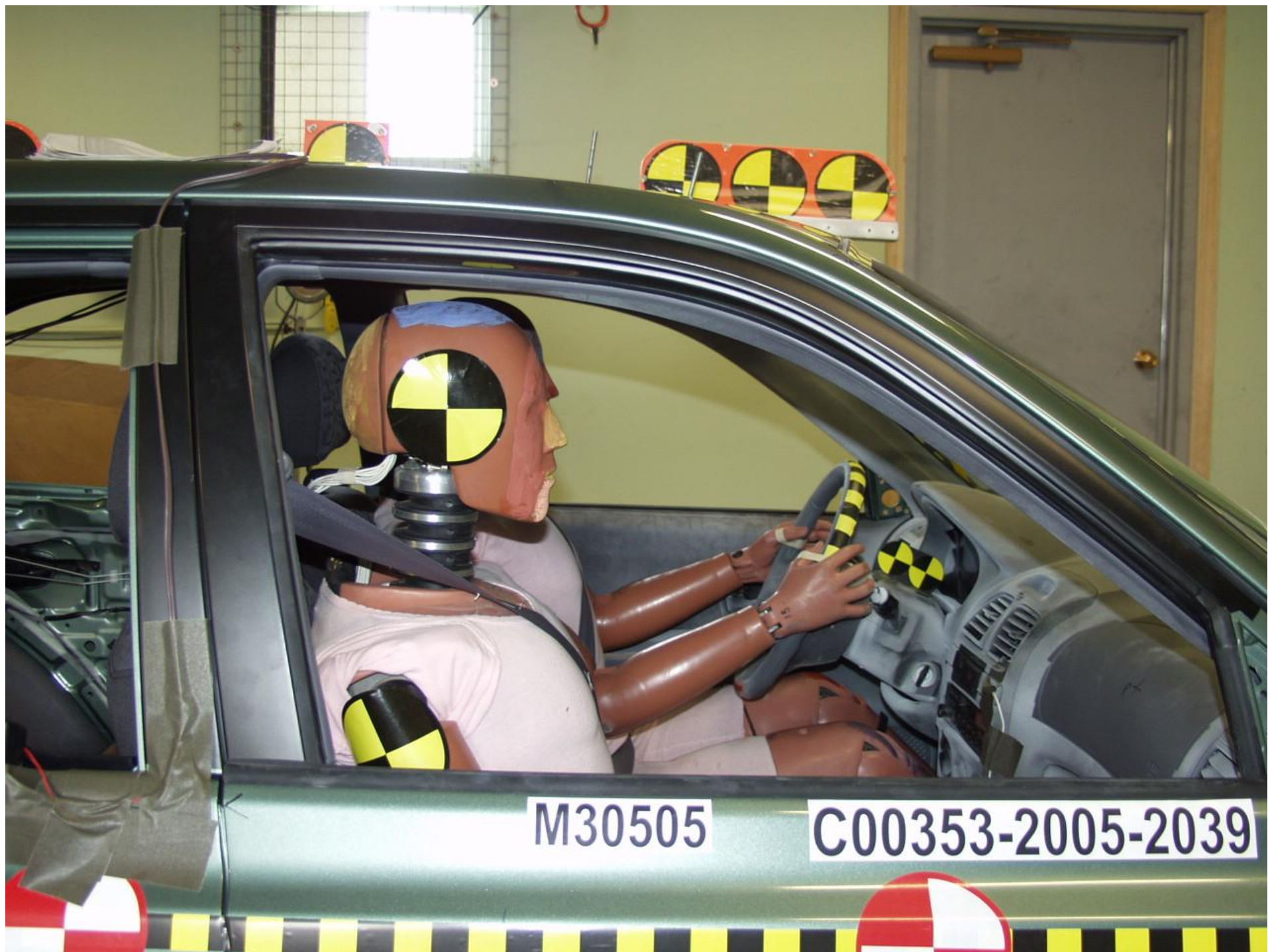
Figure A-46 PRE-TEST PASSENGER POSITION VIEW
