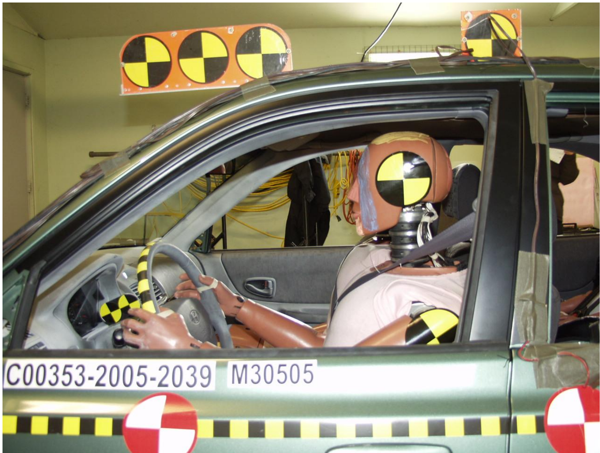
Figure A-32 PRE-TEST DRIVER POSITION VIEW
