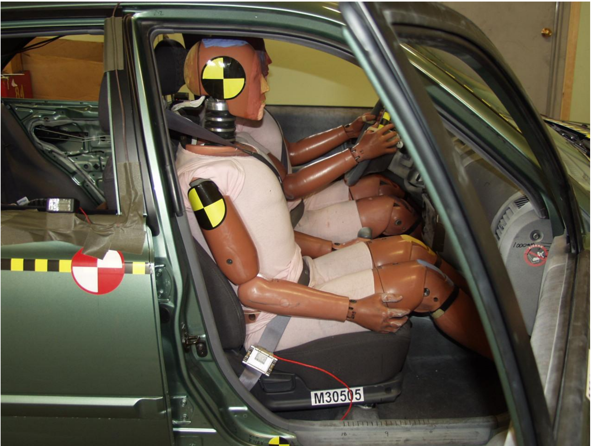
Figure A-48 PRE-TEST PASSENGER AND INTERIOR VIEW
