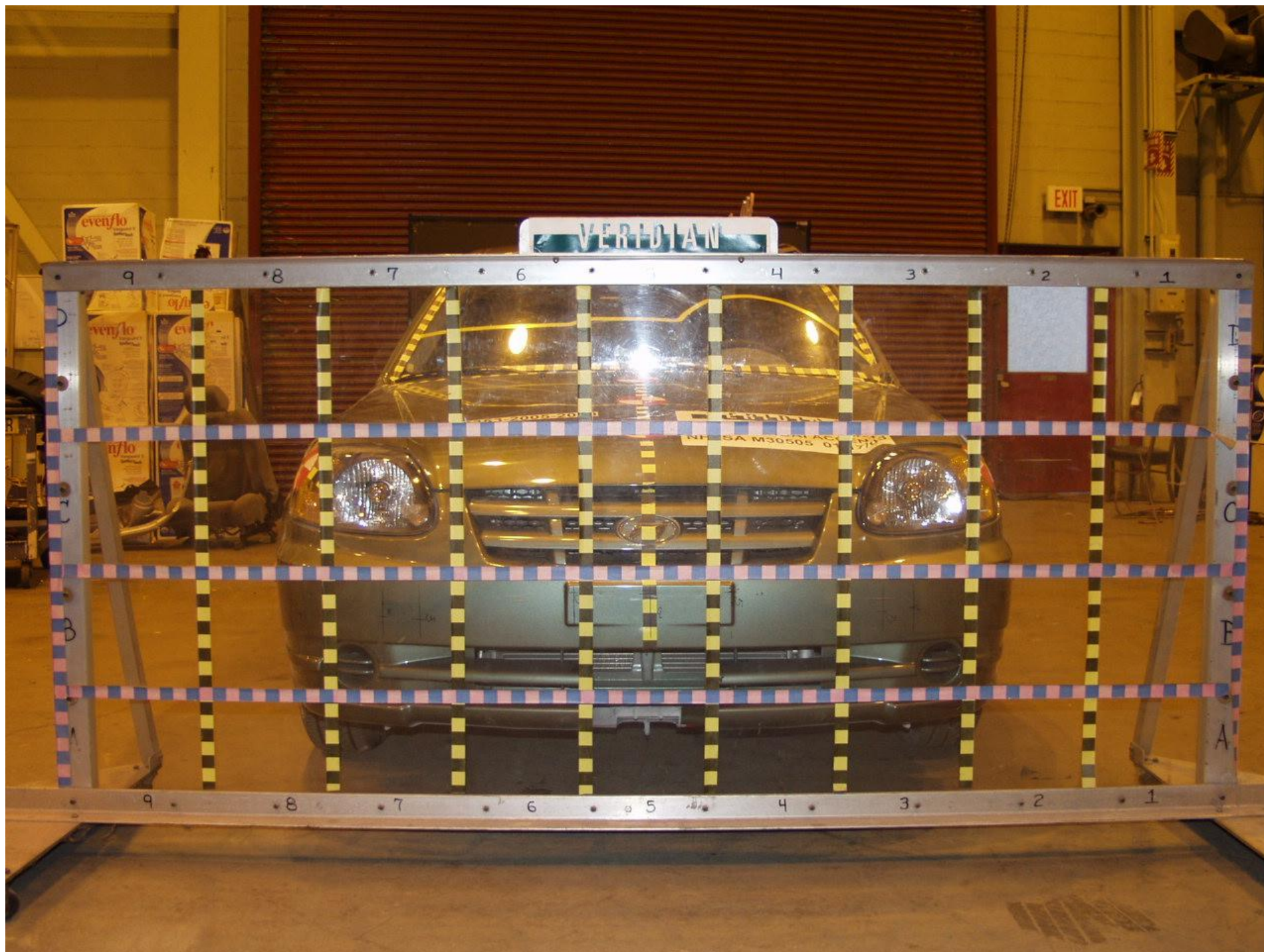
Figure A-1 LOAD CELL LOCATIONS
