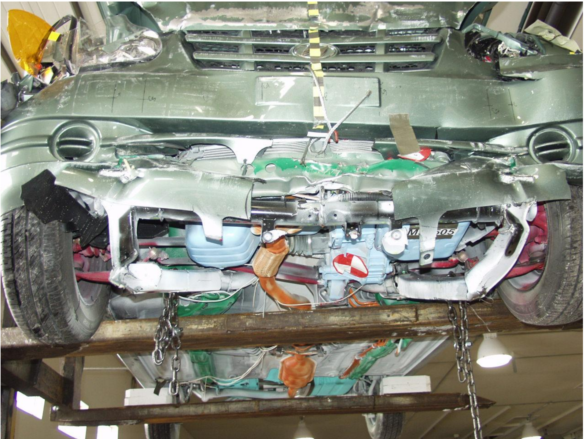
Figure A-25 POST-TEST FRONT UNDERBODY VIEW
