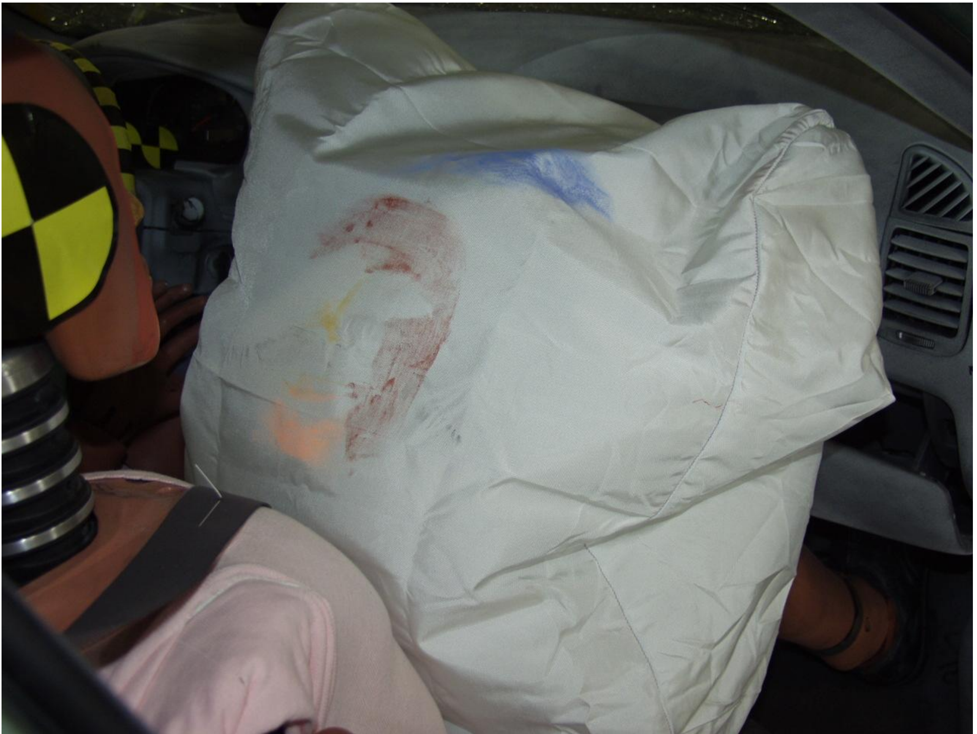
Figure A-57 POST-TEST PASSENGER CONTACT TO AIRBAG
