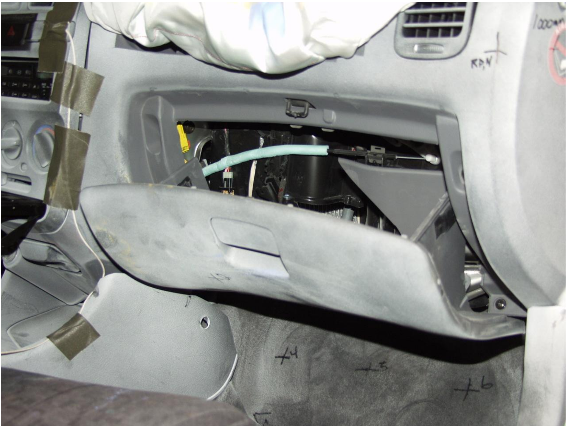
Figure A-53 POST-TEST PASSENGER KNEE BOLSTER VIEW
