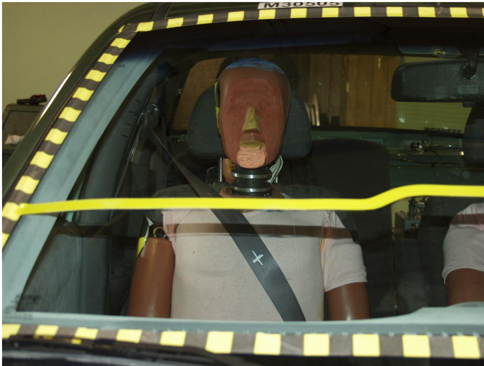
Figure A-44 PRE-TEST PASSENGER HEAD LOCATION
