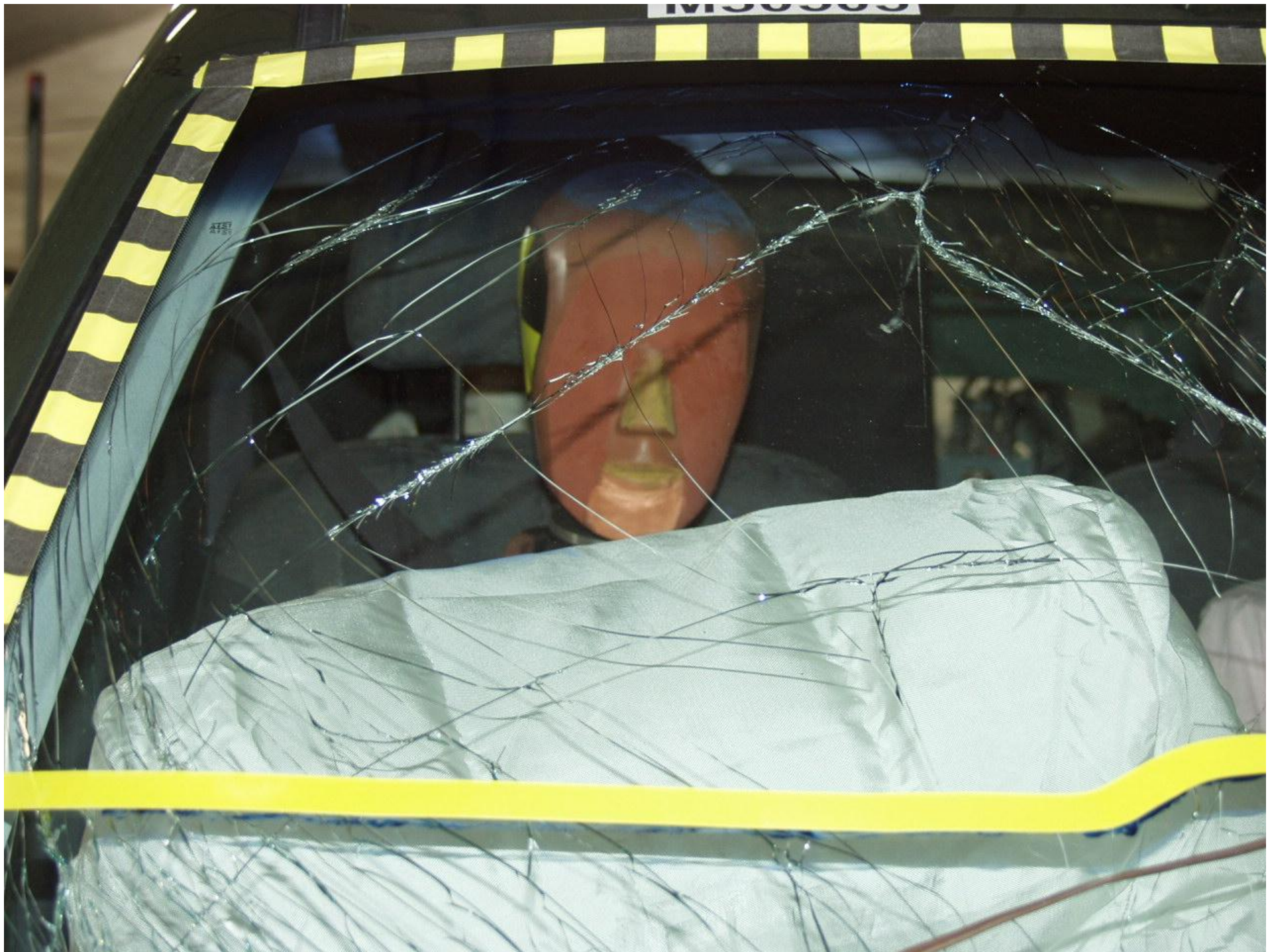
Figure A-45 POST-TEST PASSENGER HEAD LOCATION
