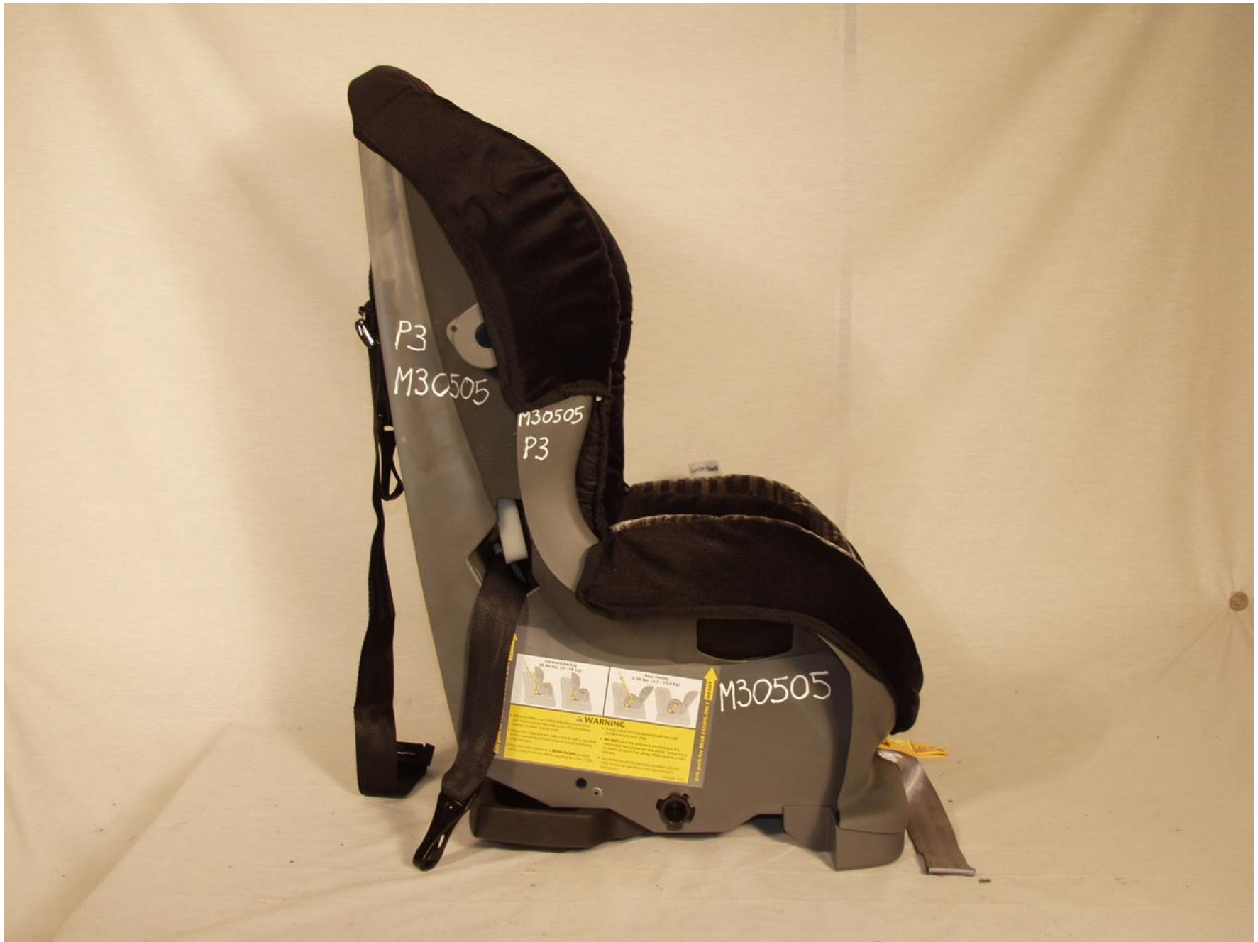
Figure 3-9: POST-TEST RIGHT SIDE VIEW OF POSITION 3CRS
