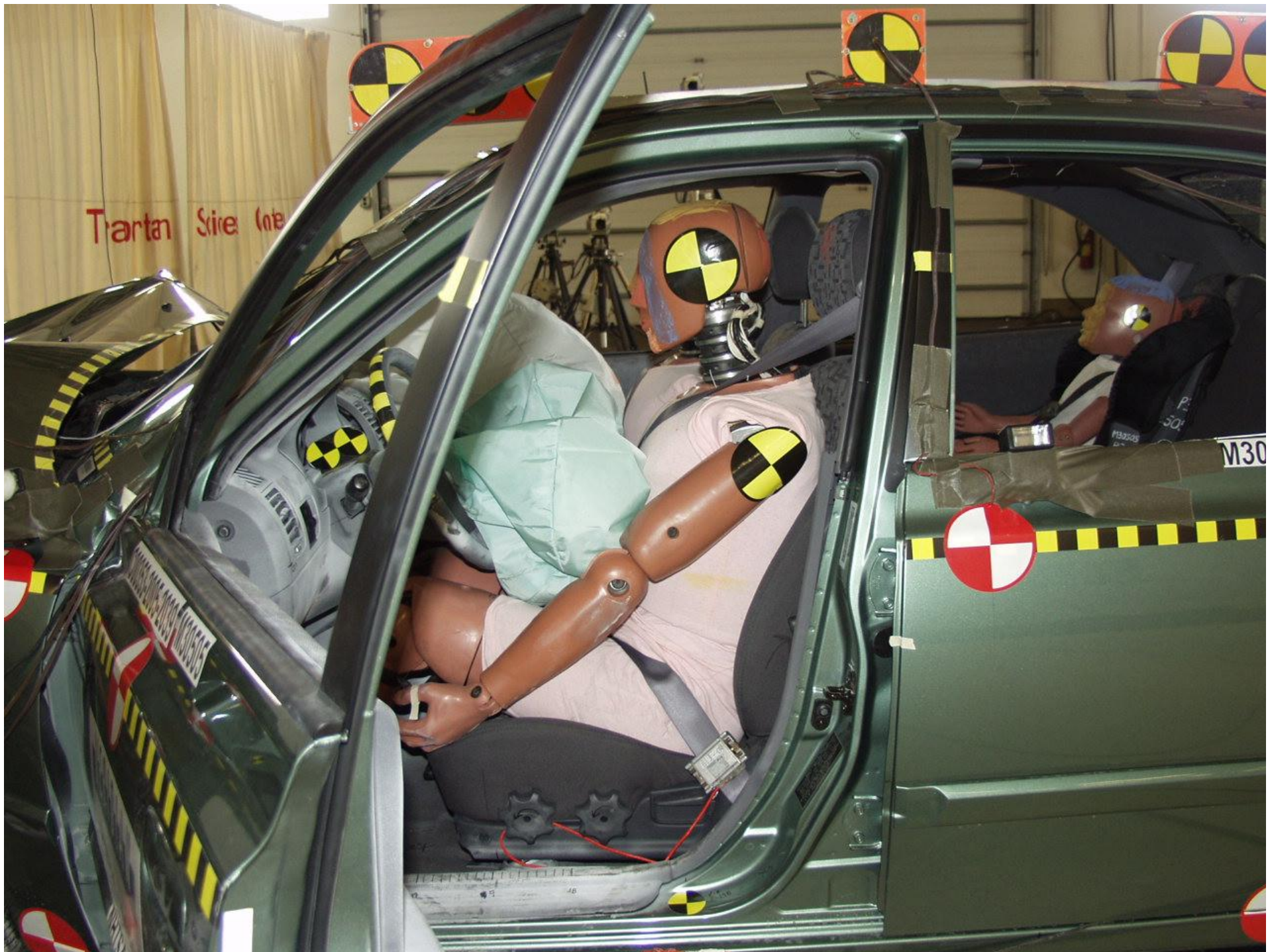
Figure A-35 POST-TEST DRIVER AND INTERIOR VIEW
