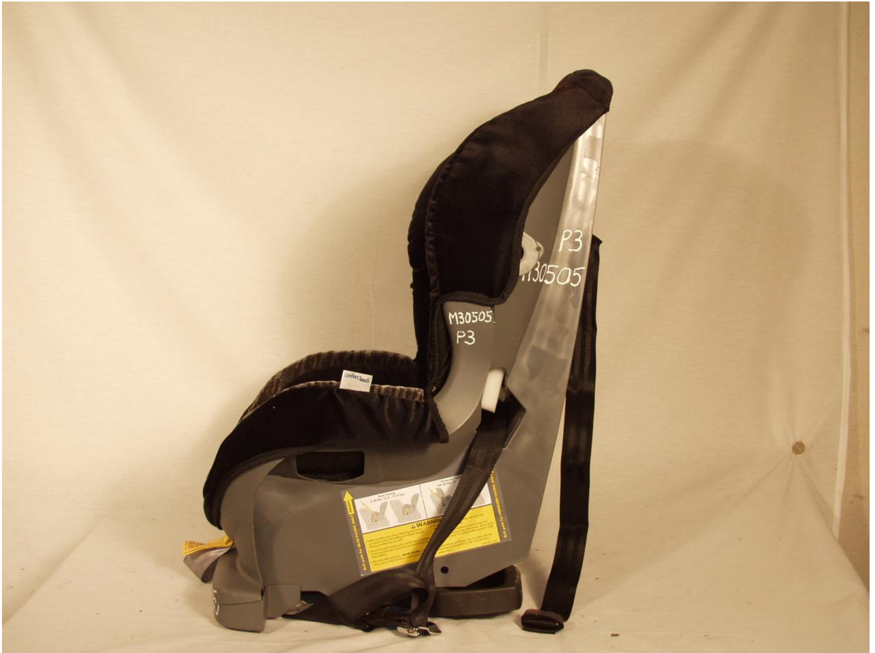
Figure 3-7: POST-TEST LEFT SIDE VIEW OF POSITION 3CRS
