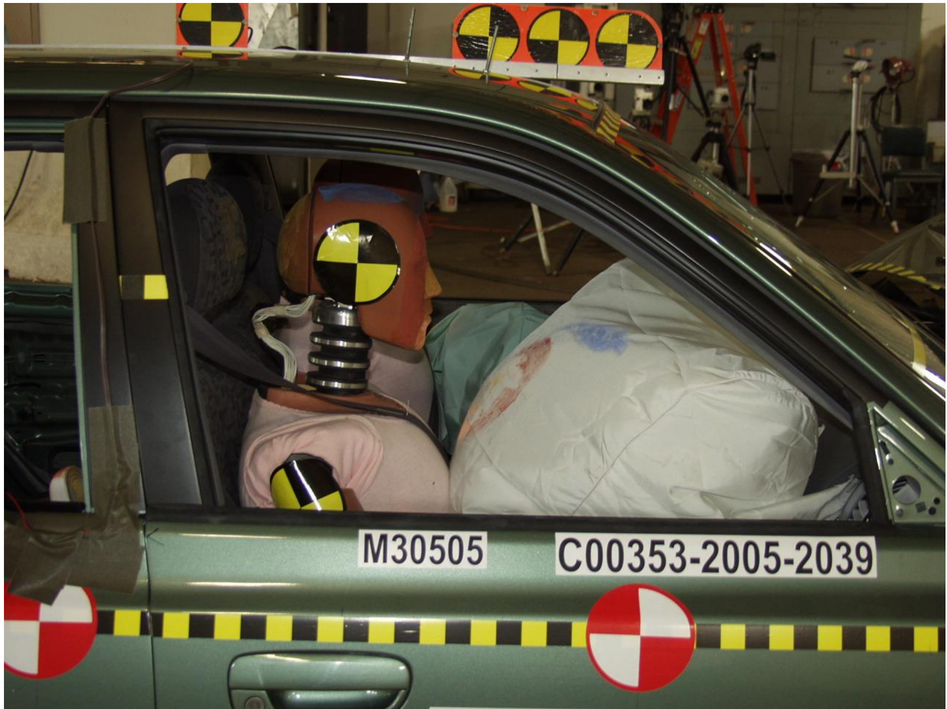
Figure A-47 POST-TEST PASSENGER POSITION VIEW
