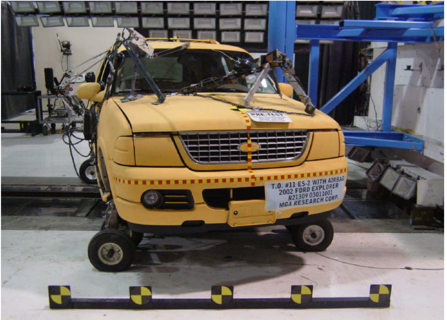
Pre-Test Vehicle Positioned Against Pole (left side)
