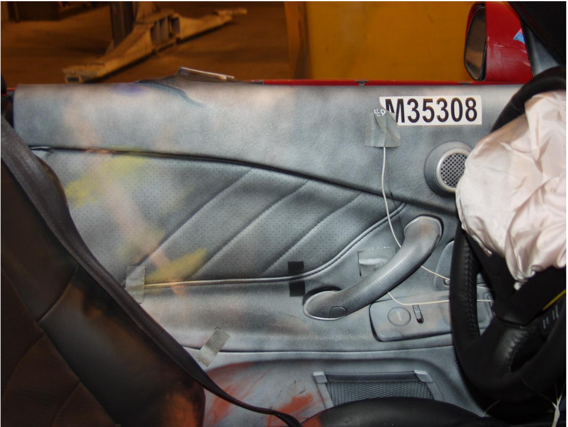
Figure A-34 POST-TEST INTERIOR OF FRONT DOOR SHOWING SID IMPACT LOCATIONS
