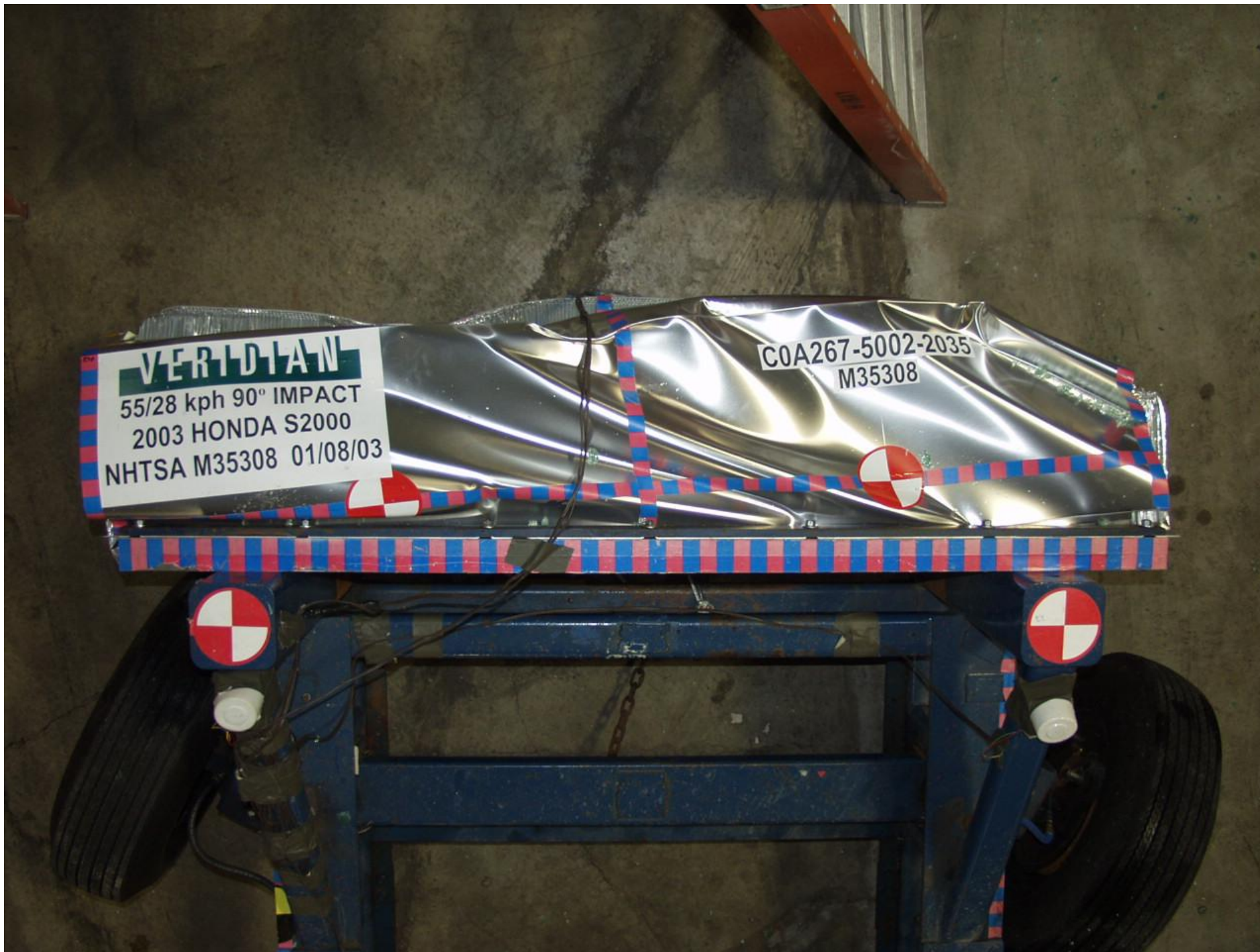
Figure A-22 POST-TEST TOP VIEW OF IMPACTOR FACE
